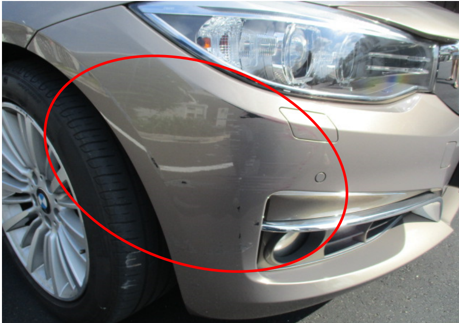
Photo 2 shows the paint graze marks found on the right portion of the BMW's front bumper (circled).
