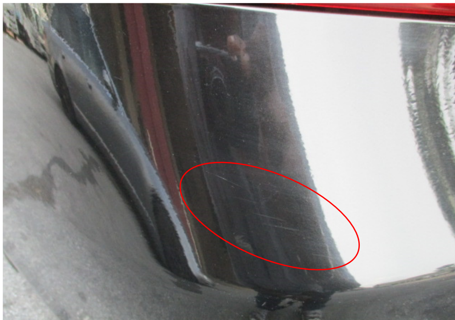
Photo 17 shows a closer view of the paint scratch marks found on the left portion of the Toyota's rear bumper (circled).
