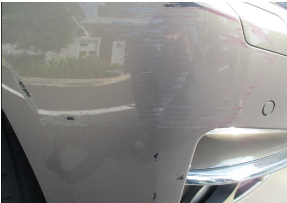
Photo 3 shows a closer view of the paint graze marks found on the right portion of the BMW's front bumper.
