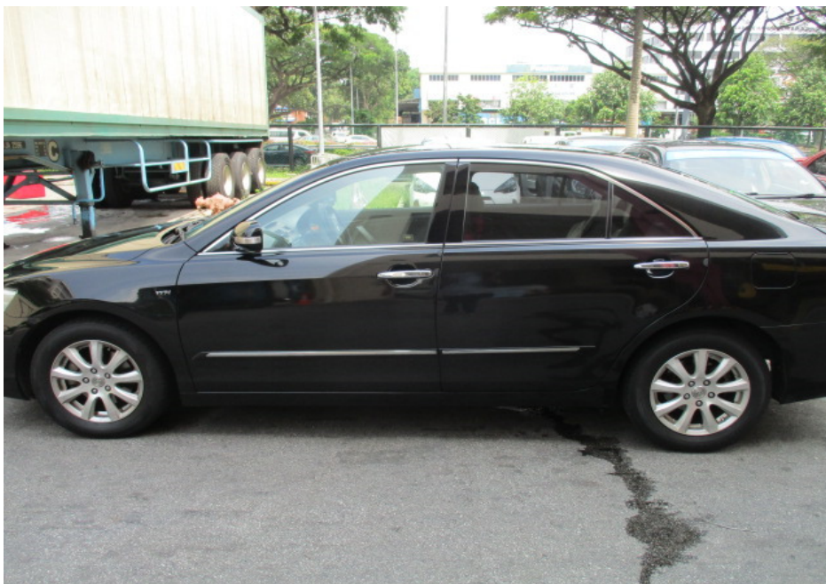
Photo 9 shows the general view of the Toyota's left portion at the time of inspection. Its left portion was observed to have sustained relatively minor impact damage, which had affected its left passenger door and rear bumper only.
