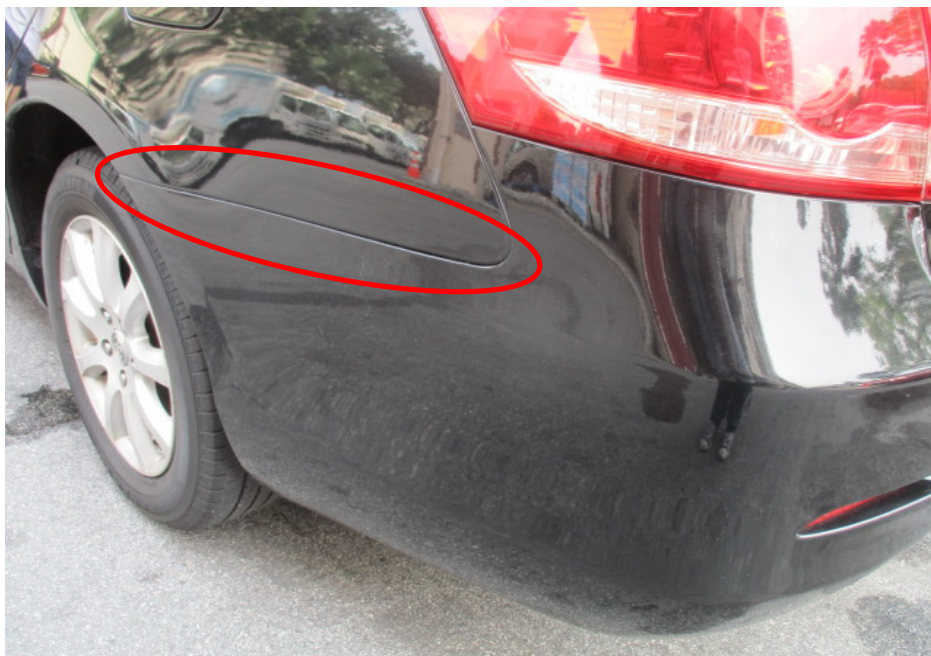
Photo 19 shows no obvious misalignment at the corner edges of the Toyota's rear bumper, adjacent to its rear left fender (circled). This would indicate that the impact onto the rear portion of the Toyota was relatively light.
