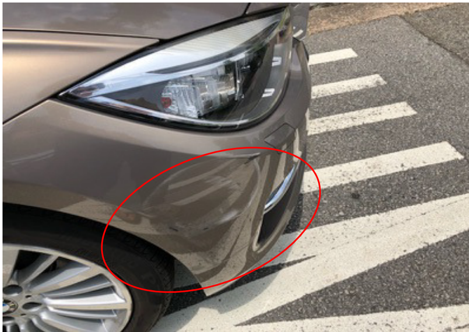
Photo 7 shows a closer view of the condition of the BMW's front bumper as depicted in the photographs that were taken by Ms Tan post- accident. The same paint graze marks on the right front portion of the BMW were observed (circled).
