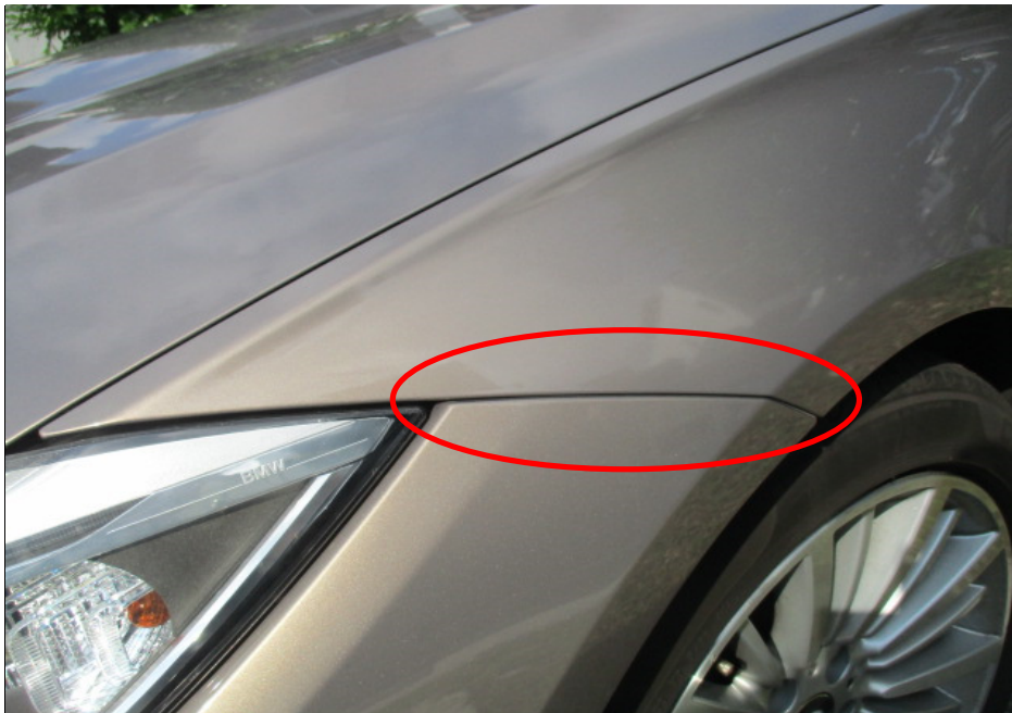
Photo 5 shows no obvious misalignment at the corner edges of the BMW's front bumper, adjacent to its front left fender (circled). This would indicate that the impact onto the frontal portion of the BMW was relatively light.
