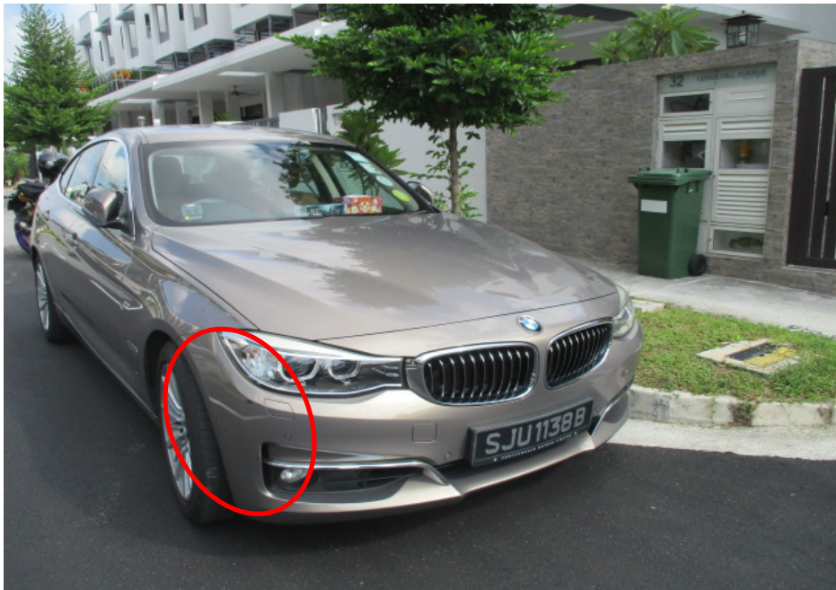
Photo 1 shows the general right view of the front of the BMW at the time of our inspection. Its right frontal portion was observed to have sustained relatively minor impact damage, which had affected its front bumper (circled).
