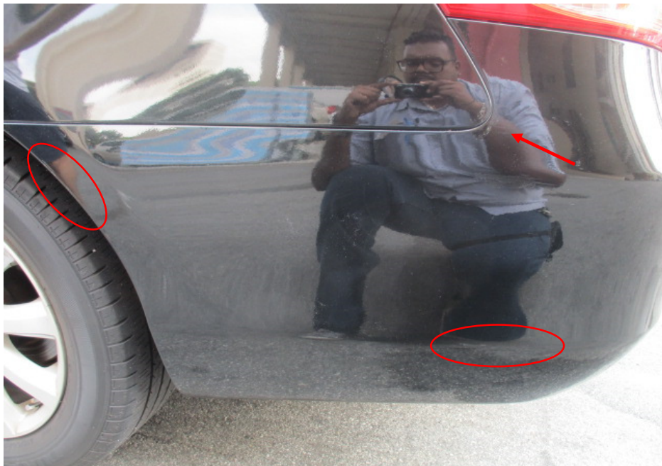
Photo 12 shows the paint scratch marks (arrowed) and paint graze marks (circled) found on the left rear portion of the Toyota, on the rear bumper.
