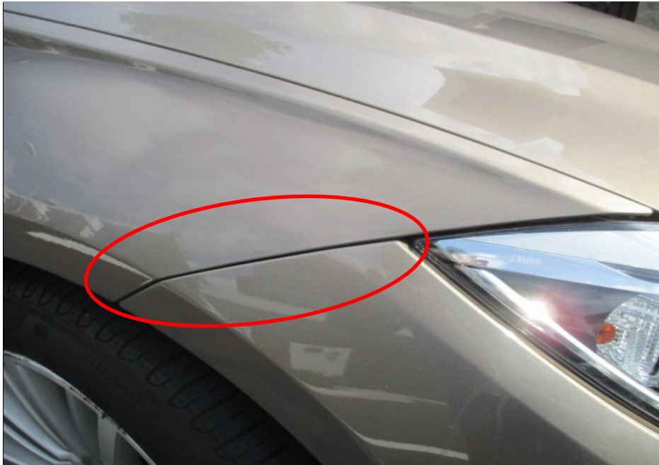
Photo 4 shows no obvious misalignment at the corner edges of the BMW's front bumper, adjacent to its front right fender (circled). This would indicate that the impact onto the frontal portion of the BMW was relatively light.
