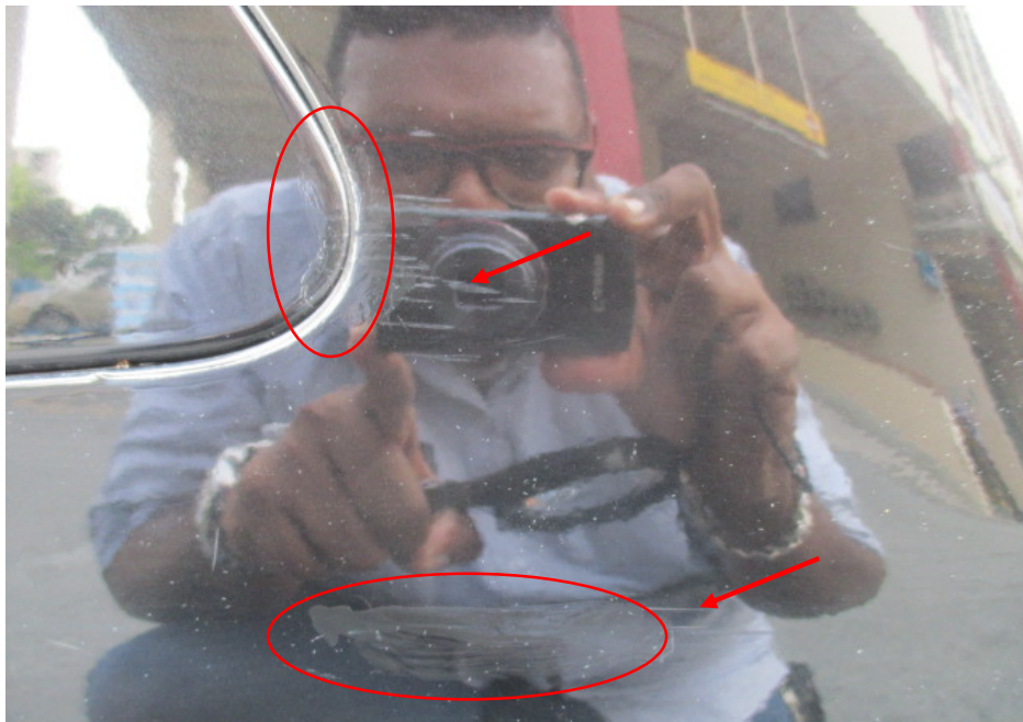
Photo 16 shows upon closer examination, we observed that several areas around the paint scratch marks (arrowed) had been painted over (circled).
