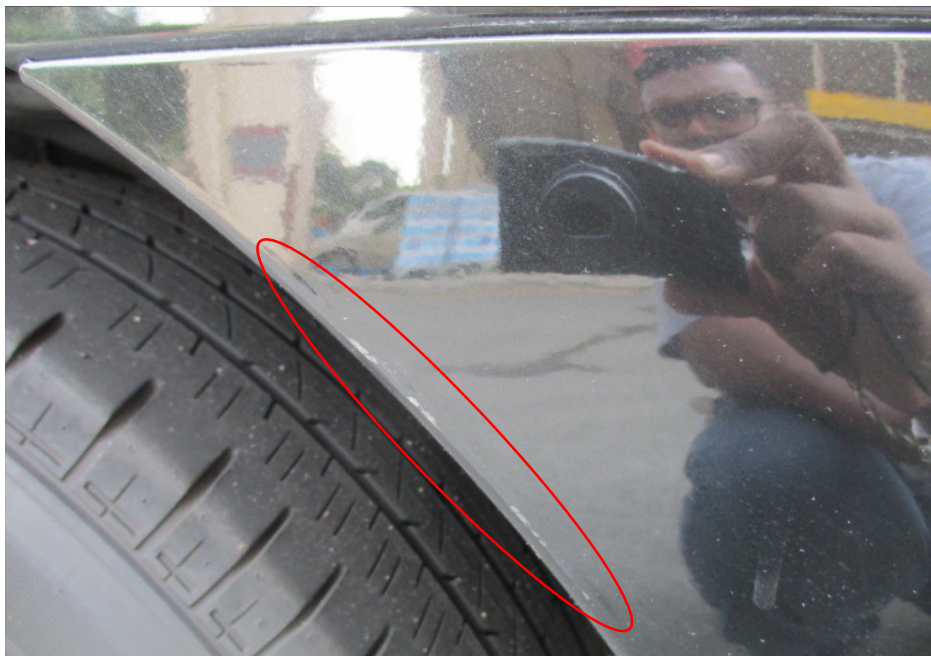
Photo 13 shows a close up view of the paint graze marks (circled) found on the left rear portion of the Toyota, on the rear bumper.
