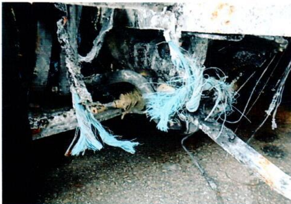
Photo 7 shows a closer view of the wirings of the Insured Vehicle, which were found with greenish residue. The presence of such greenish residue indicates internal heating of copper wires, a sign of an electrical short circuit occurring. This would then indicate that the fire to the Insured Vehicle was due to electrical nature.
