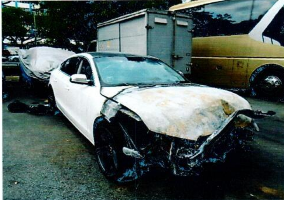
Photo 1 shows a general view of the front right body of the Insured Vehicle at the time of my inspection. The Insured Vehicle was observed to have sustained extensive fire damage at its frontal portion. Its front bumper, front bonnet, front right headlamp and front right fender were amongst the body parts that were observed to have been burnt.
