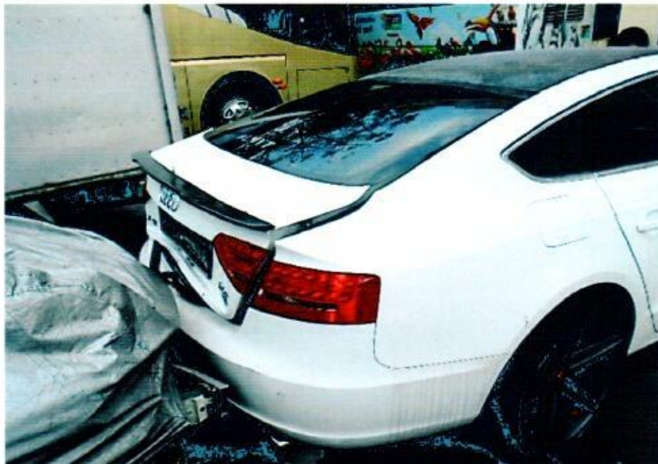
Photo 3 shows the rear body of the Insured Vehicle, which was unaffected by the fire. Its rear tailgate was however observed to be dented due to rescue operation.
