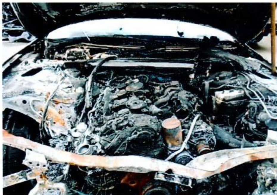
Photo 4 shows the engine compartment of the Insured Vehicle at the time of my inspection. The various parts and components inside the engine compartment were observed to have been severely burnt. This had included the intake manifold, fuel rail, belting, exhaust manifold and various hoses/pipes.
