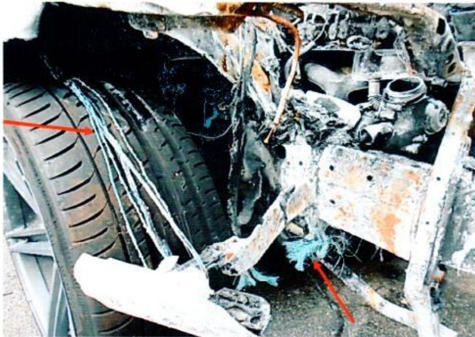
Photo 6 shows the wirings at the front right side of the engine compartment. I had found greenish residue on several stretches of wirings (arrowed) around this area of the engine compartment. Such greenish residue indicates internal heating of copper wires, a sign of an electrical short circuit occurring.
