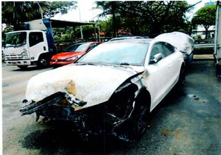
Photo 2 shows a general view of the front left body of the Insured Vehicle. The damage of fire nature was confined to the frontal portion of the Insured Vehicle. Its front bumper, front bonnet, front left headlamp, front left fender and front windscreen were amongst the body parts that were observed to have been burnt.
