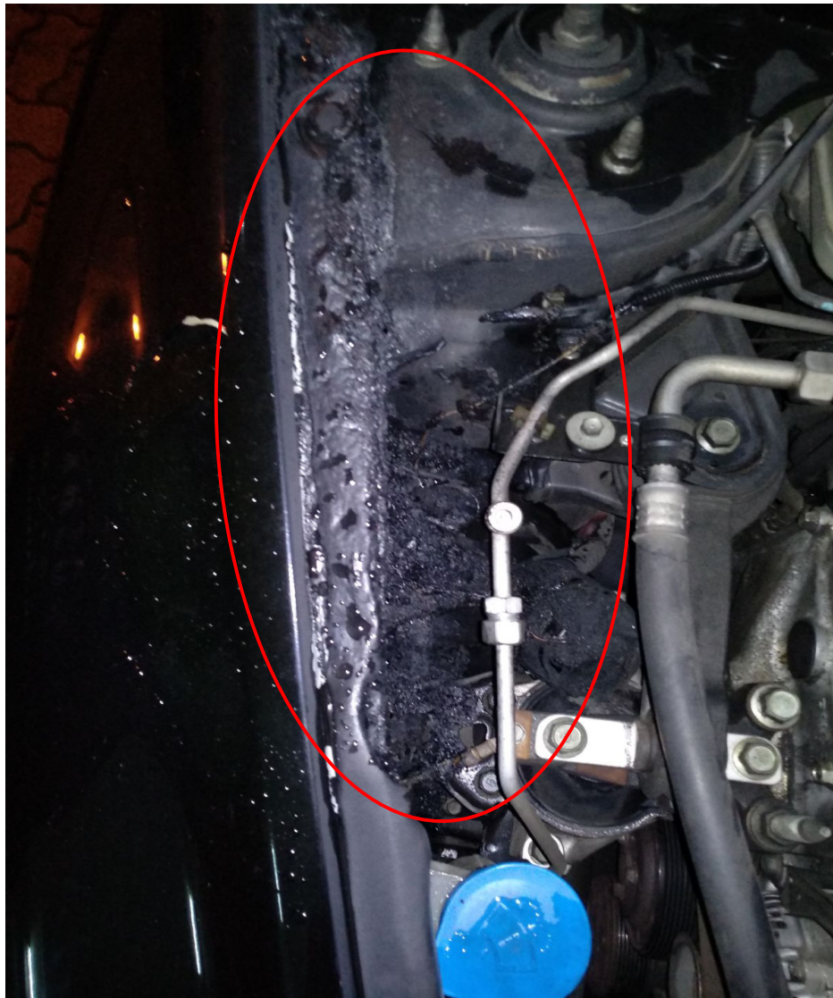
Photo 25 shows the Insured Vehicle after the fire was put out. In general, the information that could be gathered from this photograph had corresponded to the events that were related to us by Mr Kasim, which is the fire started from the right portion of the engine compartment of the Insured Vehicle (circled).
