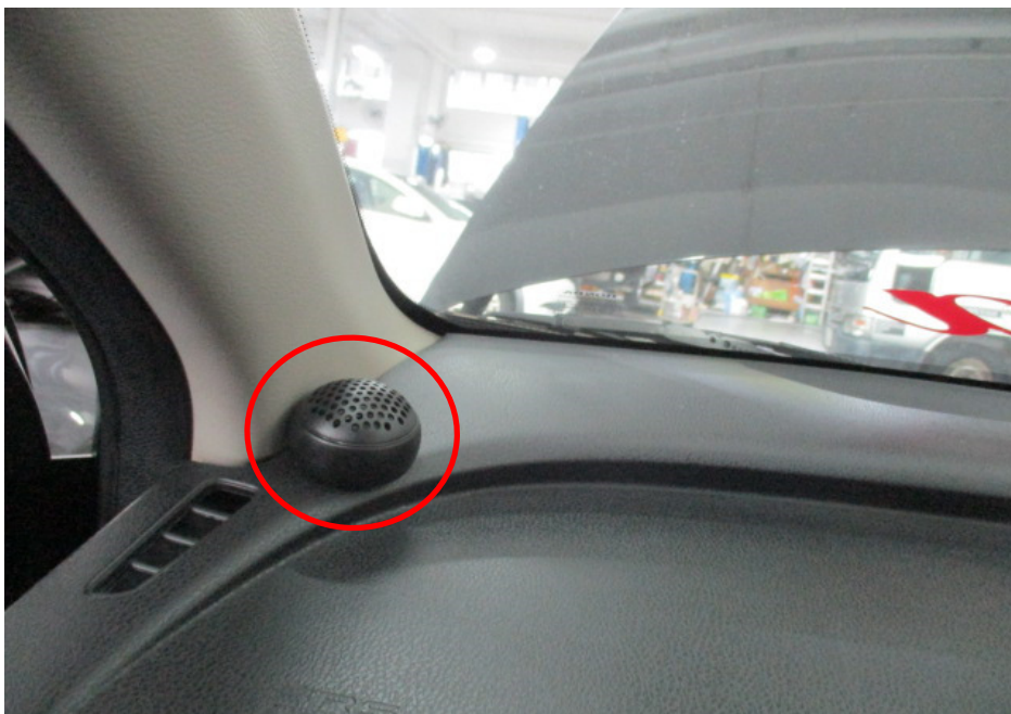
Photo 9 shows the 2nd aftermarket twitter fitted onto the left corner of the dashboard of the Insured Vehicle upon our inspection (circled).
