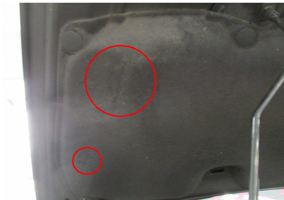
Photo 16 shows a closer view of the cracks as well as discolouration found on the insulating material on the underside of the right portion of the bonnet of the Insured Vehicle (circled) due to prolonged exposure to high heat intensity.
