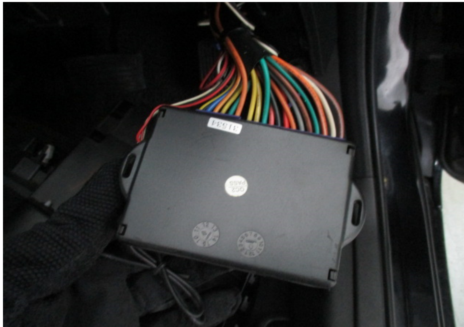
Photo 7 shows the aftermarket vehicular alarm system which is not the standard type for the Insured Vehicle.
