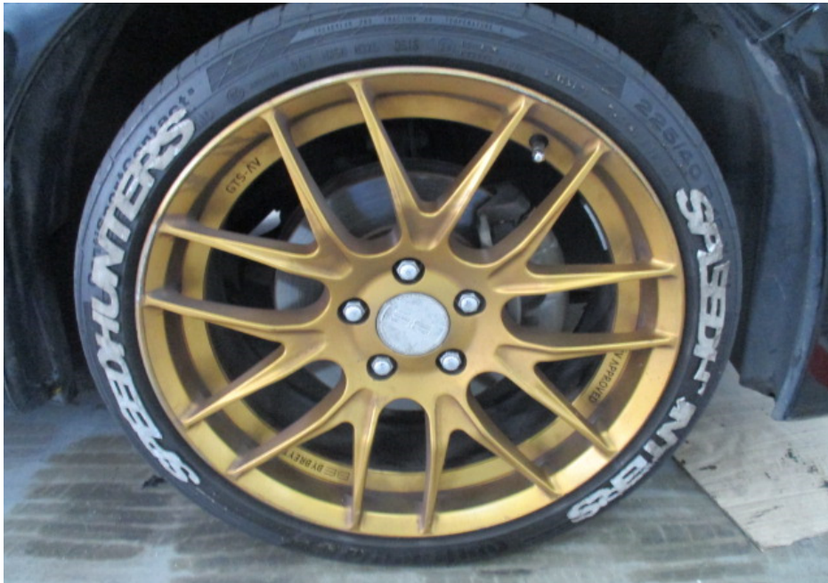
Photo 14 shows the non-standard rim and tyre found to be fitted on the Insured Vehicle at the time of our inspection. The 18- inch alloy rims fitted on the Insured Vehicle were not the standard type for the Insured Vehicle.
