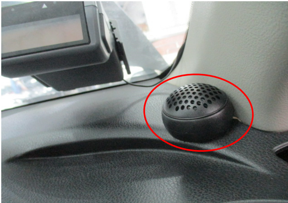
Photo 8 shows the 1st aftermarket twitter fitted onto the right corner of the dashboard of the Insured Vehicle upon our inspection (circled).
