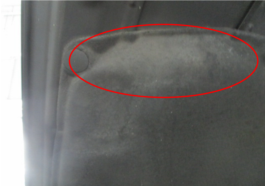
Photo 17 shows faint whitish burn marks on the underside of the right portion of the bonnet (circled) of the Insured Vehicle due to prolonged exposure to high heat intensity upon our closer examination.
