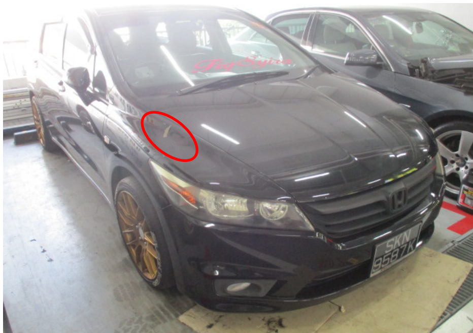
Photo 2 shows the general view of the right portion of the Insured Vehicle at the time of our inspection. The right portion of the Insured Vehicle was relatively unaffected by the fire except for the right side panel which was observed to be partially burnt and/or melted (circled).
