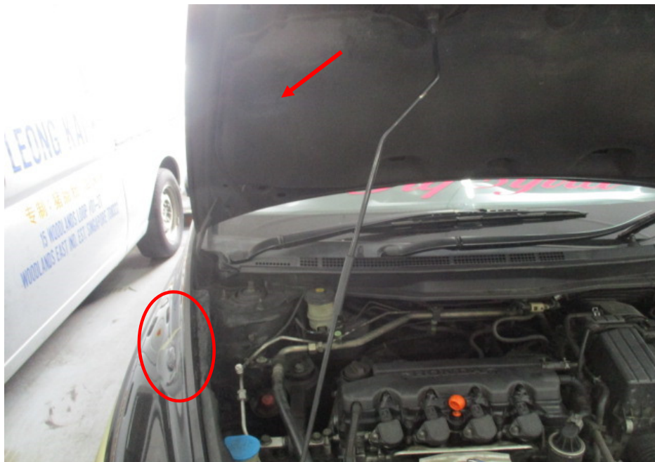
Photo 15 shows the cracks as well as discolouration found on the insulating material on the underside of the right portion of the bonnet (arrowed) due to prolonged exposure to high heat intensity. We also observed paint bubbles on the right side panel of the Insured Vehicle (circled).
