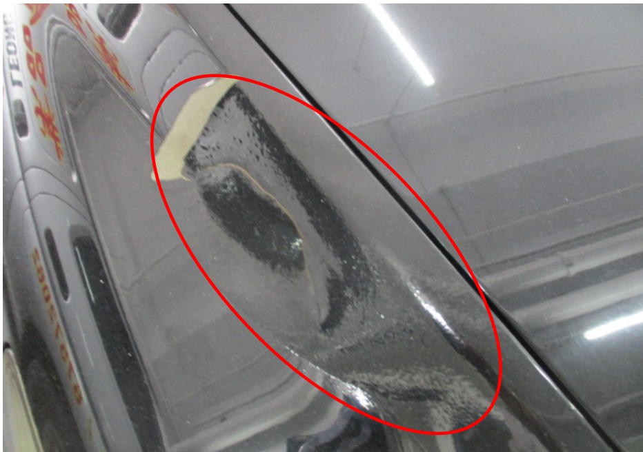
Photo 18 shows paint bubbles on the right side panel of the Insured Vehicle (circled).
