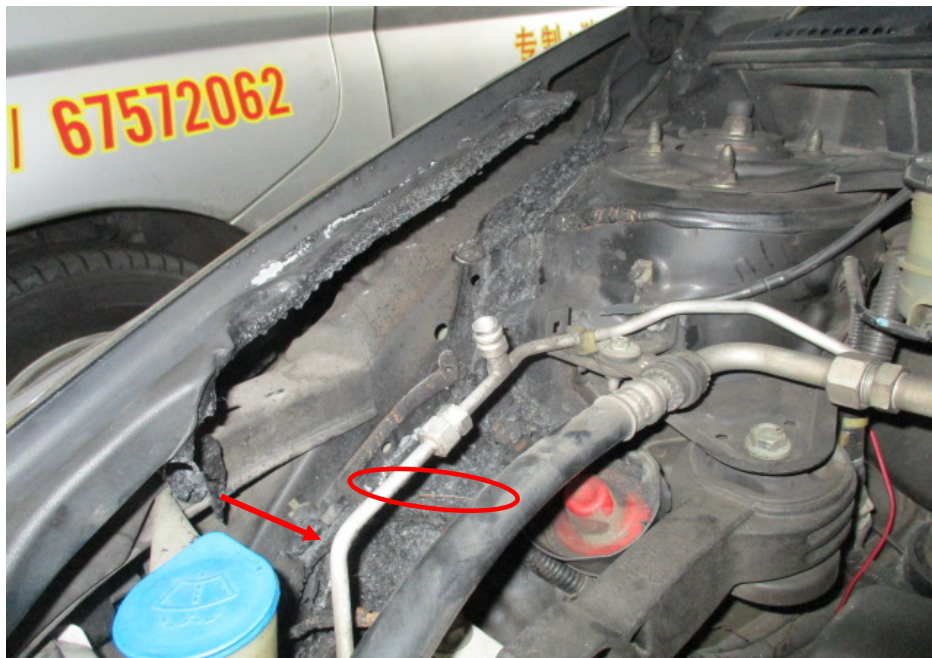
Photo 19 shows the stretches of burnt wirings from the wiring harness (arrowed) as well as the wiring leading from the vehicular alarm horn (circled). We noticed faint traces of greenish residue on some of these wirings.
