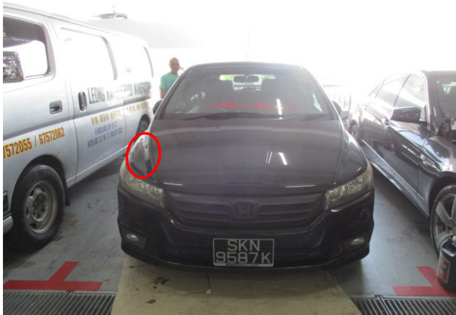
Photo 1 shows the general view of the front portion of the Insured Vehicle at the time of our inspection. The exterior body of the Insured Vehicle was relatively unaffected by the fire except for the right side panel which was observed to be partially burnt and/or melted (circled).
