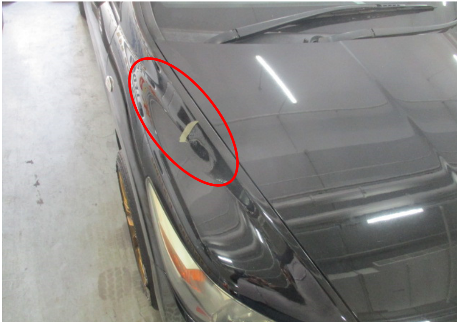
Photo 3 shows a closer view of the right side panel of the Insured Vehicle which was observed to be partially burnt and/or melted (circled).
