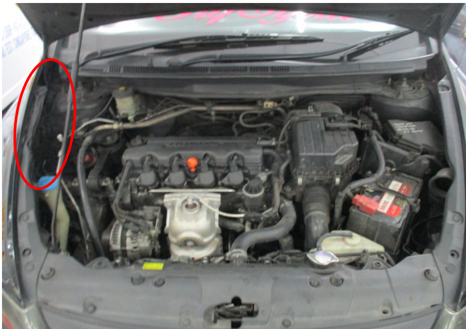
Photo 4 shows a general view of the engine compartment of the Insured Vehicle at the time of our inspection. The main engine compartment of the Insured Vehicle did not sustain any visible fire damage except for the wiring harness located at the right portion (circled).
