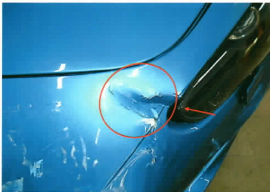
Photo 8 shows a closer view of the dents, paint cracks and graze marks on the left portion of the Insured Vehicle's front bumper (circled). There was also a slight crack on the left headlight (arrowed).
