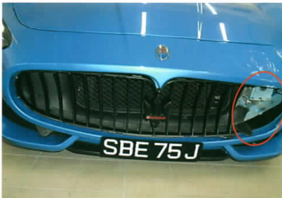
Photo 7 shows a closer view of the Insured Vehicle's buckled front grille (circled).
