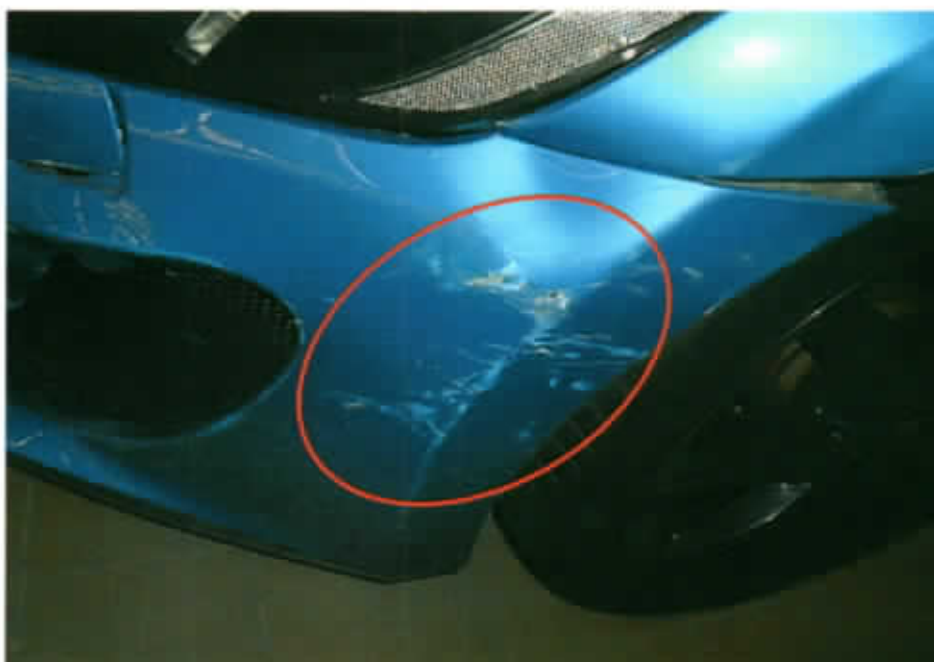
Photo 9 shows several bluish paint transfer marks observed on the left portion of the Insured Vehicle's front bumper (circled) which would appear to correspond to the Insured Vehicle being hit by the Taxi.
