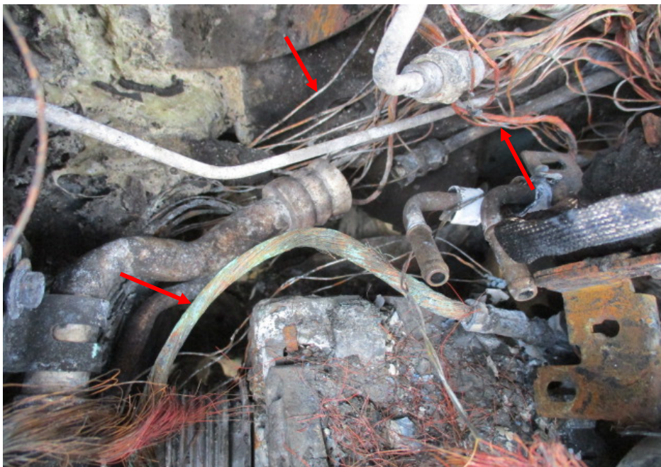
Photo 10 shows a close up view of the greenish residue found on some of the burnt stretches of original factory fitted wirings (circled). The presence of such greenish residue suggests occurrence of an electrical short circuit.
