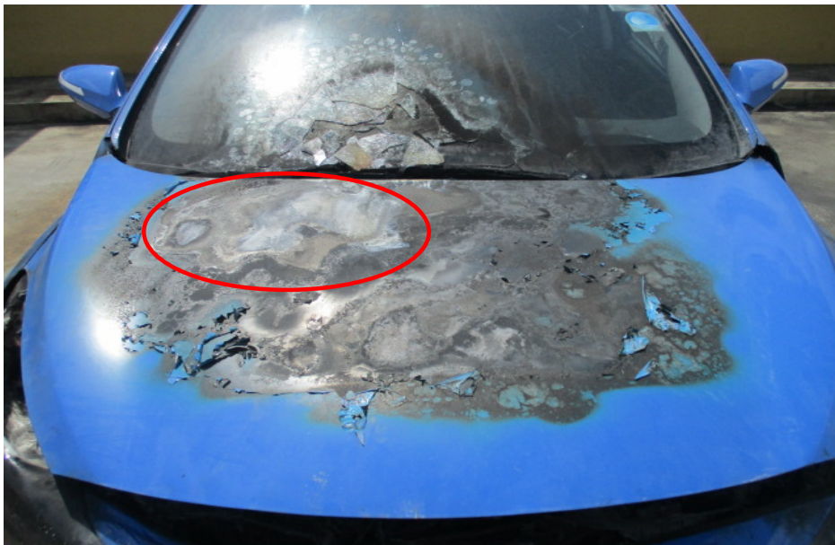
Photo 5 shows the burn pattern and whitish burn marks that were found on the rear right portion of the front bonnet of the Insured Vehicle (circled). Such whitish burn marks are a result of exposure to prolonged heat intensity, which may indicate where the fire had started. Rust would also begin to develop on these areas soon after the fire.
