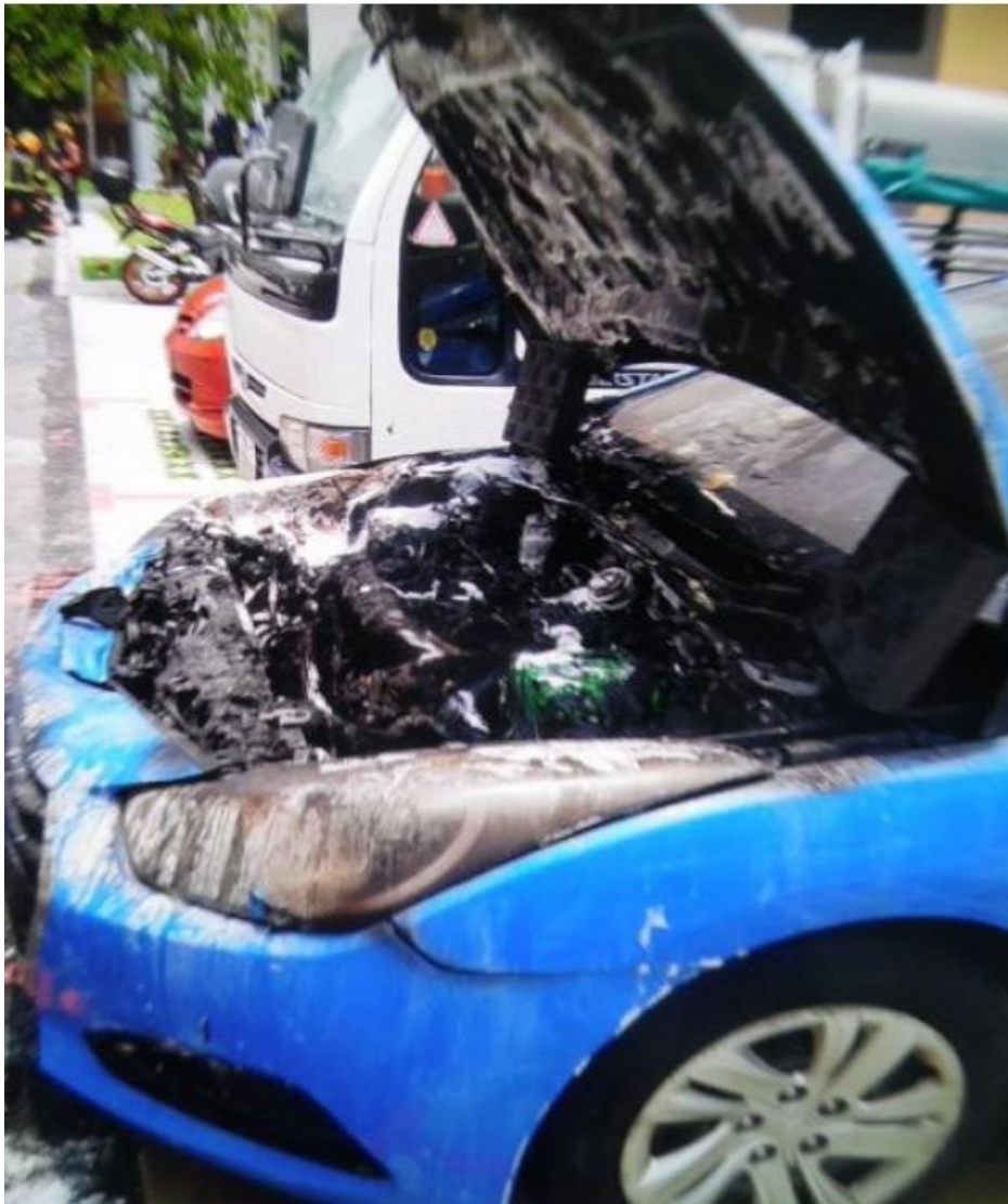
Photo 16 shows the Insured Vehicle in the parking lot after the fire was extinguished. Our close examination of this photograph showed no unusual foreign material(s) and/or object(s) found on the ground in the immediate area of the lot where the Insured Vehicle was parked.
