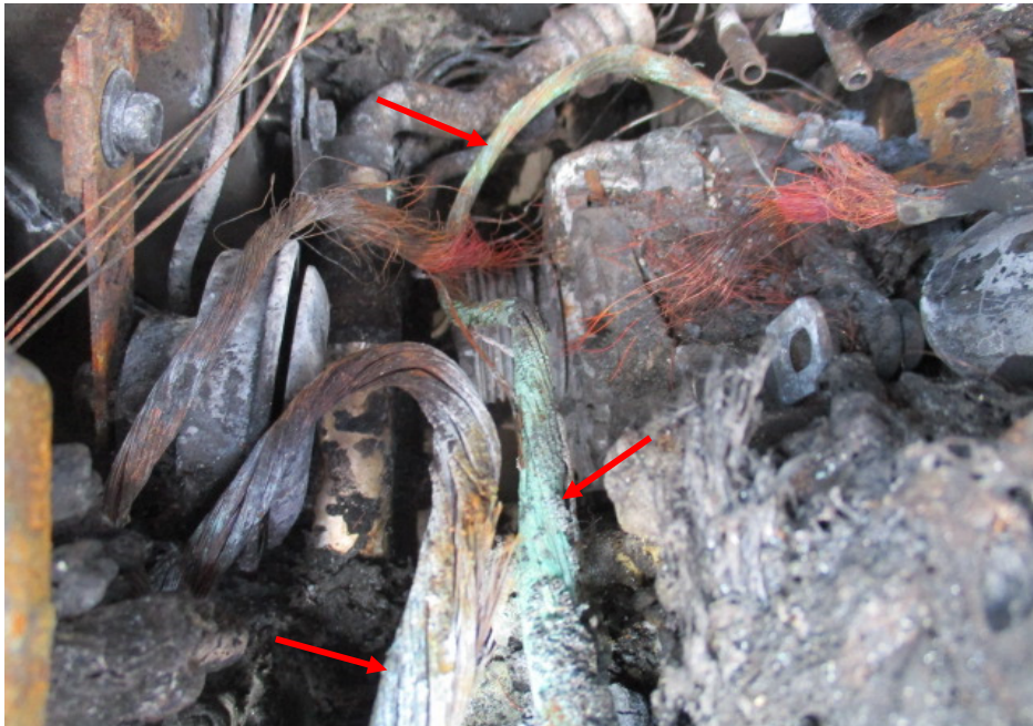
Photo 9 shows a close up view of the greenish residue found on some of the burnt stretches of original factory fitted wirings (arrowed). The presence of such greenish residue suggests occurrence of an electrical short circuit.
