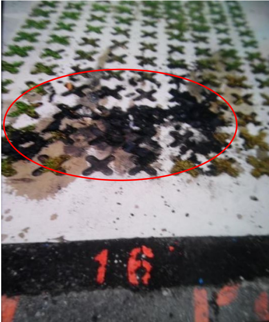
Photo 15 shows the burnt marks and/or burnt residual remains on the ground of the lot where the Insured Vehicle was parked (circled), taken after the Insured Vehicle was towed to CDGE. Our close examination of this photograph showed no unusual foreign material(s) and/or object(s) found on the ground in the lot where the Insured Vehicle was parked at the material time of incident.
