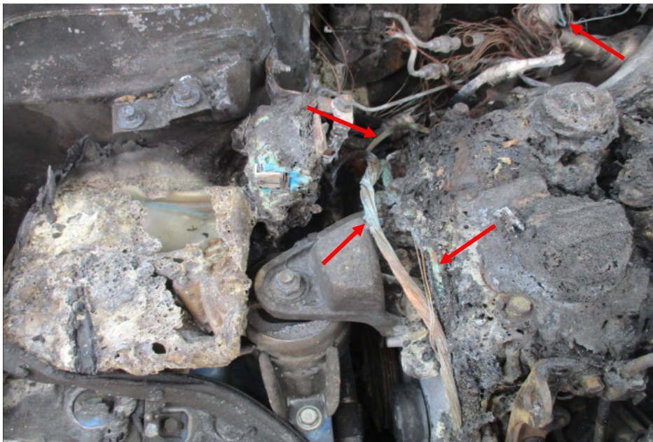
Photo 8 shows a closer view of the greenish residue found on some of the burnt stretches of original factory fitted wirings (circled). The presence of such greenish residue suggests occurrence of an electrical short circuit.
