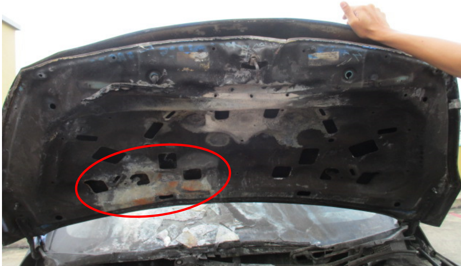
Photo 6 shows the rust that had developed on the underside of the front bonnet, around the bottom right portion (circled). The development of rust is an indication that this area was subjected to prolonged exposure to high heat intensity, which had caused the steel/metal material of the front bonnet to be exposed to natural environmental condition. Hence the fire to the Insured Vehicle can be determined to have originated towards the rear right portion of the engine compartment.
