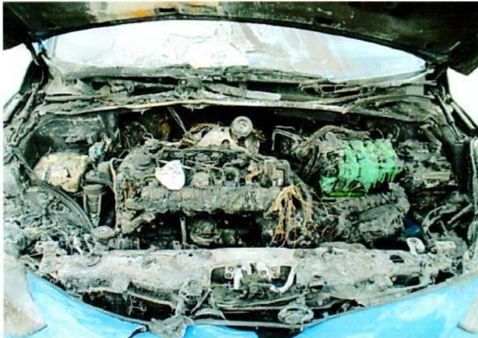
Photo 3 shows the engine compartment of the Insured Vehicle at the time of our inspection. The entire engine compartment of the Insured Vehicle was observed to be severely burnt. Most of the parts inside the engine compartment were found to be burnt and/or melted as a result of the fire.
