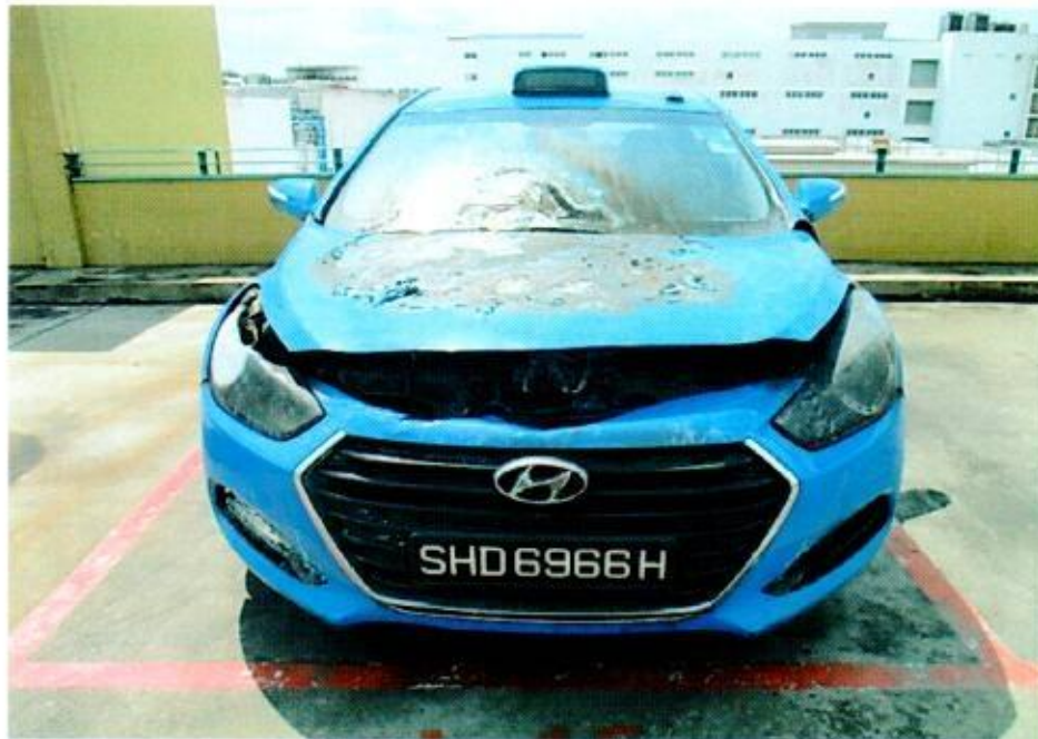
Photo 1 shows the general view of the front portion of the Insured Vehicle at the time of our inspection. The fire damage to the Insured Vehicle was confined to its front portion. Its front bumper, front bonnet, front grille, front windscreen and front headlamps were amongst the body parts that were found to have been affected as a result of the fire.
