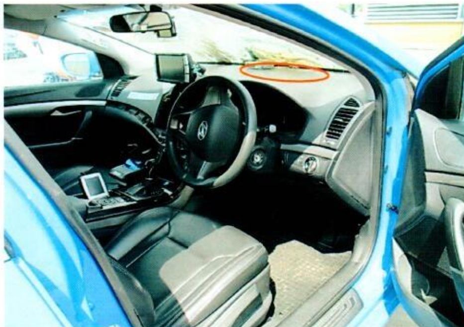
Photo 4 shows the interior compartment of the Insured Vehicle which was relatively unaffected by the fire except for the centre portion of the dashboard panel which was observed to be partially burnt and/or melted (circled).
