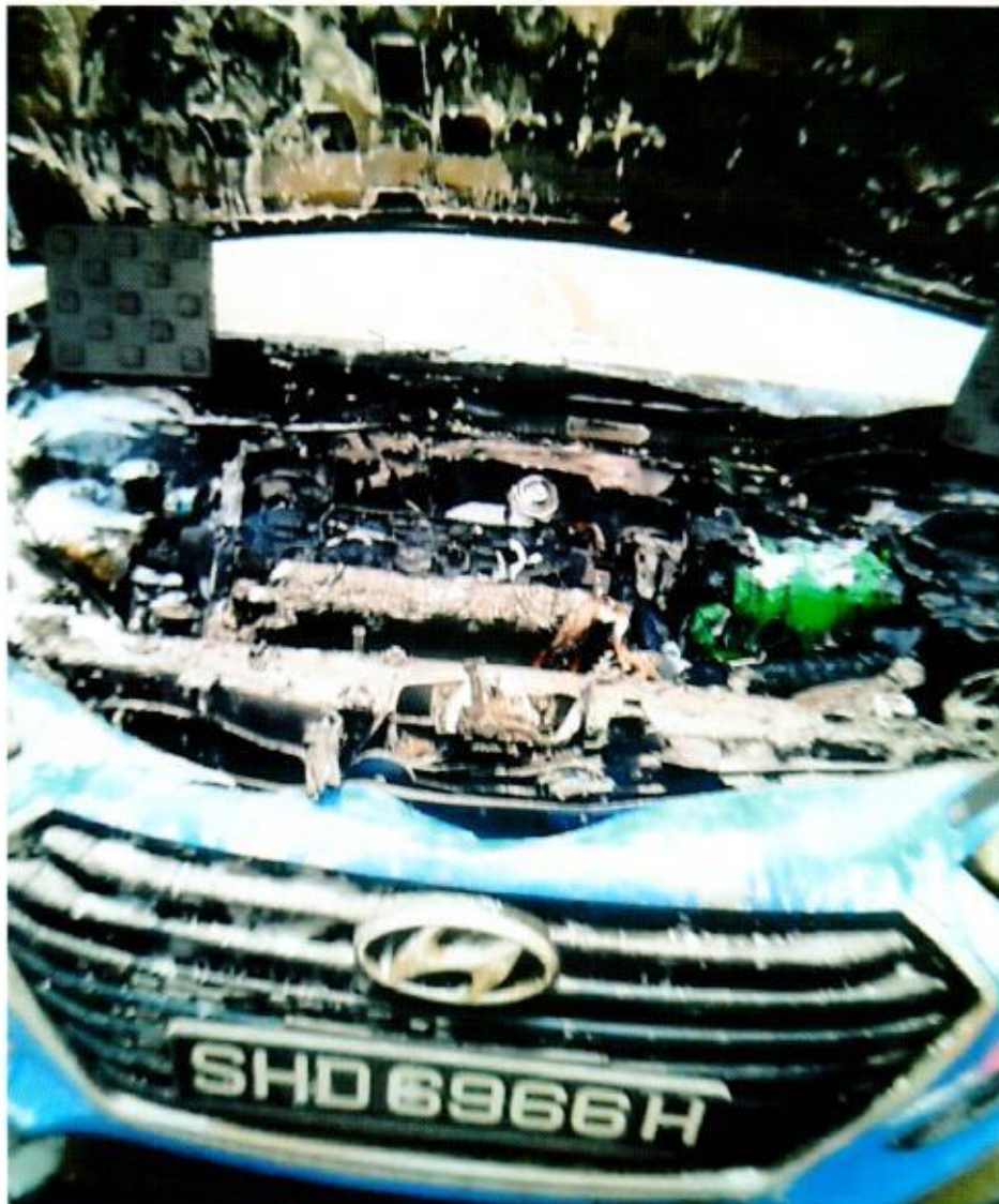
Photo 14 shows the engine compartment of the Insured Vehicle post- incident. In general, the damages sustained to the engine compartment and the fire extinguisher residue found all around the engine compartment had corresponded to the events that were related to us by Mr Toh, which is the fire had started from the engine compartment.
