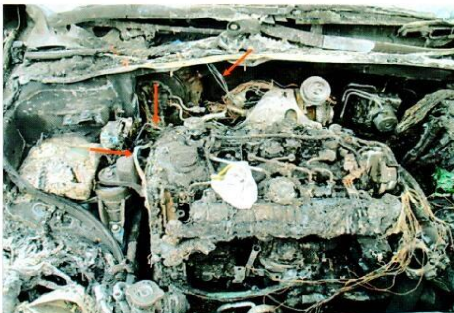
Photo 7 shows the original factory fitted wirings around the rear right portion of the engine compartment, which is in the immediate vicinity where the fire to the Insured Vehicle had likely started. We had found greenish residue on several burnt stretches of these wirings (arrowed). The presence of such greenish residue indicates internal heating of copper wires, a sign of an electrical short circuit occurring. The greenish residue is normally left behind from oxidation as a result of chemical reaction involving the copper wires.
