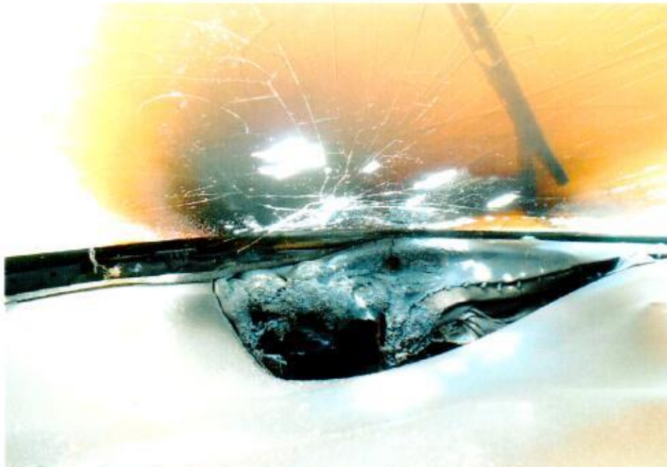
Photo 4 shows the interior compartment of the Insured Vehicle, which was observed to be partially burnt and/or melted. The front dashboard, front windscreen and roof upholstery were amongst the parts that were found to have been burnt and/or melted as a result of the fire.
