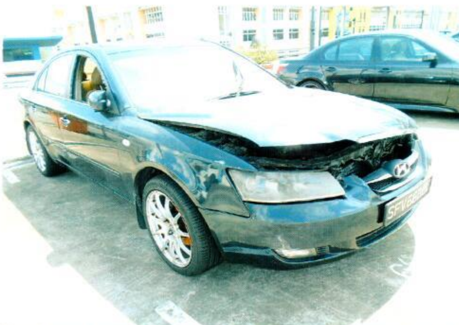
Photo 2 shows the general view of the front right portion of the Insured Vehicle at the time of our inspection. The fire damage to the Insured Vehicle was confined to its front portion. Its front bumper, front bonnet and front left headlamp were amongst the body parts that were found to have been affected as a result of the fire.
