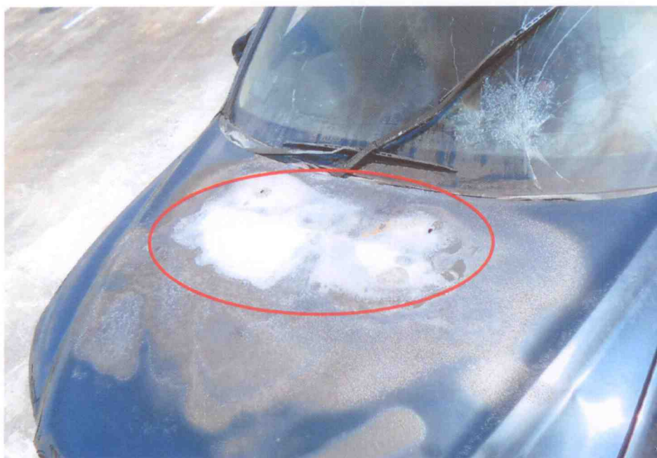
Photo 5 shows the burn pattern and whitish burn marks (circled) that were found on the top side of the front bonnet of the Insured Vehicle. Such whitish burn marks are a result of exposure to prolong heat intensity, which may indicate where the fire had started. Rust would also begin to develop on these areas soon after the fire.
