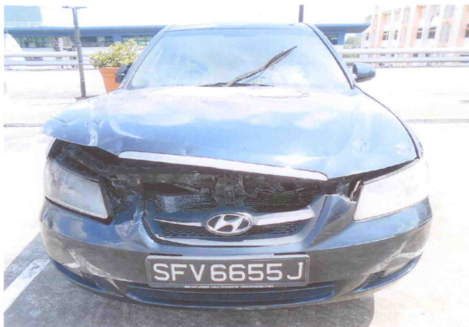
Photo 1 shows the general view of the front right portion of the Insured Vehicle at the time of our inspection. The fire damage to the Insured Vehicle was confined to its front portion. Its front bumper, front bonnet, front grille and front right headlamp were amongst the body parts that were found to have been affected as a result of the fire.
