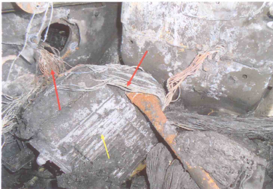
Photo 8 shows a closer view of the wirings (red arrow) which were found to have been burnt internally to its bare copper state, suggesting occurrence of an electrical short circuit. These wirings were observed to be leading to the Engine Control Module (yellow arrow) of the Insured Vehicle.
