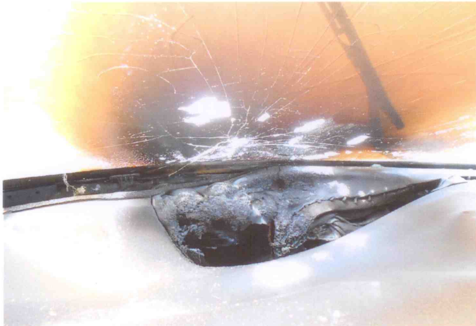
Photo 4 shows the interior compartment of the Insured Vehicle, which was observed to be partially burnt and/or melted. The front dashboard, front windscreen and roof upholstery were amongst the parts that were found to have been burnt and/or melted as a result of the fire.
