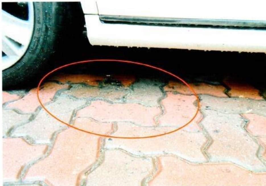
Photo 14 shows the close-up view of where the Insured Vehicle was parked at the time of incident. Further observations on the ground, we found burnt marks/ burnt residual on the red bricks at the parking lot. This reveals that there's evidence that fire incident happen at the said spot.
