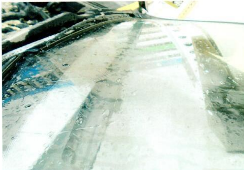
Photo 4 shows the windshield of the Insured Vehicle, which was observed to be cracked were amongst the parts that were found to have been damaged as a result of the fire.
