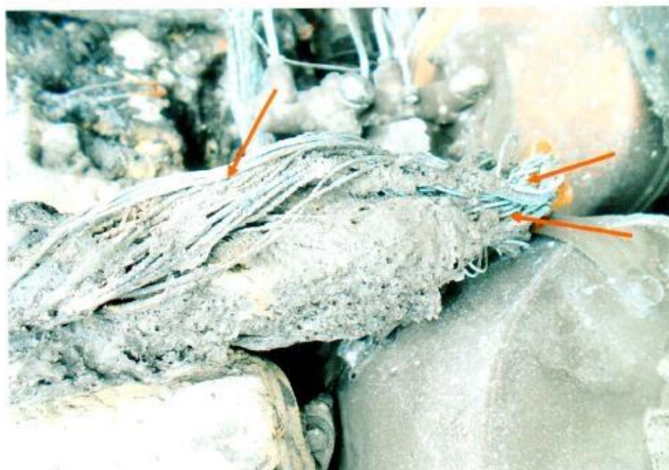
Photo 8 shows a closer view of the wirings (red arrow) which were found to have been burnt internally, suggesting occurrence of an electrical short circuit.
