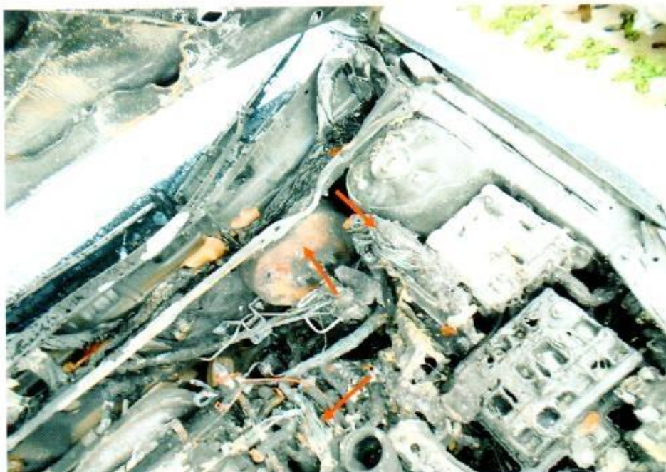
Photo 7 shows the wirings around the left rear of the engine compartment, which was in the immediate vicinity where the fire to the Insured Vehicle had likely started. The wirings (red arrow) were found to have been burnt internally, suggesting occurrence of an electrical short circuit. The wirings also appear to be an original engine wire harness of the insured vehicle.
