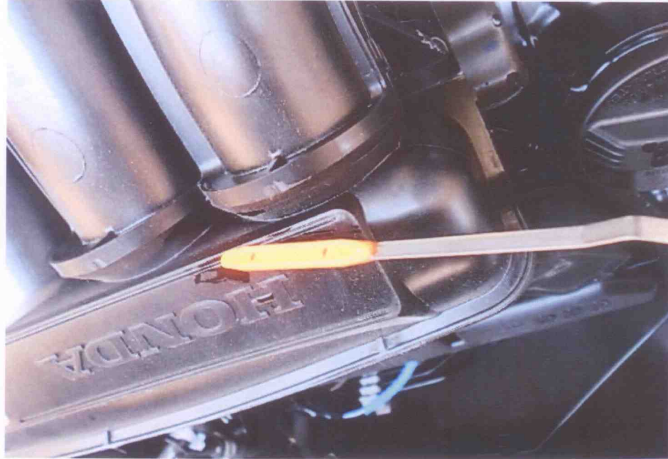
Photo 7 shows the engine oil dip stick of the Motor Car at the time of my inspection. The engine oil was observed to be of sufficient level and without any visible contamination.
