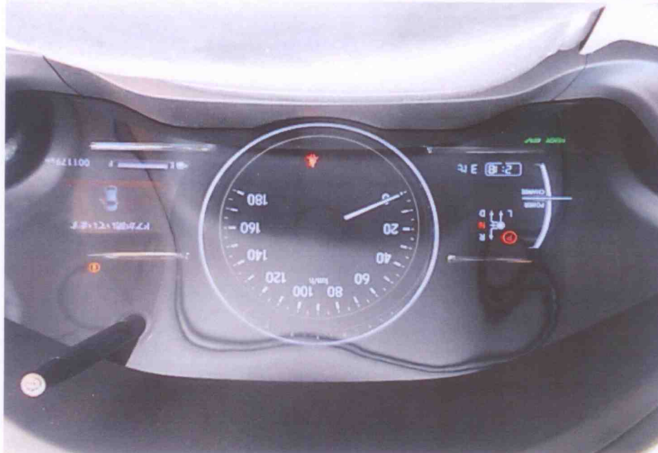
Photo 11 shows no warning lights illuminated on the instrument panel of the Motor Car after the engine was cranked. This would suggest that there was no abnormality to the various electronic operating systems of the motor car, like the ABS, EPS, TC and SRS etc.
