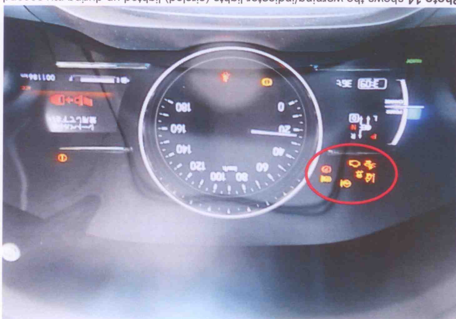
Photo 14 shows the warning/indicator lights (circled) lighted up during my second test drive of the Motor Car. During this second test drive, the Motor Car felt sluggish. The Motor Car had displayed a lack of power and was extremely slow even when the accelerator pedal was fully depressed. The air-conditioning system was also observed to be functioning intermittently ie blowing hot air with intermittent cool air.
