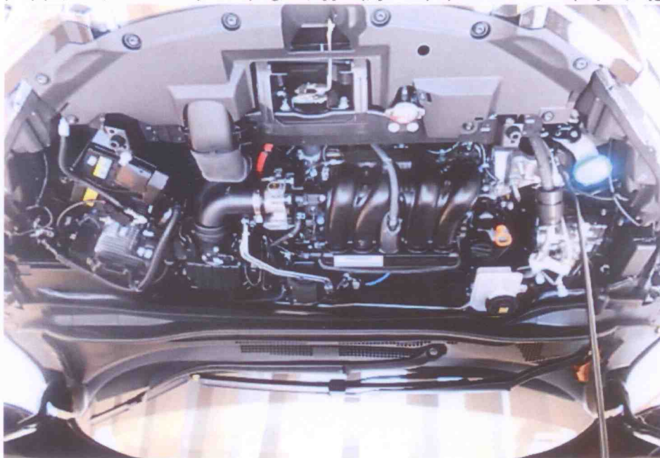
Photo 4 shows a general view of the Motor Car's engine compartment. I had observed that the various mechanical components, hoses and sensors were all intact and securely fitted/attached. The engine compartment was also observed to be relatively clean with no fluid stain(s) and/or fluid leak(s) found.
