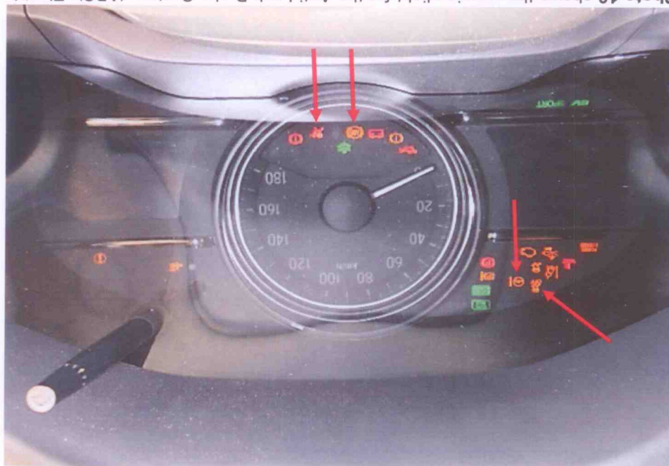
Photo 10 shows the warning light for the Anti-Lock Brake System (ABS), Electric Power Steering System (EPS), Traction Control (TC) and Supplemental Restraint System (SRS) appearing on the instrument panel of the Motor Car during the self-test of its various electronic operating systems when its engine was cranked.
