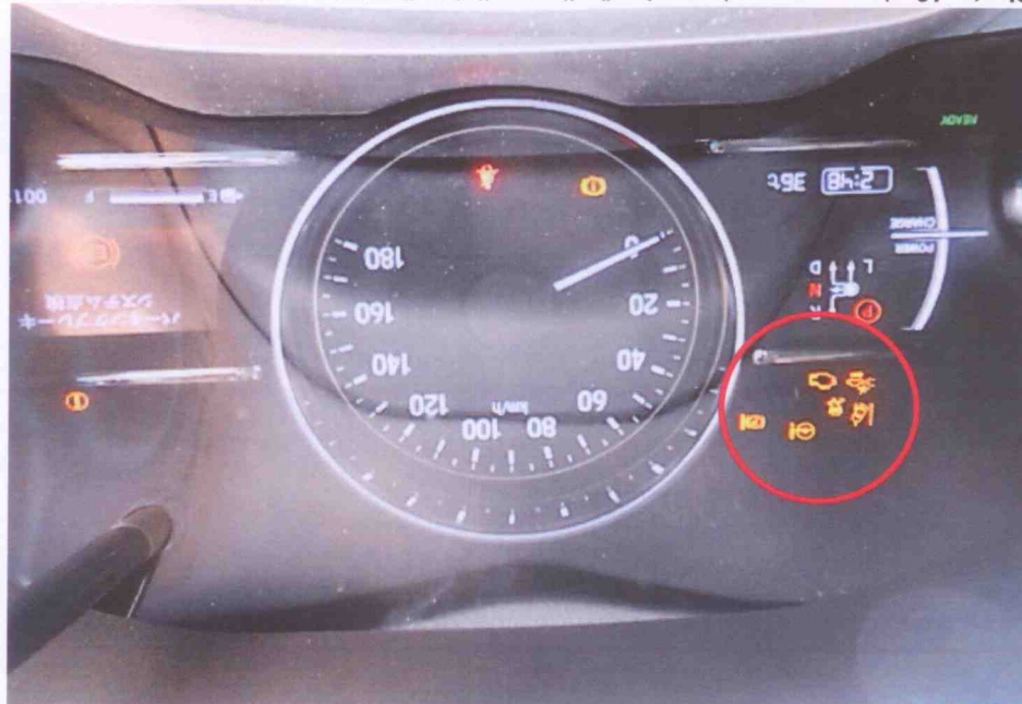
Photo 13 shows several warning/indicator lights lighted up. These lights (circled) had abruptly came on whilst the Motor Car was idling after my test drive. These lights were the warning/indicator light for the engine system, collision mitigation braking system, vehicle stability assist, electric power steering and road departure mitigation system. The lights had remained lighted up after I had turned off and restarted the engine of the Motor Car.
