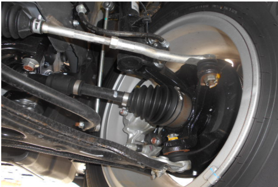
Photo 9 shows the various undercarriage components at the front right wheel of the Motor Car. The undercarriage components of the Motor Car were all observed to be intact and without any visible damage.
