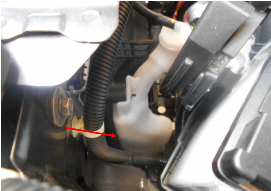
Photo 6 shows the engine coolant reservoir of the Motor Car at the time of my inspection. The engine coolant was observed to be of sufficient level (arrowed) and without any visible contamination.
