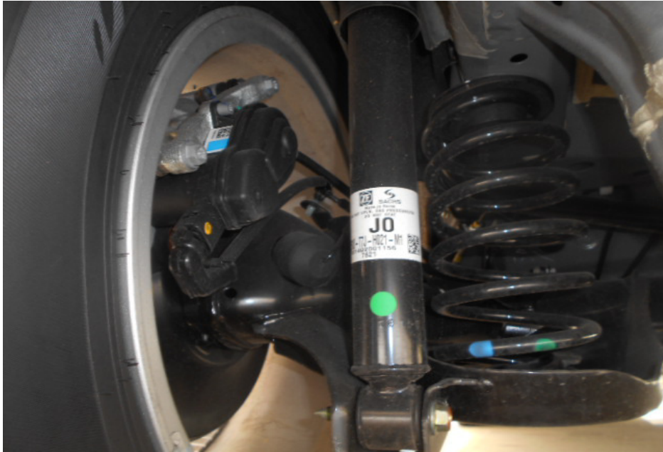
Photo 8 shows the various undercarriage components at the rear left wheel of the Motor Car. The undercarriage components of the Motor Car were all observed to be intact and without any visible damage.
