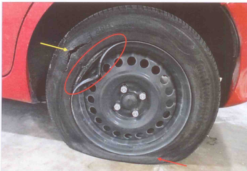
Photo 7 shows a close up view of the buckled left rear wheel rim (circled) and punctured left rear tyre (red arrow) which was most probably caused by a sharp protruding object from the motorcycle which in this case may be the right pillion foot peg. As the right pillion foot peg hit the sidewall of the left rear tyre of the Insured Vehicle while the left rear tyre was in rotation, the impact caused a tear in the sidewall, puncturing the left rear tyre (yellow arrow) followed by the buckling of the wheel rim, resulting in the wheel rim cover to be dislodged from the left rear wheel rim.
