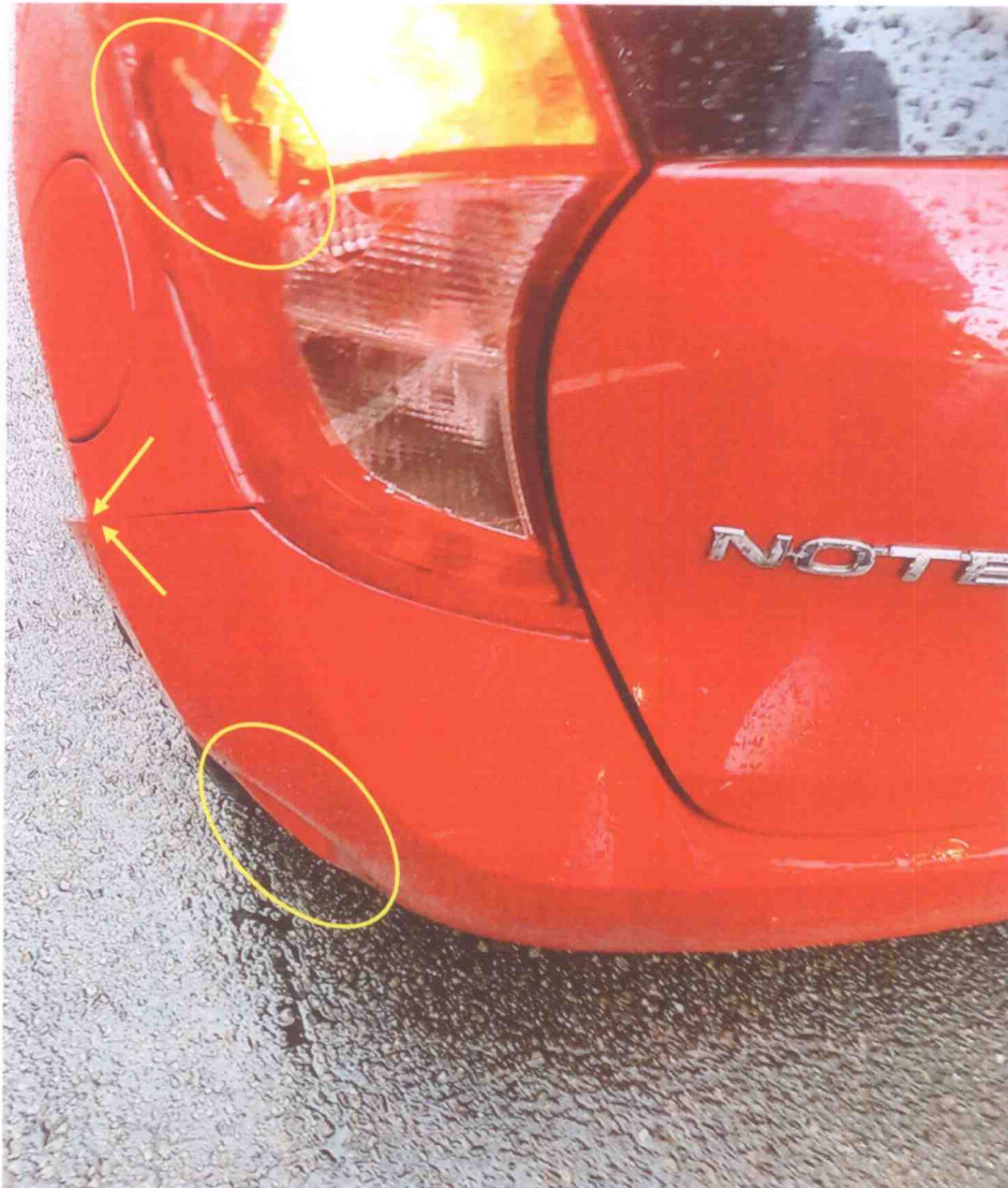
Photo 2 taken by Mr Shariff shows the misalignment of the rear bumper at the left corner edge (arrowed), the cracked left tail light and the dent on the lower left portion of the rear bumper of the Insured Vehicle (circled). The damages sustained to the Insured Vehicle seems to correlate with Mr Jabbar's statement where he could not slow down the motorcycle in time and hit the left rear portion of the Insured Vehicle. Our observation of Mr Shariff's ability to take clear post-accident photographs would suggest that there was no drink driving involved in this particular accident.
