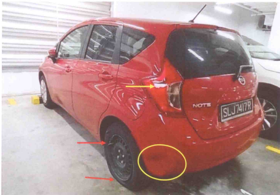
Photo 4 shows the left rear view of the Insured Vehicle during the accident reporting at TCM which was taken 4 days after the accident occurred. We observed a crack on the left tail light (yellow arrow), a dent on the lower left portion of the rear bumper (circled), a buckled rear left wheel rim and punctured rear left tyre (red arrows). The damages sustained to the Insured Vehicle seem consistent with the circumstances of the accident, where the left rear portion was hit by a motorcycle.
