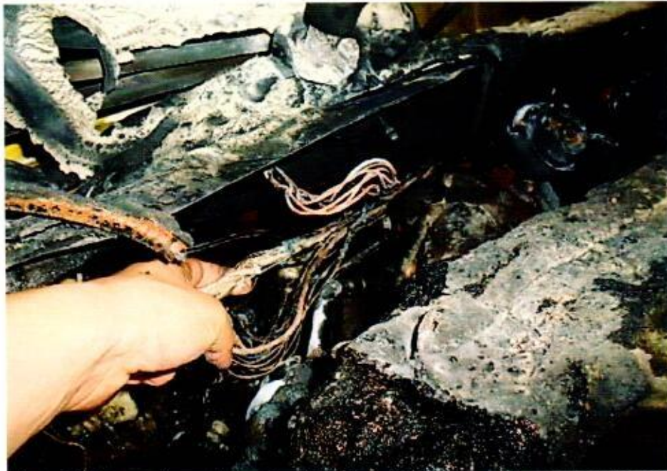
Photo 9 shows a closer view of another stretch of wirings at the rear centre area of the Insured Vehicle's engine compartment. The bright reddish colour of the copper wires suggest that the wirings were exposed to high heat. Such condition normally indicates internal heating of copper wires which is a sign of an electrical short circuit occurring. This would then appear to suggest that the cause of fire to the Insured Vehicle could have possibly been due to electrical in nature.
