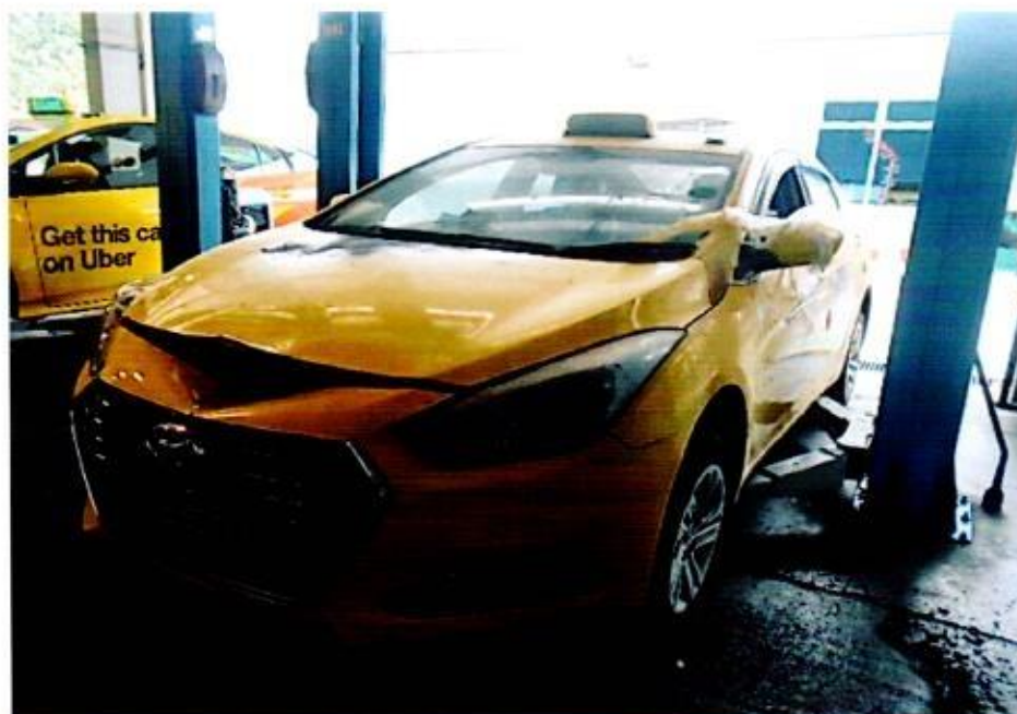
Photo 2 shows a general view of the front left body of the Insured Vehicle at the time of my inspection. The fire had affected most of the parts within the engine compartment. The mileage of the Insured Vehicle could not be recorded due to its wirings being affected by the fire.
