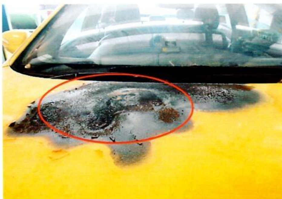
Photo 5 shows the burned marks (circled) that were found on the top side of the Insured Vehicle's front bonnet. Apart from these burned marks, there were no other marks of burnt nature found on the exterior body of the Insured Vehicle. Given this single burn mark on the exterior body, the fire can then be established to have originated within the engine compartment of the Insured Vehicle, somewhere around the rear centre of the engine compartment.
