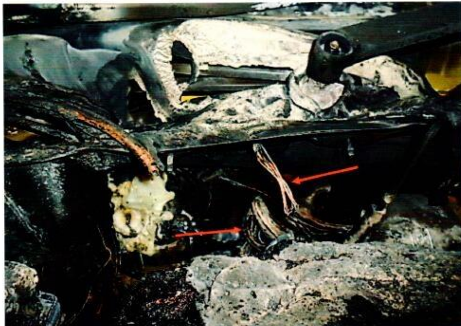
Photo 7 shows the wirings at the rear centre area of the Insured Vehicle's engine compartment, which was where the fire had originated. The wirings (arrowed) were found to be completely burned to its bare copper state. The bright reddish colour of the copper wires suggest that the wirings were exposed to high heat. Such condition normally indicates internal heating of copper wires which is a sign of an electrical short circuit occurring. The wires were likely to be original factory fitted wire harnesses of the Insured Vehicle.
