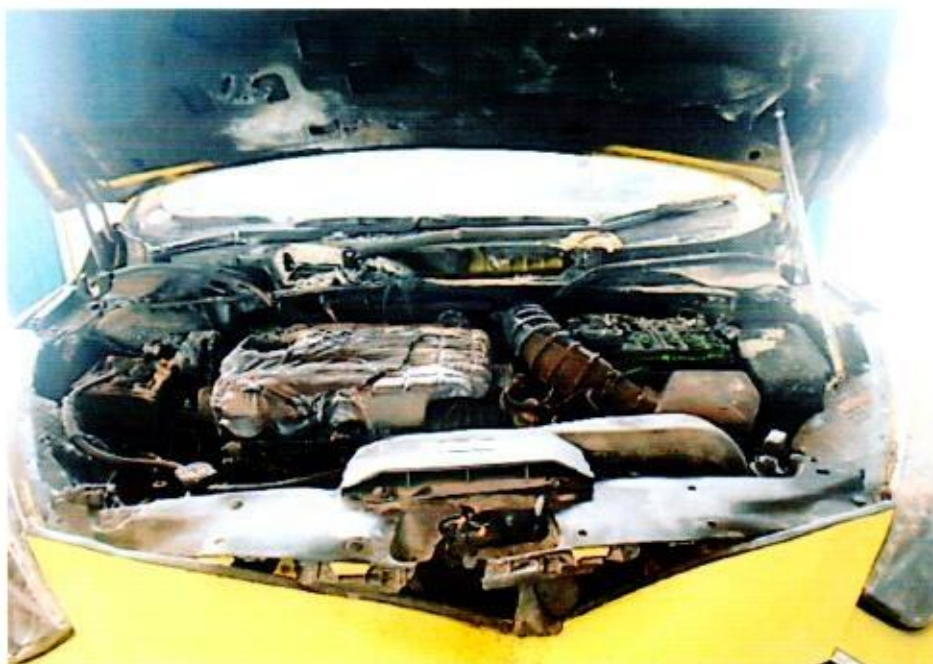
Photo 3 shows a general view of the Insured Vehicle's engine compartment at the time of my inspection. The engine compartment was observed to have sustained moderate fire damage. Parts that were made of plastic or rubber type material were observed to be partially melted. This had included the various rubber hoses, wiper panel, battery, air intake duct, bonnet insulator and brake fluid reservoir amongst others.
