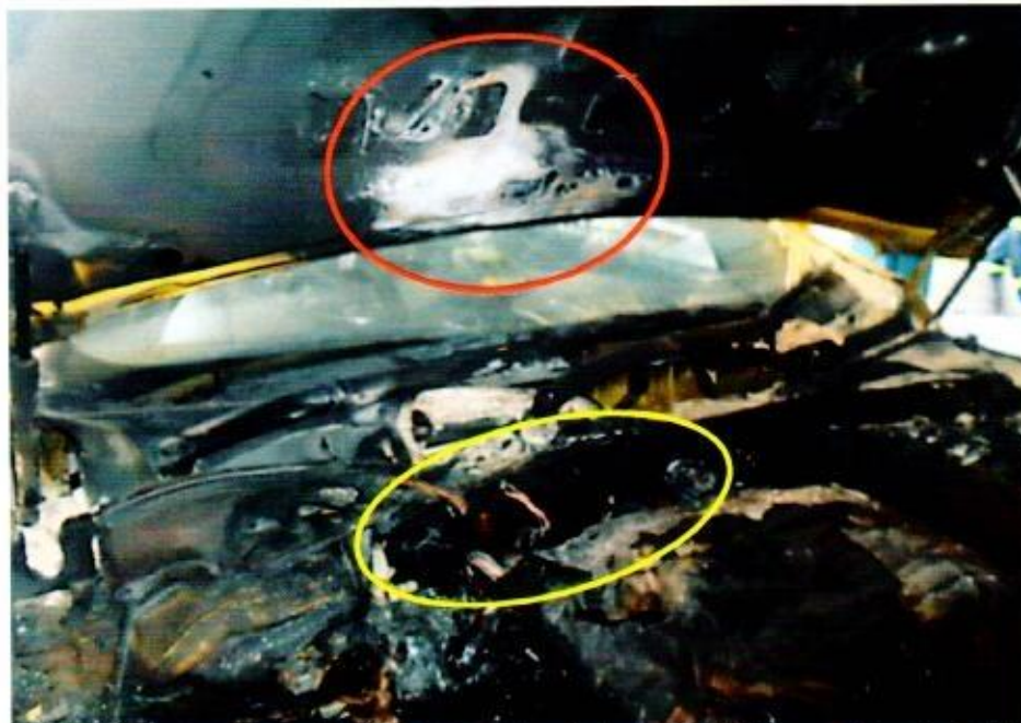
Photo 6 shows the whitish burn marks (red circle) that were found on the underside of the Insured Vehicle's front bonnet, directly under the area where the burn marks were formed on the top side of the front bonnet. Such whitish burn marks are a result of exposure to prolong heat intensity. The fire to the Insured Vehicle can then be established to have originated around the rear centre of the engine compartment (yellow circle).
