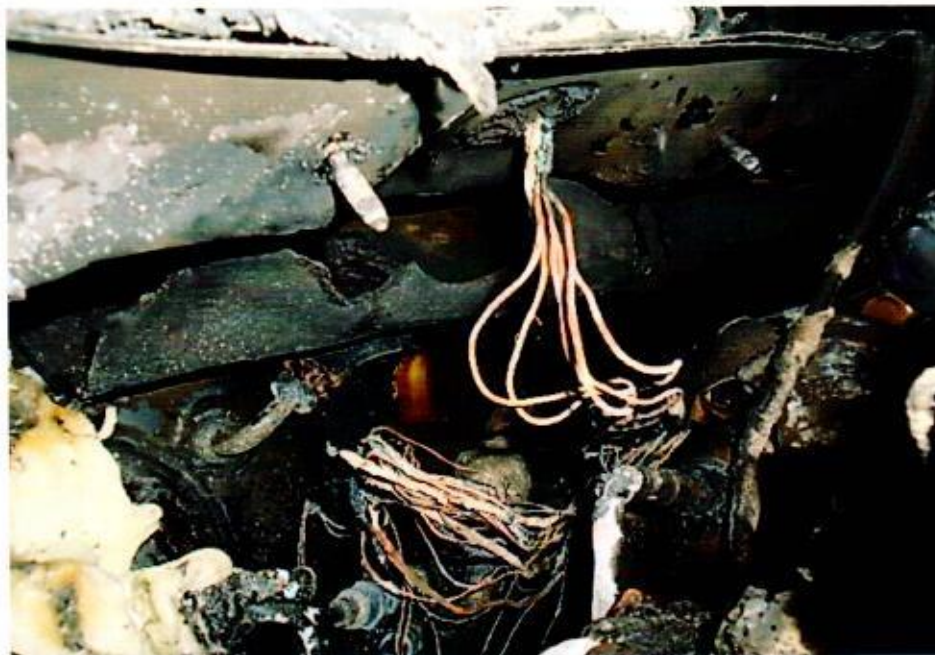
Photo 8 shows a closer view of the wirings at the rear centre area of the Insured Vehicle's engine compartment. The wirings were found to be completely burned to its bare copper state. Such condition normally indicates internal heating of copper wires which is a sign of an electrical short circuit occurring.
