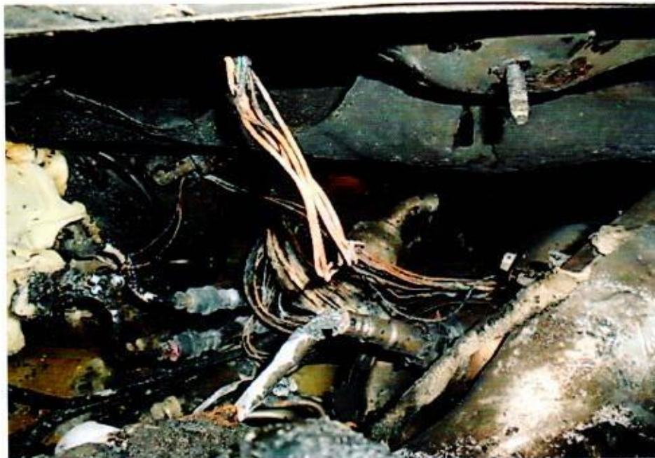
Photo 10 shows the burnt wirings at the rear centre area of the Insured Vehicle's engine compartment. The bright reddish colour of the copper wires suggest that the wirings were exposed to high heat, indicating internal heating of copper wires, which is a sign of an electrical short circuit occurring.
