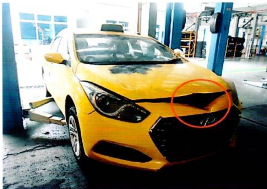
Photo 1 shows a general view of the front right body of the Insured Vehicle at the time of my inspection. The fire had affected most of the parts within the engine compartment. The damage to the front bumper (circled) was a result of firefighting operation.
