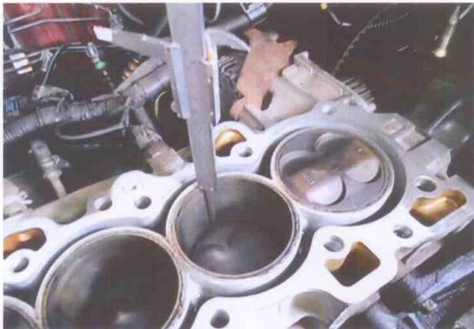
Photo 11 shows measurement of the stroke for cylinder 2 of the Honda engine that I had inspected.
