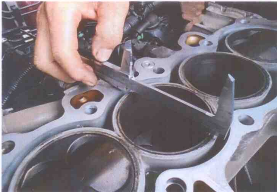
Photo 13 shows measurement being carried out to the bore of cylinder 3 of the Honda engine. The bore and stroke measurements of the Honda engine were carried out using a Vernier Caliper.
