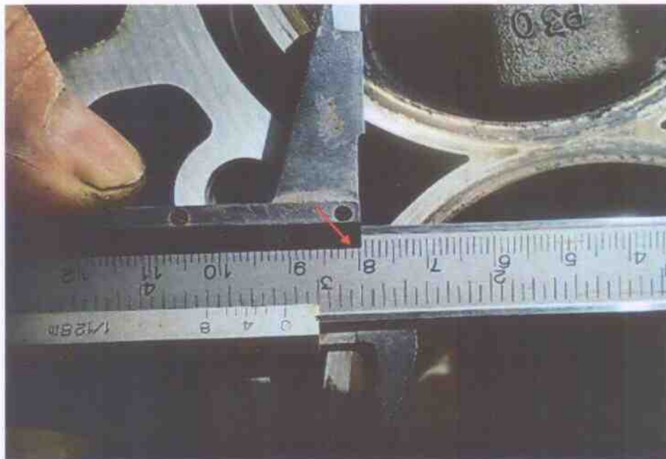
Photo 18 shows the bore measurement of cylinder 4, which was recorded to be 81.00mm.
