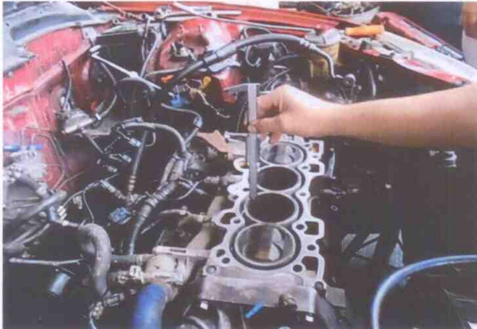
Photo 15 shows measurement of the stroke for cylinder 3 of the Honda engine that I had inspected. The stroke measurement of cylinder 3 was recorded to be 77.20mm.
