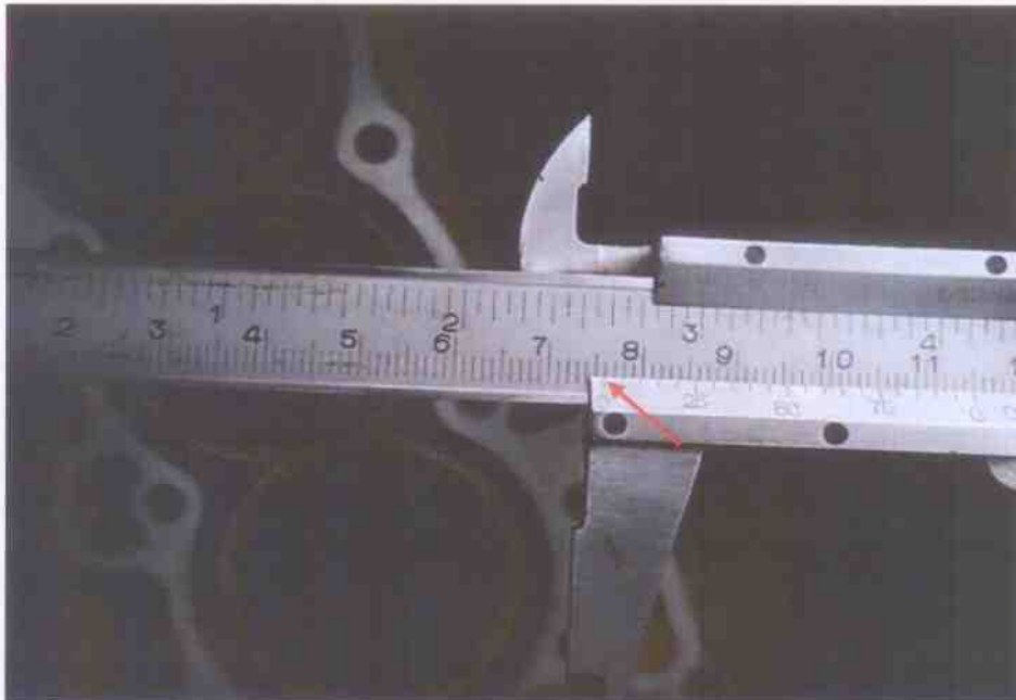
Photo 20 shows the stroke measurement of cylinder 4, which was recorded to be 75.90mm.
