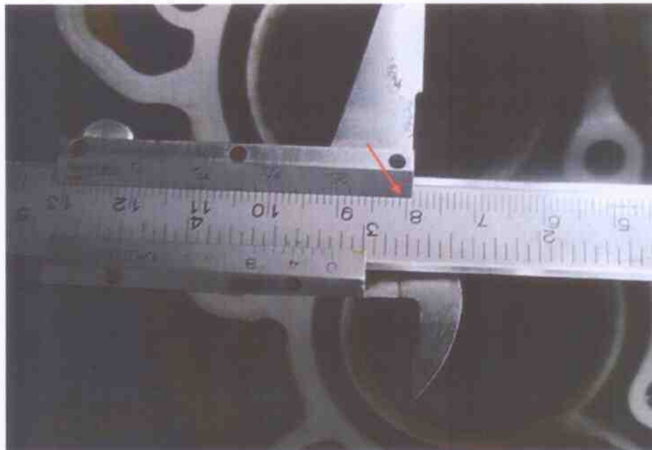
Photo 10 shows the bore measurement of cylinder 2, which was recorded to be 80.50mm.
