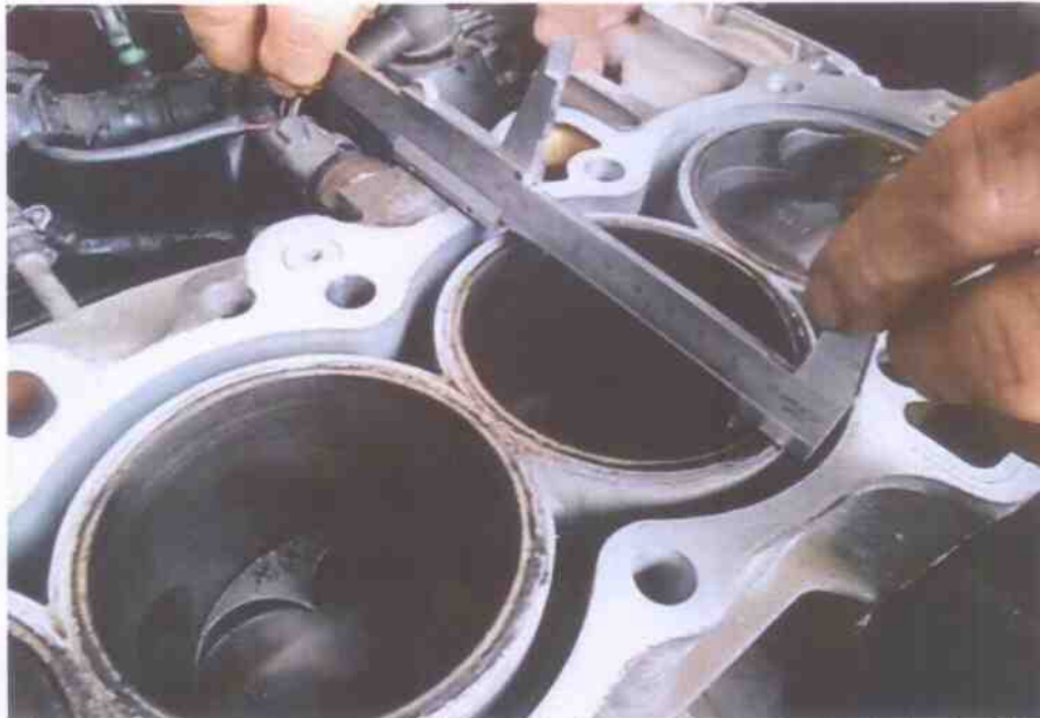
Photo 9 shows measurement being carried out to the bore of cylinder 2 of the Honda engine. The bore and stroke measurements of the Honda engine were carried out using a Vernier Caliper. The bore measurement of cylinder 2 was recorded to be 80.50mm.
