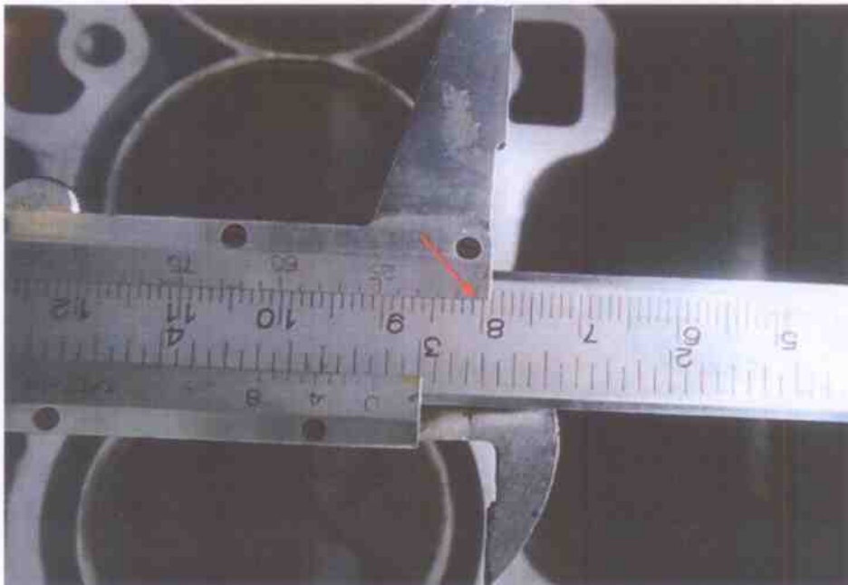
Photo 6 shows the bore measurement of cylinder 1, which was recorded to be 80.70mm.
