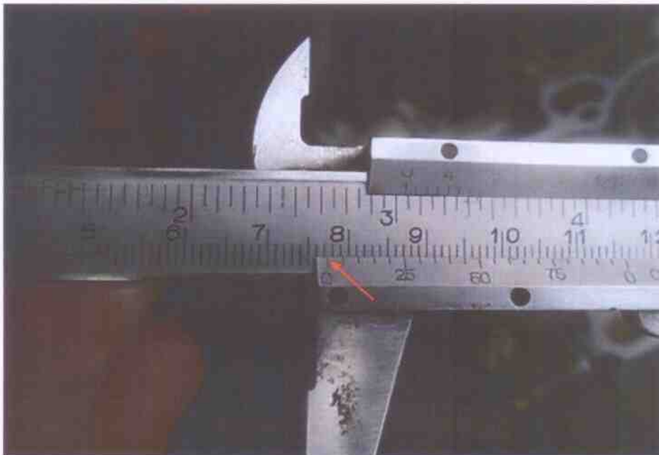
Photo 16 shows the stroke measurement of cylinder 3, which was recorded to be 77.20mm.
