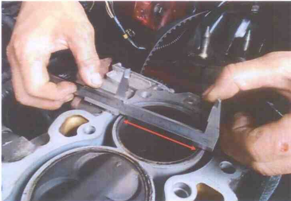
Photo 5 shows measurement being carried out to the bore of cylinder 1 of the Honda engine. The bore and stroke measurements of the Honda engine were carried out using a Vernier Caliper. The bore measurement of cylinder 1 was recorded to be 80.70mm.
