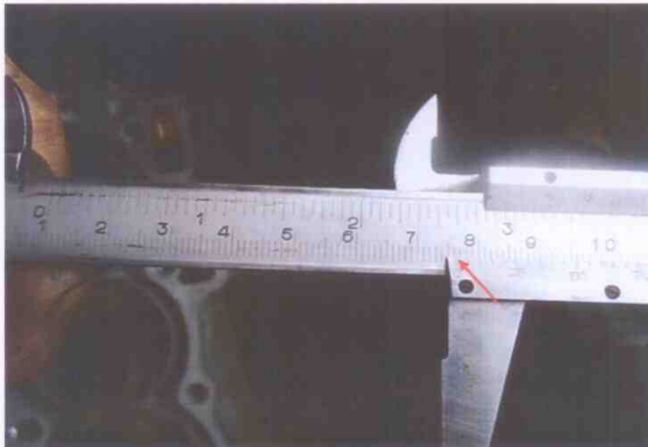
Photo 8 shows the stroke measurement of cylinder 1, which was recorded to be 76.10mm.
