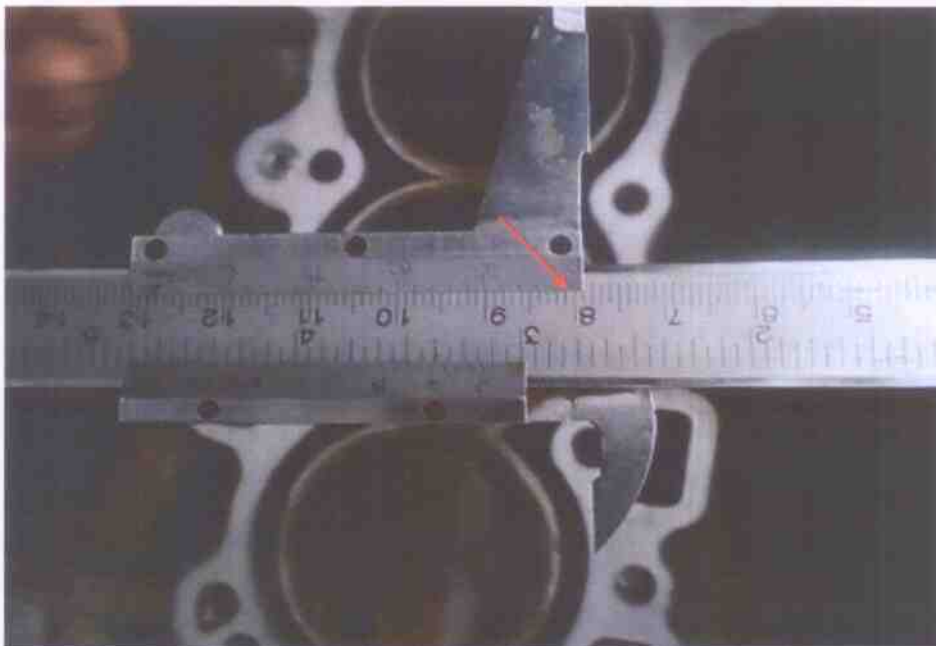
Photo 14 shows the bore measurement of cylinder 3, which was recorded to be 80.30mm.
