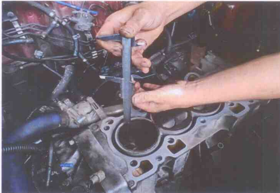
Photo 19 shows measurement being carried out to the stroke of cylinder 4 of the Honda engine. The bore and stroke measurements of the Honda engine were carried out using a Vernier Caliper.
