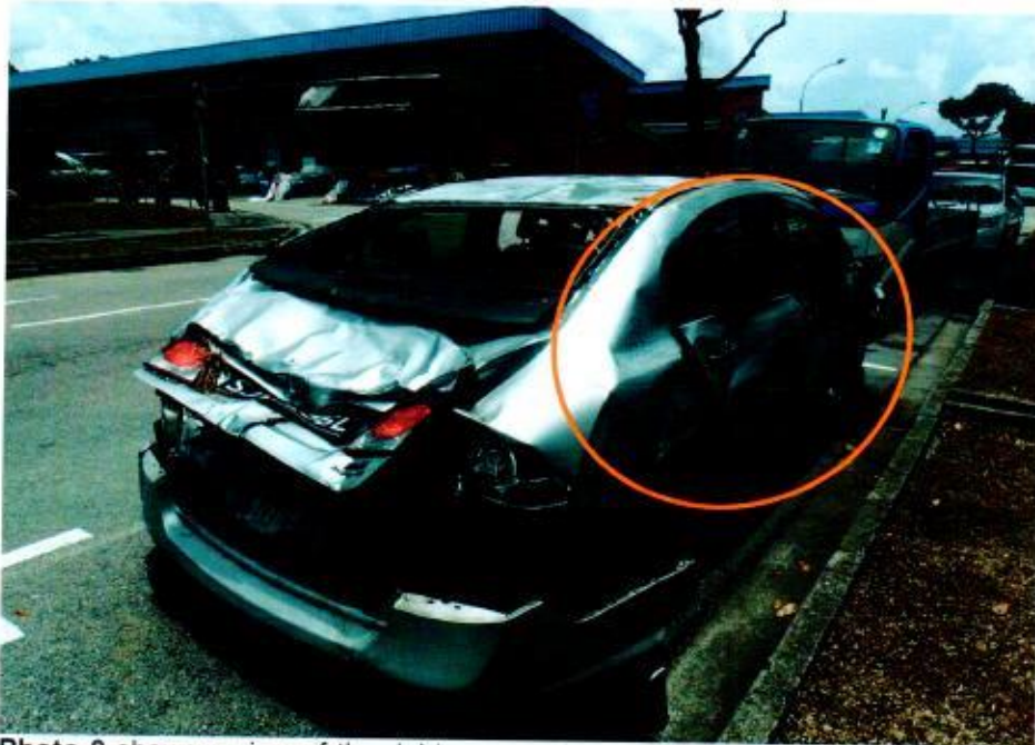
Photo 9 shows a view of the right rear portion of the Insured Vehicle during our physical inspection. The Insured Vehicle sustained extensive damages as a result of the incident. The buckled right portion (circled) seems to be consistent with Mr Thina's statement in which the Insured Vehicle had flipped over on its right side after the steering wheel locked.
