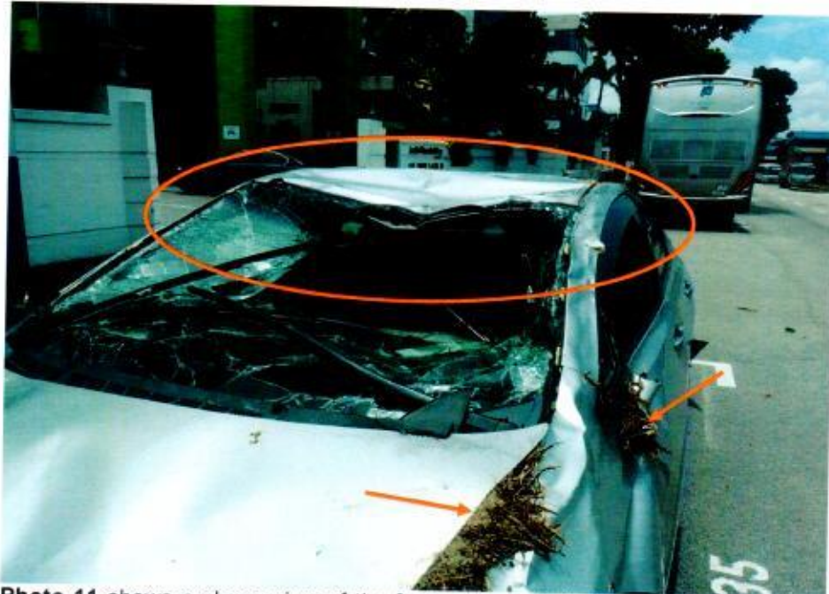
Photo 11 shows a closer view of the front portion of the Insured Vehicle during our physical inspection. The buckled hood (circled), dried leaves and/or soil particles (arrowed) that were found stuck at the left side of the front bonnet and left side mirror seem to correlate with Mr Thina's statement in which the Insured Vehicle had flipped over on its right side before coming to a stop in an overturned near the central divider.
