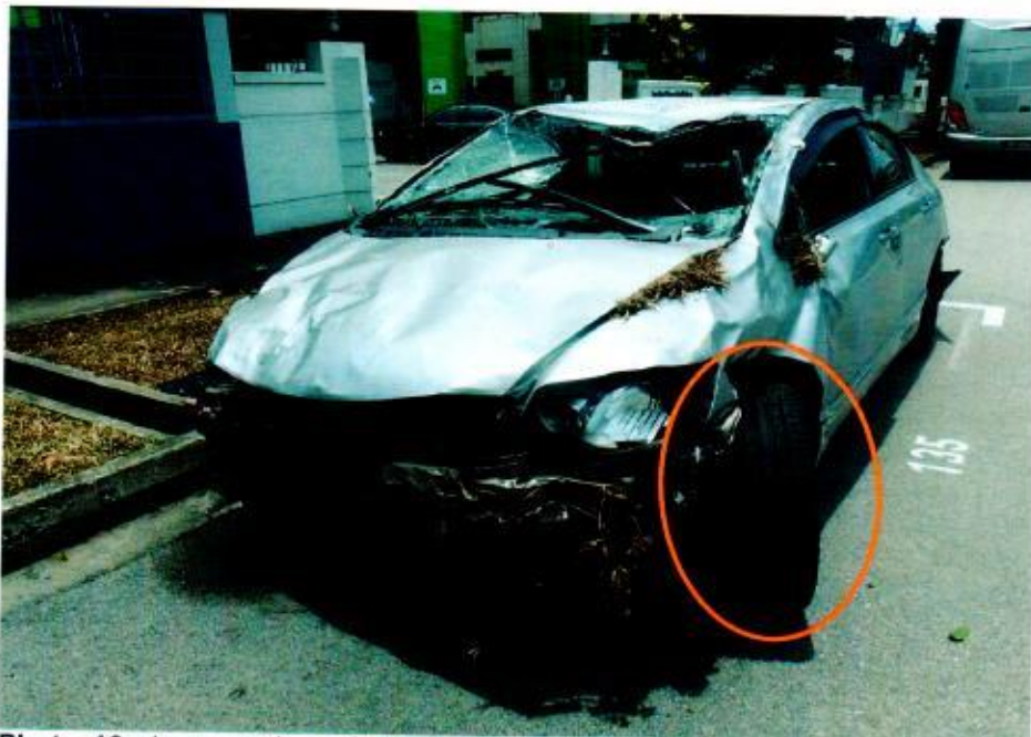
Photo 10 shows a view of the front portion of the Insured Vehicle during our physical inspection. The angle of the front left tyre seems to correlate with Mr Thina's statement in which the steering wheel had locked after he made a hard left turn to avoid the dog.
