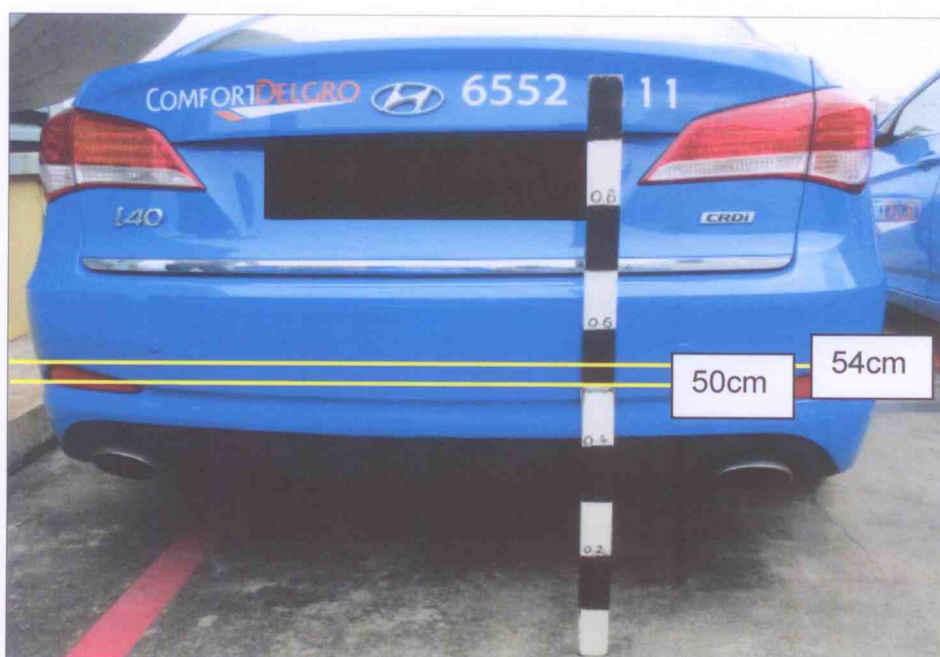
Photo 14 shows the height measurement being conducted on the rear portion of the Taxi (using a similar make and model). The height of the paint graze marks on the lower left portion of the Taxi's rear bumper was between the ranges of 50cm to 54cm above ground level.
