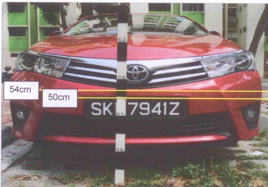
Photo 15 shows the height measurement being conducted on the front portion of the Toyota. The faint paint graze marks found on the front left portion of the Toyota are within the 50cm to 54cm height range.
