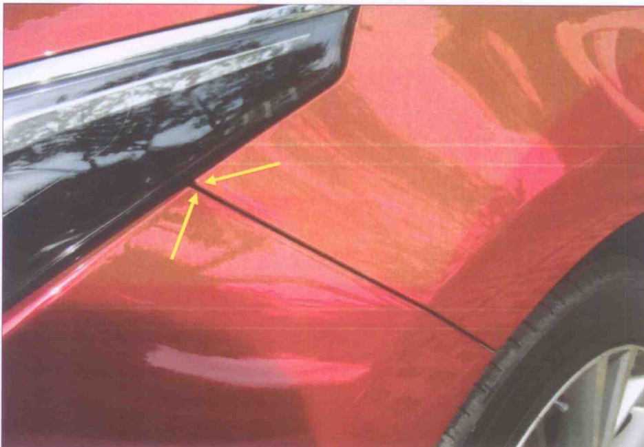
Photo 10 shows a close up view of the left corner edge of the front bumper of the Toyota. We observed that there was no misalignment at the corner edges (arrowed).
