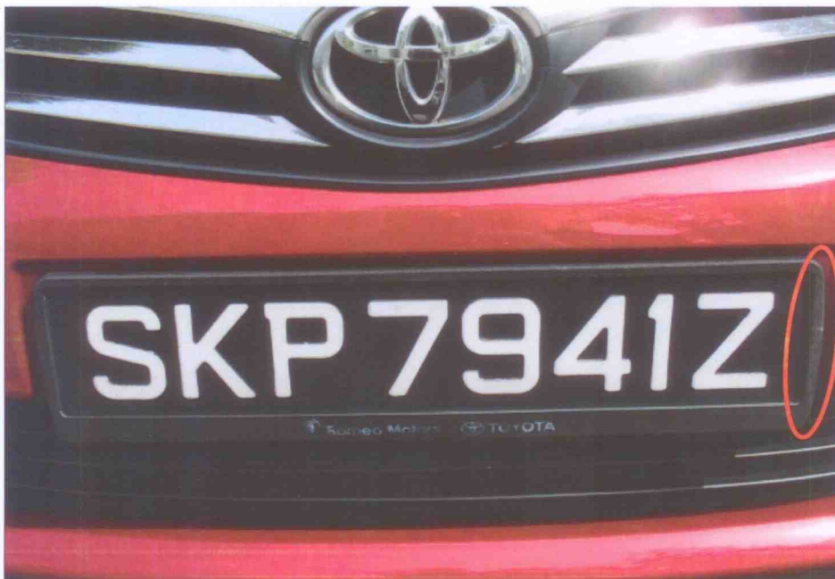
Photo 4 shows at the time of our inspection, we noted that there was a slight distortion on the left side of the Toyota's front number plate frame, indicating that it had sustained an impact directly onto its front number plate frame (circled).
