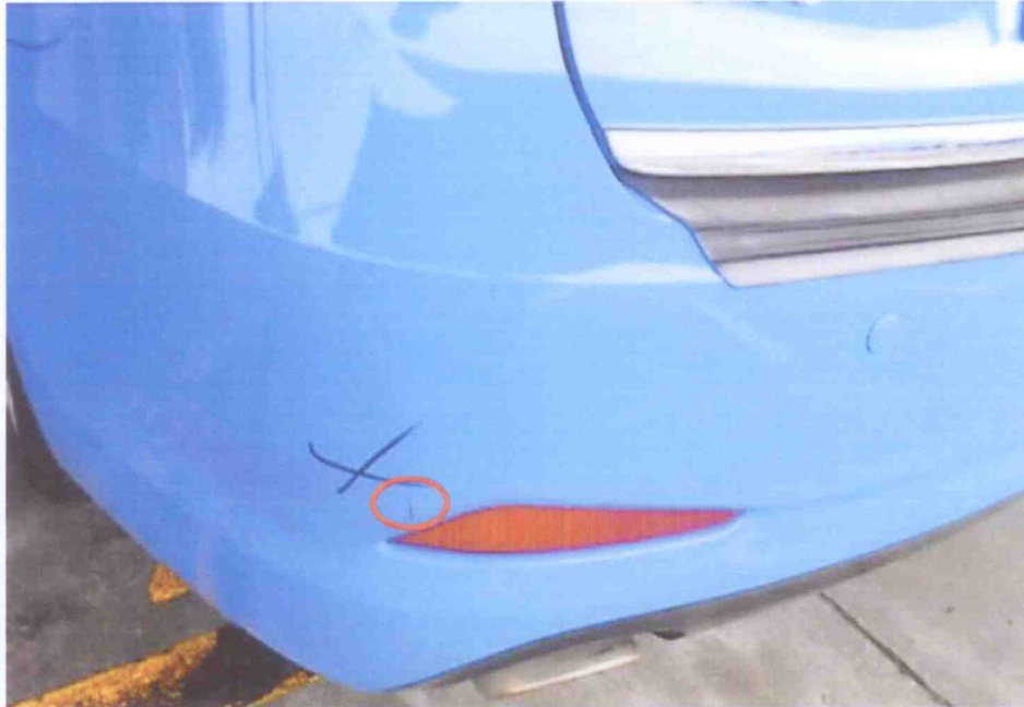
Photo 2 shows upon closer examination of the photographs taken at the time of accident reporting, we observed that the Taxi had sustained paint graze marks to the lower left portion of the rear bumper as marked by the 'X' (circled).
