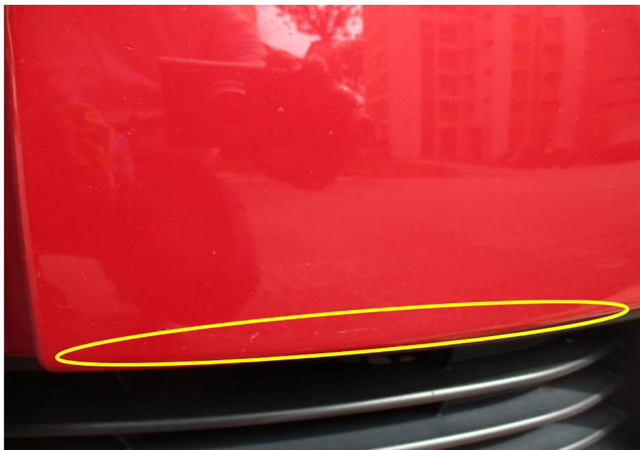
Photo 6 shows a close up view of the paint scratch marks and paint chips found at the left portion of the front bumper, above the air vent (circled).
