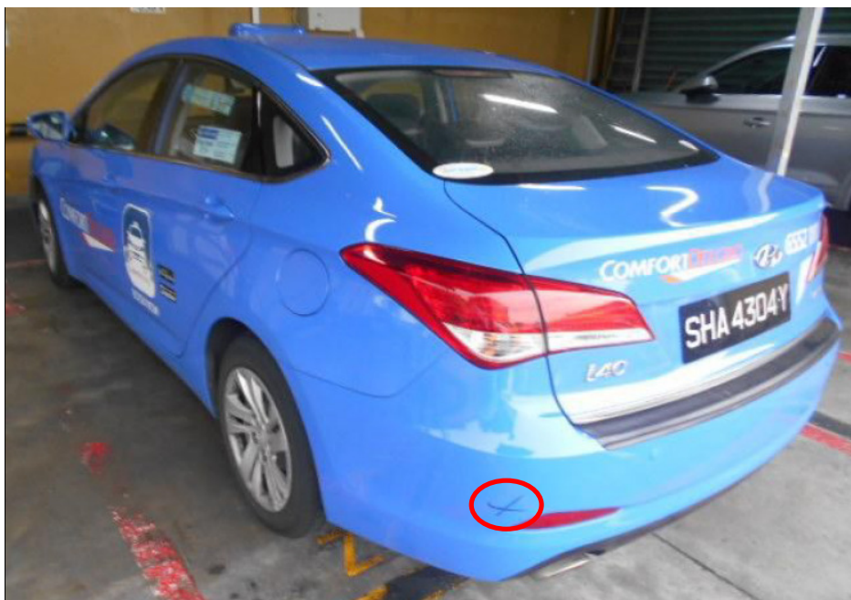
Photo 1 shows a general view of the rear portion of the Taxi at the time of reporting, which was about 3 days after the accident. We noted that the Taxi had sustained an impact onto its rear lower left portion as marked by the 'X' (circled).
