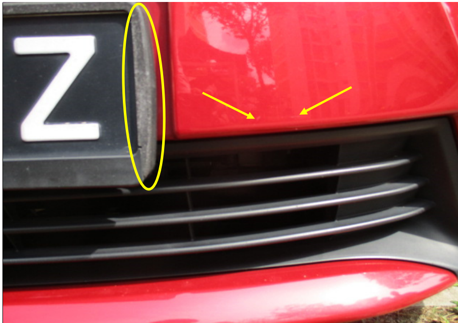
Photo 5 shows a closer view of the slight distortion on the left side of the Toyota's front number plate frame (circled). Paint scratch marks and paint chips were found at the left portion of the front bumper, above the air vent (arrowed).
