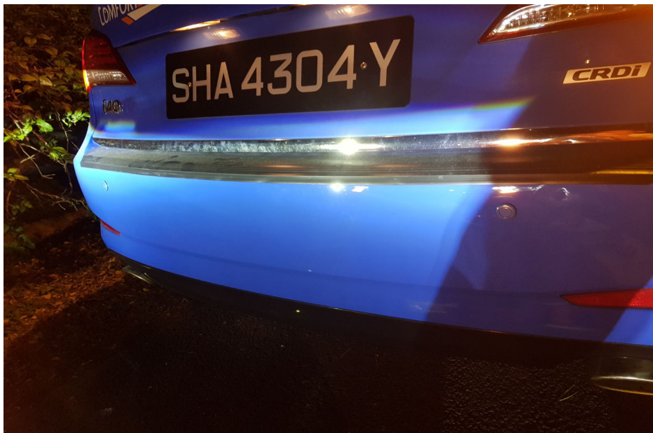
Photo 11 shows the rear bumper of the Taxi after the accident. Mr Ong did not take any photograph of the left portion of the Taxi's rear bumper as Mr Ching had told him that the damages were sustained to the right portion of the rear bumper as stated in Mr Ong's accident report. Upon closer examination of the photograph, we could not find any damages to the right portion of the Taxi's rear bumper.
