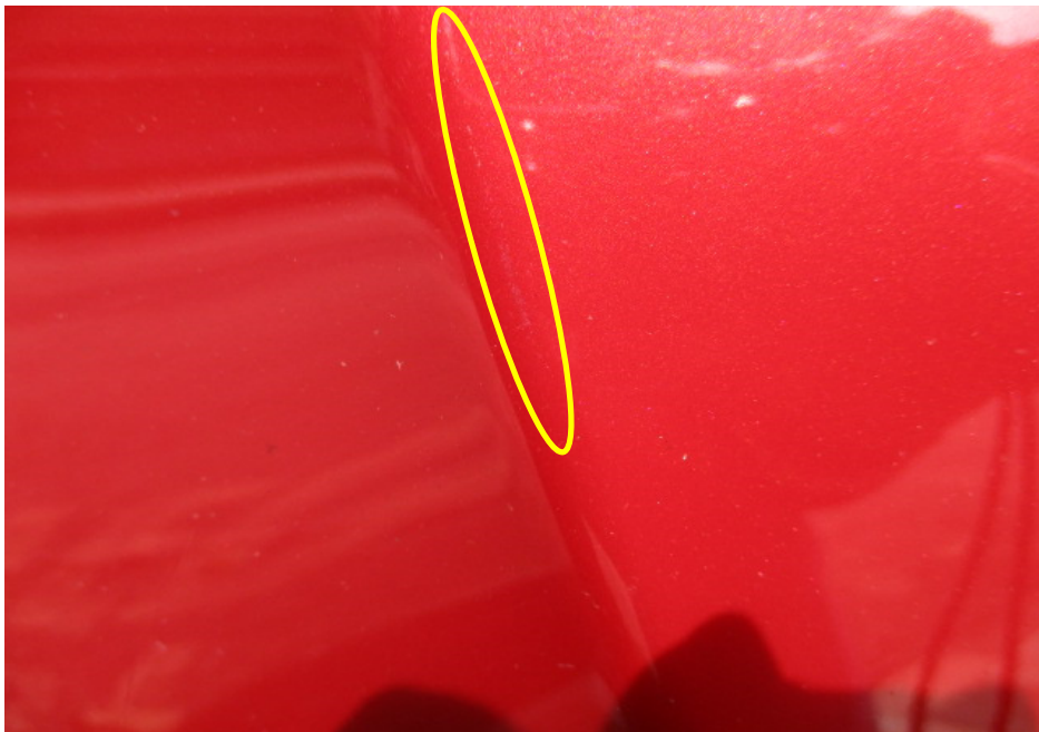
Photo 8 shows a close up view of the faint paint graze marks observed on the front left portion of the Toyota (circled).
