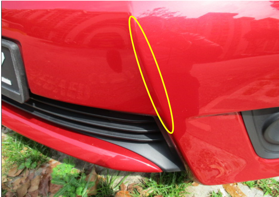
Photo 7 shows the faint paint graze marks observed on the front left portion of the Toyota (circled).
