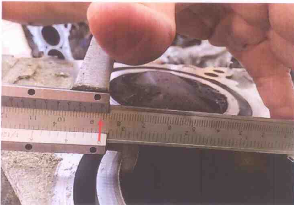
Photo 13 shows the bore measurement of cylinder 2, which was recorded to be 86.00mm.
