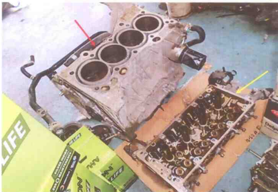
Photo 6 shows the top block (yellow arrow) of the Honda engine separated from its bottom block (red arrow). This was to enable me to carry out measurements of its cylinders, in particular the bore and stroke measurements of each cylinder, which typically can be used to determine the engine displacement or more commonly referred to as engine cc.
