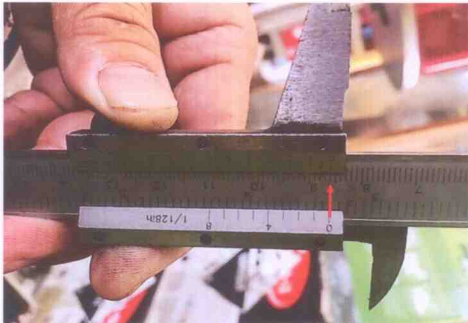
Photo 19 shows the stroke measurement of cylinder 3, which was recorded to be 86.00mm.
