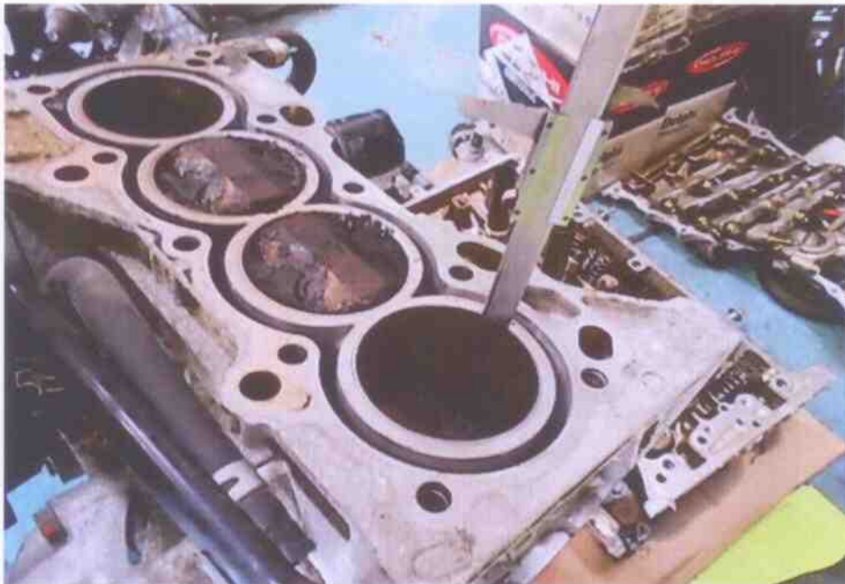
Photo 22 shows measurement being carried out to the stroke of cylinder 4 of the Honda engine. The bore and stroke measurements of the Honda engine were carried out using a Vernier Caliper.
