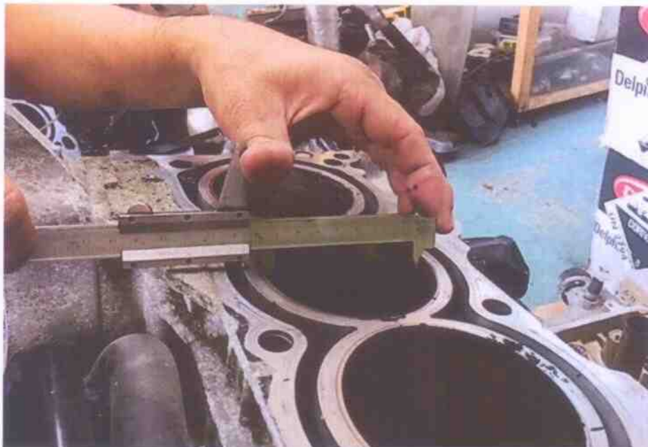
Photo 12 shows measurement being carried out to the bore of cylinder 2 of the Honda engine. The bore and stroke measurements of the Honda engine were carried out using a Vernier Caliper.
