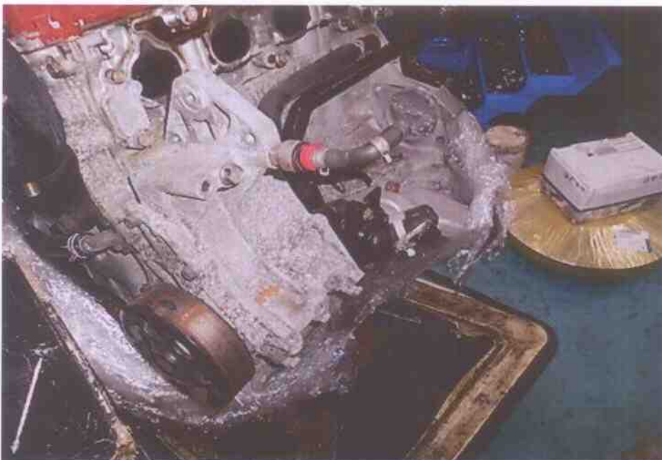
Photo 4 shows a general view of the Honda engine that I had inspected. My visual examination of the engine housing revealed the housing to be of serviceable/satisfactory condition. There was no crack and/or hole observed on the engine housing.
