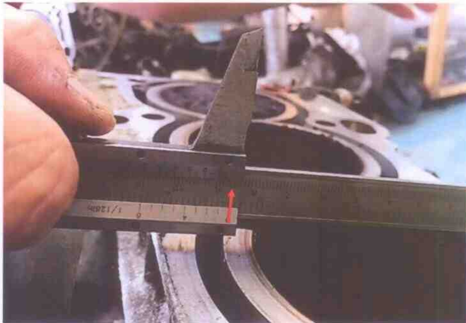
Photo 17 shows the bore measurement of cylinder 3, which was recorded to be 85.50mm.
