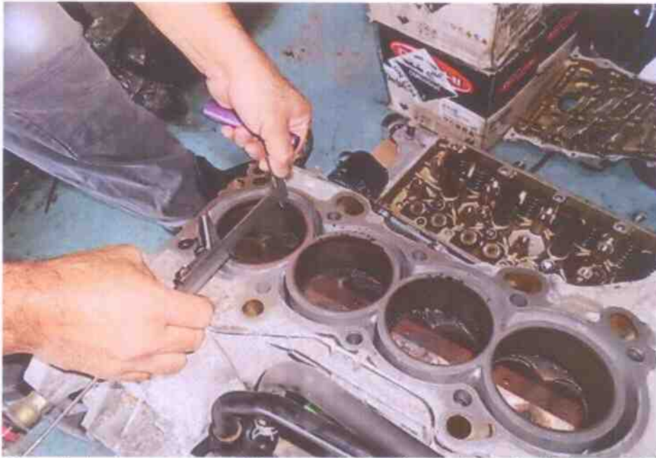
Photo 7 shows measurement being carried out to the bore of cylinder 1 of the Honda engine. The bore and stroke measurements of the Honda engine were carried out using a Vernier Caliper.
