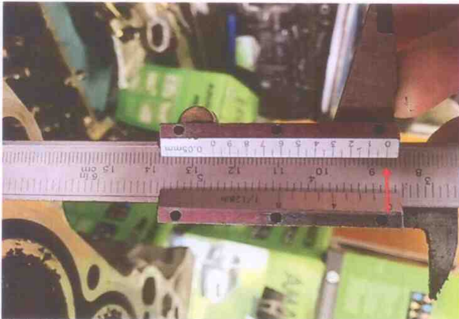
Photo 11 shows the stroke measurement of cylinder 1, which was recorded to be 86.00mm.
