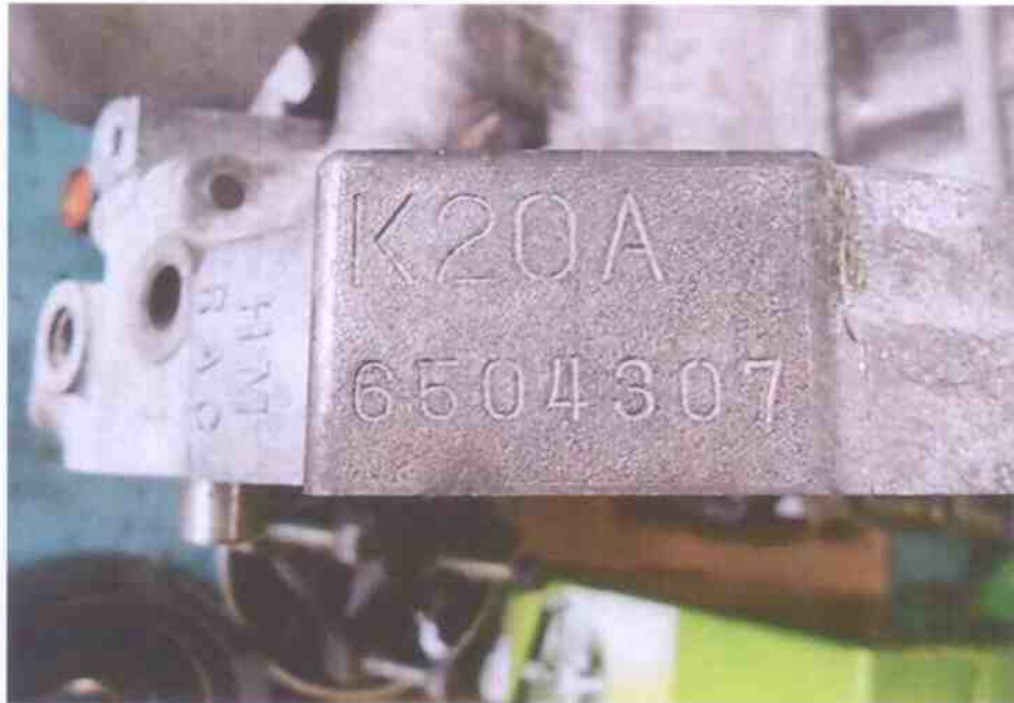
Photo 5 shows the engine number engraved on the housing of the Honda engine that I had inspected. The engine number was K20A6504307.
