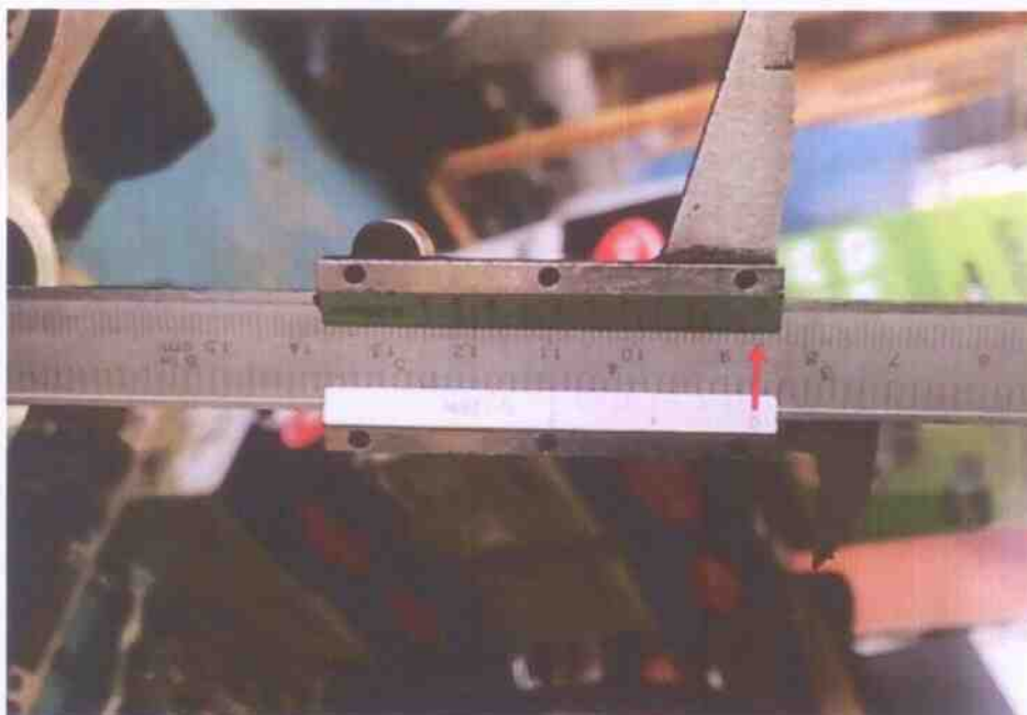
Photo 23 shows the stroke measurement of cylinder 4, which was recorded to be 85.50mm.
