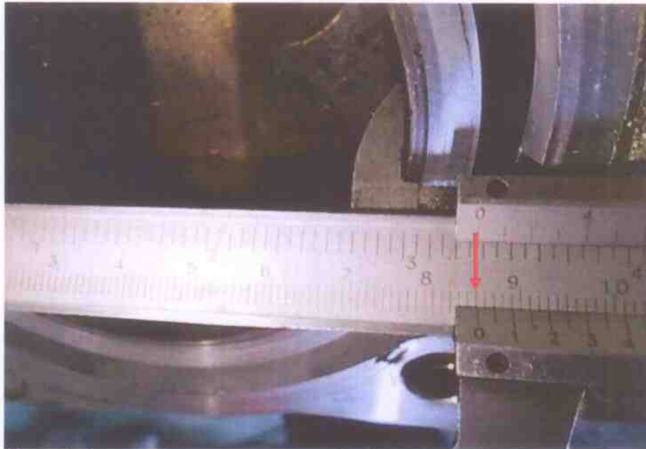
Photo 9 shows the bore measurement of cylinder 1, which was recorded to be 85.00mm.
