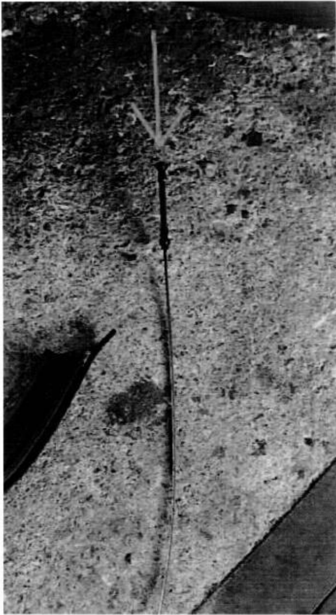
Front bonnet lock cable – jammed - during survey bonnet spring lever is jammed.
