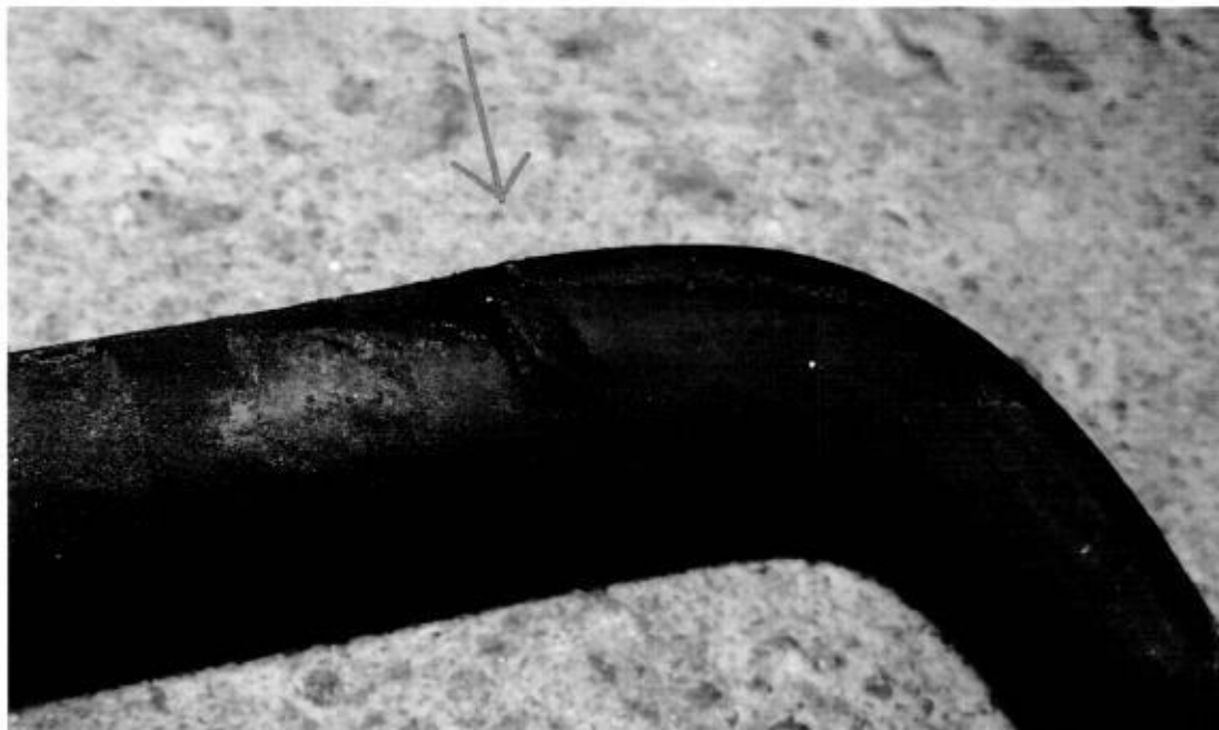
Bypass hose - torn
