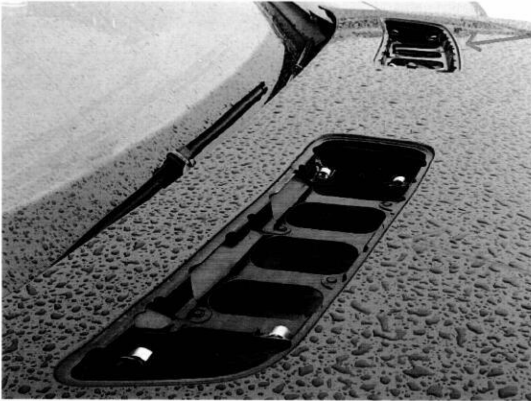
Front bonnet top air vent – during survey already cracked and missing due to bonnet body buckled
