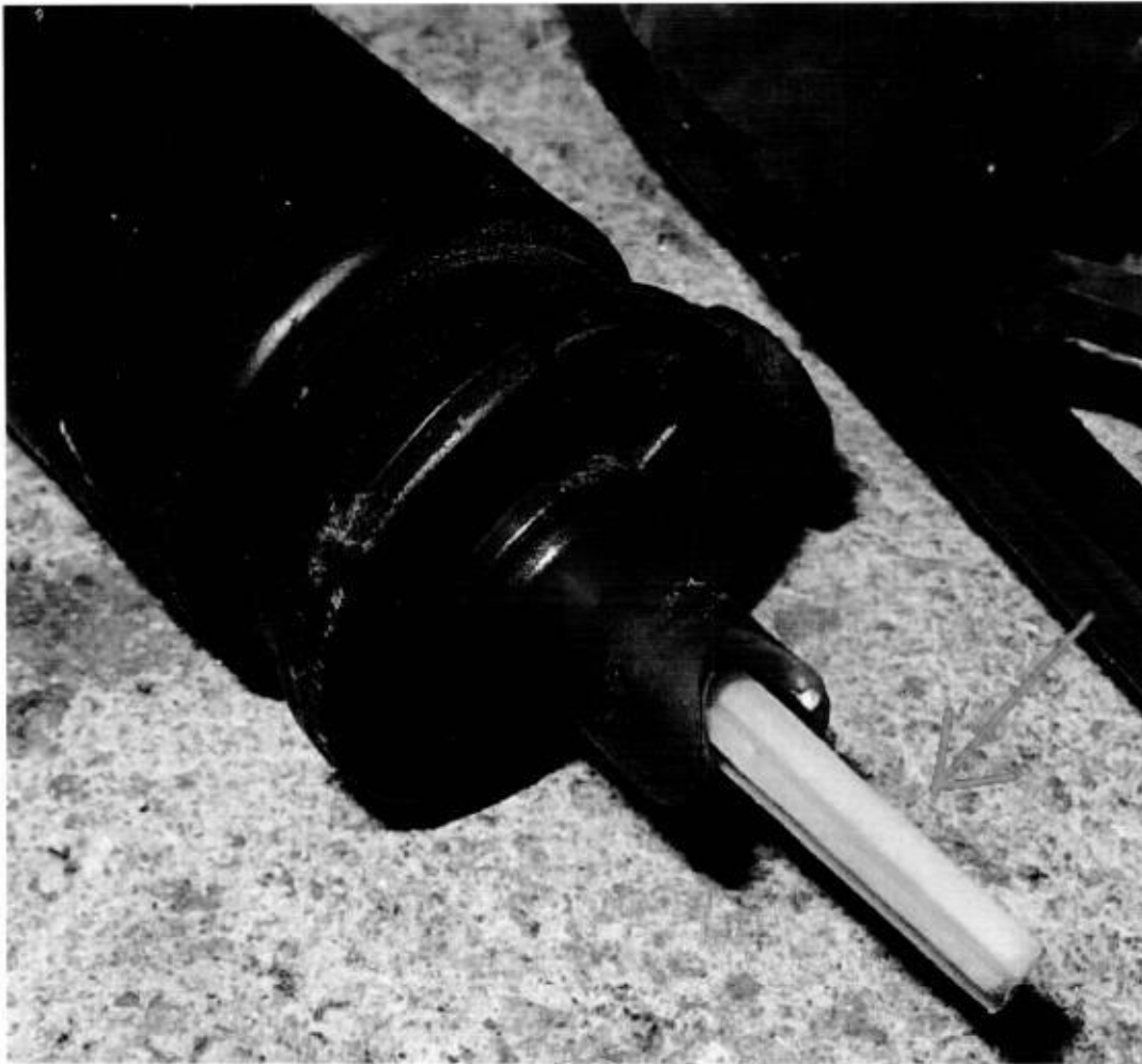
Front nozzle pump LH – damaged / jammed
