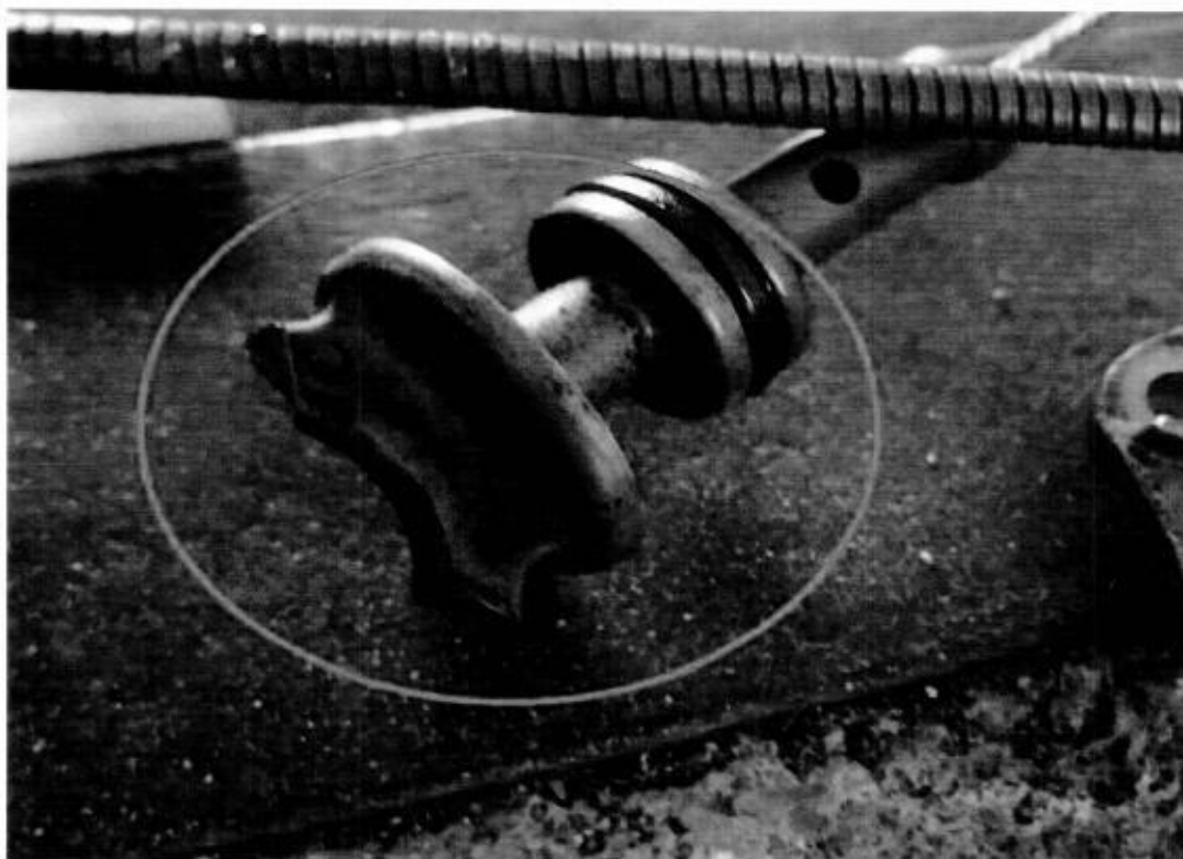
Engine oil dipstick – cracked
