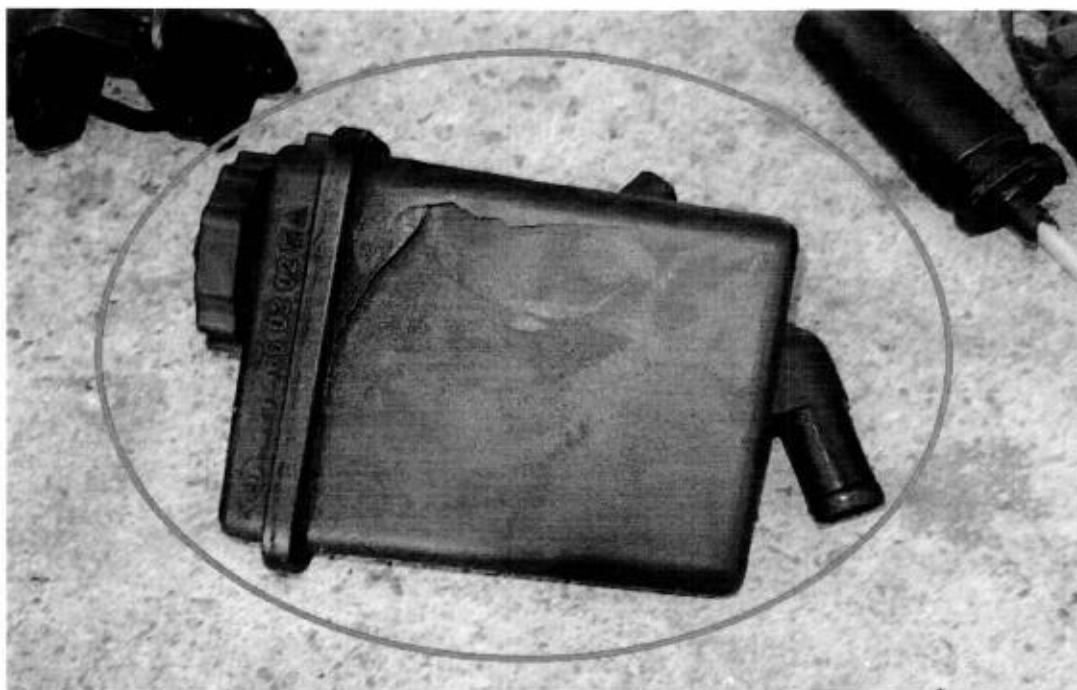
Power steering tank – cracked
