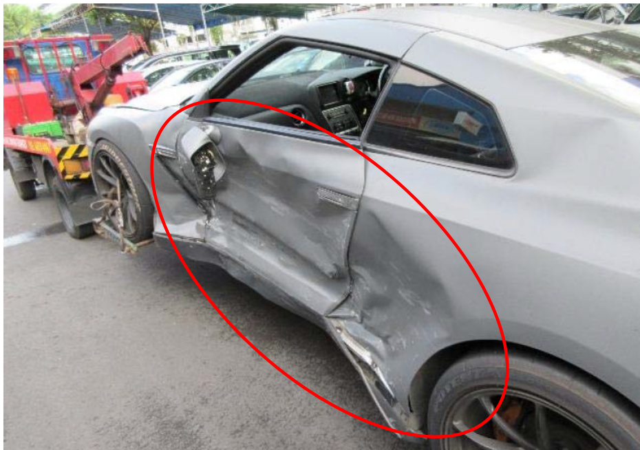
Photo 2 shows the left portion of the Insured Vehicle during the accident reporting. The extensive damages sustained seem to correlate with the Insured Vehicle being hit by another vehicle at it left portion (circled).
