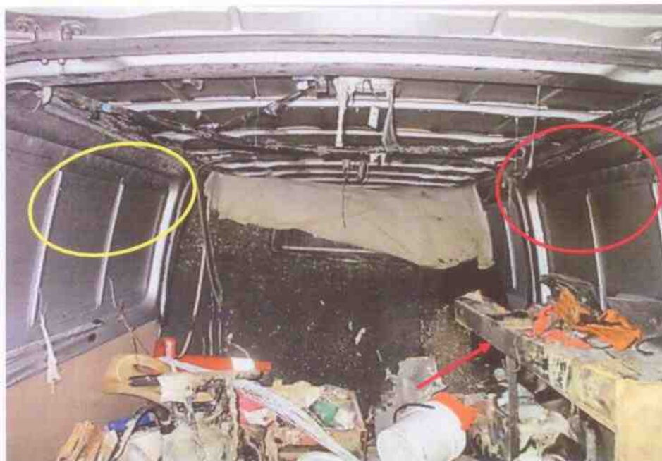
Photo 18 shows the higher concentration of burn marks on the right side panel (red circle) as compared to the left side panel (yellow circle) of the rear cabin of the Insured Vehicle. There were also high heat intensity burn marks (whitish burn marks) found on the wooden shelves (arrowed) and metallic items that were stored around the immediate vicinity to where the fire had likely started.
