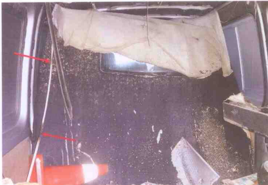
Photo 13 shows the 2nd LED light strip fitted on the left side panel of the rear cabin of the Insured Vehicle which had sustained fire damage (arrowed).
