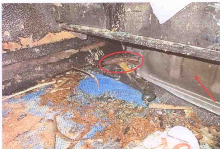
Photo 20 shows the rust that had developed on the surfaces of the metallic items (circled) and vehicle body (arrowed) at the immediate vicinity where the fire had likely started. Prolonged exposure to high heat intensity usually causes the bare steel/metal material of these items and vehicle body to be exposed to natural environmental condition. The rust that had developed on these surfaces would also support our findings of where the fire to the Insured Vehicle had originated.
