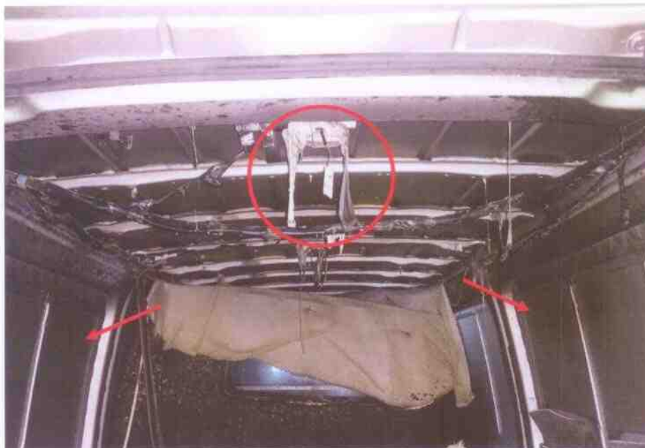
Photo 8 shows a closer view of the cabin lighting (circled) and side panels (arrowed) of the rear cabin of the Insured Vehicle that were partially melted and/or burnt as a result of the fire.
