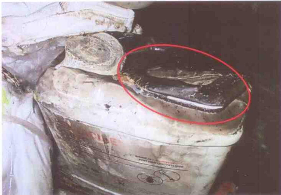
Photo 17 shows a close up view of the top portion of 1 of the partially melted and/or burnt containers wet with fluid (circled).
