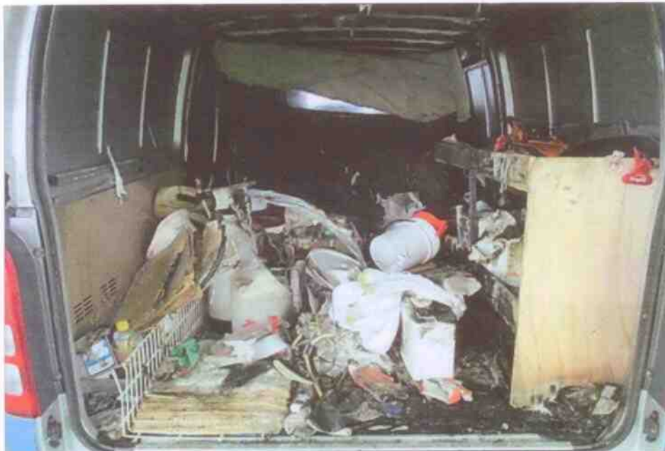
Photo 15 shows the many containers containing flammable fluids and hazardous chemicals stored at the rear cabin of the Insured Vehicle which were used for pest control purposes. Such items included pesticides, insecticides and rodent poison pellets, amongst others.
