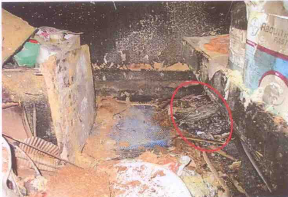
Photo 21 shows upon closer examination of the right side of the rear cabin of the Insured Vehicle as well as around the immediate vicinity to where the fire had likely started, we found a partially melted and/or burnt plastic bag containing metal hooks placed in the centre of coils made out of metal wires (circled).
