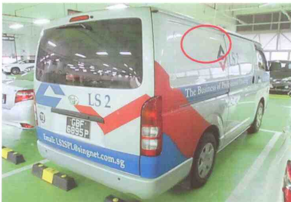
Photo 2 shows the general view of the right rear portion of the Insured Vehicle at the time of our inspection. The exterior body of the Insured Vehicle had sustained minor fire damage at the right rear portion (circled).
