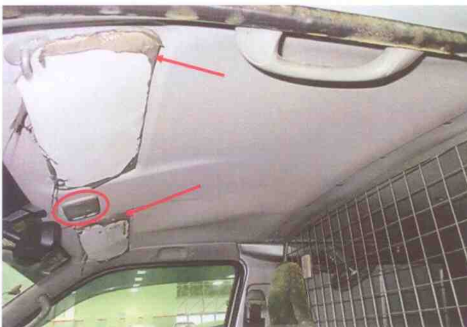
Photo 6 shows a closer view of the sun visors (arrowed) and the cabin lighting (circled) that were partially melted and/or burnt as a result of the fire.
