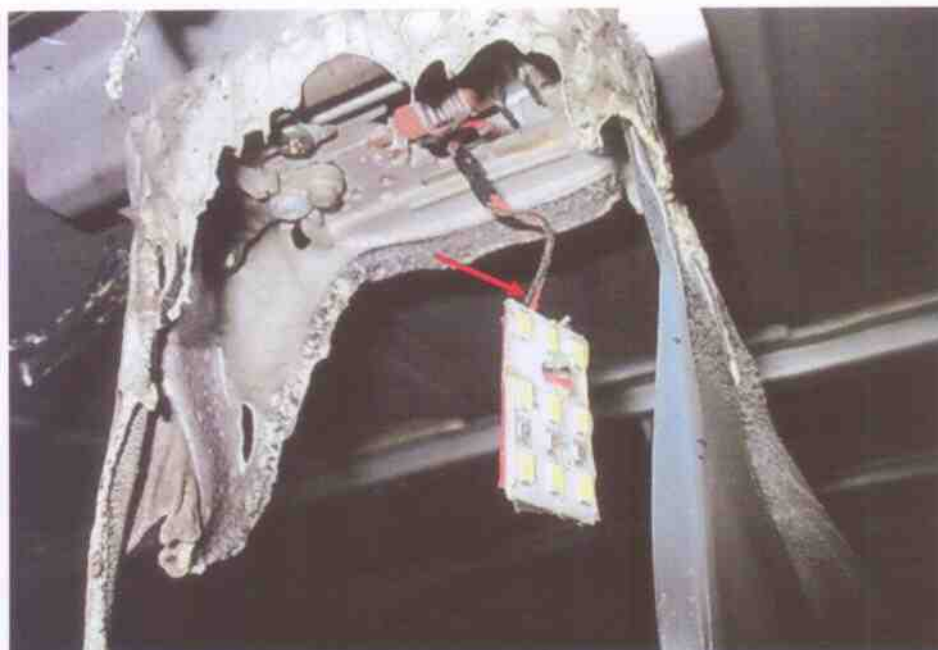
Photo 24 shows a close up view of the faint traces of greenish residue there were found on the wirings of the rear cabin LED light strip of the Insured Vehicle (arrowed). The presence of such greenish residue suggests occurrence of an electrical short circuit.
