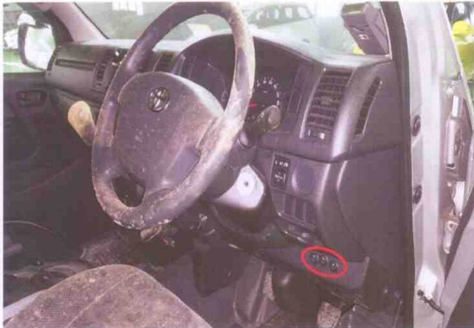
Photo 10 shows the 3 aftermarket on/off switches fitted above the foot pedals of the Insured Vehicle upon our inspection (circled).
