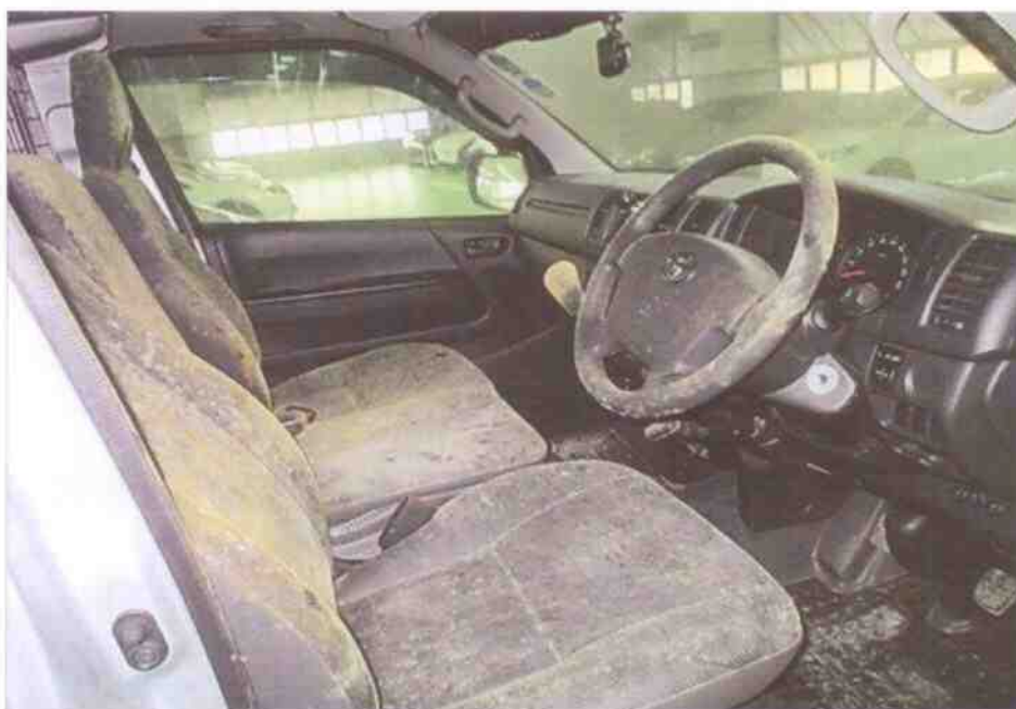
Photo 5 shows the interior compartment of the Insured Vehicle, which was covered in fire extinguisher residue at the time of our inspection. Some of the interior components were partially melted and/or burned as a result of the fire. These had included the seats, sun visors, roof upholstery, cabin lights and side panels, amongst others.
