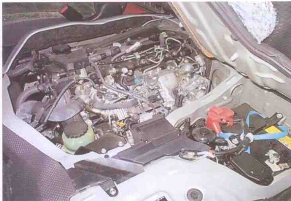
Photo 4 shows a general view of the engine compartment of the Insured Vehicle at the time of our inspection. The engine compartment of the Insured Vehicle was relatively unaffected by the fire.
