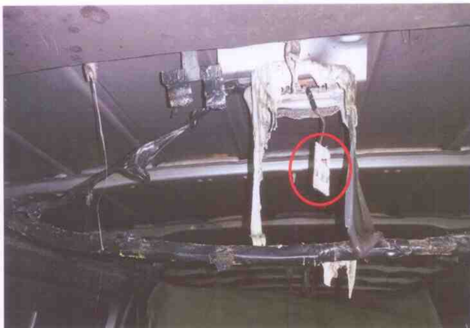
Photo 14 shows a close up view of the rear cabin LED light strip of the Insured Vehicle which had sustained fire damage (circled).
