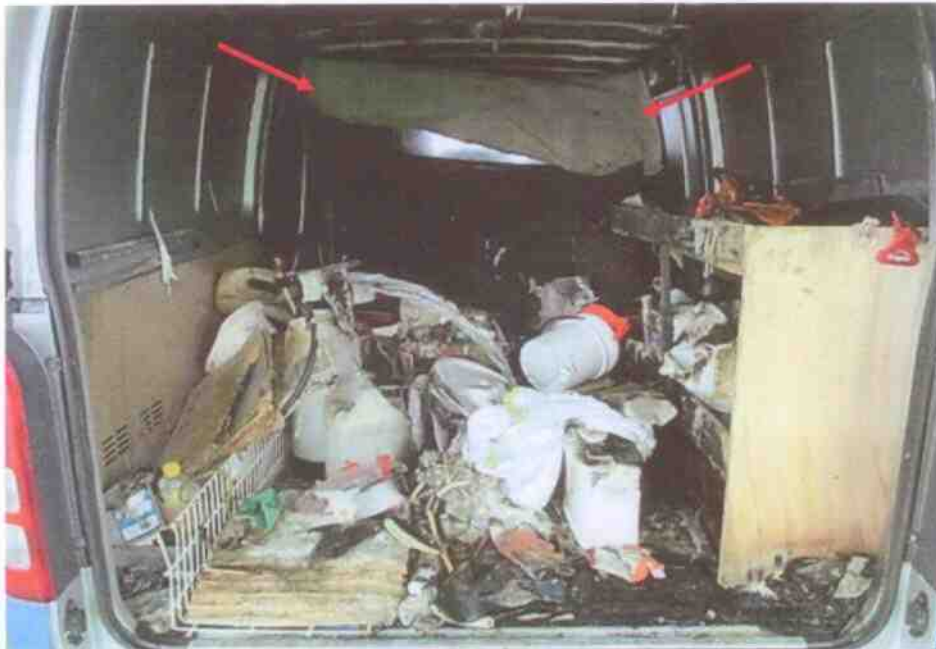
Photo 7 shows a closer view of the roof upholstery (arrowed) of the rear cabin that was partially melted and/or burnt as a result of the fire.
