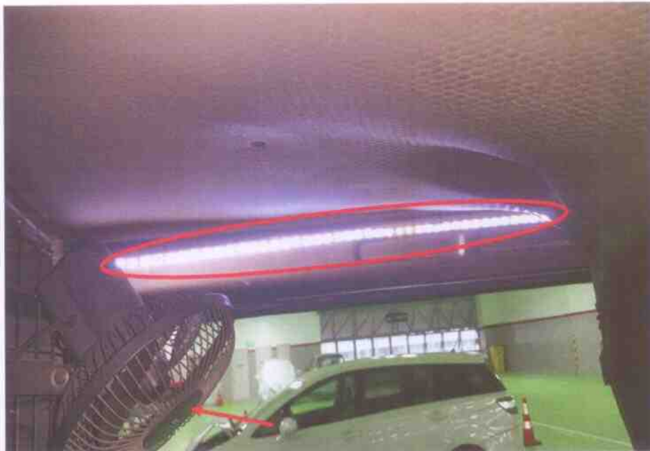
Photo 12 shows the 1st LED light strip fitted on the right side panel of the rear cabin (circled) after the 1st switch was turned on. The mini fan was fitted directly behind the centre console of the Insured Vehicle (arrowed).
