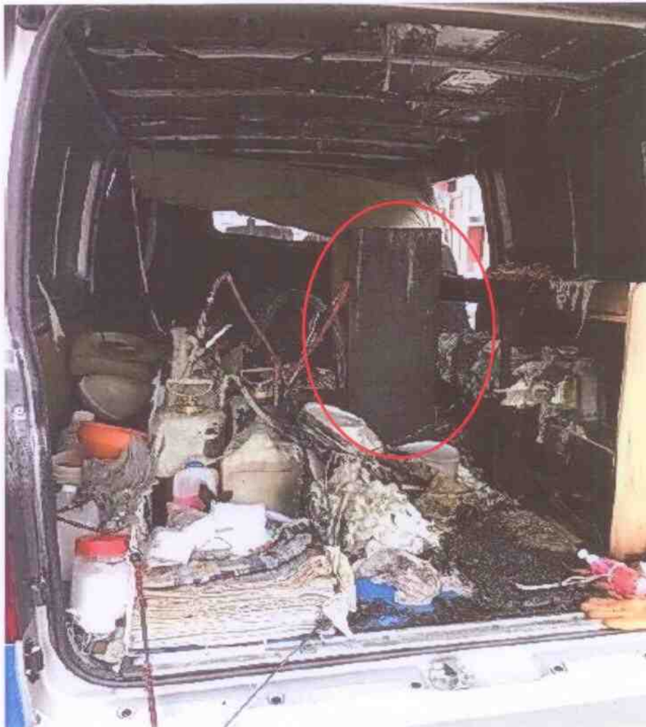
Photo 25 shows the rear cabin of the Insured Vehicle after the fire was extinguished. In general, the information that could be gathered from this photograph pertaining to the nature of fire damage had corresponded to the events that were related to us by Mr Seah, which is the fire had started from the right side of the rear cabin of the Insured Vehicle (circled).
