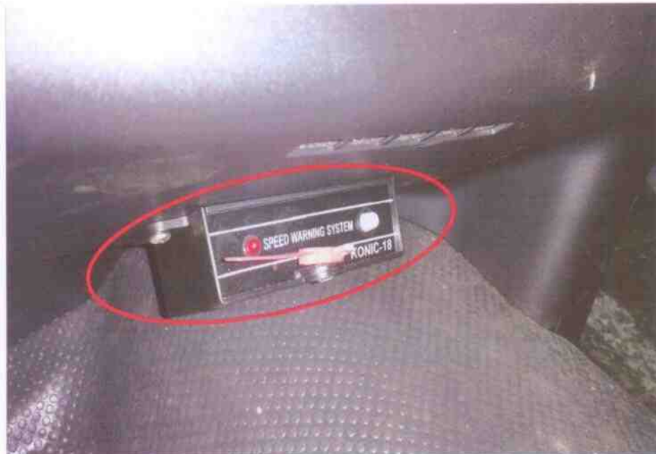
Photo 9 shows the vehicle speed limiter device fitted underneath the glove compartment of the Insured Vehicle upon our inspection (circled).
