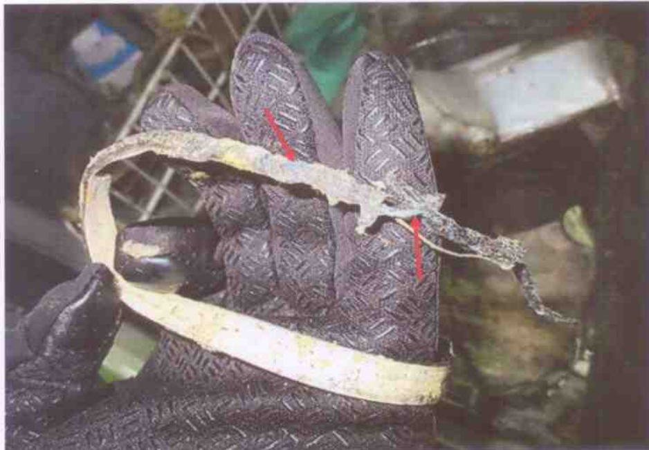
Photo 23 shows a close up view of the faint traces of greenish residue there were found on the LED light strip that was fitted along the left side panel of the rear cabin of the Insured Vehicle (arrowed). The presence of such greenish residue suggests occurrence of an electrical short circuit.
