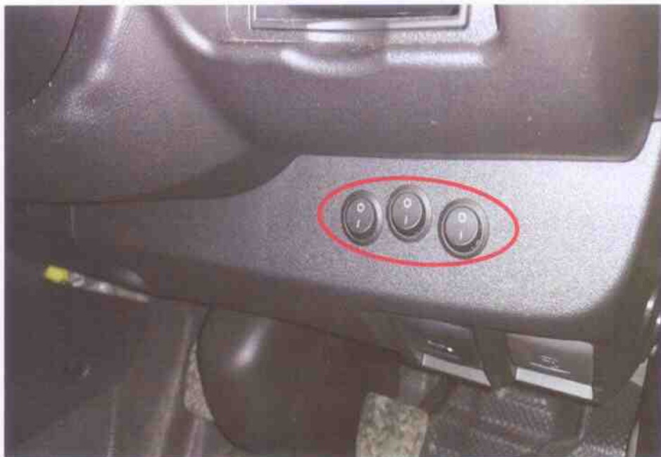
Photo 11 shows a closer view of the 3 aftermarket on/off switches fitted above the foot pedals of the Insured Vehicle (circled) upon our inspection.
