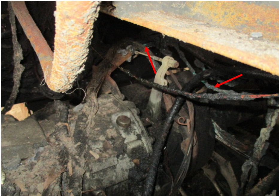
Photo 12 shows several original factory fitted wirings below the sub engine compartment with greenish residue (arrowed). The presence of such greenish residue suggests occurrence of an electrical short circuit.
