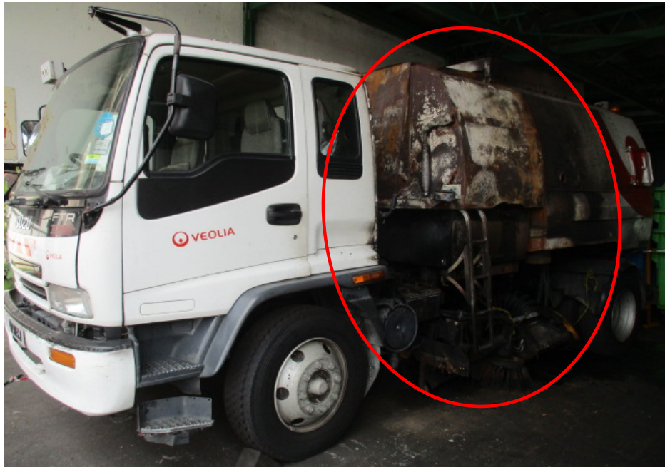
Photo 3 shows the left side of the Insured Vehicle at the time of our inspection. The exterior body of the Insured Vehicle was relatively unaffected by the fire except for the centre portion. The fire damage to the Insured Vehicle was confined to its centre portion. The fire damage was observed to be most severe at its left centre portion (circled).
