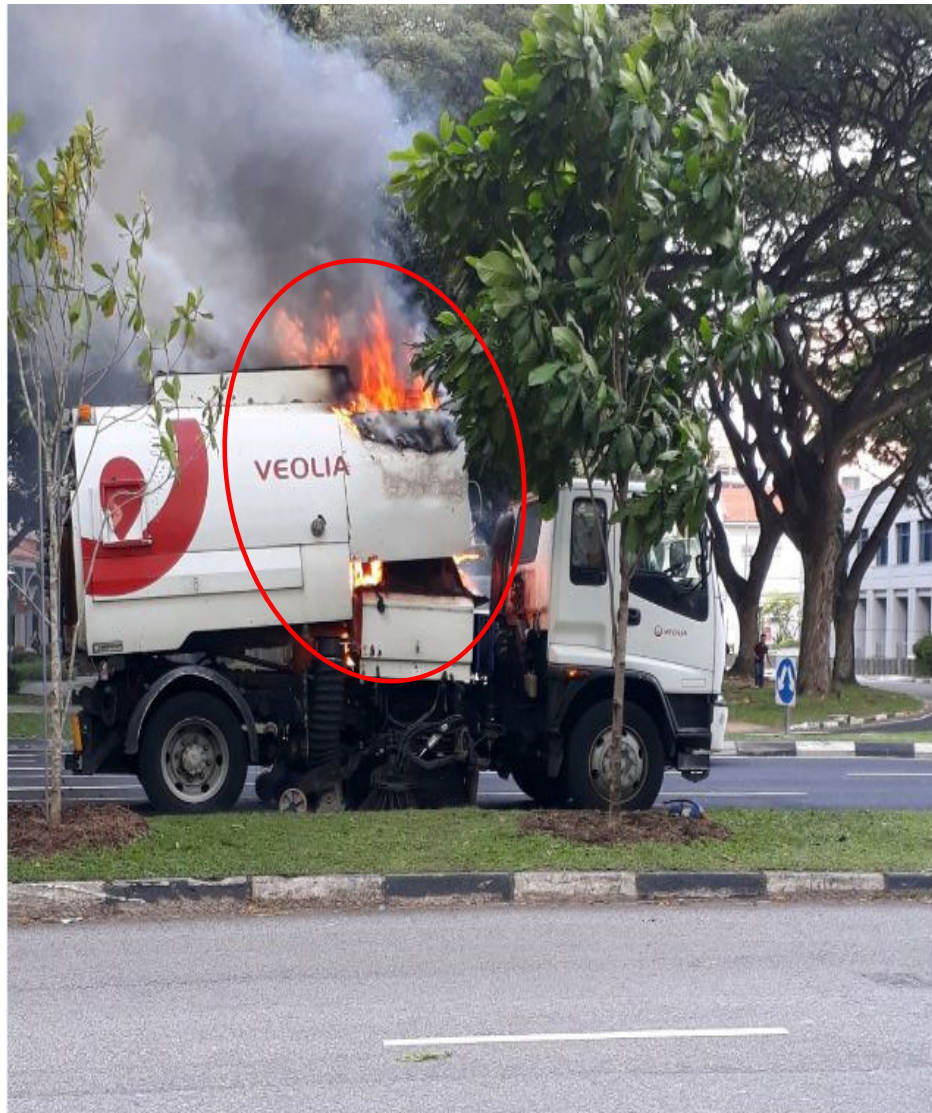
Photo 22 shows the left centre portion of the Insured Vehicle engulfed in flames before the arrival of the SCDF. In general, the information gathered from this photograph had corresponded to Ms Khairil's statement, which is the fire started from the left portion of the sub engine and that he tried to raise the sub engine compartment but it could not be raised fully (circled).
