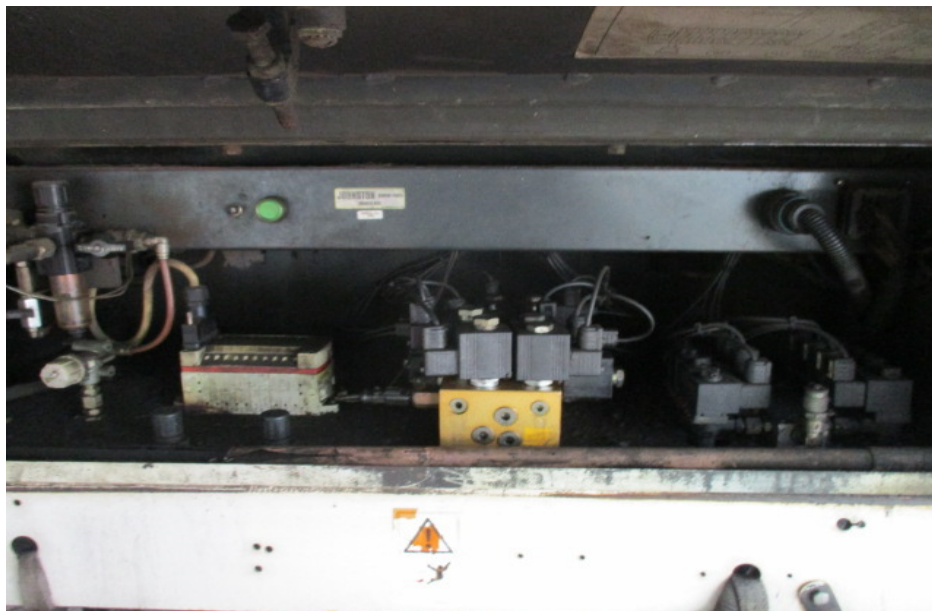
Photo 10 shows a closer view of the external control panel which is used to raise the sub engine compartment of the Insured Vehicle to reveal the sub engine under normal operational conditions. However due to the fire affecting the electrical system of the Insured Vehicle, we were unable to gain access to the sub engine to access the degree of fire damage.
