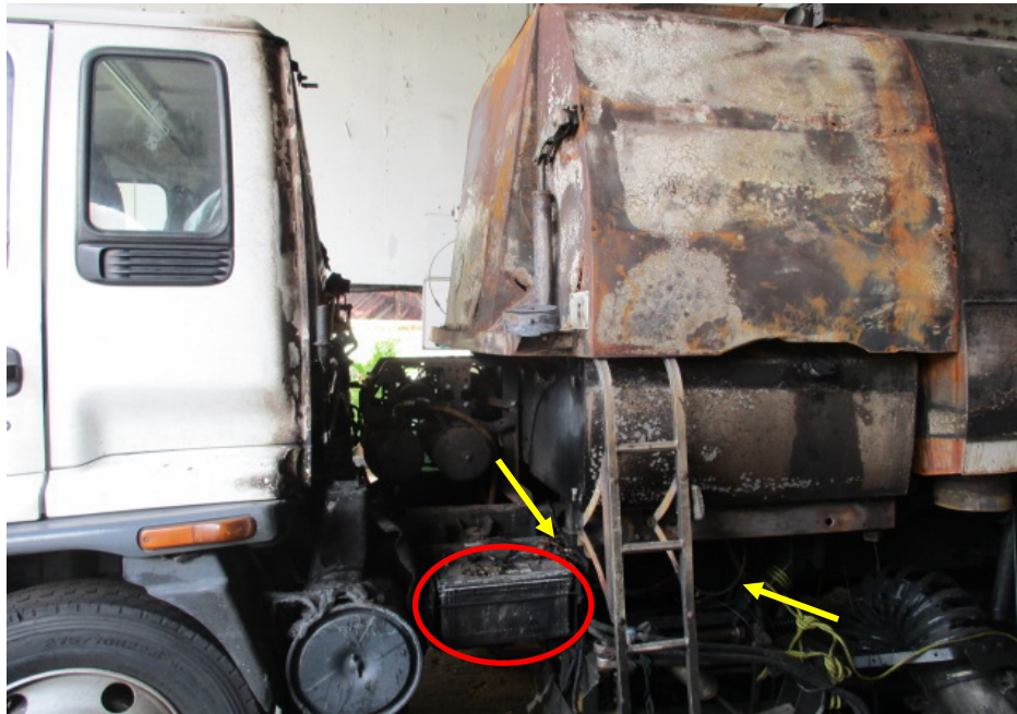
Photo 14 shows the several stretches of burnt wirings leading from the battery (circled) of the Insured Vehicle which had traces of greenish residue (arrowed). The presence of such greenish residue suggests occurrence of an electrical short circuit.
