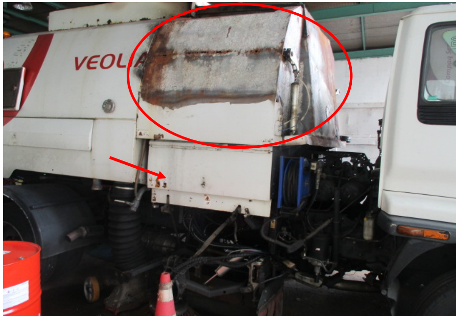
Photo 9 shows the right portion of the sub engine compartment which was badly burnt as a result of the fire (circled). Under normal operational conditions, the sub engine compartment of the Insured Vehicle can be raised to reveal the sub engine via an external control panel which is located at the right centre portion of the Insured Vehicle (arrowed).
