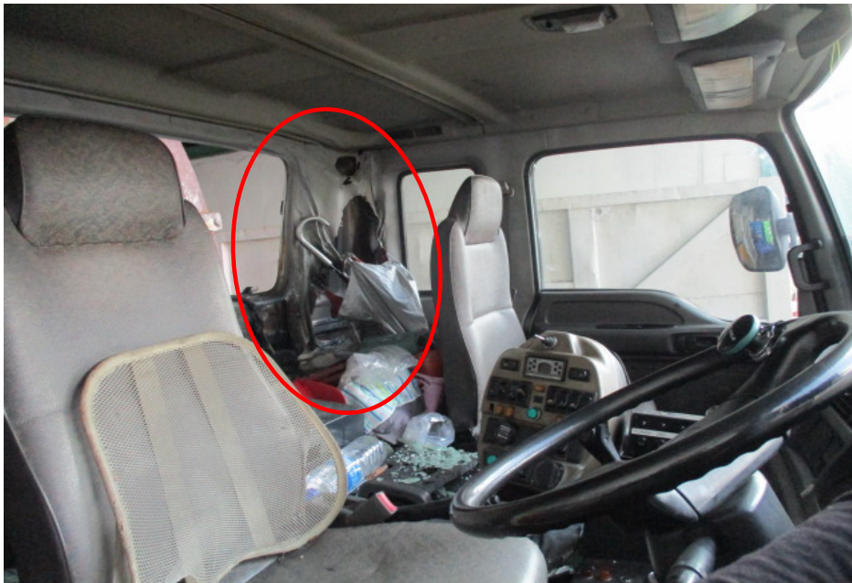
Photo 6 shows the interior compartment of the Insured Vehicle at the time of inspection. The rear portion of the interior compartment was significantly affected by the fire (circled).
