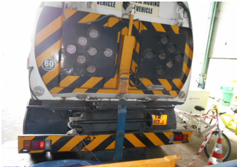
Photo 4 shows the rear portion of the Insured Vehicle at the time of our inspection. The fire damage to the Insured Vehicle was confined to its centre portion. The rear portion was observed to have been unaffected by the fire.
