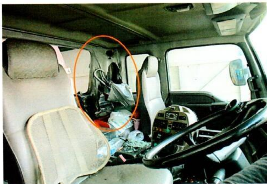
Photo 6 shows the interior compartment of the Insured Vehicle at the time of inspection. The rear portion of the interior compartment was significantly affected by the fire (circled).
