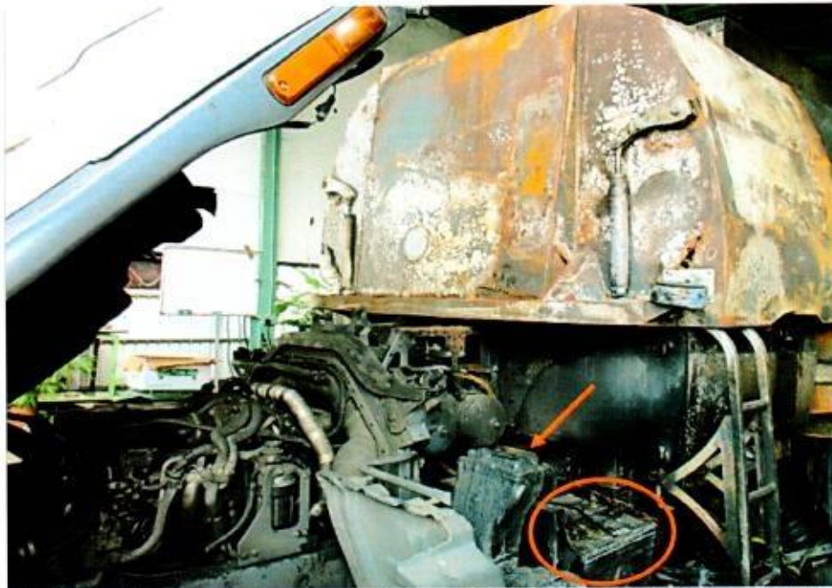
Photo 11 shows upon closer examination around the areas in closest proximity to the sub engine which was where the fire to the Insured Vehicle had likely started, we had found several stretches of burnt wiring with greenish residue. These wirings were original factory fitted wirings below the sub engine compartment (arrowed). We also found traces of greenish residue on several stretches of burnt wiring leading from the battery of the Insured Vehicle (circled). The presence of such greenish residue suggests occurrence of an electrical short circuit.
