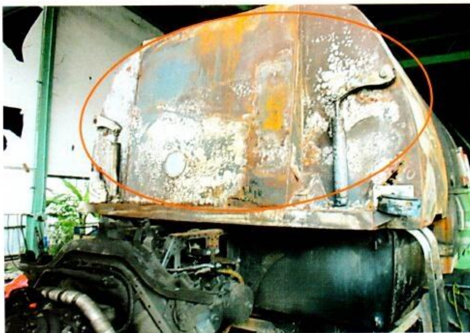
Photo 8 shows the sub engine compartment of the Insured Vehicle where the burn pattern and whitish burn marks were found (circled). Such whitish burn marks are a result of exposure to prolonged heat intensity, which had caused the steel/metal material of the sub engine compartment to be exposed to natural environmental condition. Hence the rust that had developed around the sub engine compartment of the Insured Vehicle is an indication that the fire to the Insured Vehicle had originated from the sub engine.
