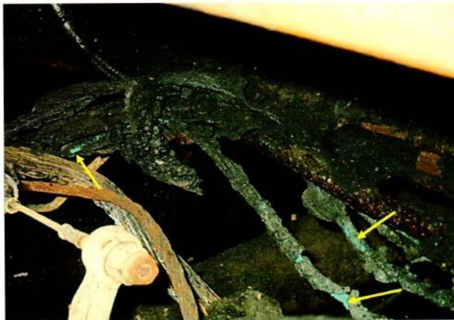
Photo 13 shows a close up view of the greenish residue found on some of the burnt wirings below the sub engine compartment of the Insured Vehicle (circled). The presence of such greenish residue suggests occurrence of an electrical short circuit.
