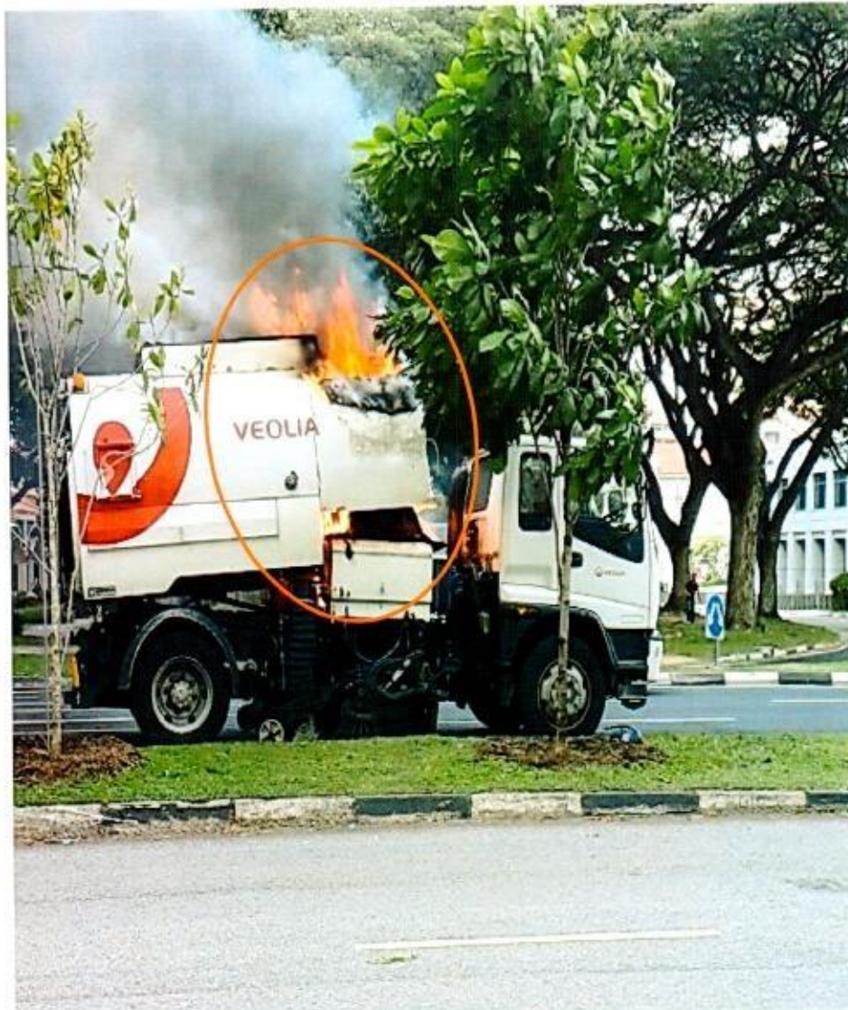
Photo 22 shows the left centre portion of the Insured Vehicle engulfed in flames before the arrival of the SCDF. In general, the information gathered from this photograph had corresponded to Ms Khairil's statement, which is the fire started from the left portion of the sub engine and that he tried to raise the sub engine compartment but it could not be raised fully (circled).
