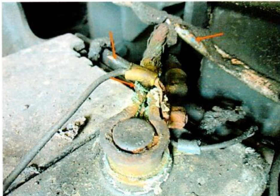
Photo 17 shows a close up view of the greenish residue found on some of the burnt wirings leading from the battery of the Insured Vehicle (arrowed). The presence of such greenish residue suggests occurrence of an electrical short circuit.
