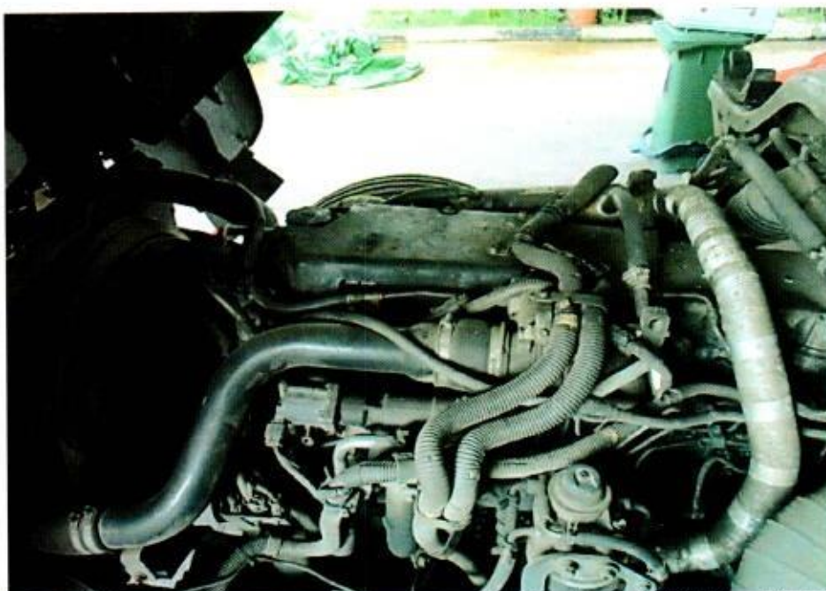
Photo 5 shows the main engine compartment of the Insured Vehicle which is situated beneath the front cabin at the time of our inspection. The main engine compartment of the Insured Vehicle was relatively unaffected by the fire.
