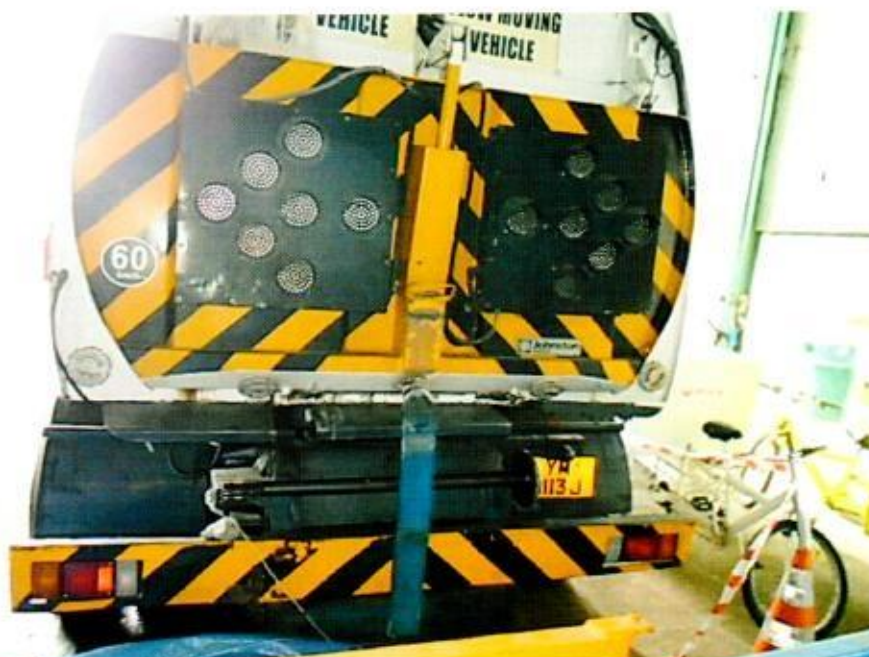
Photo 4 shows the rear portion of the Insured Vehicle at the time of our inspection. The fire damage to the Insured Vehicle was confined to its centre portion. The rear portion was observed to have been unaffected by the fire.
