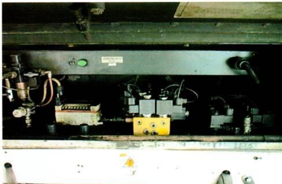
Photo 10 shows a closer view of the external control panel which is used to raise the sub engine compartment of the Insured Vehicle to reveal the sub engine under normal operational conditions. However due to the fire affecting the electrical system of the Insured Vehicle, we were unable to gain access to the sub engine to access the degree of fire damage.
