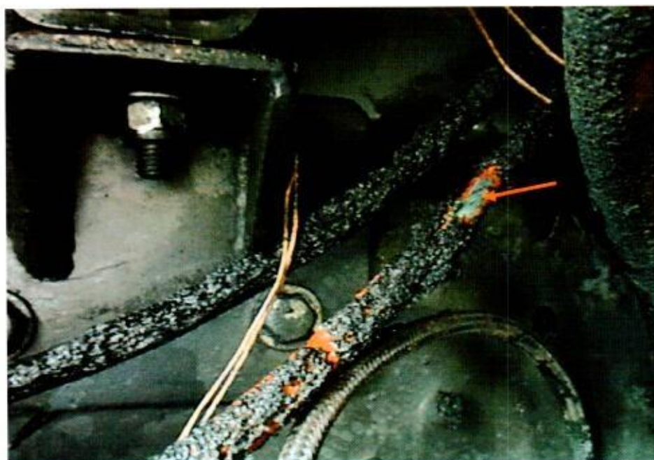
Photo 15 shows a closer view of the greenish residue found on some of the burnt wirings leading from the battery of the Insured Vehicle (arrowed). The presence of such greenish residue suggests occurrence of an electrical short circuit.
