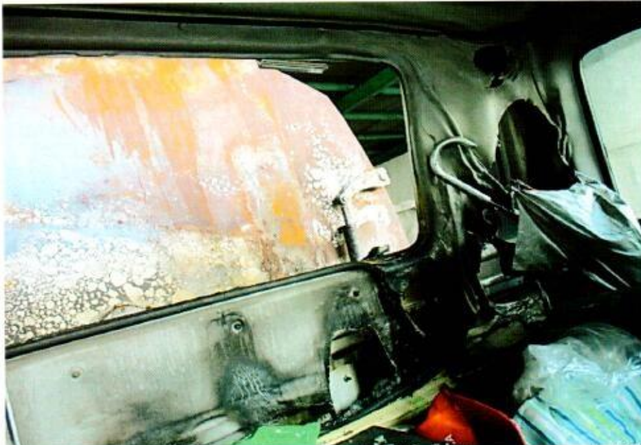
Photo 7 shows a closer view of the rear portion of the interior compartment which was significantly affected by the fire.
