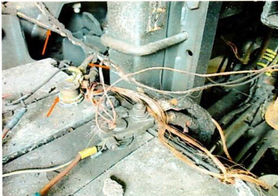
Photo 16 shows a closer view of the greenish residue found on some of the burnt wirings leading from the battery of the Insured Vehicle (arrowed). The presence of such greenish residue suggests occurrence of an electrical short circuit.
