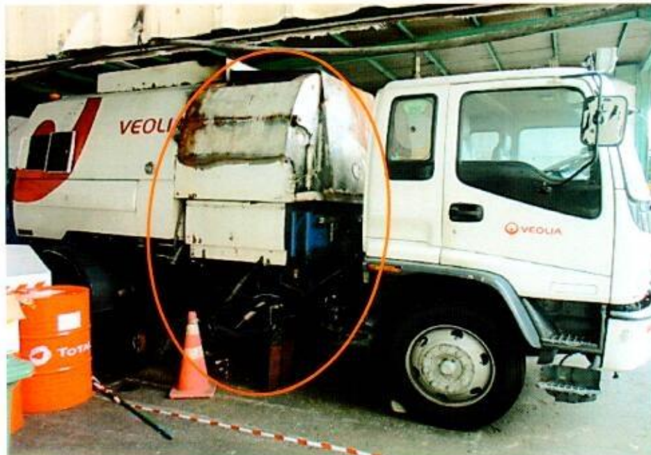
Photo 2 shows the right side of the Insured Vehicle at the time of our inspection. The exterior body of the Insured Vehicle was relatively unaffected by the fire except for the centre portion. The fire damage to the Insured Vehicle was confined to its centre portion (circled).
