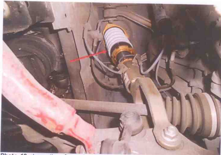
Photo 18 shows the aftermarket front left suspension (arrowed) of the insured vehicle. The insured vehicle was fitted with aftermarket front and rear suspension system.
