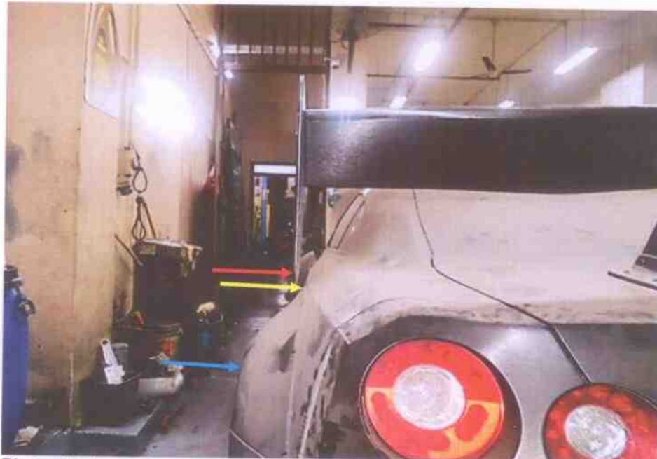
Photo 10 shows the rear spoiler (red arrow) protruding laterally out of the insured vehicle's main body (yellow arrow). This was at the rear left side of the insured vehicle. The additional body panel (blue arrow) for the wide body type of bodykit is fabricated and attached by bolts onto the main body of the insured vehicle, at the wheel arc area above the 4 wheels. Fitting such type of bodykits causes the insured vehicle to be wider laterally.
