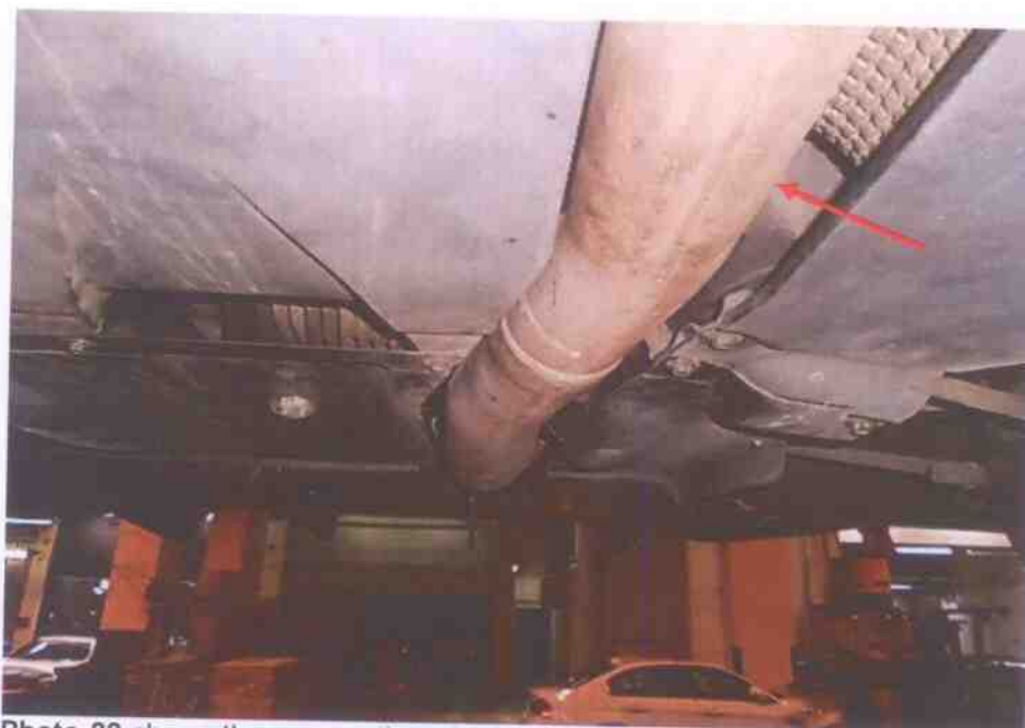
Photo 22 shows the rear section of the exhaust, from the middle pipe (arrowed) to the rear muffler. The rear section of the insured vehicle's exhaust system was observed to be an aftermarket type.
