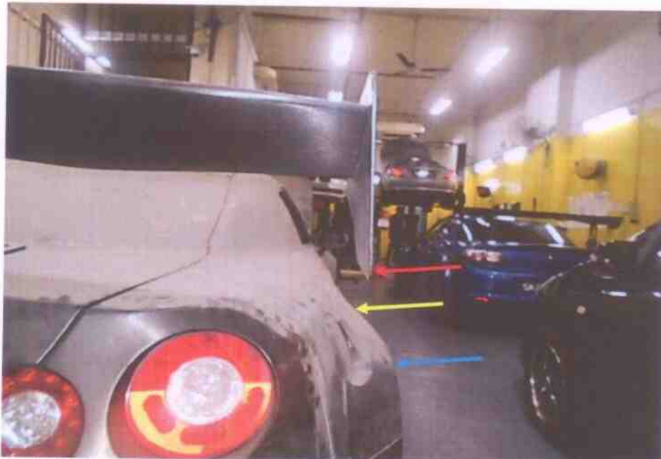
Photo 9 shows the rear spoiler (red arrow) protruding laterally out of the insured vehicle's main body (yellow arrow). This was at the rear right side of the insured vehicle. The additional body panel (blue arrow) for the wide body type of bodykit is fabricated and attached by bolts onto the main body of the insured vehicle, at the wheel arc area above the 4 wheels. Fitting such type of bodykits causes the insured vehicle to be wider laterally.
