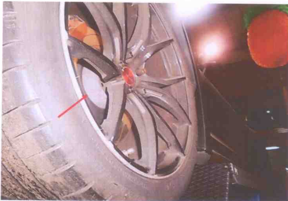
Photo 12 shows the wheel spacer (arrowed) that was additionally fitted at the front left wheel. Such wheel spacer was found to be fitted on all the 4 wheels of the insured vehicle, "pushing" the 4 wheels of the insured vehicle outwards, becoming flush with the protruded body line of the insured vehicle.
