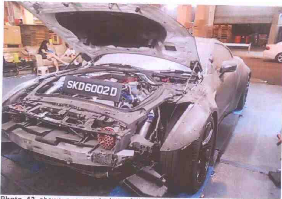
Photo 13 shows a general view of the engine compartment of the insured vehicle. Several modifications were found fitted in the engine compartment. This had included an aftermarket air intake system with all piping; an aftermarket intercooler; a non-original engine coolant reservoir tank; and some non-original fluid carry hoses.
