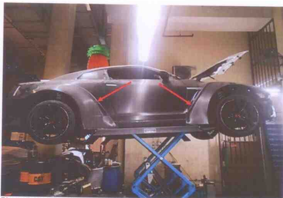
Photo 7 shows the insured vehicle hoisted during my inspection. Exteriorly the insured vehicle was observed to be fitted with a set of wide body type of bodykit. For such bodykits, an additional body panel (arrowed) is fabricated and attached by bolts onto the main body of the insured vehicle, at the wheel arc area above the 4 wheels. Fitting such type of bodykits causes the insured vehicle to be wider laterally.
