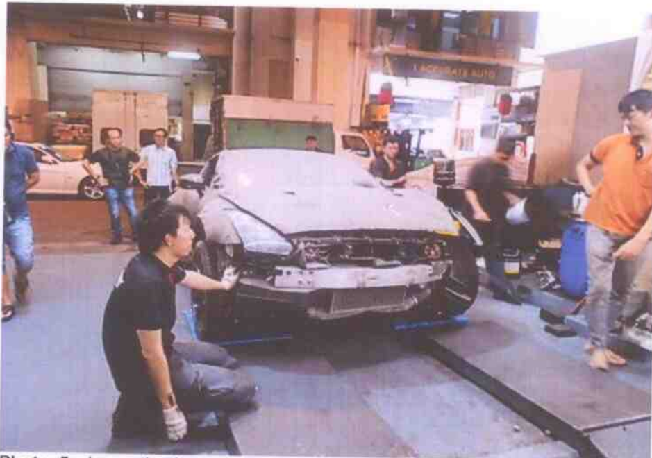
Photo 5 shows the insured vehicle being moved onto a hoist for a detailed inspection. Generally, the insured vehicle was observed to be of good condition. It had however sustained impact damages that were confined to its frontal portion. Its front bumper, front bonnet, front fenders and front headlamps were amongst the body parts that were observed to have been damaged.
