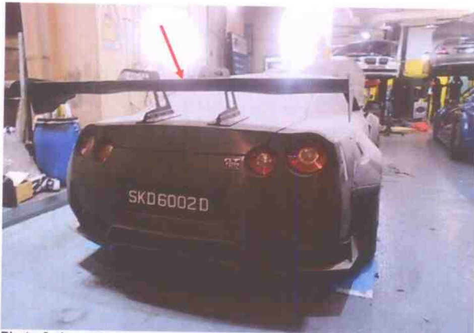
Photo 8 shows the rear spoiler (arrowed) fitted on the insured vehicle. The type of rear spoiler is commonly referred to as "GT wing". The overall length of the rear spoiler was observed to have laterally protruded out of the insured vehicle's main body.
