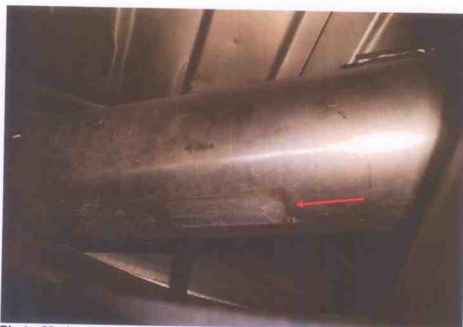
Photo 23 shows the rear muffler of the insured vehicle. The rear section of the insured vehicle's exhaust system, from the middle pipe to the rear muffler, was observed to be an aftermarket type. The tag (arrowed) of this aftermarket exhaust was intact and not tampered with.
