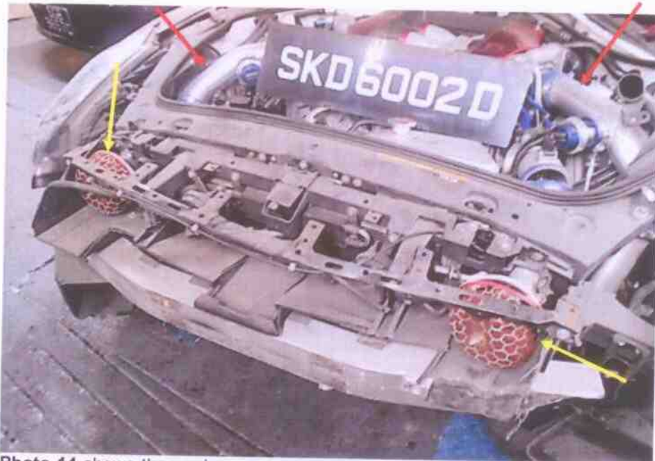
Photo 14 shows the engine compartment of the insured vehicle. An aftermarket air system was observed to be fitted on the insured vehicle. This had included non-original air filters (yellow arrow) and piping (red arrow).
