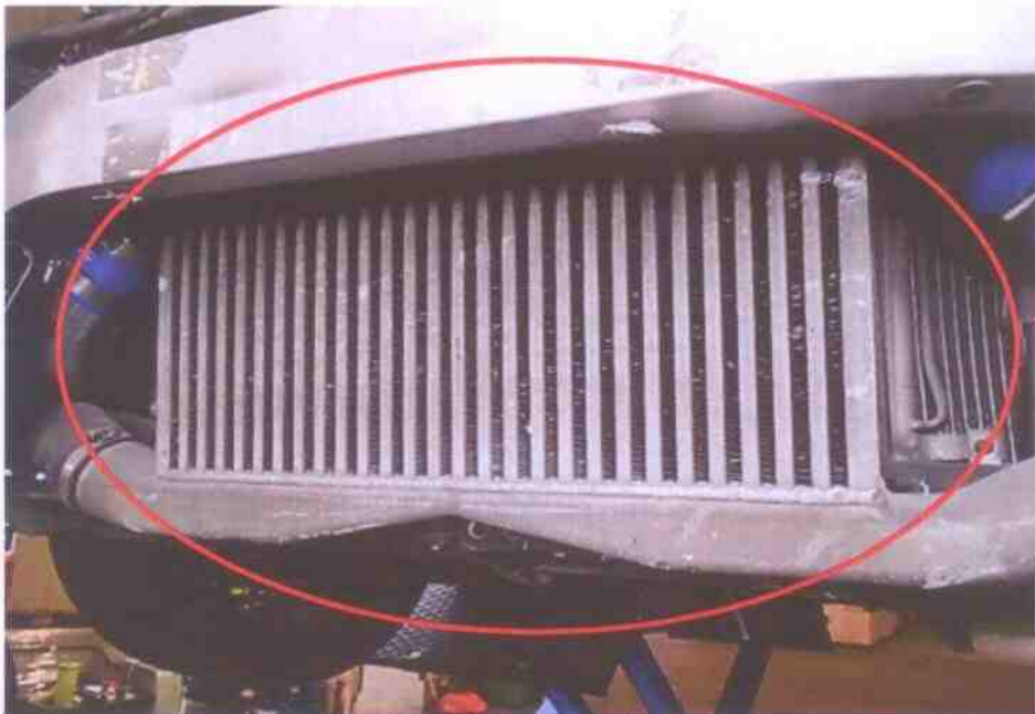
Photo 16 shows the aftermarket intercooler (circled) that was observed on the insured vehicle.
