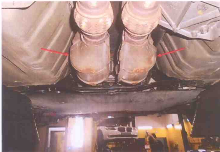
Photo 20 shows the catalytic converters (arrowed) of the insured vehicle. The catalytic converters and front sections of the exhaust were closely examined and I did not find any sign(s) or indication(s) of any weld mark(s) to suggest that the catalytic converters and/or front sections of the exhaust were tampered with.
