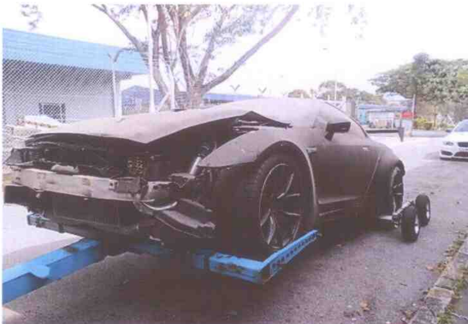
Photo 2 shows the insured vehicle at Traffic Police Pound prior to being towed to Teamwork Garage Pte Ltd. The method of towing was by, what is commonly referred to as king dolly method. Such method of towing is usually used when the towed vehicle is an all-wheel drive vehicle or rear wheel drive vehicle. The 4 wheels of the towed vehicle are lifted off ground during the towing.
