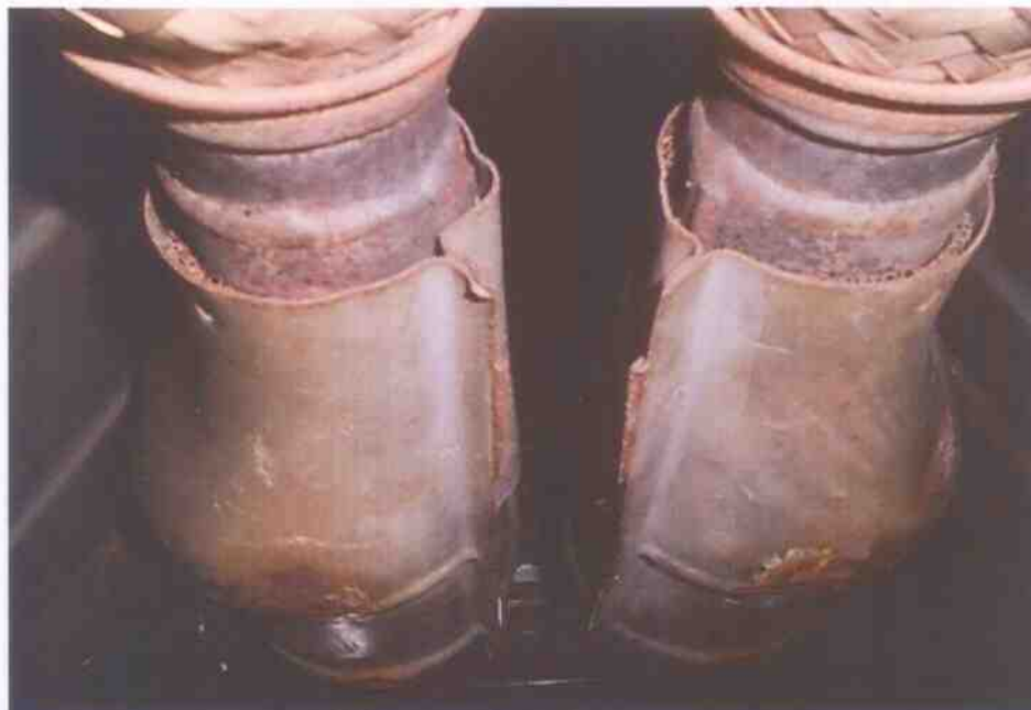
Photo 21 shows a closer view of the catalytic converters of the insured vehicle. The catalytic converters and front sections of the exhaust were closely examined and I did not find any sign(s) or indication(s) of any weld mark(s) to suggest that the catalytic converters and/or front sections of the exhaust were tampered with.
