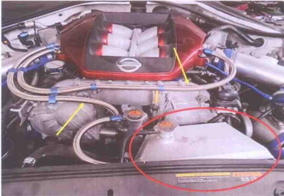
Photo 15 shows the engine compartment of the insured vehicle and the non-original engine coolant reservoir tank (circled) and some various non-original fluid carry hoses (yellow arrow).
