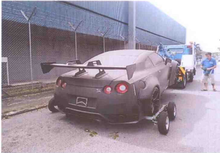
Photo 1 shows the insured vehicle at Traffic Police Pound prior to being towed to Teamwork Garage Pte Ltd. The method of towing was by, what is commonly referred to as king dolly method. Such method of towing is usually used when the towed vehicle is an all-wheel drive vehicle or rear wheel drive vehicle. The 4 wheels of the towed vehicle are lifted off ground during the towing.
