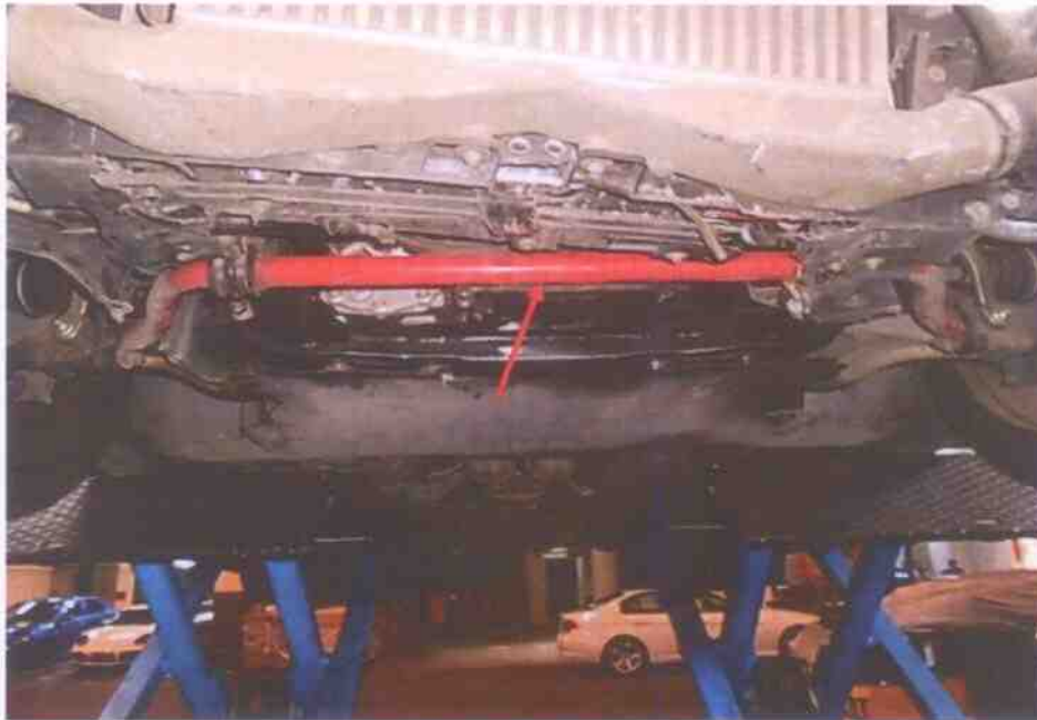
Photo 17 shows the aftermarket front anti-roll bar (arrowed) fitted on the insured vehicle.
