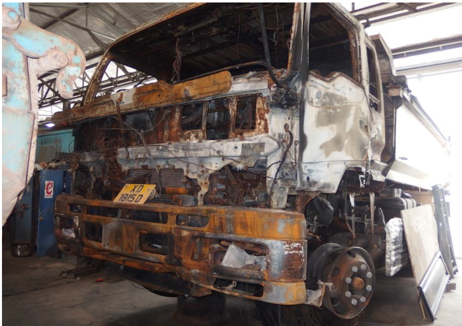
Photo 1 shows a general view of the front left body of the Insured Vehicle at the time of inspection. The Insured Vehicle was observed to have sustained extensive fire damage at its frontal portion. The body panels at the frontal portion were found to have been burnt to char.
