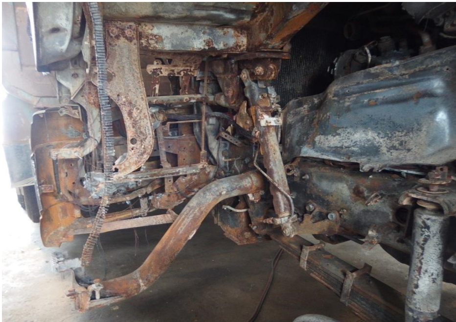
Photo 4 shows the underside of the Insured Vehicle, at its front left area. The various undercarriage components at the front underside of the Insured Vehicle was observed to be affected. This had included components of the braking system and steering system.
