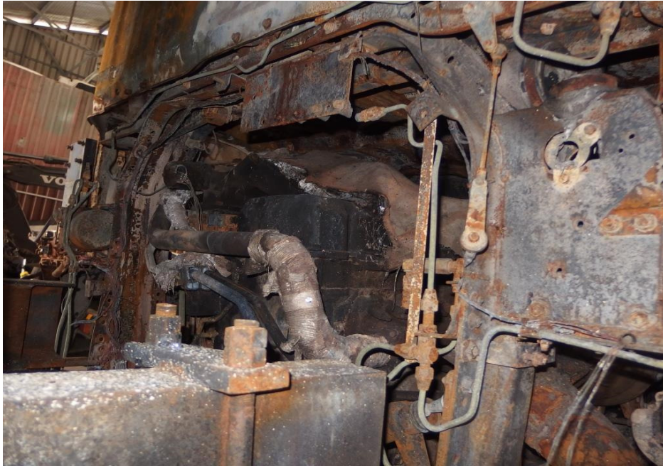
Photo 5 shows the engine compartment, which was located at the back of the Insured Vehicle's front cabin. The various parts and components within the engine compartment of the Insured Vehicle were all affected by the fire. This had included the engine of the Insured Vehicle.
