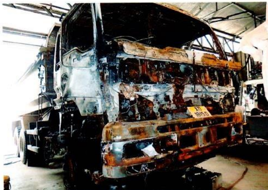
Photo 1 shows a general view of the front right body of the Insured Vehicle at the time of inspection. The Insured Vehicle was observed to have sustained extensive fire damage at its frontal portion. The body panels at the frontal portion and the undercarriage components at the front underside were found to have been burnt to char.
