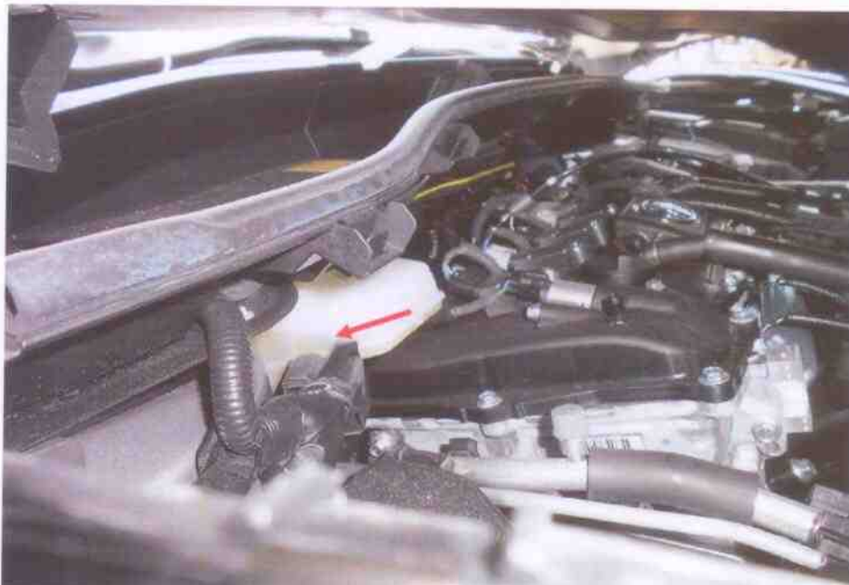
Photo 13 shows we had observed from the left side opening caused by the accident's impact that some visible parts and components inside the engine compartment to be intact and unaffected by the accident. Fluid component such as brake fluid was visible and found to be of sufficient level for operating purposes. Visually, there was also no contamination found to this fluid.
