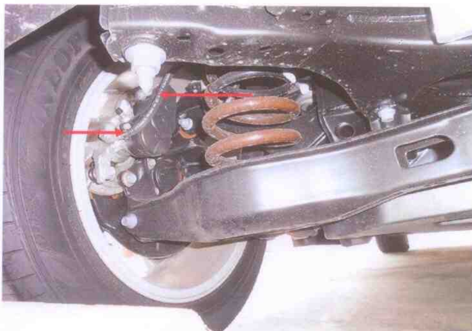
Photo 17 shows the brake hose (arrowed) at the rear left wheel of the Motor Car. Our visual inspection of the various mechanical components of the Motor Car's braking system revealed all to be intact and without visible damage, indicating that the braking system was likely to be in serviceable condition at the material time of accident.
