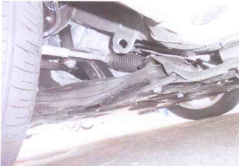
Photo 16 shows our subsequent checks on the underside of the Motor Car also revealed no fluid stain. Visually, the various undercarriage components of the Motor Car were all observed to be intact and without any visible damage.
