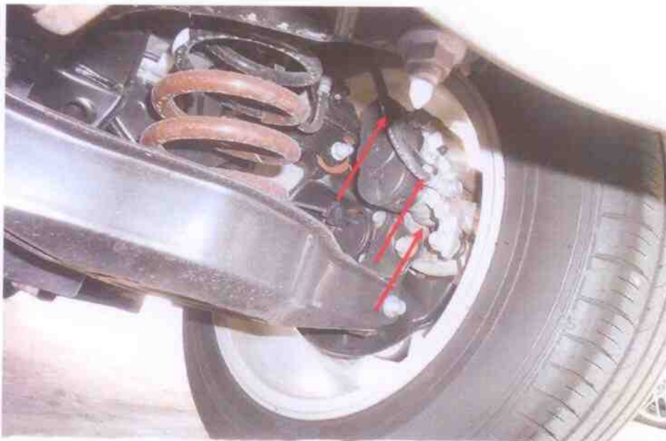
Photo 20 shows the various undercarriage components at the rear right wheel of the Motor Car. We did not observe any leakage of brake fluid at the time of our inspection of the Motor Car. Our visual inspection of the various mechanical components of the Motor Car's braking system revealed all to be intact and without visible damage, indicating that the braking system was likely to be in serviceable condition at the material time of accident.
