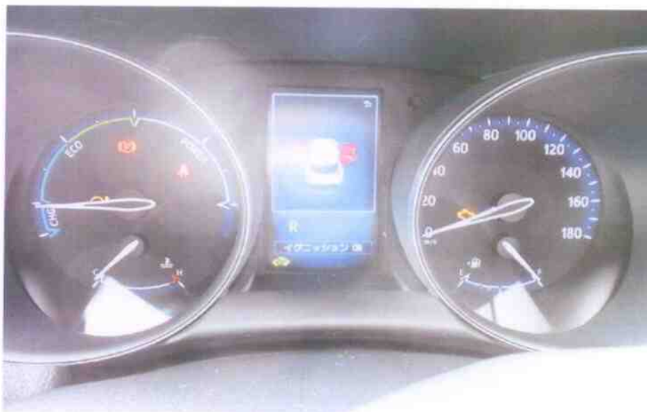
Photo 1 shows the mileage of the Motor Car at the time of our inspection was not recorded due to the Motor Car's system malfunction likely due to the accidents collision impact.
