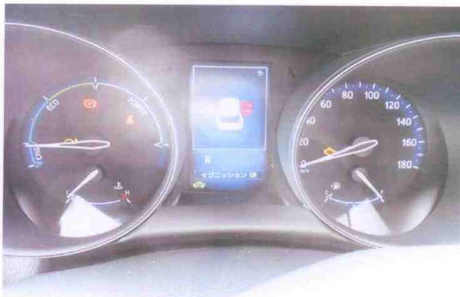
Photo 23 shows the warning indicators were observed to be lighted up upon pressing on the start button but no cranking of engine was observed. It was observed to be stuck to the 'Reverse Mode' even after we shifted to other modes. This indicates that the Motor Car electronic systems were malfunction likely due to the accident's collision impact.
