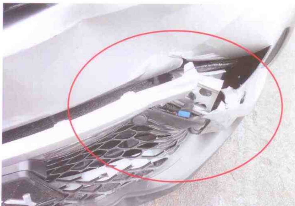
Photo 6 shows a close up view of the front left lower bumper of the Motor Car at the time of our inspection. It had sustained damages likely due to the accident.
