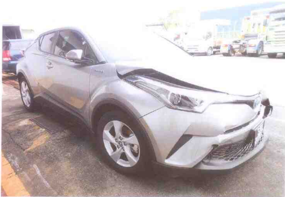
Photo 3 shows a general view of the front right body of the Motor Car at the time of our inspection. The Motor Car was observed to have sustained relatively minor damages at the frontal, front left & front right portion.
