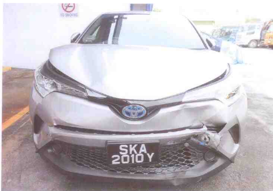
Photo 2 shows a general view of the front body of the Motor Car at the time of our inspection. The Motor Car was observed to have sustained relatively minor damages at the frontal, front left & front right portion.
