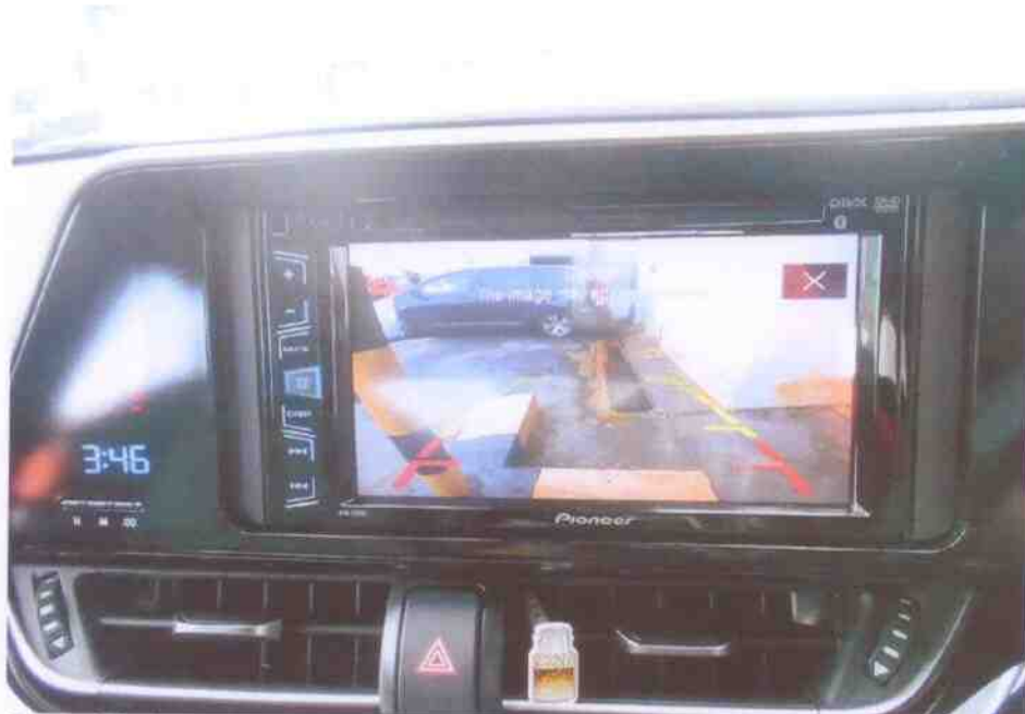
Photo 24 shows the reverse camera showed the rear view upon pressing on the start button but no cranking of engine was observed. It was observed to be stuck to the 'Reverse Mode' even after we shifted to other modes. This indicates that the Motor Car electronic systems were malfunction likely due to the accident's collision impact.
