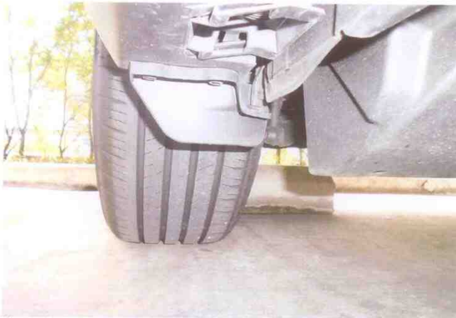
Photo 11 shows the condition of the rear right tyre of the Motor Car, which was observed to be in serviceable condition with remaining tread depth of approximately 7mm. The tyre was also observed to be sufficiently inflated for vehicular operation.
