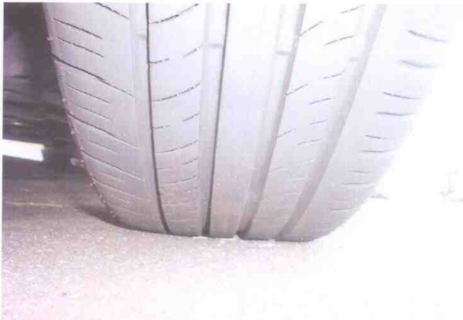
Photo 8 shows the condition of the front left tyre of the Motor Car, which was observed to be in serviceable condition with remaining tread depth of approximately 7mm. The tyre was also observed to be sufficiently inflated for vehicular operation.
