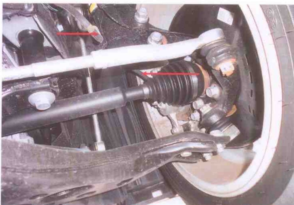
Photo 18 shows the brake hose (arrowed) at the front right wheel of the Motor Car. Our visual inspection of the various mechanical components of the Motor Car's braking system, including its brake calliper, revealed all to be intact and without visible damage, indicating that the braking system was likely to be in serviceable condition at the material time of accident.
