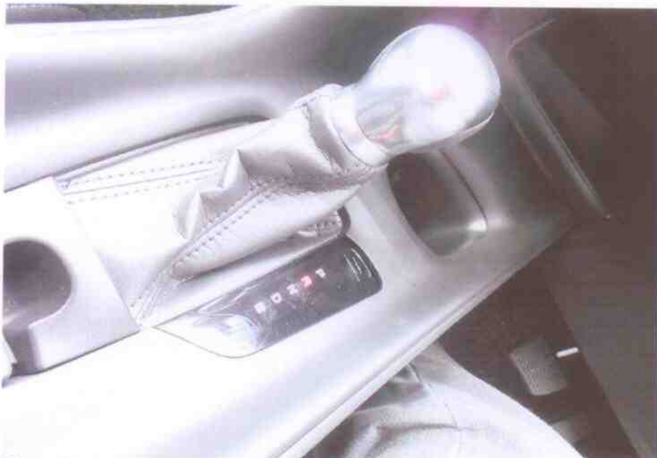
Photo 25 shows the gear knob was shifted to the 'Parking Mode' but the indicator still showed the 'Reverse mode'. Upon pressing on the start button but no cranking of engine was observed. It was observed to be stuck to the 'Reverse Mode' even after we shifted to other modes. This indicates that the Motor Car electronic systems were malfunction likely due to the accident's collision impact.
