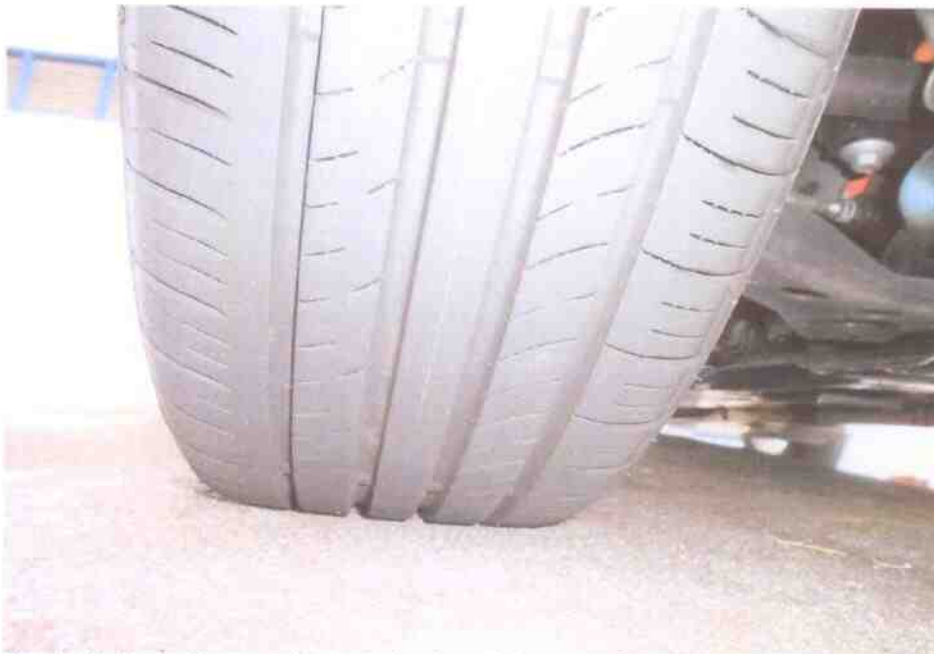
Photo 9 shows the condition of the front right tyre of the Motor Car, which was observed to be in serviceable condition with remaining tread depth of approximately 6mm. The tyre was also observed to be sufficiently inflated for vehicular operation.
