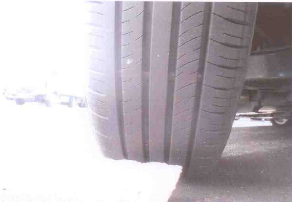
Photo 10 shows the condition of the rear left tyre of the Motor Car, which was observed to be in serviceable condition with remaining tread depth of approximately 7mm. The tyre was also observed to be sufficiently inflated for vehicular operation.
