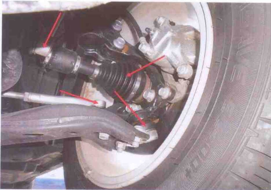
Photo 19 shows the various undercarriage components at the front left wheel of the Motor Car, in particular the steering tie rod (arrowed). The various steering components were all found to be intact, suggesting that the steering system of the Motor Car was likely to be in serviceable condition.
