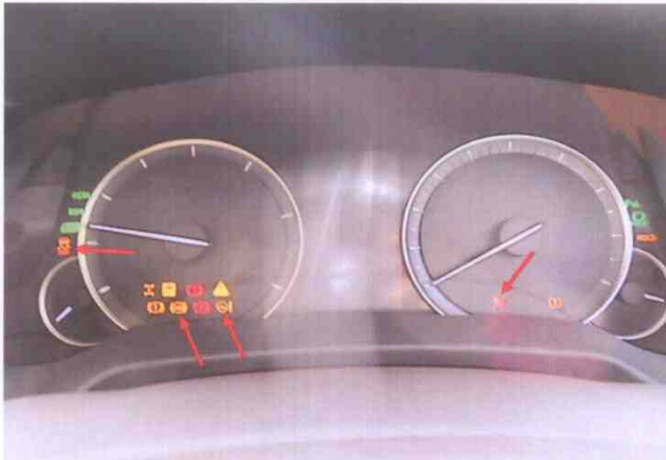
Photo 7 shows the warning light for Anti-Lock Brake System (ABS), Electric Power Steering System (EPS), Traction Control (TC) and Supplemental Restraint System (SRS) appearing on the instrument panel of the motor car during the self-test of its various electronic operating systems when its engine was cranked.
