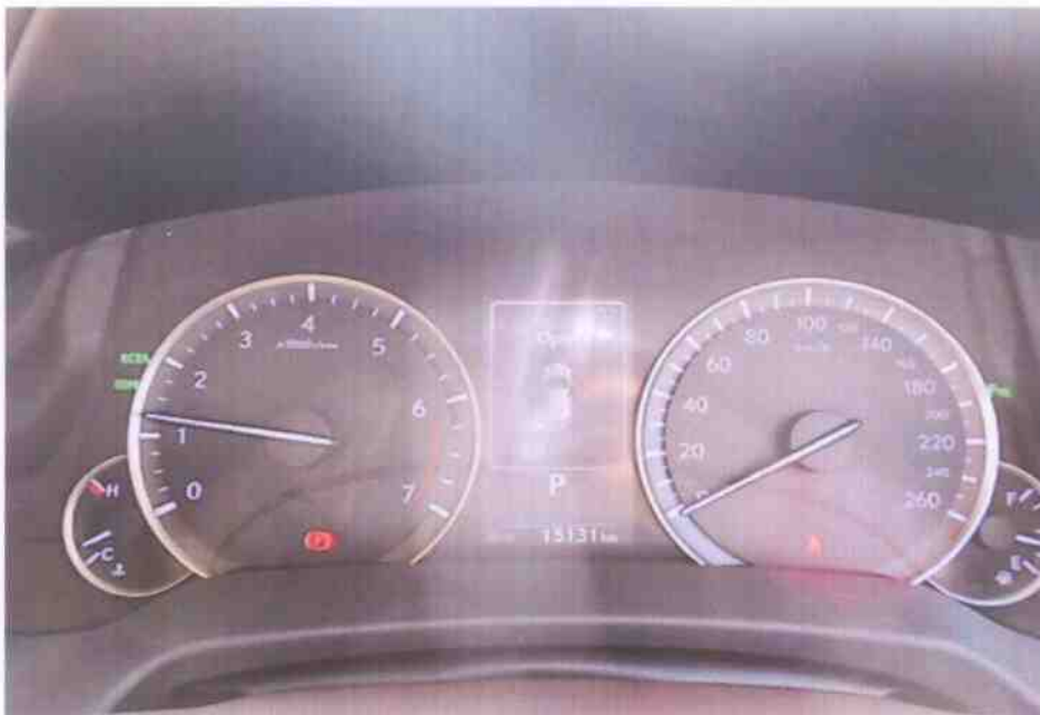
Photo 8 shows no warning lights illuminated on the instrument panel of the motor car after the engine was cranked. This would suggest that there was no abnormality to the various electronic operating systems of the motor car, like the ABS, EPS, TC and SRS etc.
