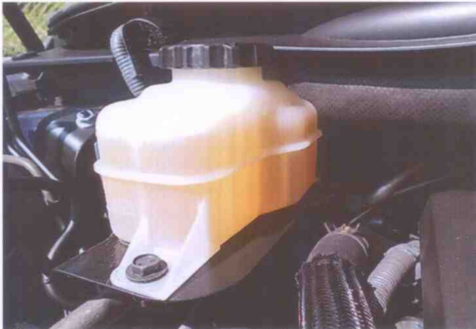
Photo 5 shows the brake fluid reservoir of the motor car at the time of my inspection. The brake fluid was observed to be of sufficient level for operating purposes and without any visible contamination.
