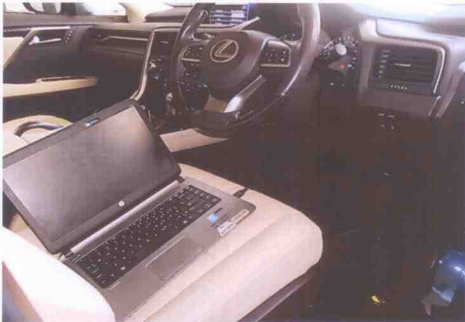
Photo 9 shows an electronic scan being carried out to the motor car to primarily check whether there was any electronic fault recorded in the various control modules of the motor car like the engine control module and transmission control module amongst others.
