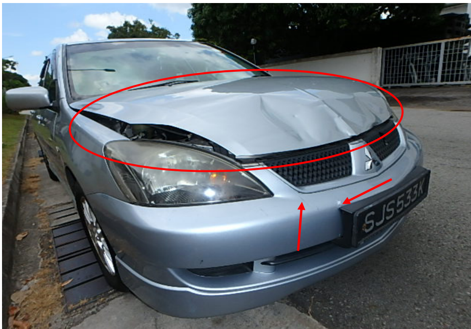
Photo 6 shows the general front view of the Insured Vehicle during the physical inspection at CHM. The Insured Vehicle had sustained damages to its front bumper (arrowed) and front bonnet. The front bonnet was observed to be buckled (circled). These damages seemed to corroborate with Ms Kaur's statement in which she might have been rear-ended by another vehicle, causing her to panic and accidentally stepping on the accelerator which resulted in the front portion of the Insured Vehicle going under the rear portion of the Lorry
