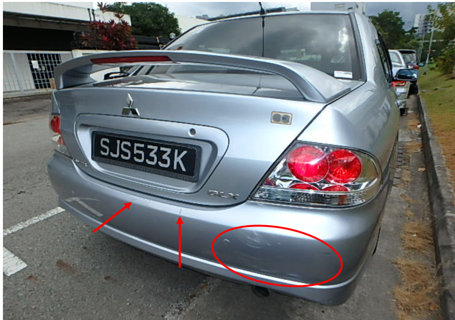
Photo 3 shows the general rear view of the Insured Vehicle during the physical inspection at CHM. Paint graze marks were found at the centre portion of the rear bumper (arrowed) and paint cracks were found at the right portion of the rear bumper. (circled).
