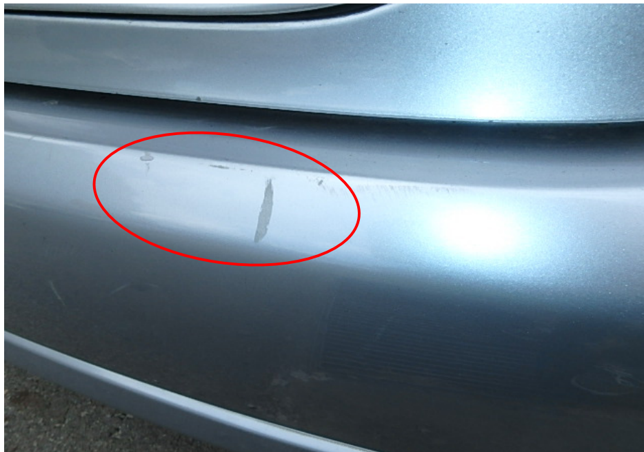
Photo 4 shows a close up view of the paint graze marks found at the centre portion of the rear bumper of the Insured Vehicle (circled), suggesting that the Insured Vehicle might have been rear-ended by another vehicle.
