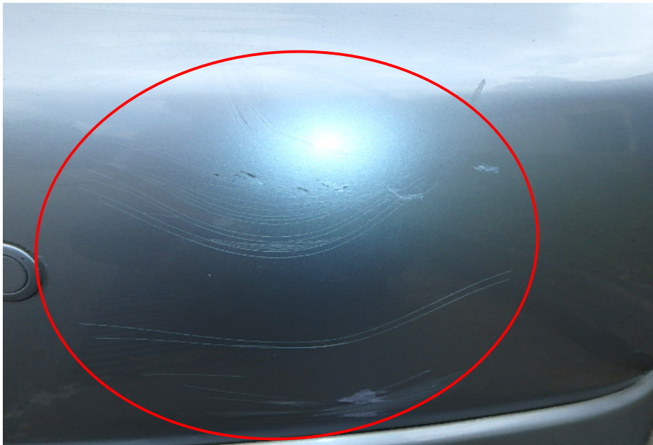
Photo 5 shows a close up view of the paint cracks found at the right portion of the rear bumper of the Insured Vehicle (circled), suggesting that the Insured Vehicle might have been rear-ended by another vehicle.
