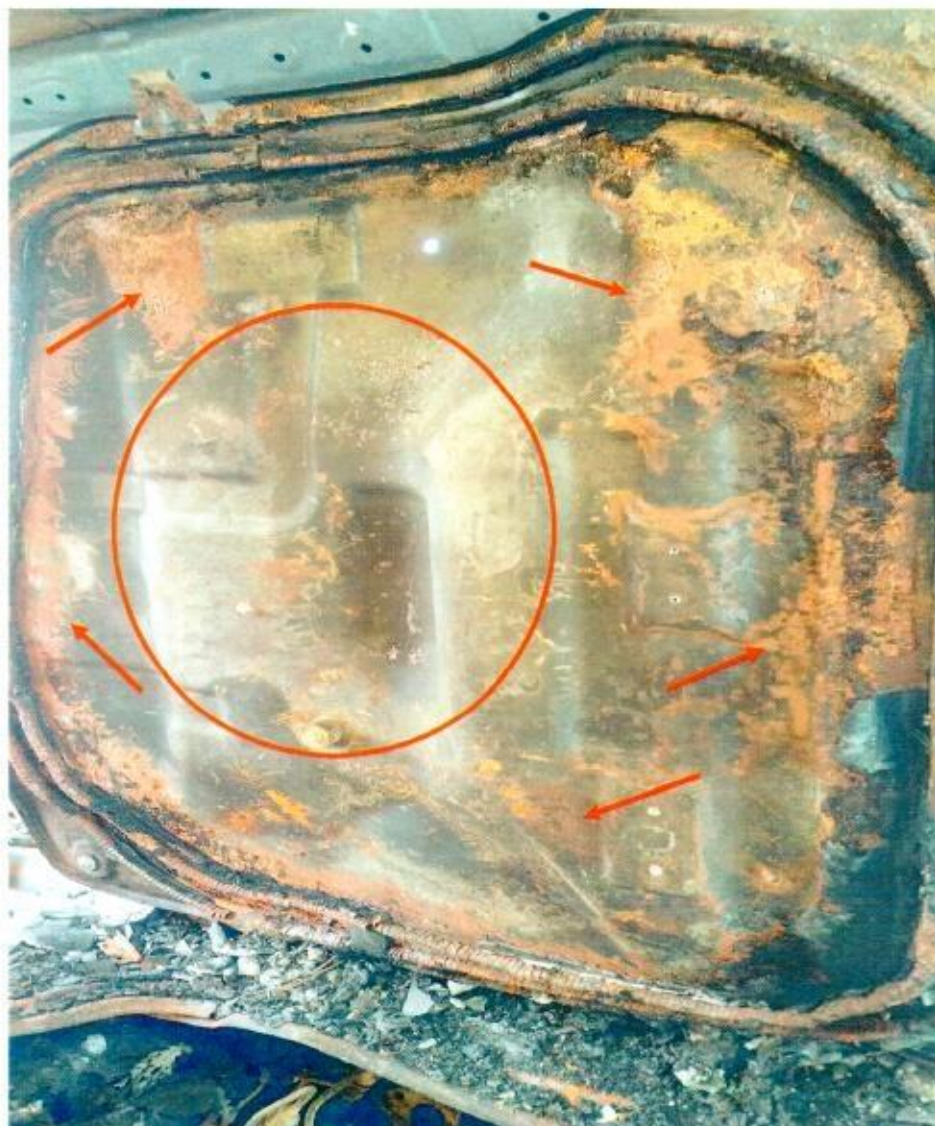
Photo 6 shows the whitish burn marks that were found on the underside of the passenger side engine access panel of the Insured Vehicle (circled). Such whitish burn marks are a result of exposure to prolonged heat intensity. Rust would also begin to develop on these areas soon after the fire. The development of rust is an indication that the area was exposed to prolonged exposure to high heat intensity, which had caused the steel/metal material of the passenger side engine access panel to be exposed to natural environmental condition. Hence the rust that had developed around the underside of the passenger side engine access panel of the Insured Vehicle (arrowed) is an indication that the fire to the Insured Vehicle had originated from the engine compartment.
