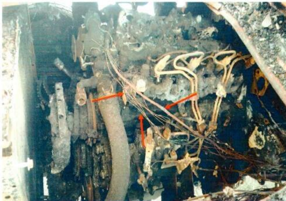
Photo 7 shows the wirings around the centre portion of the engine compartment which is near to the vicinity where the fire to the Insured Vehicle had likely started. We observed greenish residue on the wirings at the centre portion of the engine compartment (arrowed).
