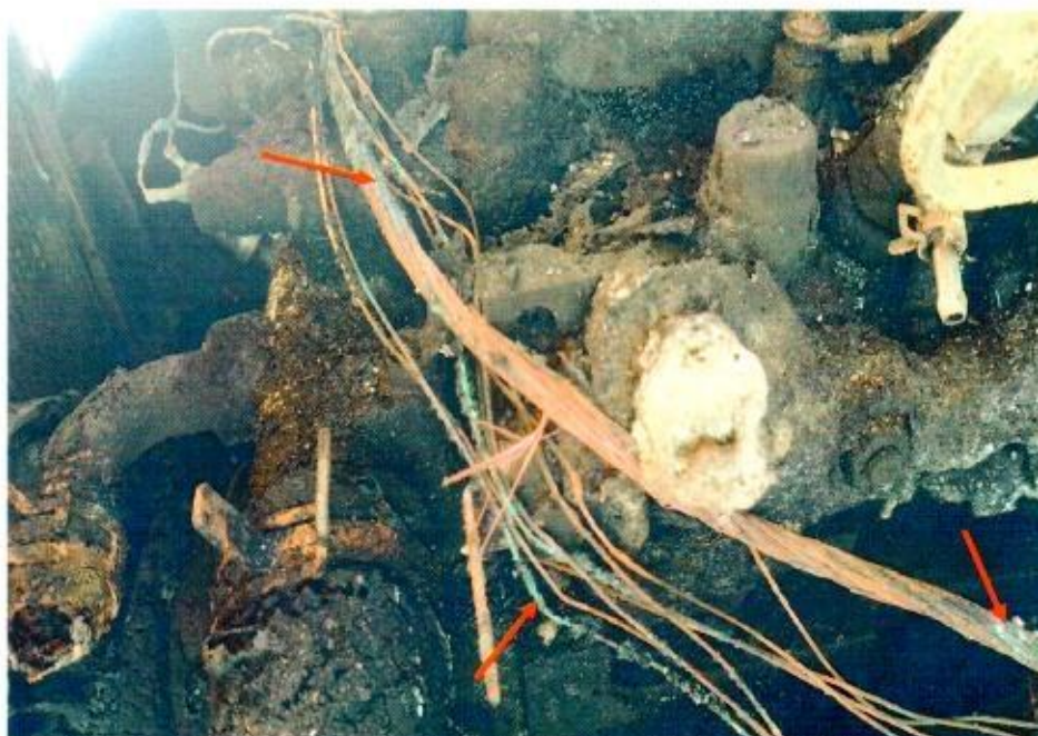
Photo 8 shows a closer view of the greenish residue found on the wirings at the centre portion of the engine compartment (arrowed). This seems to suggest the occurrence of an electrical short circuit.
