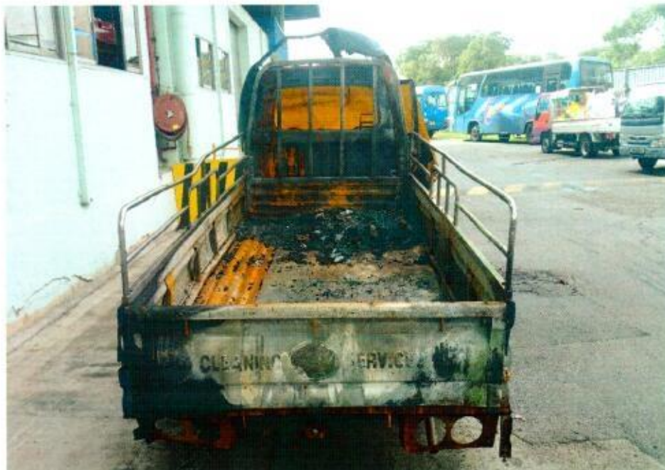
Photo 3 shows the general view of the rear body of the Insured Vehicle at the time of our inspection. The Insured Vehicle was observed to have sustained extensive fire damage all around. Rust had accumulated all over the Insured Vehicle as a result of exposure to environmental condition for a period of time.
