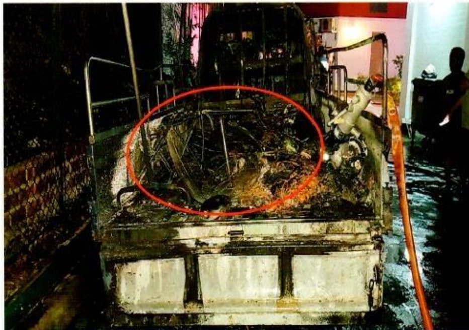
Photo 23 shows the rear portion of the Insured Vehicle after the fire was extinguished. In general, the information gathered from this photograph had corresponded to Ms Sharifah's statement, which is there was old furniture placed at the rear carriage deck of the Insured Vehicle when the fire started (circled).
