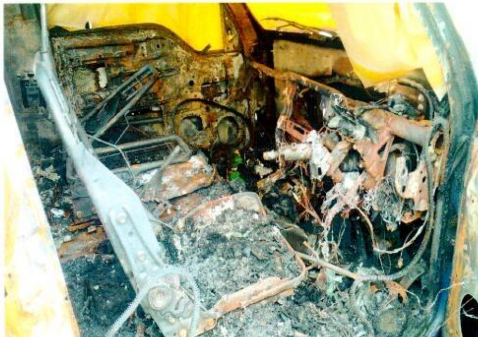
Photo 4 shows the general view of the interior compartment of the Insured Vehicle at the time of our inspection. Its interior compartment was completely burnt as a result of the fire.
