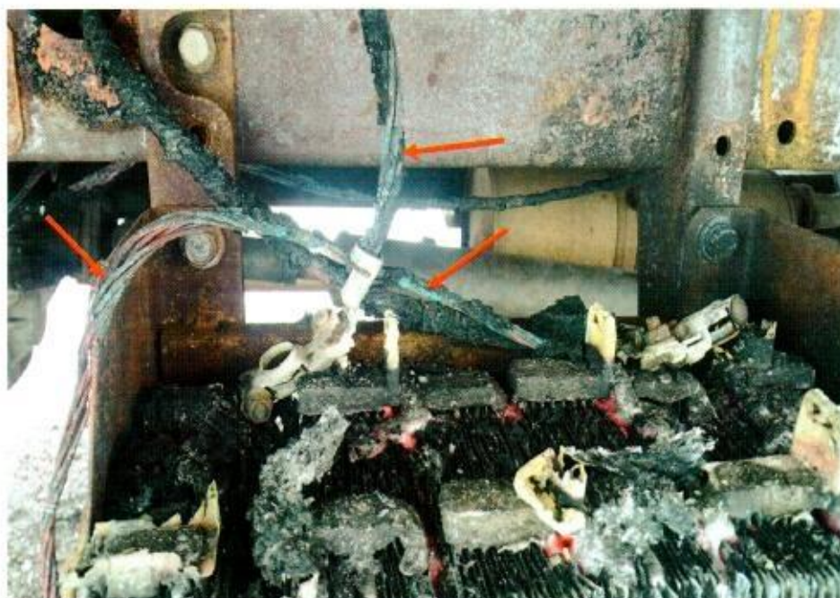
Photo 10 shows a close up view of the greenish residue found on the wirings leading from the battery of the Insured Vehicle (arrowed). This seems to suggest the occurrence of an electrical short circuit.
