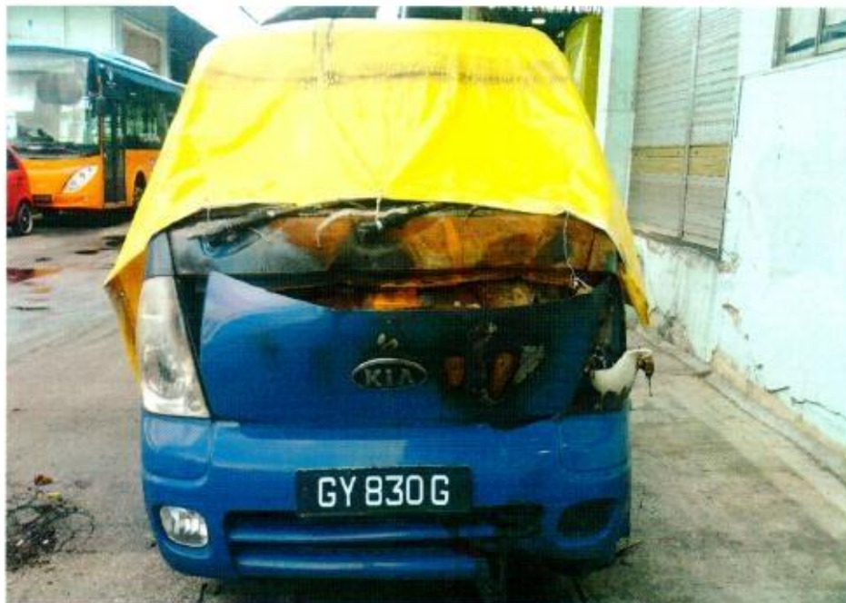
Photo 1 shows the general view of the front portion of the Insured Vehicle at the time of our inspection. The Insured Vehicle was observed to have sustained extensive fire damage all around. Its engine compartment and interior compartment were completely burnt. Rust had accumulated all over the Insured Vehicle as a result of exposure to environmental condition for a period of time.
