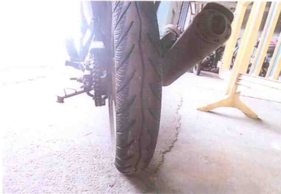
Photo 8 shows the rear tyre of the Motorcycle. The rear tyre was observed to be in serviceable condition with remaining tread depth of approximately 1.6mm. The tyre was also observed to be sufficiently inflated for vehicular operation.
