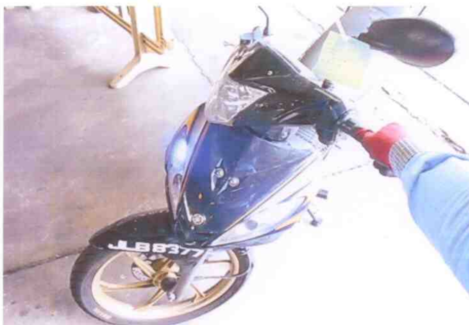
Photo 15 shows steering system test was conducted on the steering. It was observed to be in serviceable condition when we are able to turn the steering to the full left & right.
