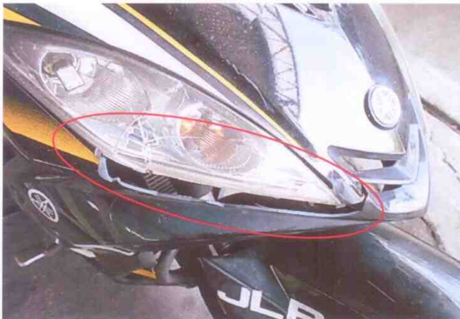
Photo 6 shows a closer view of the front right head lamp & front fairing of the Motorcycle at the time of our inspection. It was observed to be damage likely due to the accident. (Circled)
