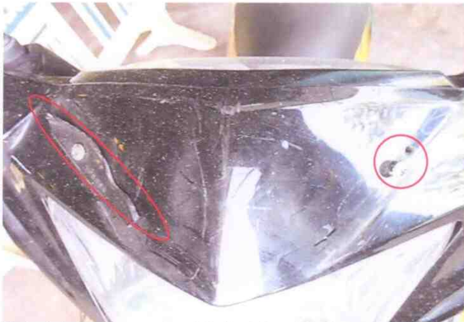
Photo 4 shows a close-up view of the front visor of the Motorcycle at the time of our inspection. It was observed to be broken & missing likely due to the accident.
