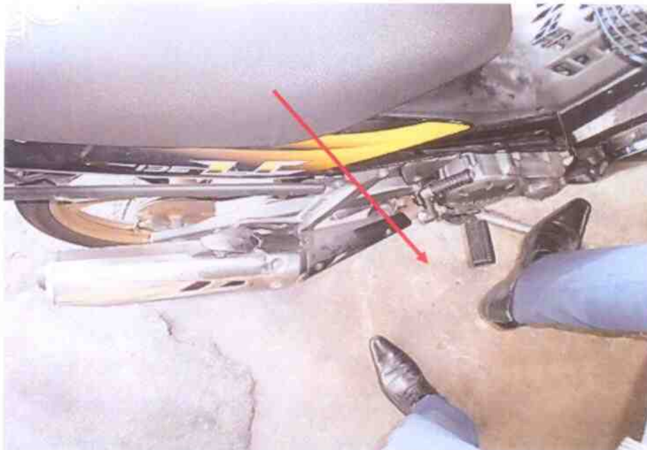
Photo 18 shows testing of the braking of the rear brake in progress. There was some resistance felt (spongy like feel) upon stepping on the brake pedal.
