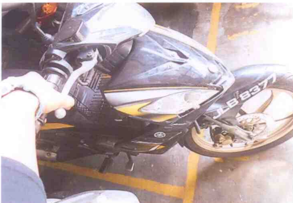
Photo 17 shows static testing of the braking of the front brake in progress. There was some resistance felt (spongy like feel) upon pressing the brake lever.
