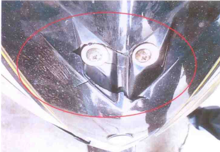
Photo 5 shows a close-up view of the front fairing of the Motorcycle at the time of our inspection. It was observed to be cracked likely due to the accident.
