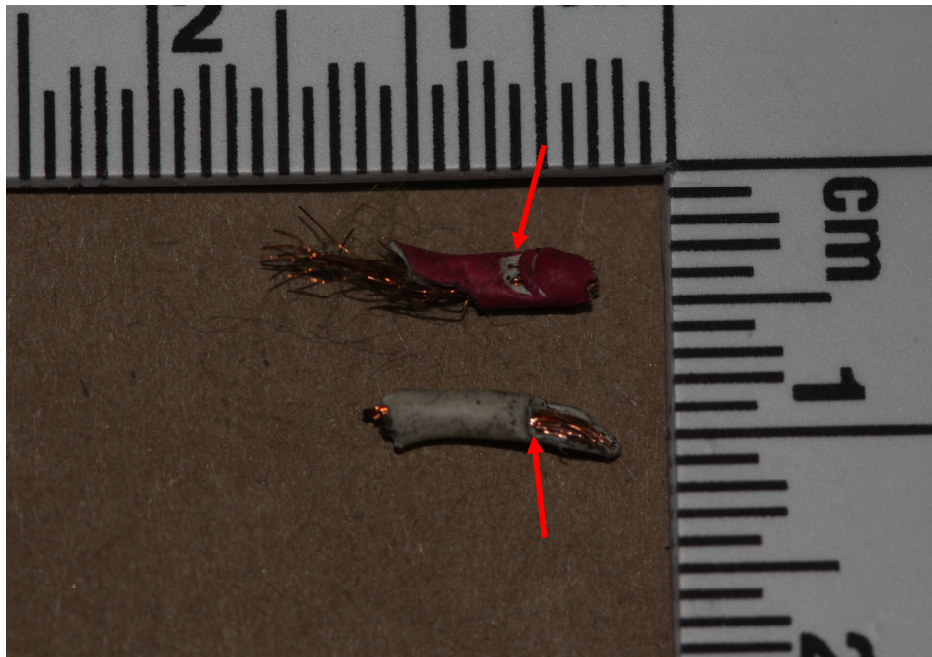
Photo 3 shows the affected sections of the wire that were cut completely and subsequently seized by the Police. The copper wires at the 2 areas where the wire was cut (arrowed) was noted to be unaffected.
