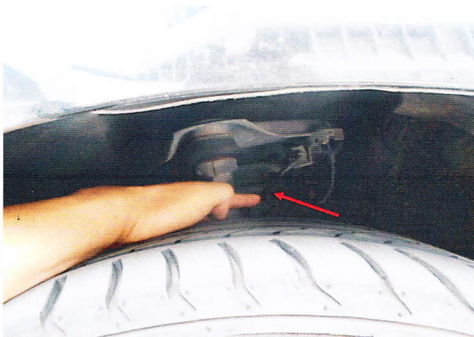
Photo 3 shows the cut wire, at the stretch where it was cut (arrowed). The wire is visible if one was to kneel or bend down at the front right tyre. I was also able to easily extend my hand to touch the wire, at the stretch where it was cut.
