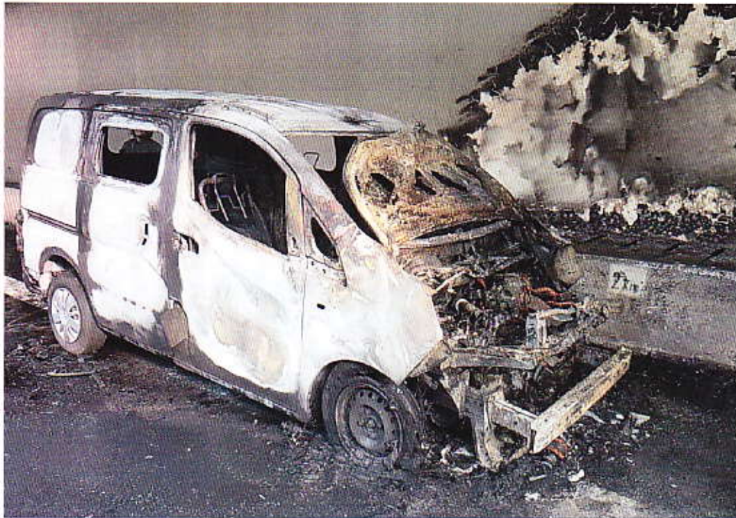
Photo 15 shows a general view of the Motor Vehicle's condition after the fire was extinguished. The fire burnt pattern mark was observed to be from the front portion.
