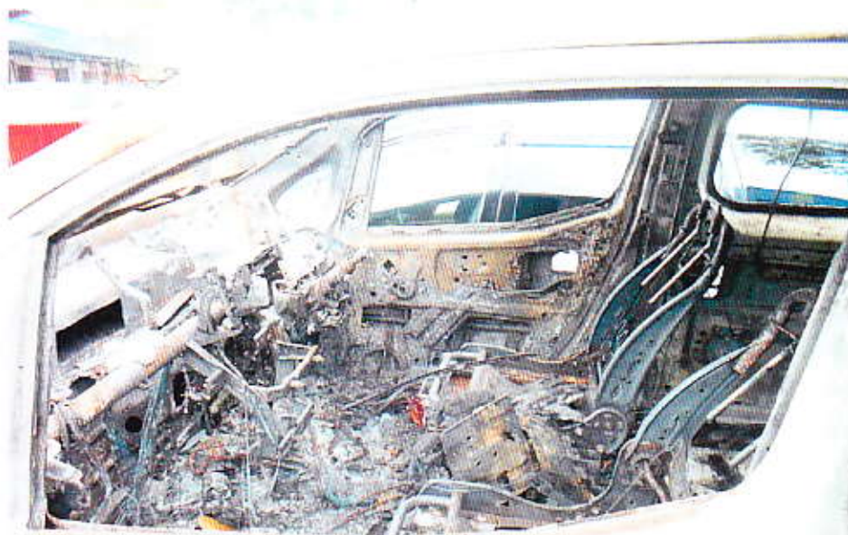
Photo 2 shows the interior view of the Insured vehicle, it was observed to have sustained with severe damages due to the fire.
