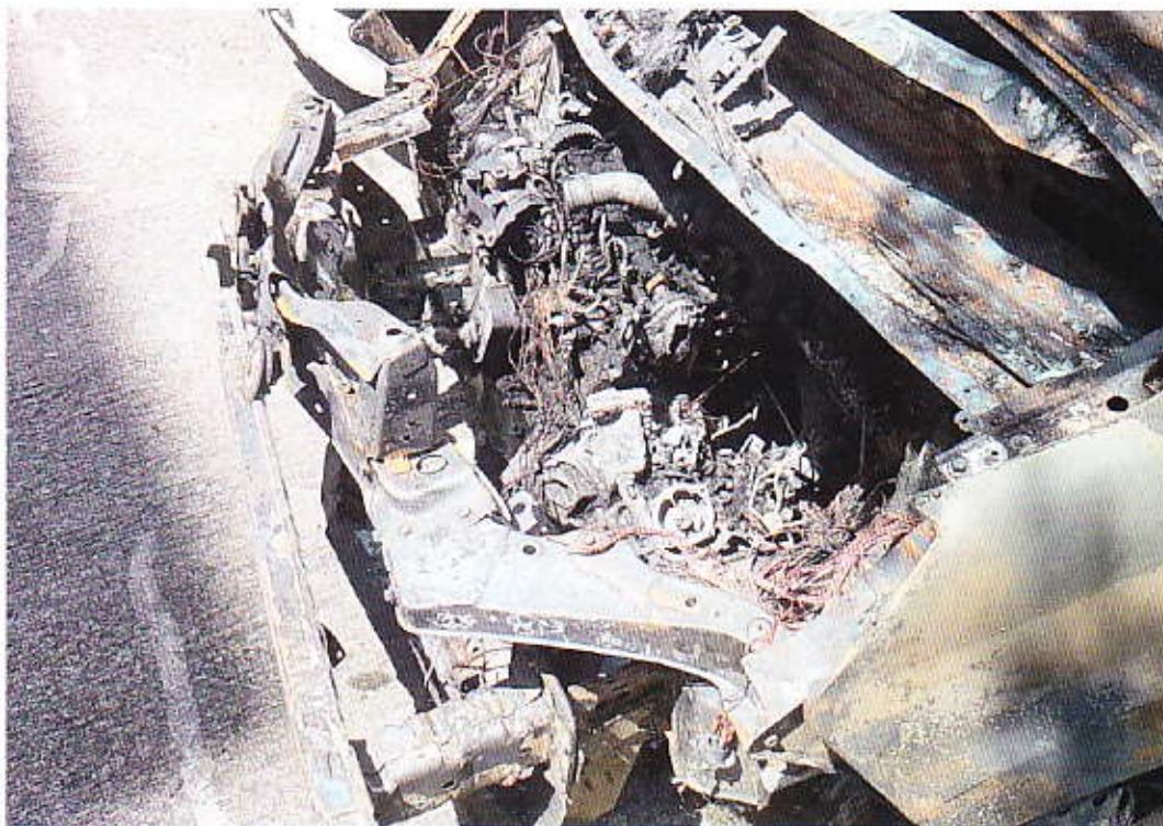
Photo 18 shows a close-up view of the burnt engine compartment after being towed.
