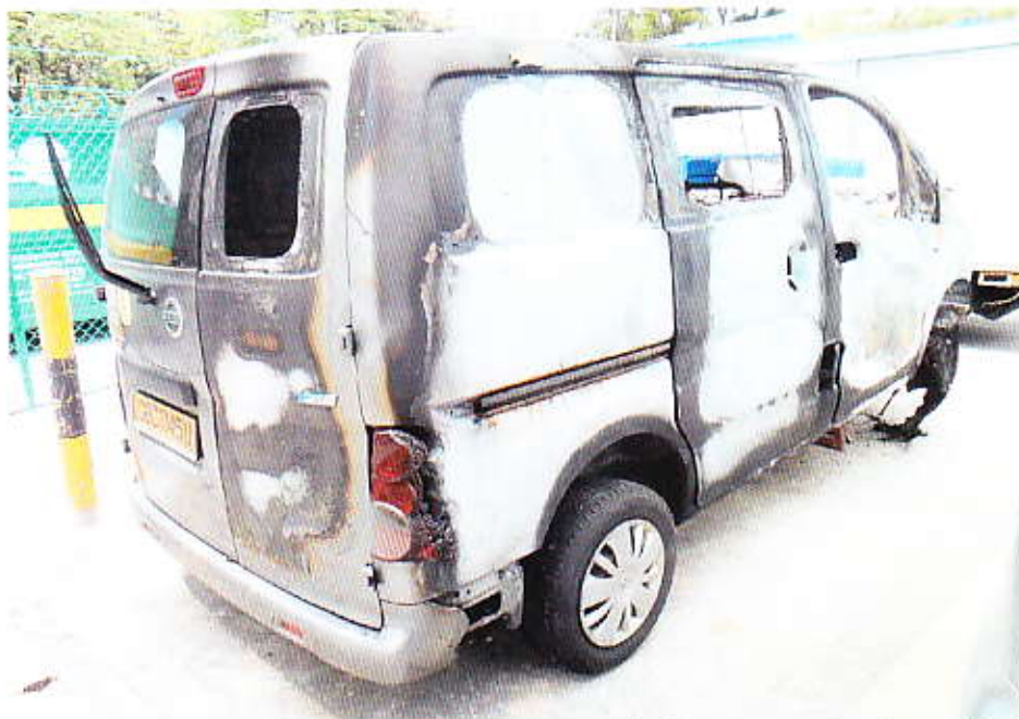
Photo 7 shows the whitish burn marks are a result of exposure to prolonged heat intensity. Rust would normally start to develop around these areas soon after a fire as prolonged exposure to high heat intensity usually causes steel/metal material body parts to be exposed to natural environmental condition. The rust that had developed on the Motor Vehicle is an indication that it had sustained exposure to prolonged high heat intensity.
