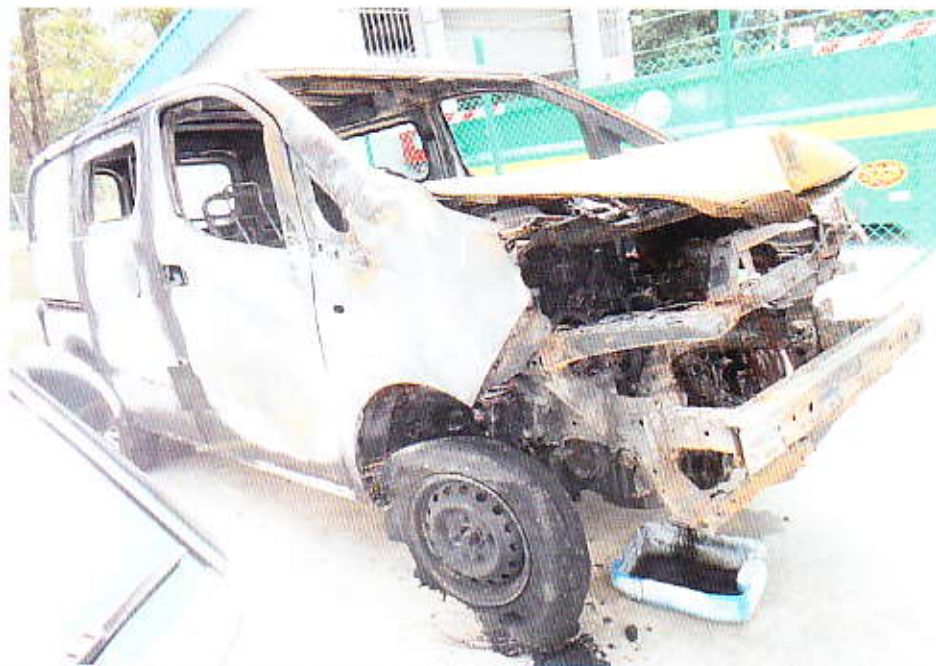
Photo 3 shows the right side of the Insured Vehicle at the time of our inspection. The Insured Vehicle was noted to have sustained fire damages that severely effected on most parts of the Insured Vehicle.
