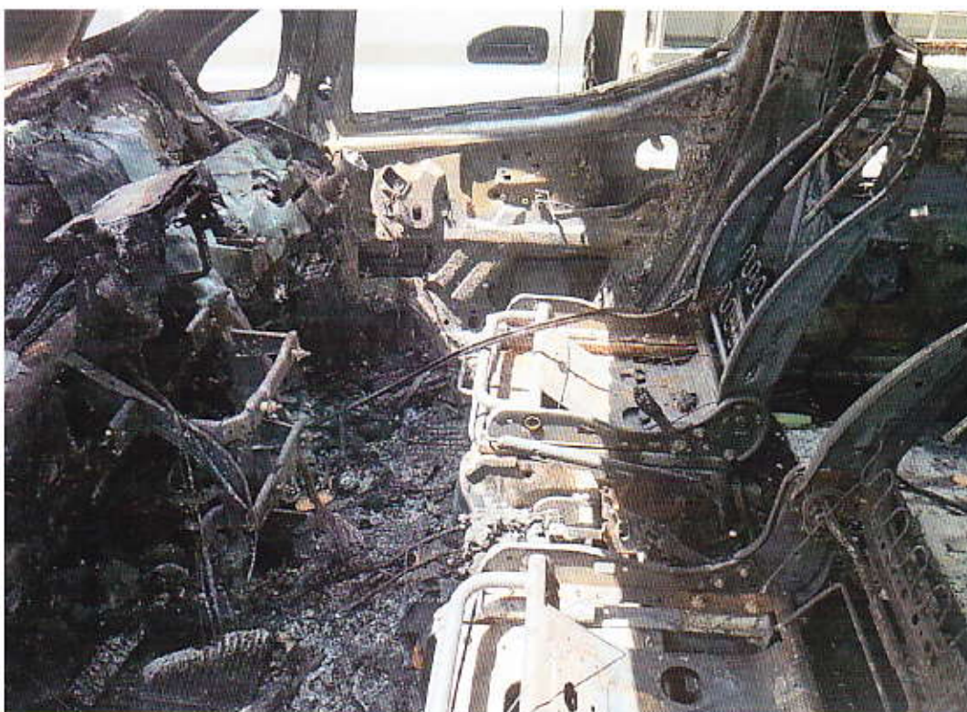
Photo 19 shows a close up view of the burnt interior compartment after being towed.
