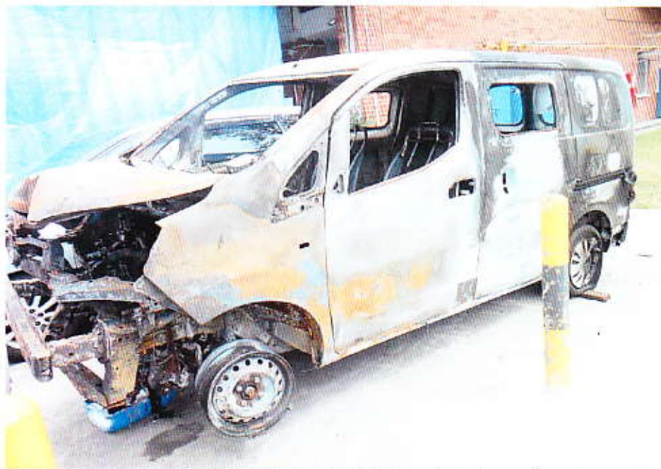
Photo 4 shows the left side of the Insured Vehicle at the time of our inspection. The Insured Vehicle was noted to have sustained fire damages that severely effected on most parts of the Insured Vehicle.
