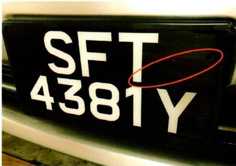
Photo 10 shows the condition of the Toyota's front number plate as depicted in the photographs that were taken by the witness post- accident. The same crack towards the left side of the front number plate was observed (circled).
