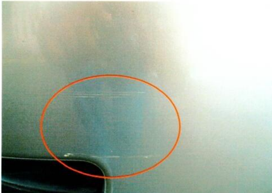
Photo 4 shows a close up view of the graze marks found on the left portion of the Toyota's front bumper (circled).
