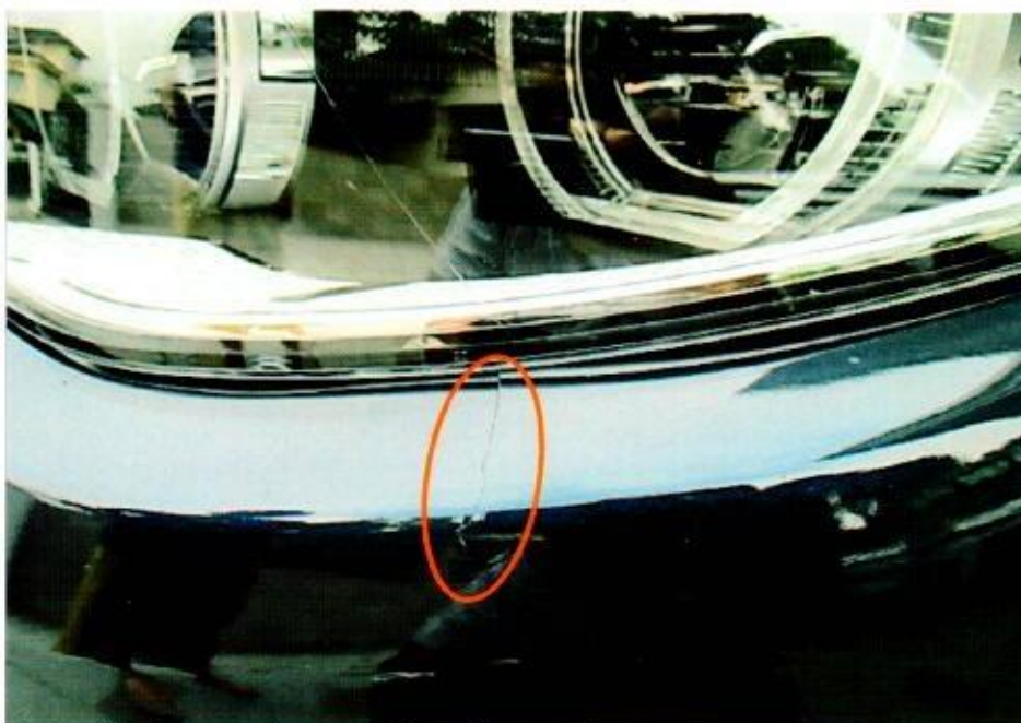
Photo 17 shows a close up view of the relatively minor paint crack on the left portion of the front bumper, below the left headlight (circled).
