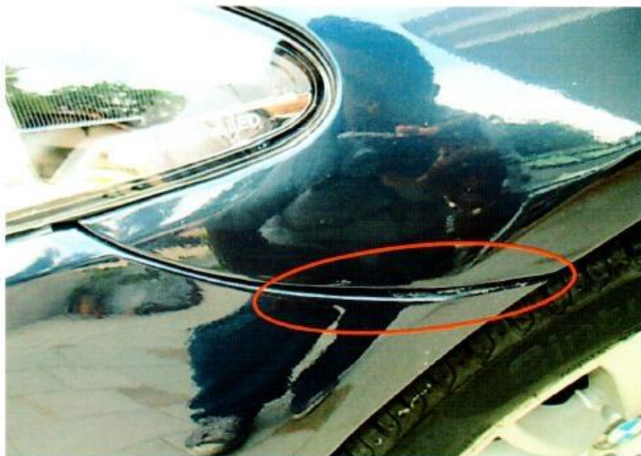
Photo 18 shows a misalignment at the left corner edge of the BMW's front bumper (circled). The paint cracks on the left portion of the front bumper were a result of load/force pressing onto the front bumper, inwards. This load/force was significant, causing the misalignment.
