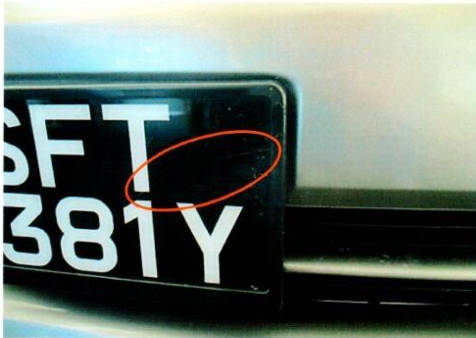
Photo 2 shows the cracked front number plate of the Toyota (circled). This was towards the left side of the front number plate.
