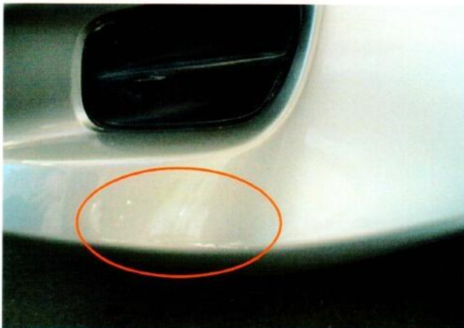
Photo 5 shows a close up view of the graze marks found on the lower left portion of the Toyota's front bumper (circled).
