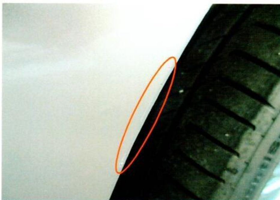
Photo 7 shows a close up view of the graze marks found on the Toyota's left front tyre fender (circled).
