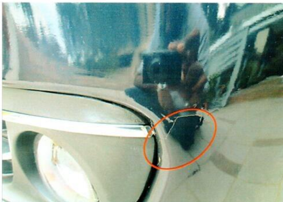
Photo 16 shows a close up view of the relatively minor paint crack on the left portion of the front bumper, adjacent to the left fog lamp cover (circled).
