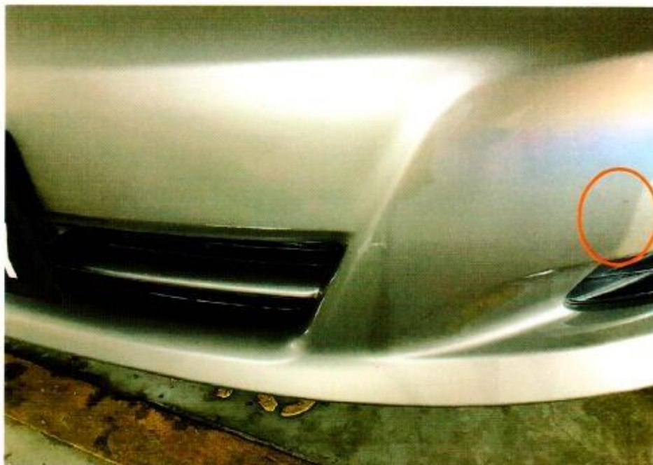
Photo 11 shows the condition of the Toyota's front bumper as depicted in the photographs that were taken by the witness post- accident. The same graze marks on the lower left portion of the front bumper were observed (circled).
