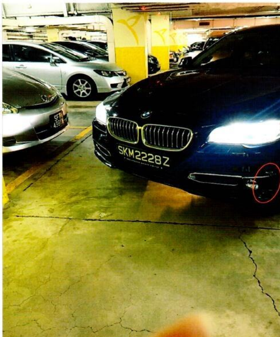
Photo 19 shows the Involved Motor Cars at the accident scene after the BMW had reversed out of the parking lot. Upon closer examination, we noticed the same graze marks on the lower left portion of the BMW's front bumper that we observed during our physical inspection (circled)
