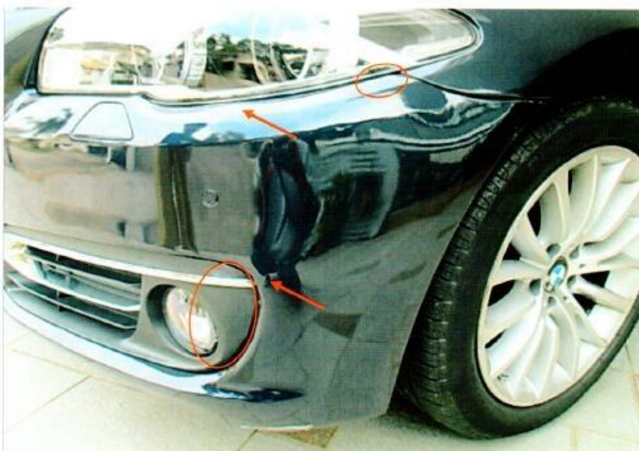
Photo 13 shows upon closer inspection, we note that there were graze marks on the left portion of the front bumper as well as on the left fog lamp cover (circled). We also found relatively minor paint cracks on the left portion of the front bumper, adjacent to the left fog lamp cover as well as below the left headlight (arrowed).
