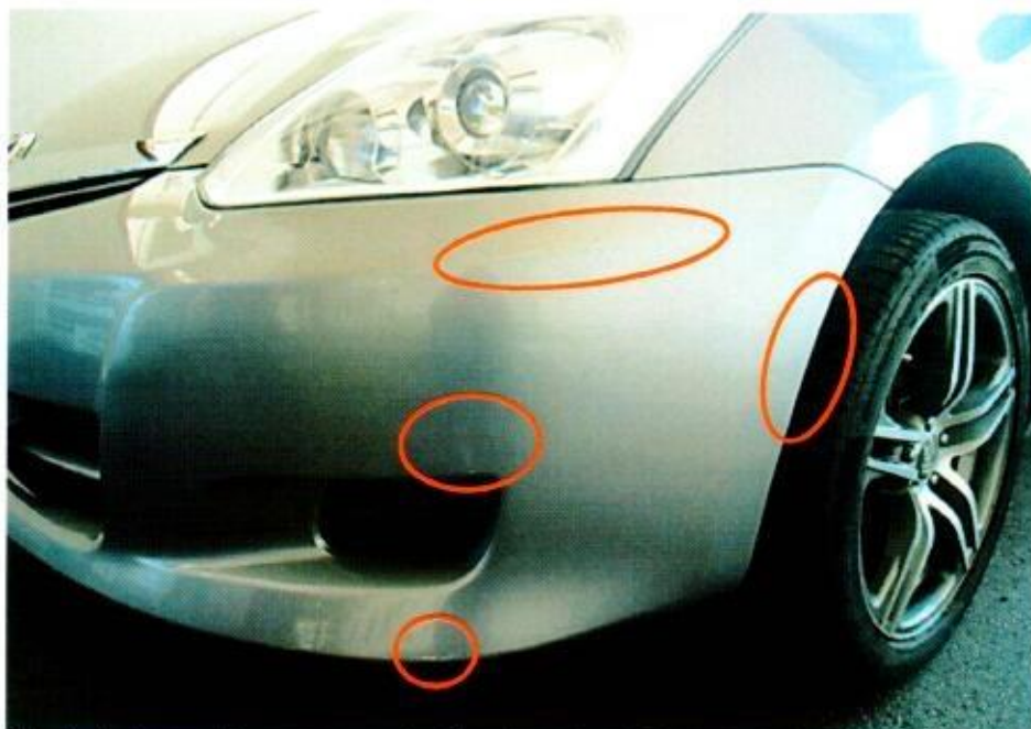
Photo 3 shows the graze marks found on the left portion of the Toyota's front bumper (circled).
