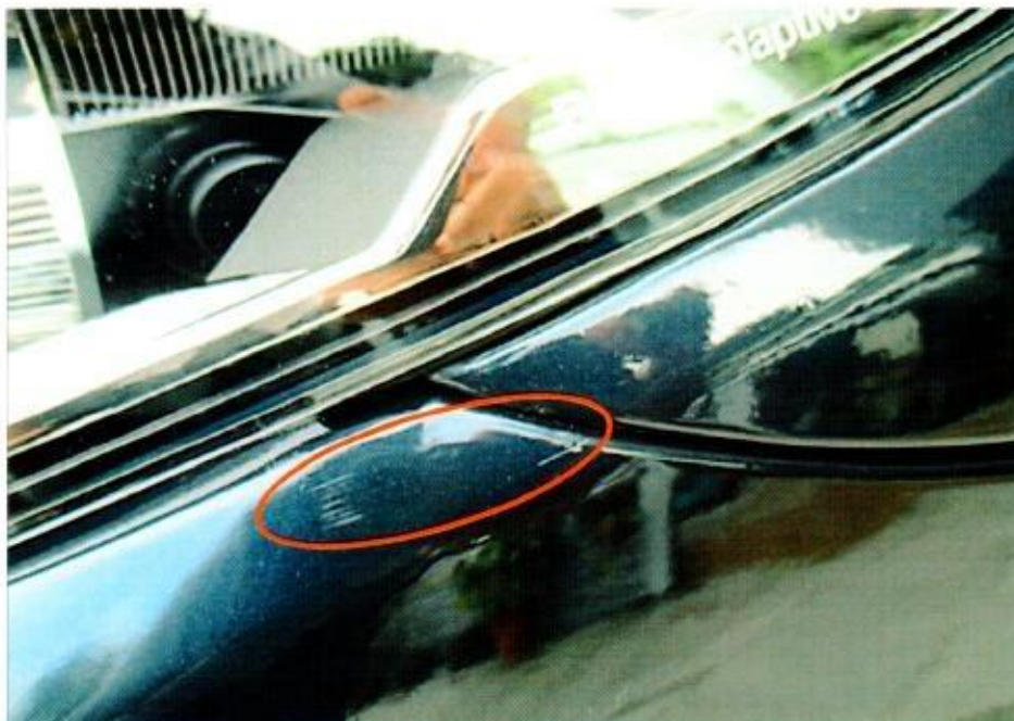
Photo 14 shows a close up view of the graze marks found on the left portion of the front bumper (circled).
