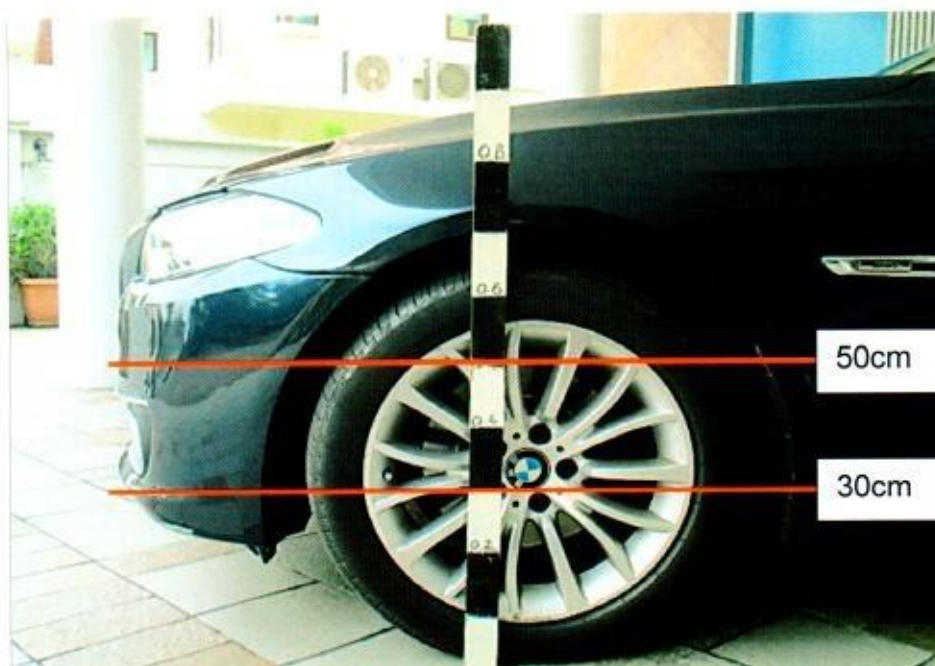
Photo 21 shows the height measurement being conducted on the left front portion of the BMW. The paint graze marks on the left portion of the front bumper and paint crack adjacent to the left fog lamp cover of the BMW are within the 30cm to 50cm range.
