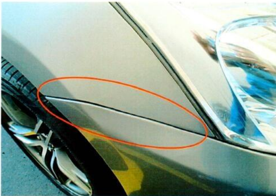
Photo 9 shows no obvious misalignment at the corner edges of the Toyota's front bumper, adjacent to its front right fender (circled). This would indicate that the impact onto the frontal portion of the Toyota was relatively light.
