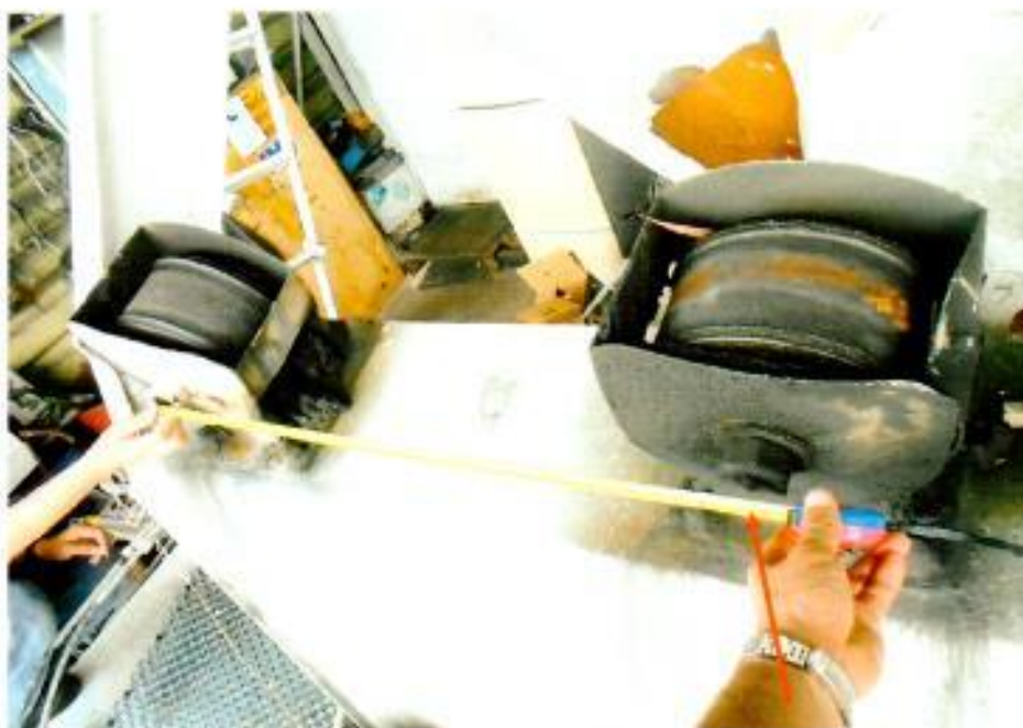
Photo 19 shows a measurement on the roller spacing for GETHI manufacturer. It was measured as 32 inches from centre to centre of the 02 rollers.
