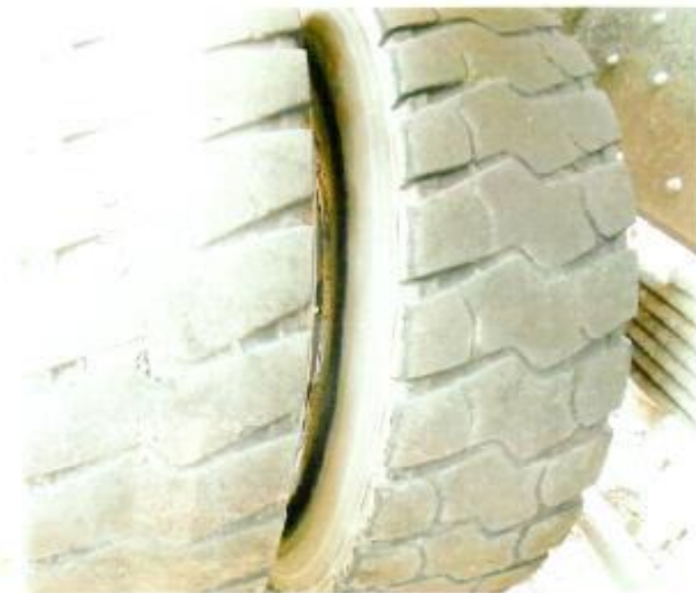
Photo 22 shows the condition of the rear right tyre of the Insured Vehicle, which was observed to be in serviceable condition with remaining tread depth of approximately 2mm.
