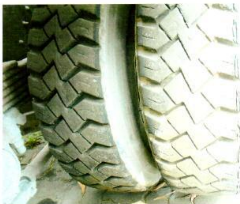
Photo 18 shows the condition of the rear left tyre of the Insured Vehicle, which was observed to be in serviceable condition with remaining tread depth of approximately 10mm.
