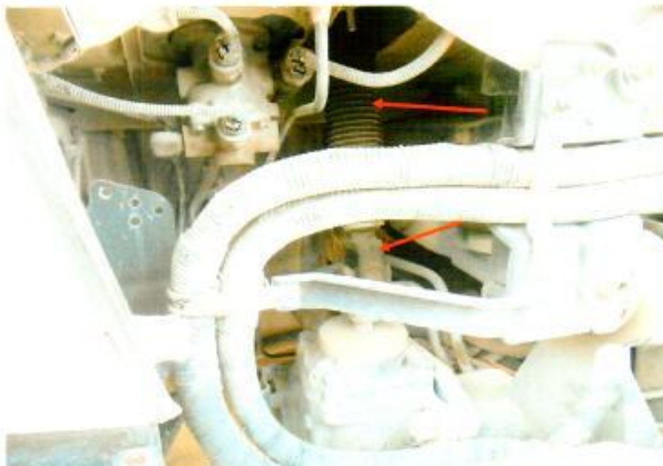
Photo 32 shows the steering wheel rod of the Insured Vehicle. It was observed to be intact and undamaged not affected by the accident's impact.
