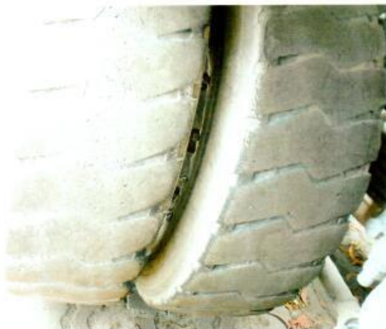
Photo 17 shows the condition of the left tyre (3 rd Row) of the Insured Vehicle, which was observed to be in serviceable condition with remaining tread depth of approximately 2mm.
