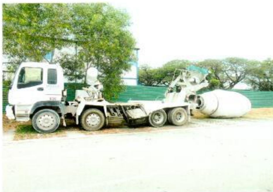
Photo 6 shows the full general view on the left side of the Insured Vehicle at the time of our inspection. The Insured Vehicle was noted to have sustained extensive damages that severely effected on most parts of the left side of the Insured Vehicle.
