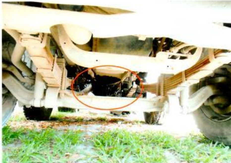
Photo 28 shows a general view on the undercarriage of the Insured Vehicle. It was observed to have fluid leakage at around the transmission area.
