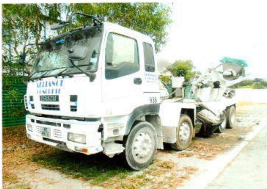
Photo 5 shows the front left side of the Insured Vehicle at the time of our inspection. The Insured Vehicle was noted to have sustained extensive damages that severely effected on most parts of the left side of the Insured Vehicle.
