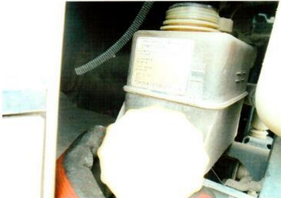
Photo 26 shows the power steering fluid reservoir of the Insured Vehicle. It was found to be sufficient level without contamination for operational purposes.
