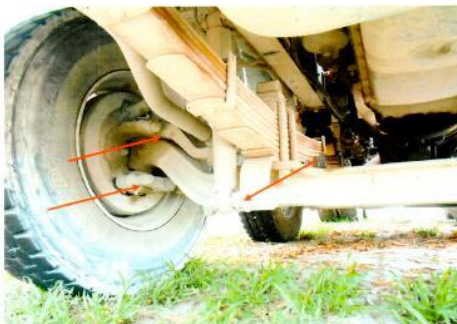
Photo 30 shows the undercarriage components at the front right wheel of the Insured Vehicle. The various undercarriage components were all observed to be intact and without any visible damage. This had included the steering rack and steering linkages (arrowed) of the Insured Vehicle.
