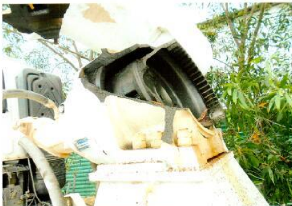
Photo 9 shows the mixer motor gear that was affected due to the accident's impact at time of our inspection.
