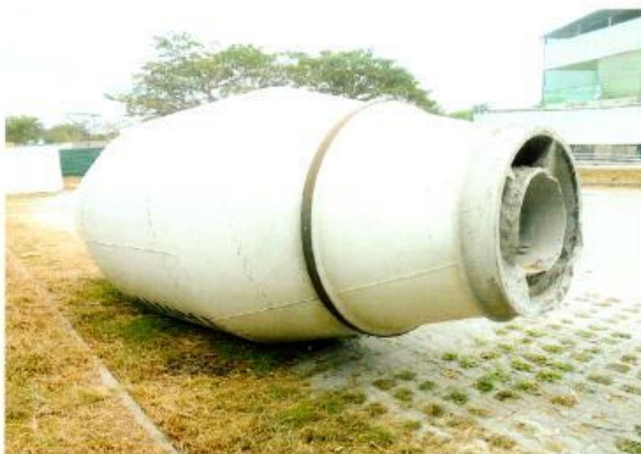
Photo 12 shows the rear view of cement mixer drum that was dislodged from the holding bracket at time of our inspection.
