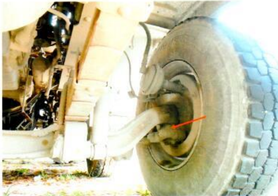
Photo 31 shows the undercarriage components at the front left wheel of the Insured Vehicle. The various undercarriage components of the Insured Vehicle were all observed to be intact and without any visible damage. This had included the steering rack (arrowed) of the Insured Vehicle, which was observed to be securely attached to the front left wheel.
