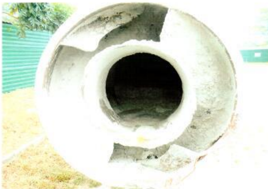
Photo 14 shows the internal view of cement mixer drum that was dislodged from the holding bracket at time of our inspection. Left over hardened cement were observed to be inside the drum.
