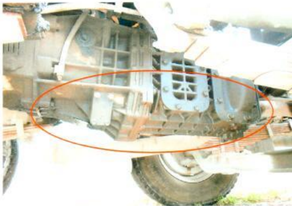
Photo 29 shows fluid leakage at around the transmission area. Further investigation found that the fluid stain was a pre-existed prior the accident & not a fresh fluid. This was due to some dirt observed associated with the fluid stain.
