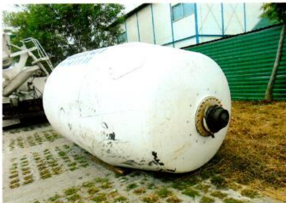
Photo 13 shows the front view of cement mixer drum that was dislodged from the holding bracket at time of our inspection.
