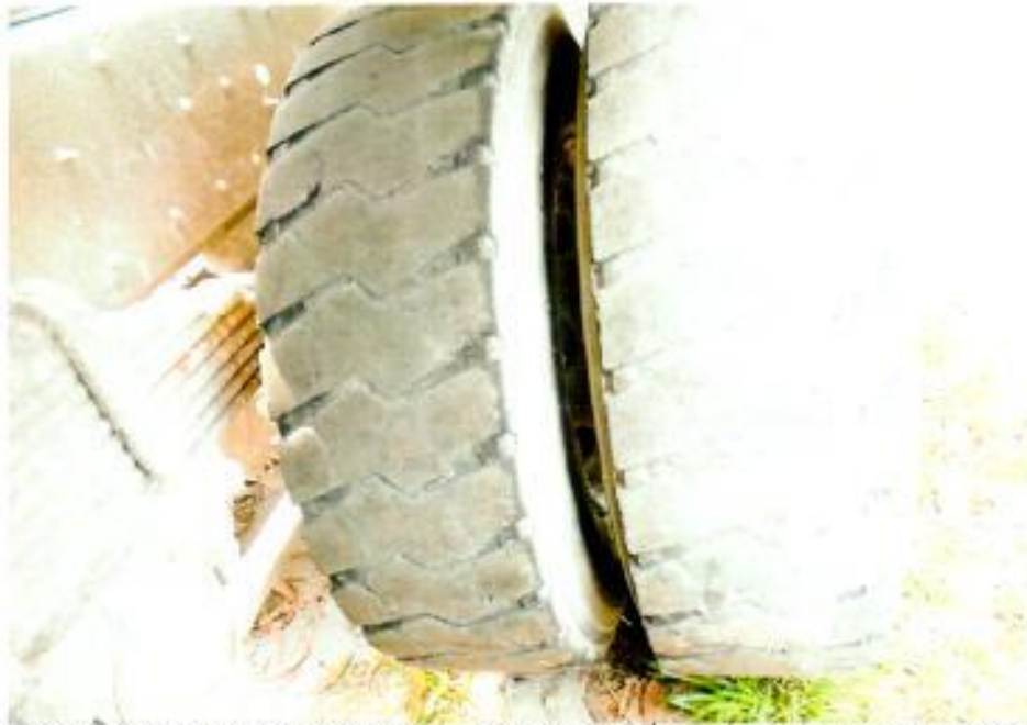
Photo 21 shows the condition of the right tyre (3 rd Row) of the Insured Vehicle, which was observed to be in serviceable condition with remaining tread depth of approximately 3mm.
