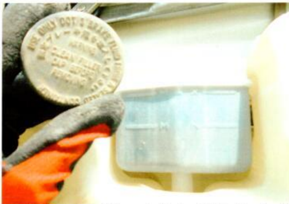
Photo 27 shows the brake fluid reservoir of the Insured Vehicle. It was found to be sufficient level without contamination for operational purposes.
