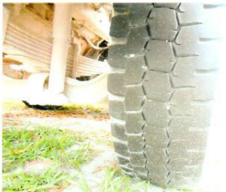
Photo 15 shows the condition of the front left tyre of the Insured Vehicle, which was observed to be in serviceable condition with remaining tread depth of approximately 5mm.
