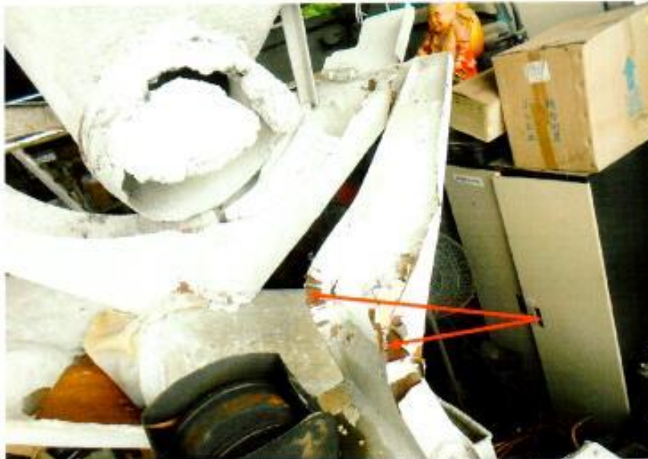
Photo 44 shows the material failure that was believed to cause the drum to give way. It was observed to be in a corroded condition.
