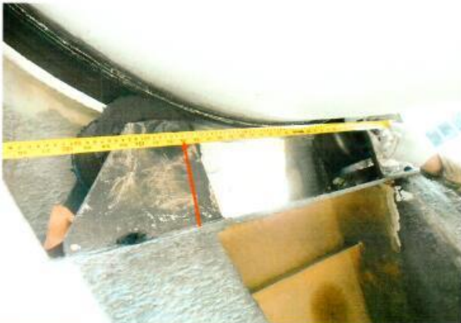
Photo 19 shows a measurement on the roller spacing for CESCO manufacturer. It was measured as 29 inches from centre to centre of the 02 rollers.
