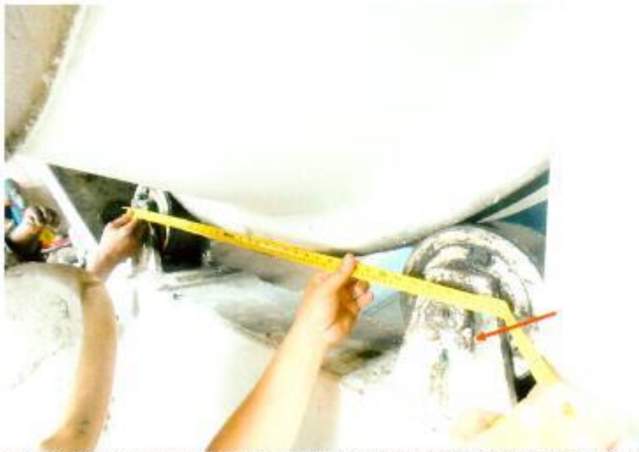
Photo 19 shows a measurement on the roller spacing for ZICOM manufacturer. It was measured as 36 inches from centre to centre of the 02 rollers.
