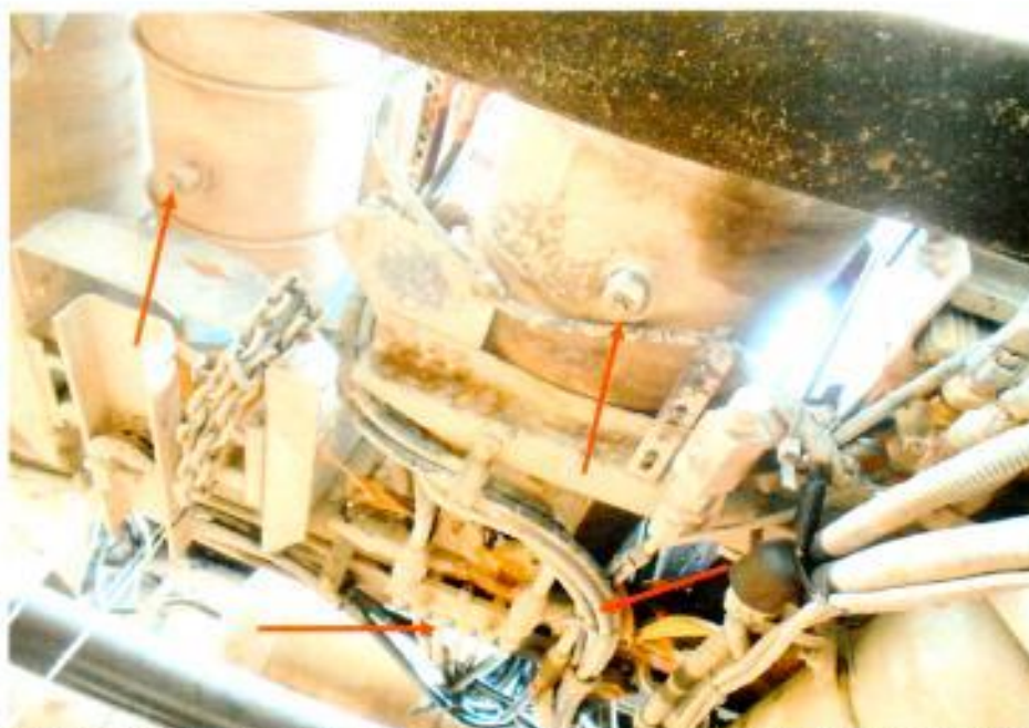
Photo 33 shows the air tanks, valves, pipes and hoses, which are some of the components for the air-assisted braking system of the Insured Vehicle. These components were mainly located around the right centre body of the Insured Vehicle, and were unaffected by the accident.
