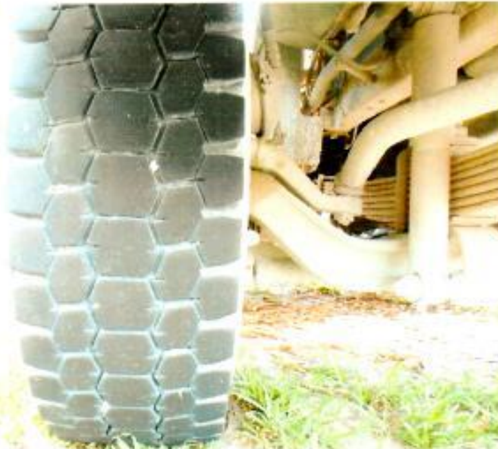
Photo 19 shows the condition of the front right tyre of the Insured Vehicle, which was observed to be in serviceable condition with remaining tread depth of approximately 10mm.
