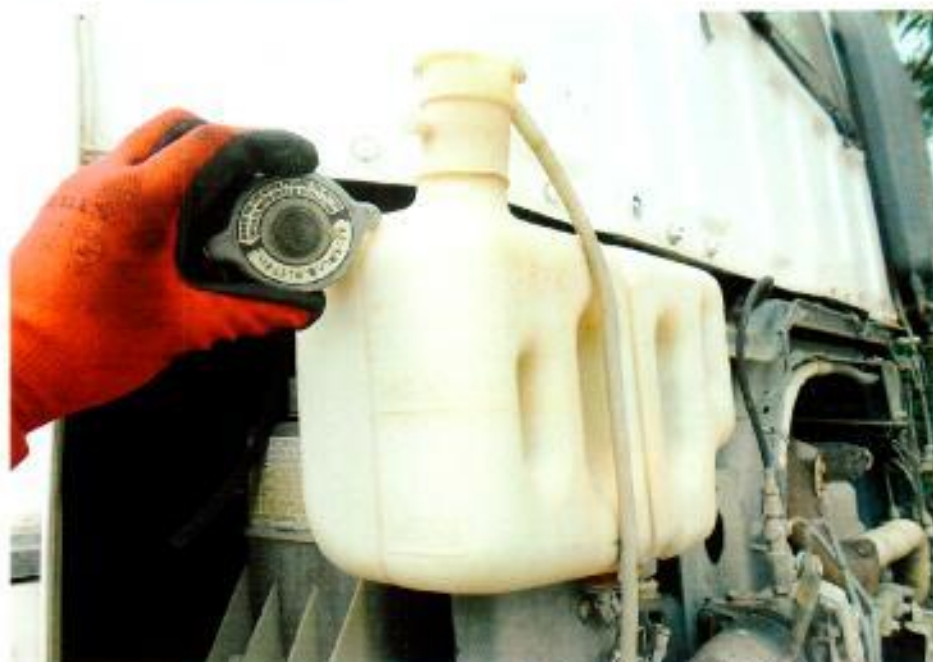
Photo 25 shows the engine coolant reservoir of the Insured Vehicle. It was found to be sufficient level without contamination.
