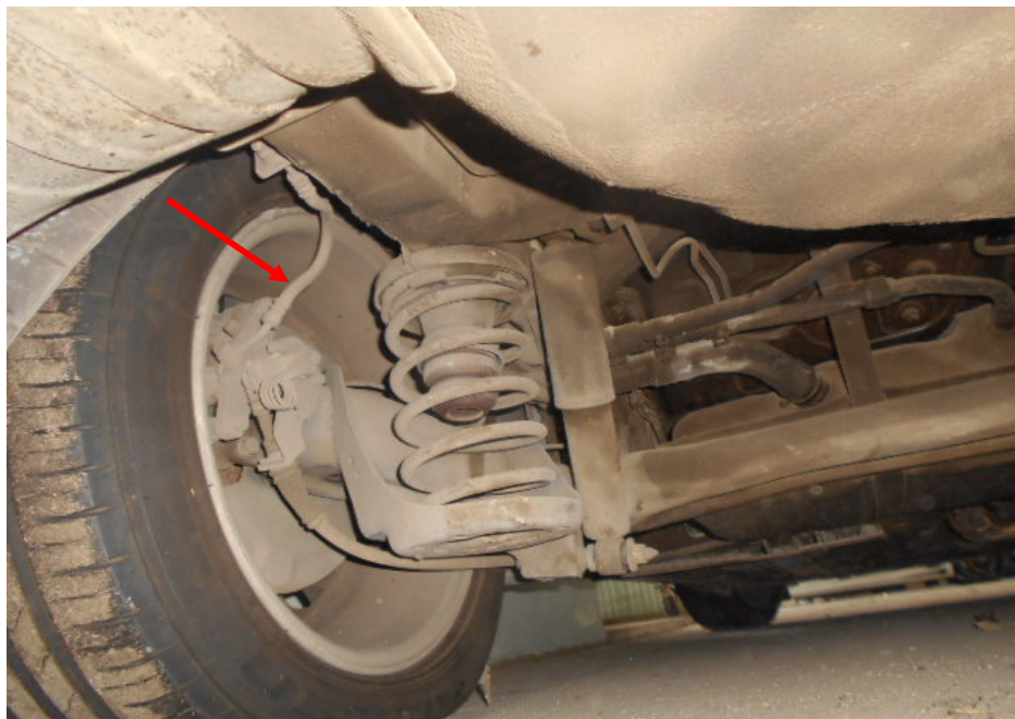
Photo 15 shows the brake hose/pipe (arrowed) at the rear left wheel of the Police Car. I did not observe any leakage of brake fluid at the time of my inspection of the Police Car. Static tests of the Police Car's braking system had indicated that there was no internal leakage of pressure/vacuum.
