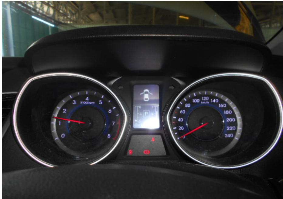
Photo 21 shows no warning lights illuminated on the instrument panel of the Police Car after the engine was cranked. This would suggest that there was no abnormality to the various electronic operating systems of the Police Car, like the ABS, EPS, TC and SRS etc.
