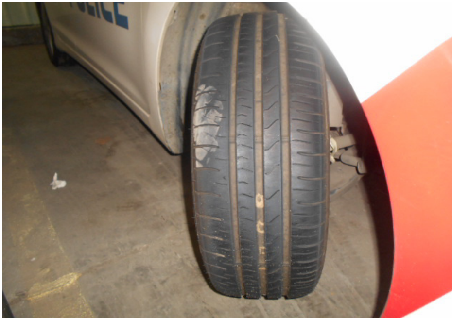
Photo 7 shows the condition of the front right tyre of the Police Car, which was observed to be in serviceable condition with remaining tread depth of approximately 6mm. The tyre was also observed to be sufficiently inflated for vehicular operation with no tear, cut or burst mark(s).
