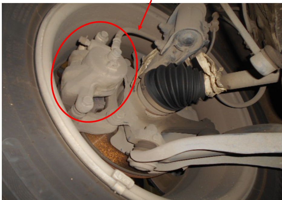
Photo 16 shows the brake hose/pipe (arrowed) at the front right wheel of the Police Car. No leakage of brake fluid was observed. Visual examination of the various components of the braking system like the brake caliper (circled), brake booster, brake pedal etc had revealed all to be intact and without visible damage. The braking system of the Police Car was likely to be in serviceable condition.
