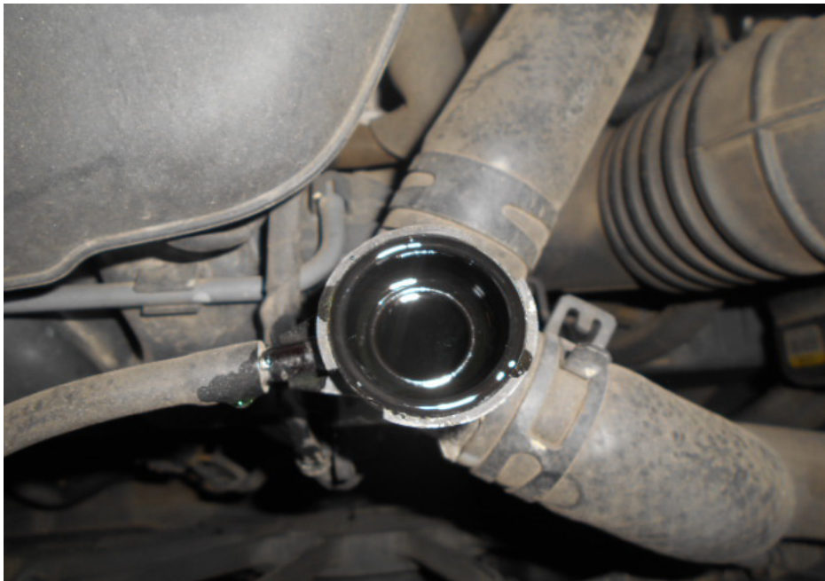
Photo 12 shows checks being carried out to the engine coolant of the Police Car at the time of my inspection. The engine coolant was observed to be of sufficient level and without any visible contamination.
