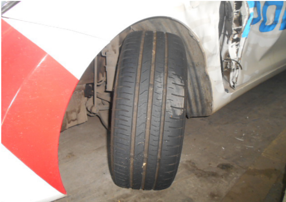
Photo 6 shows the condition of the front left tyre of the Police Car, which was observed to be in serviceable condition with remaining tread depth of approximately 6mm. The tyre was sufficiently inflated for vehicular operation with no tear, cut or burst mark(s) on the outer and the inner sidewalls as well as across the tread. The 4 tyres of the Police Car were wrapped around standard alloy wheel rims that were without any significant damage apart for some relatively minor kerb grazing type of damage on the outer side of the wheel rims.
