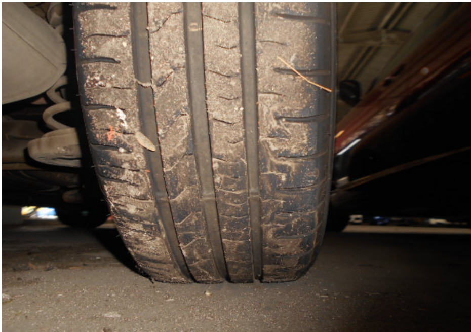
Photo 9 shows the condition of the rear right tyre of the Police Car, which was observed to be in serviceable condition with remaining tread depth of approximately 6mm. There was also no tear, cut or burst mark(s) on the outer and the inner sidewalls as well as across the tread of the Police Car's 4 tyres.
