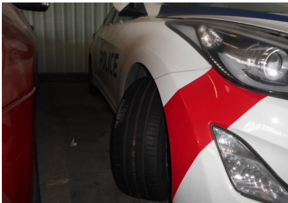
Photo 17 shows the front left wheel of the Police Car turned to its full right. During my static steering system test, I did not experience any abnormal free play and/or resistance when I had turned the steering wheel towards the left and right. This would suggest that the steering system of the Police Car was likely to be in serviceable condition.
