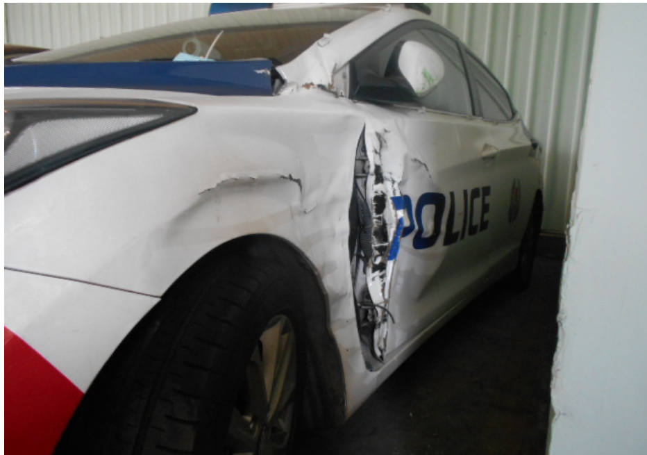
Photo 3 shows a closer view of the damaged area of the Police Car at the time of my inspection. Its left front fender, left front door, left wing mirror and front bonnet were damaged as a result of the accident.
