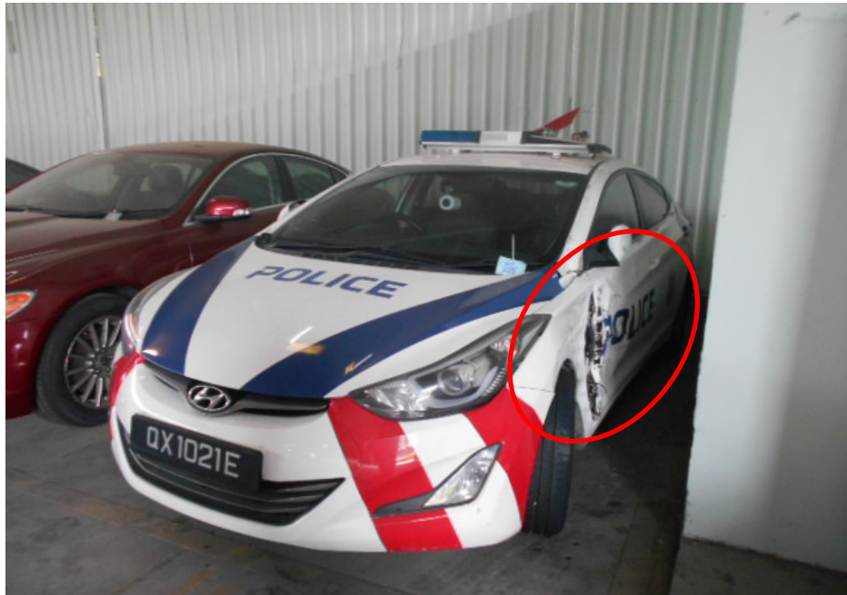
Photo 2 shows a general view of the front left body of the Police Car at the time of my inspection. The Police Car was observed to have sustained damage at its left front portion and left centre portion (circled). Its left front fender, left front door and front bonnet were damaged as a result of the accident. Its front left undercarriage was also observed to have been affected. The mileage of the Police Car at the time of my inspection was recorded to be 142,663km.
