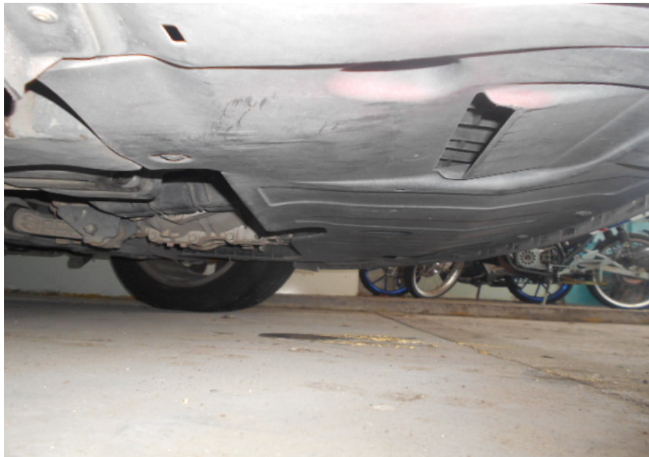
Photo 14 shows the front underside of the Police Car. I did not find any sign(s) or indication(s) of fluid leak and/or fluid stain(s) on the underside of the Police Car.
