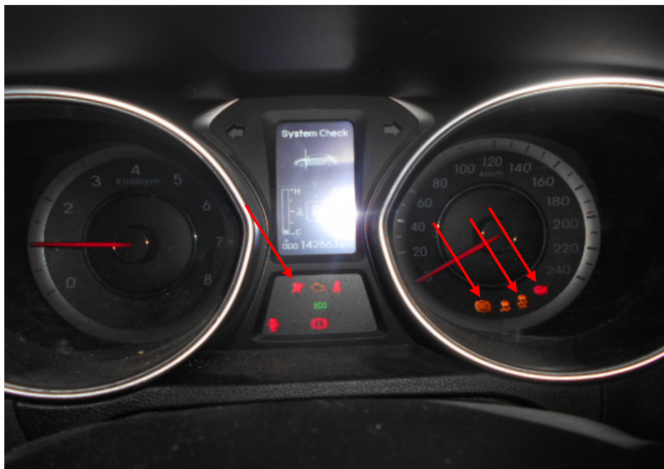
Photo 20 shows the warning light for Anti-Lock Brake System (ABS), Electric Power Steering System (EPS), Traction Control (TC) and Supplemental Restraint System (SRS) appearing on the instrument panel of the Police Car during the self-test of its various electronic operating systems when its engine was cranked.
