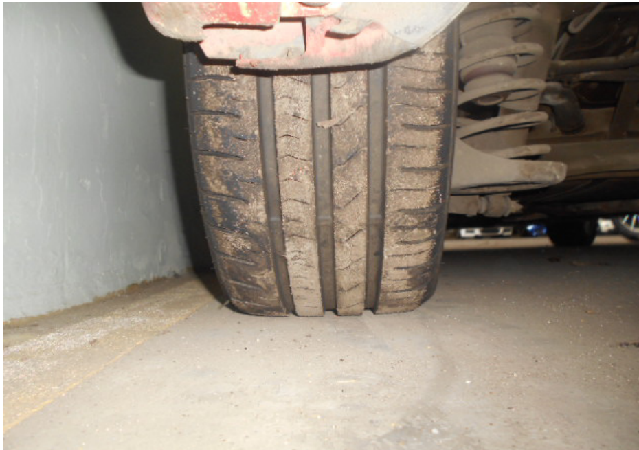
Photo 8 shows the condition of the rear left tyre of the Police Car, which was observed to be in serviceable condition with remaining tread depth of approximately 6mm. The tyre, which was wrapped around alloy wheel rim, was also observed to be sufficiently inflated for vehicular operation. The 4 tyres of the Police Car were wrapped around standard alloy wheel rims that were without any significant damage apart for some relatively minor kerb grazing type of damage on the outer side of the wheel rims
