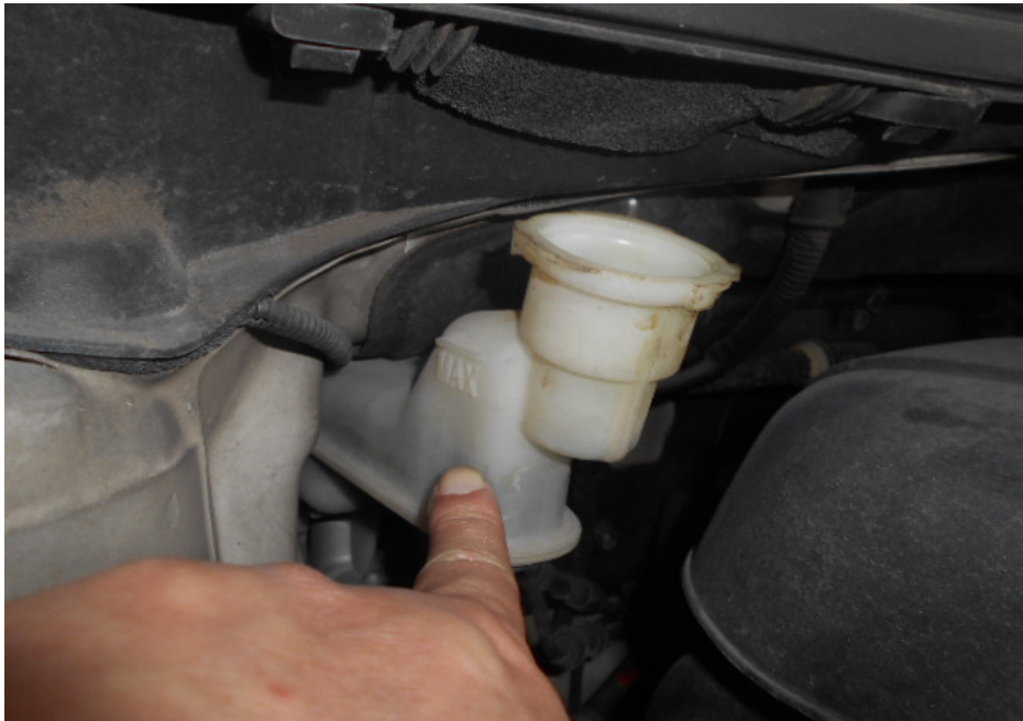
Photo 11 shows the brake fluid reservoir of the Police Car at the time of my inspection. The brake fluid was observed to be of sufficient level (as indicated by my finger) and without any visible contamination.
