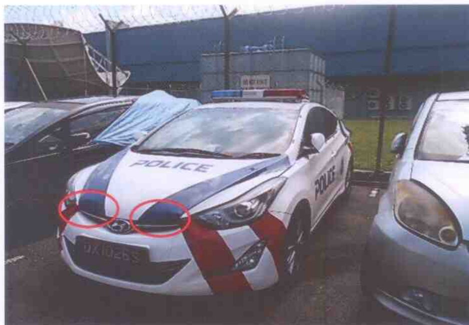
Photo 3 shows a general view of the front left body of the Police Car at the time of my inspection. The Police Car was observed to have sustained relatively minor damage at its frontal portion. Its front bumper, front bumper lower grille, front number plate and front bonnet (circled) were damaged as a result of the accident. The mileage of the Police Car at the time of my inspection was recorded to be 111,492km.
