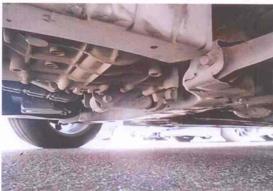
Photo 13 shows the underside of the Police Car, at the area where the engine housing and transmission housing are located. I did not find any sign(s) or indication(s) of fluid leak and/or fluid stain(s) on the underside of the Police Car.
