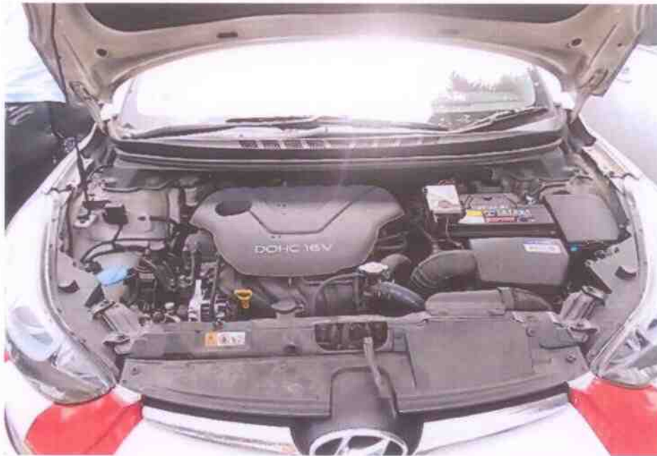
Photo 9 shows a general view of the Police Car's engine compartment. The various parts and components inside the engine compartment were unaffected by the accident. There was also no sign(s) or indication(s) of fluid leakage and/or fluid stain within the engine compartment.
