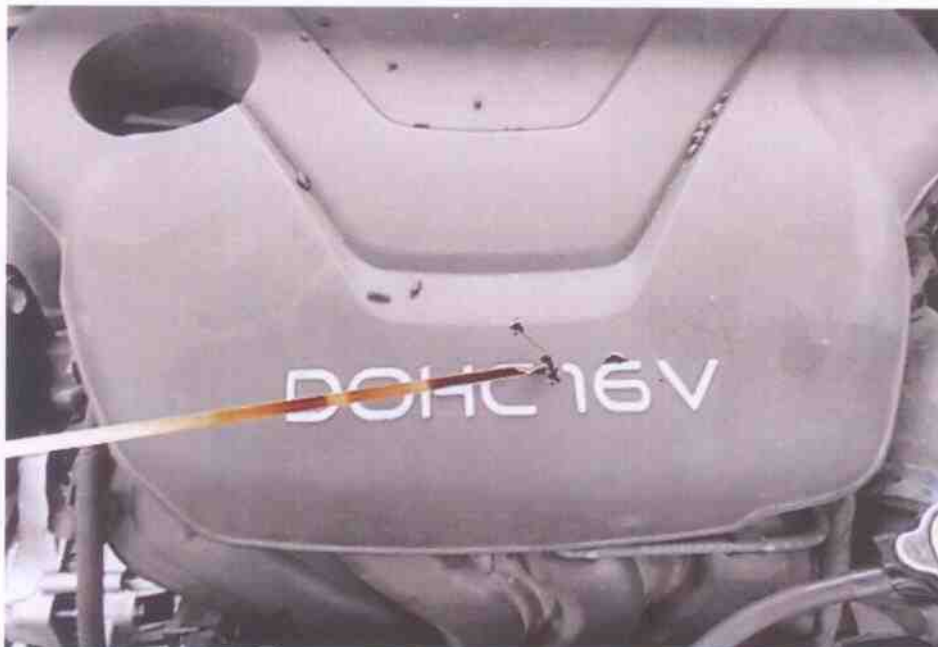
Photo 12 shows the engine oil dip stick of the Police Car at the time of my inspection. The engine oil was observed to be of sufficient level and without any visible contamination.
