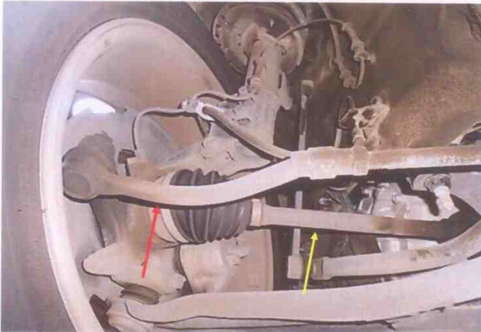
Photo 18 shows the various undercarriage components at the front left wheel of the Police Car, which had included the steering tie rod (red arrow) and front left drive shaft (yellow arrow). The various undercarriage components of the Police Car were all found to be intact without any visible damage.
