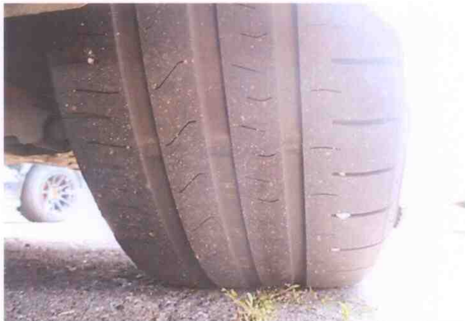
Photo 7 shows the condition of the rear left tyre of the Police Car, which was observed to be in serviceable condition with remaining tread depth of approximately 5mm. The tyre, which was wrapped around alloy wheel rim, was also observed to be sufficiently inflated for vehicular operation. The 4 tyres of the Police Car were wrapped around standard alloy wheel rims that were without any significant damage apart for some relatively minor kerb grazing type of damage on the outer side of the wheel rims.
