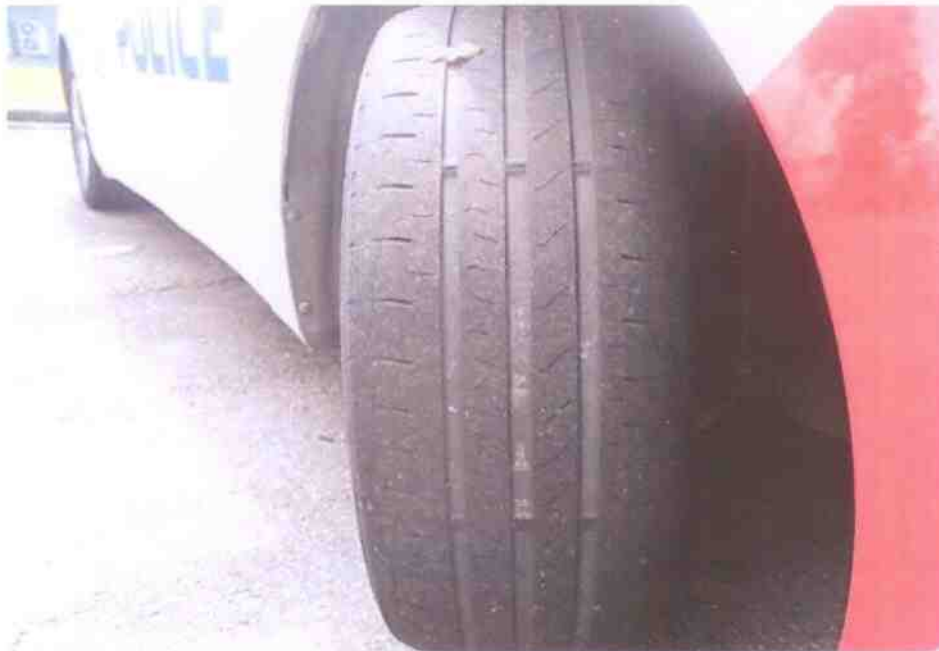
Photo 6 shows the condition of the front right tyre of the Police Car, which was observed to be in serviceable condition with remaining tread depth of approximately 3mm. The tyre was also observed to be sufficiently inflated for vehicular operation with no tear, cut or burst mark(s).
