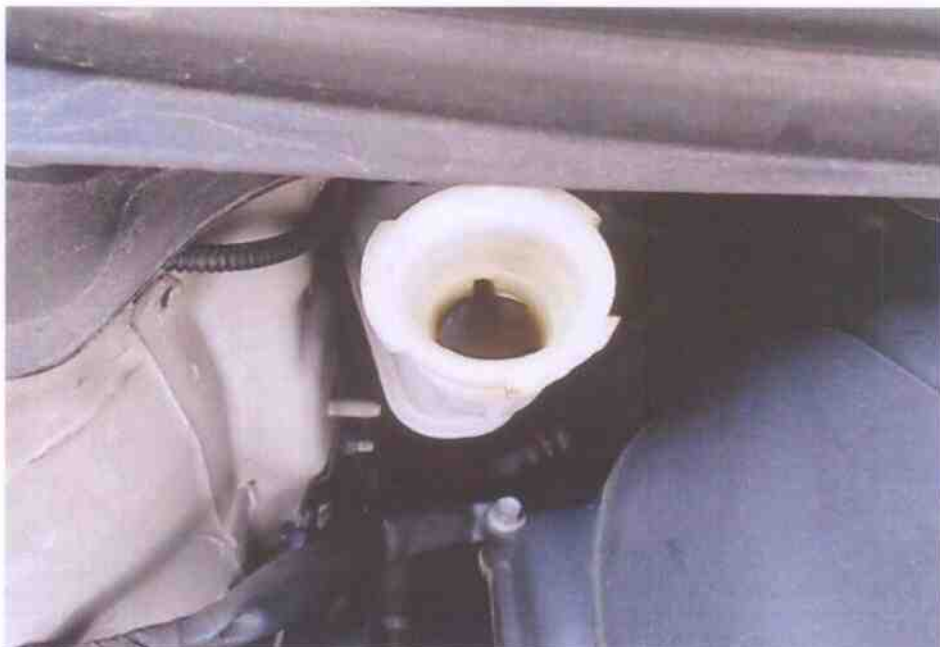
Photo 10 shows the brake fluid reservoir of the Police Car at the time of my inspection. The brake fluid was observed to be of sufficient level and without any visible contamination.
