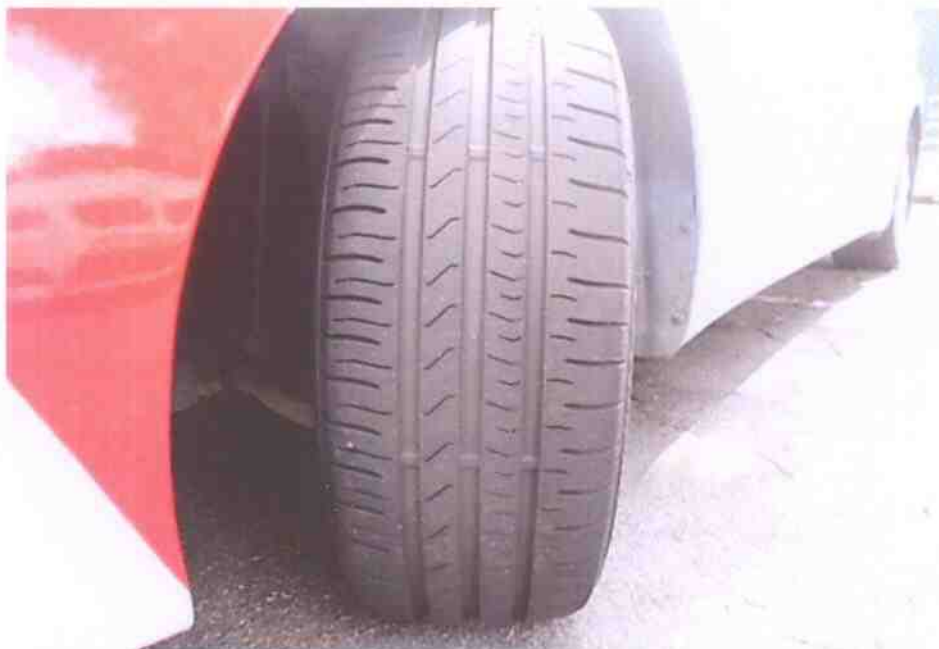
Photo 5 shows the condition of the front left tyre of the Police Car, which was observed to be in serviceable condition with remaining tread depth of approximately 5mm. The tyre was sufficiently inflated for vehicular operation with no tear, cut or burst mark(s) on the outer and the inner sidewalls as well as across the tread. The 4 tyres of the Police Car were wrapped around standard alloy wheel rims that were without any significant damage apart for some relatively minor kerb grazing type of damage on the outer side of the wheel rims.
