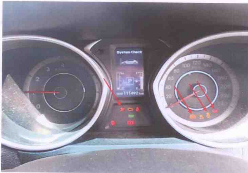
Photo 19 shows the warning light for Anti-Lock Brake System (ABS), Electric Power Steering System (EPS), Traction Control (TC) and Supplemental Restraint System (SRS) appearing on the instrument panel of the Police Car during the self-test of its various electronic operating systems when its engine was cranked.
