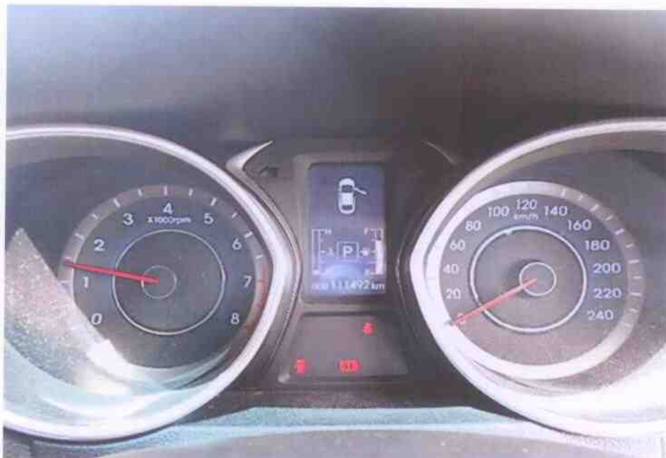
Photo 20 shows no warning lights illuminated on the instrument panel of the Police Car after the engine was cranked. This would suggest that there was no abnormality to the various electronic operating systems of the Police Car, like the ABS, EPS, TC and SRS etc.
