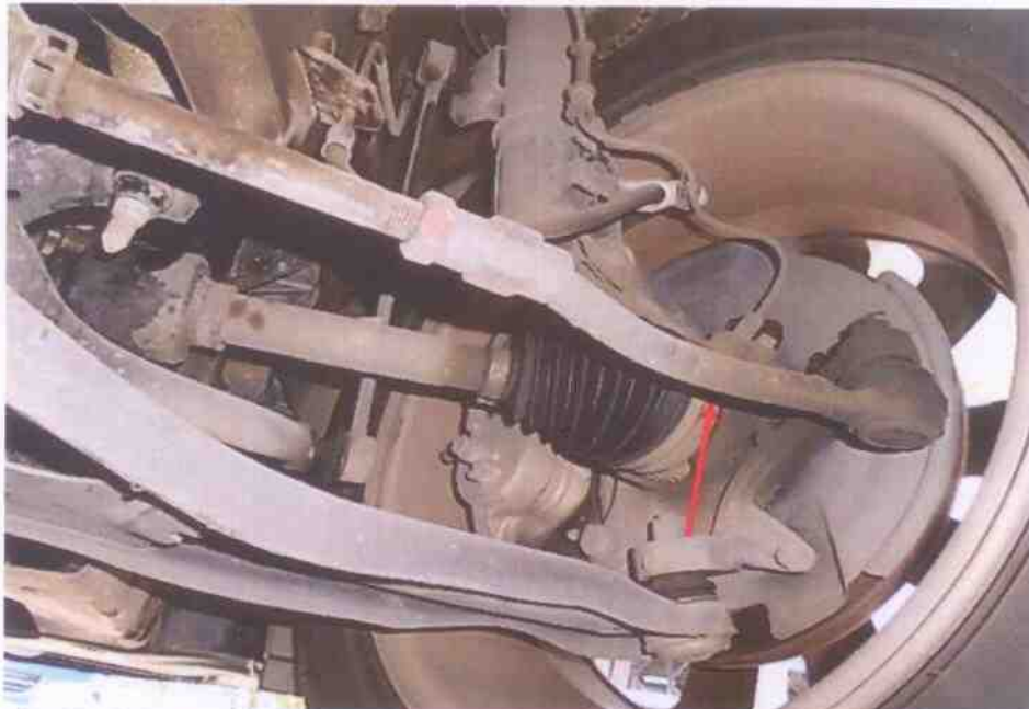
Photo 17 shows the various undercarriage components at the front right wheel of the Police Car, in particular the steering tie rod (arrowed). The various steering components were all found to be intact, suggesting that the steering system of the Police Car was likely to be in serviceable condition at the material time of accident. There was also no sign of fluid stain observed on the various undercarriage components at the front right wheel of the Police Car.
