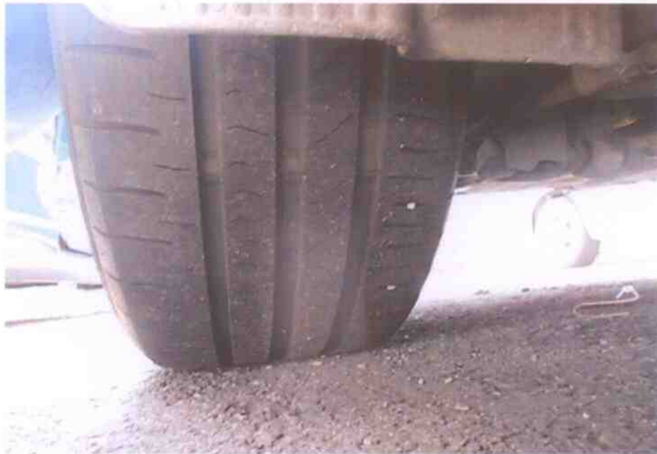
Photo 8 shows the condition of the rear right tyre of the Police Car, which was observed to be in serviceable condition with remaining tread depth of approximately 5mm. There was also no tear, cut or burst mark(s) on the outer and the inner sidewalls as well as across the tread of the Police Car's 4 tyres.
