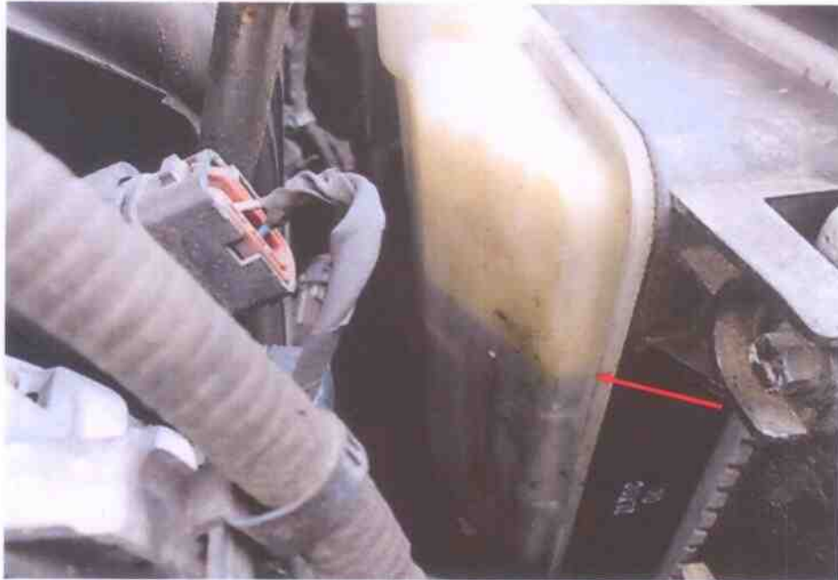
Photo 11 shows checks being carried out to the engine coolant of the Police Car at the time of my inspection. The engine coolant was observed to be of sufficient level (arrowed) and without any visible contamination.
