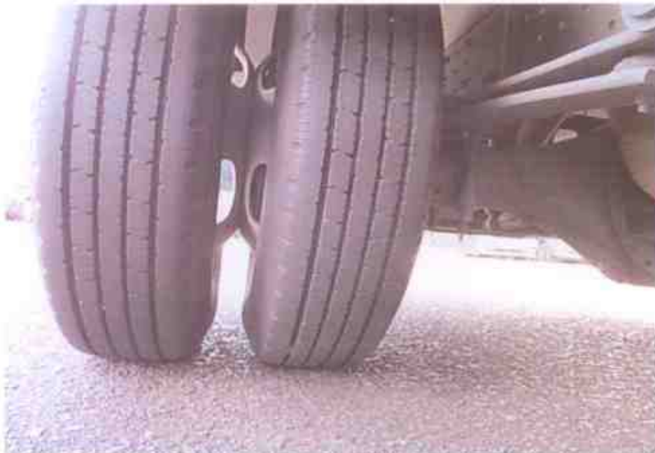
Photo 10 shows the condition of the rear right tyres of the Motor Lorry, which were observed to be in serviceable condition with remaining tread depth of approximately 6mm. There was also no tear, cut or burst mark(s) on the outer and the inner sidewalls as well as across the tread of the 6 tyres that were fitted on the Motor Lorry.
