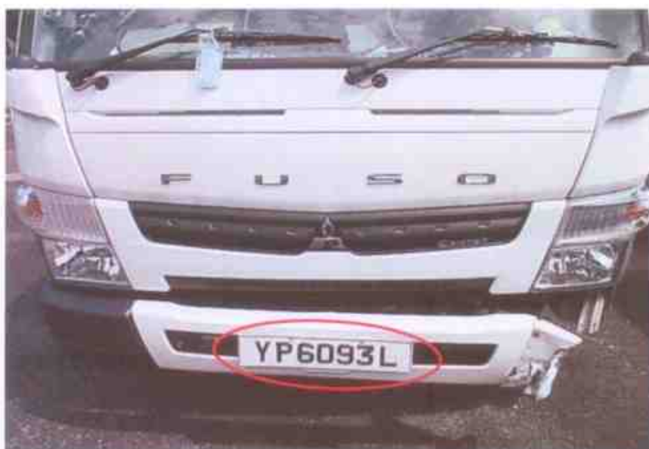
Photo 3 shows a closer view of the bent front number plate of the Motor Lorry at the time of our inspection (circled).
