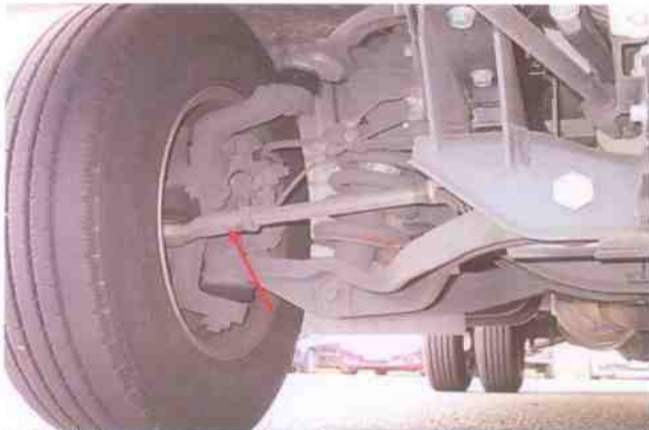
Photo 19 shows the various undercarriage components at the front right wheel of the Motor Lorry, in particular the steering tie rod end (arrowed). The various steering mechanical components were all found to be intact, suggesting that the steering system of the Motor Lorry was likely to be in serviceable condition at the material time of accident. There was also no sign of fluid stain(s) observed on the various undercarriage components.
