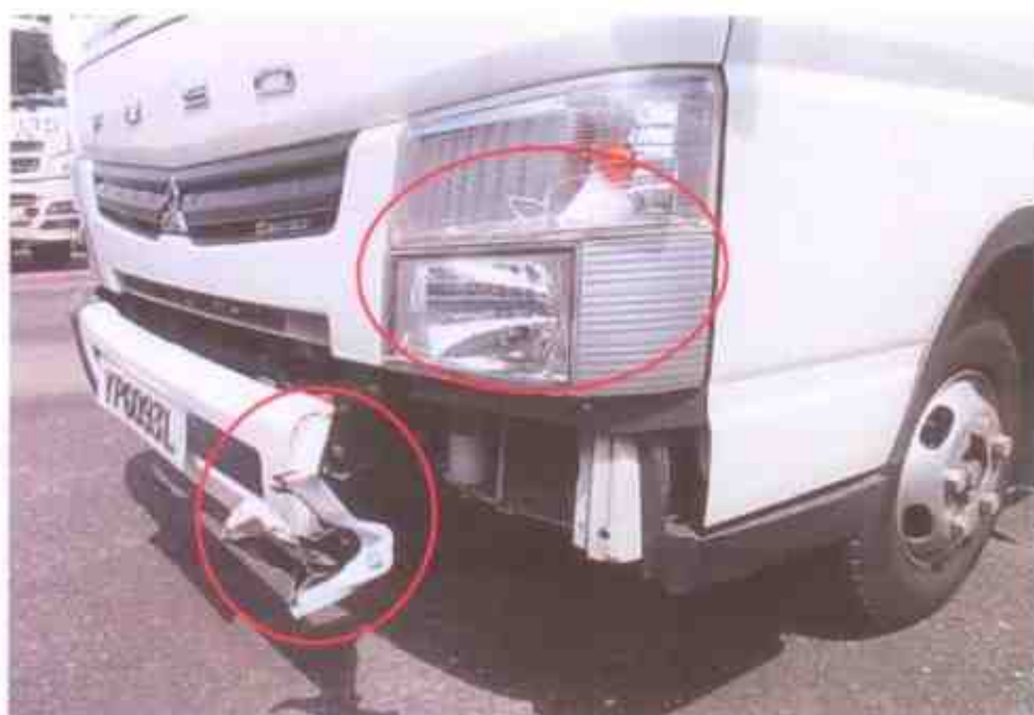
Photo 5 shows a closer view of the buckled front bumper and cracked left headlight of the Motor Lorry at the time of our inspection (circled).
