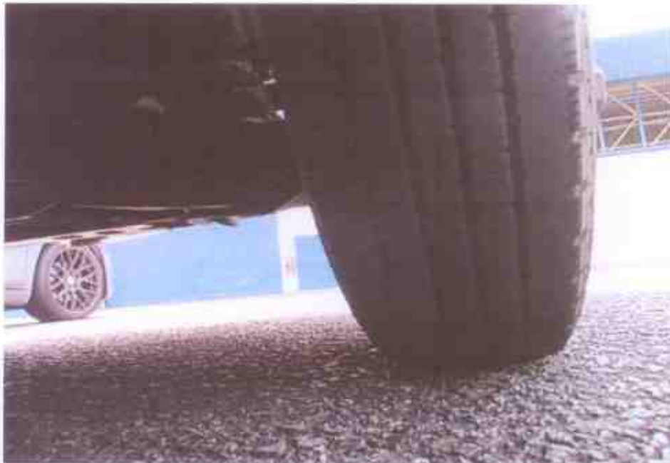
Photo 8 shows the condition of the front right tyre of the Motor Lorry, which was observed to be in serviceable condition with remaining tread depth of approximately 6mm. The tyre, which was wrapped around standard alloy wheel rim, was also observed to be sufficiently inflated for vehicular operation.
