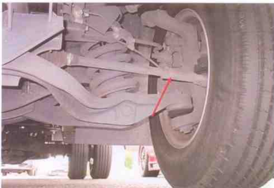
Photo 20 shows the various undercarriage components at the front left wheel of the Motor Lorry, in particular the steering tie rod end (arrowed). The various steering mechanical components of the Motor Lorry were all found to be intact without any visible damage. There was also no sign of fluid stain(s) observed on the various undercarriage components.
