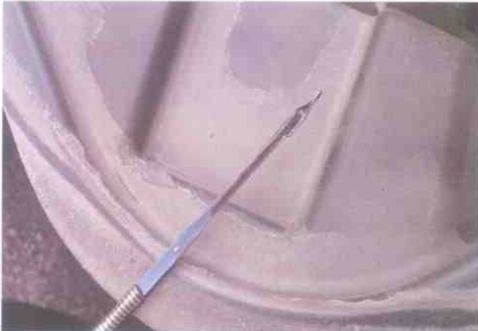
Photo 15 shows the engine oil dipstick of the Motor Lorry at the time of our inspection. The engine oil was observed to be of sufficient level and without any visible contamination.
