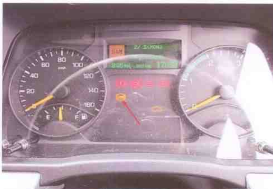
Photo 21 shows the warning lights for the various electronic operating systems of the Motor Lorry appearing on its instrument panel when the ignition was turned on, in particular the ABS light (arrowed). However no test could be carried out on the functionality of these systems at the time of our inspection (engine unable to be started).
