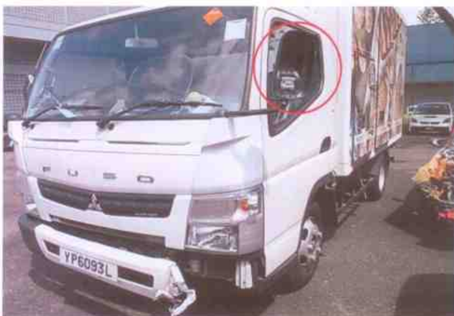
Photo 4 shows a closer view of the dislodged left side mirror of the Motor Lorry at the time of our inspection (circled).
