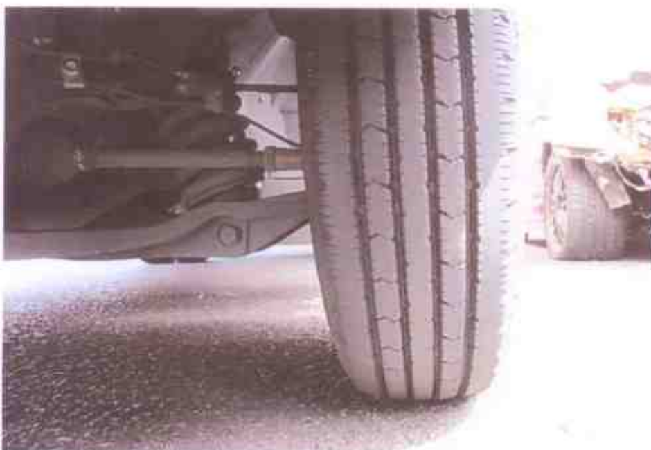
Photo 7 shows the condition of the front left tyre of the Motor Lorry, which was observed to be in serviceable condition with remaining tread depth of approximately 8mm. The tyre, which was wrapped around standard alloy wheel rim, was also observed to be sufficiently inflated for vehicular operation. There was no tear, cut or burst mark(s) on the outer and the inner sidewalls as well as across the tread of the 6 tyres that were fitted on the Motor Lorry.
