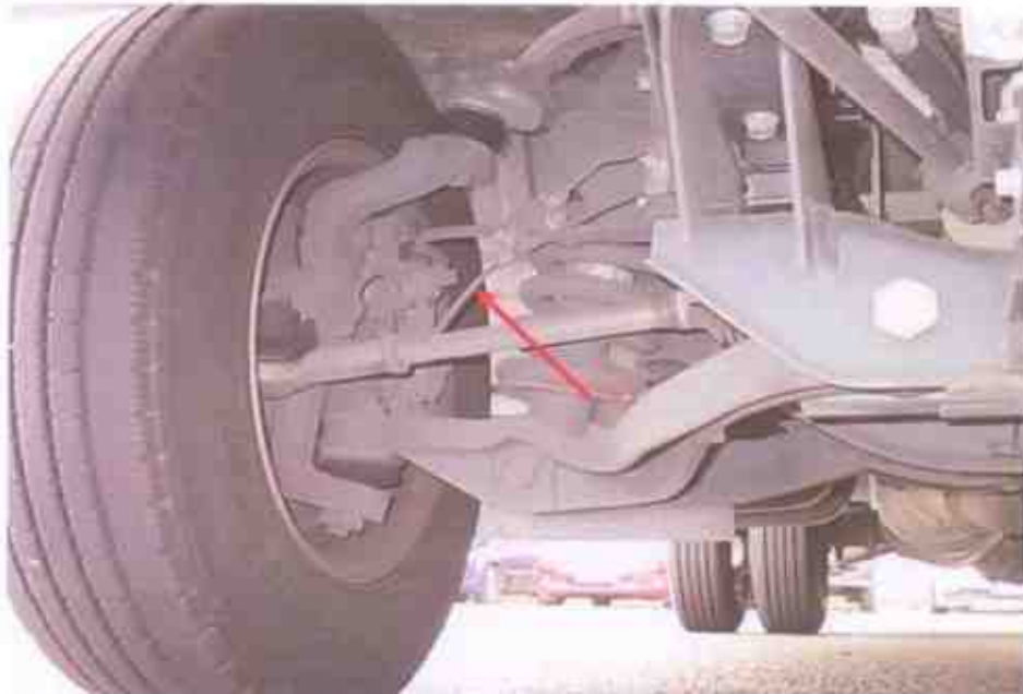
Photo 17 shows the brake pipe (arrowed) at the rear left wheel of the Motor Lorry. We did not observe any leakage of brake fluid at the time of our inspection of the Motor Lorry. Our static tests of the Motor Lorry's braking system, along with our visual examination of the various mechanical components in the braking system, had indicated that there was no internal leakage of pressure/vacuum. Hence the braking system of the Motor Lorry was likely to be in serviceable condition at the material time of accident.
