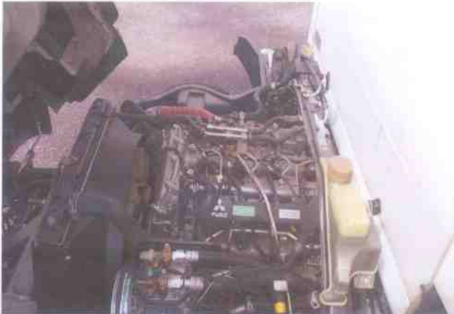
Photo 11 shows a general view of the Motor Lorry's engine compartment, which was accessed by lifting the front cabin of the Motor Lorry. The various parts and components inside the engine compartment were unaffected by the accident. There was also no sign(s) or indication(s) of fresh fluid leakage and/or fluid stain within the engine compartment (photograph shows the engine compartment as viewed from the left front side of the Motor Lorry).
