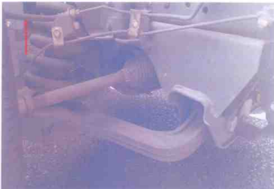
Photo 18 shows the undercarriage components at the front right wheel of the Motor Lorry, in particular the brake hose (arrowed). The Motor Lorry's braking system was likely to be in serviceable condition at the material time of accident.
