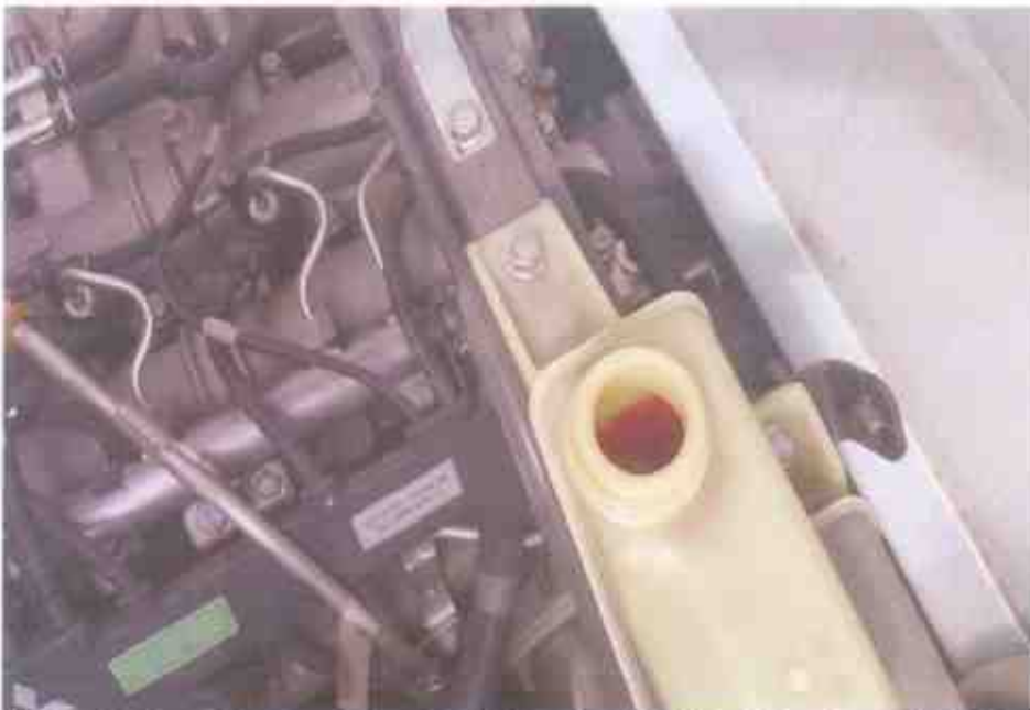
Photo 14 shows the power steering fluid reservoir of the Motor Lorry at the time of our inspection. The power steering fluid was observed to be of sufficient level and without any visible contamination.
