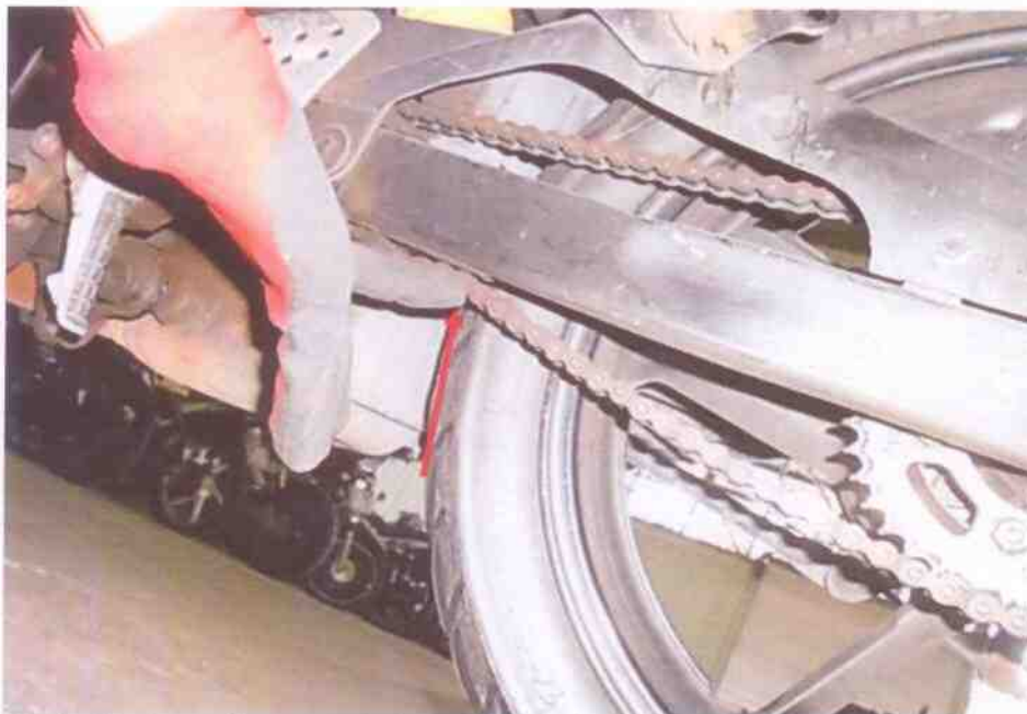
Photo 11 shows the general view of the chain gear (arrowed) of the Motorcycle. Free play tension test was conducted but found unacceptable due to its tension was too loose at time of our inspection. However, its gear chain was found adequately lubricated for operating purposes.
