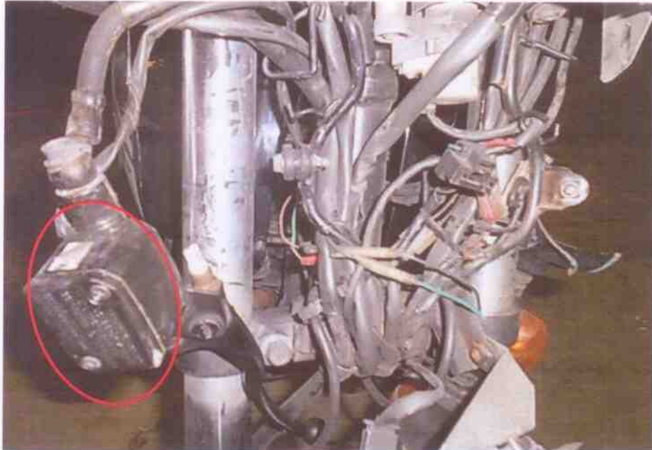
Photo 12 shows the hand brake segment (circled) was observed to be broken off & separated from the handle bar likely due to the result of the accident. Hence, we are unable to conduct any tests on the steering system of the Motorcycle.
