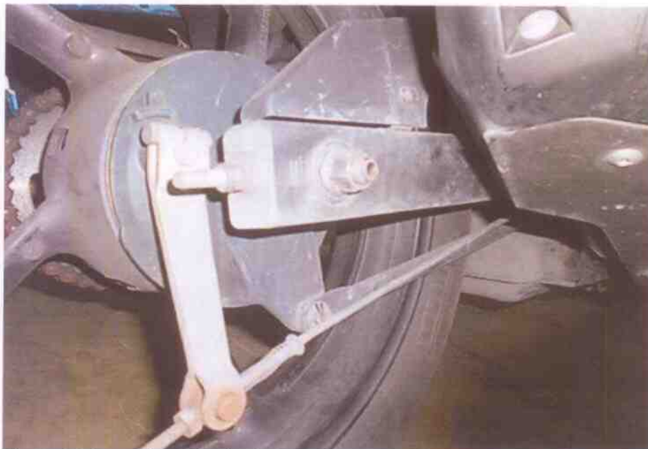
Photo 15 shows the rear wheel of the Motorcycle. The type of brake system for the rear wheel was of mechanical type, controlled by the brake foot pedal of the motorcycle. Our checks of the cable spring and drum. This is all part of the components in the rear braking system of the Motorcycle reveal all to be intact and without damages.
