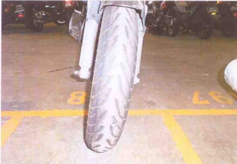
Photo 7 shows the front tyre of the Motorcycle at the time of our inspection. The pattern of the tread was clearly visible. There was no tear, burst mark(s) and/or punctured hole(s) on the sidewalls as well as across the tread of the front tyre.
