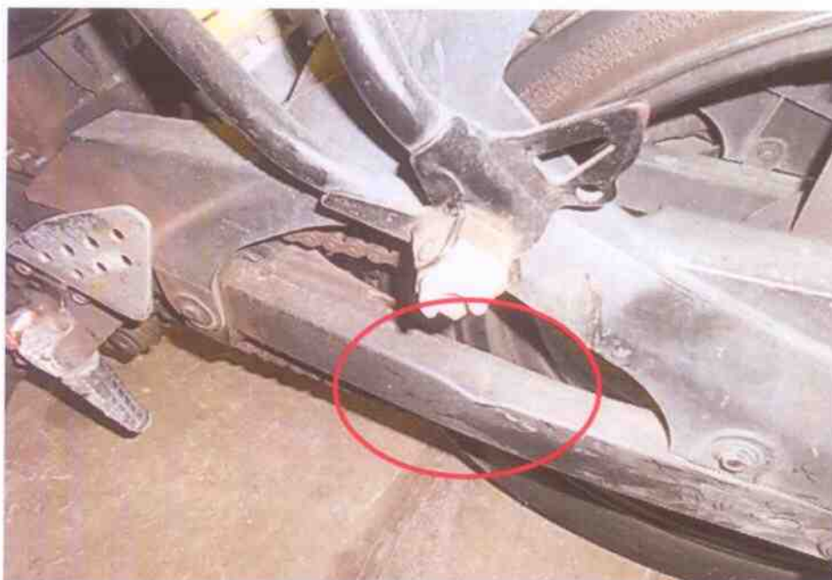
Photo 9 shows the misalignment of the drive train support bar likely due to the accident's collision impact.
