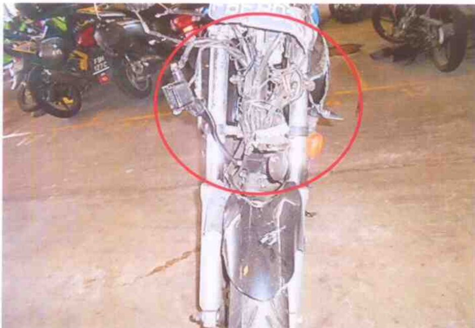
Photo 5 shows a close-up view of the frontal portion of the Motorcycle at the time of our inspection. The Motorcycle was observed to have sustained relatively extensive impact including missing speedometer & dislodged brake fluid reservoir (circled) likely due to the accident collision.
