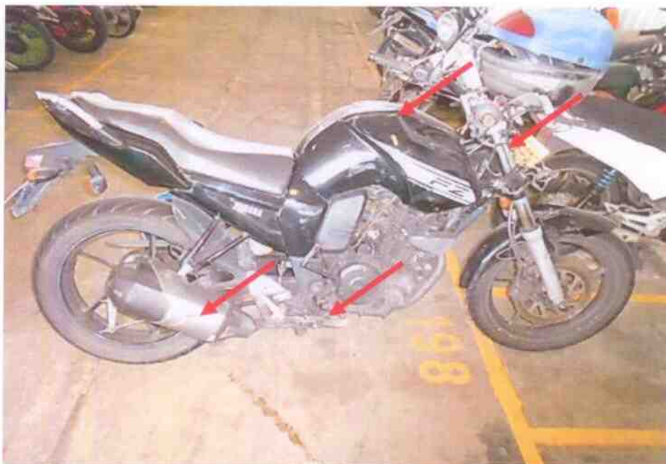
Photo 2 shows a general view of the right body of the Motorcycle at the time of our inspection. The Motorcycle was observed to have sustained with relatively extensive impact due to the accident collision. Amongst the body parts damaged was its front fork, brake pedal, fuel tank.
