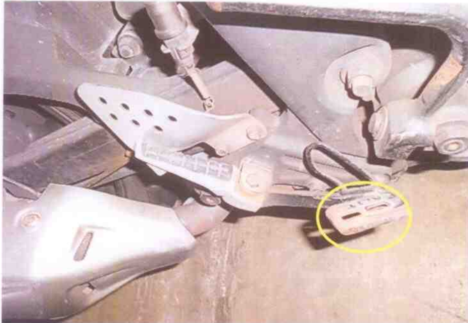
Photo 14 shows the foot brake pedal of the Motorcycle (yellow circled), which observed to be buckled in as the result of the accidents. Hence, we are unable to conduct any brake test.
