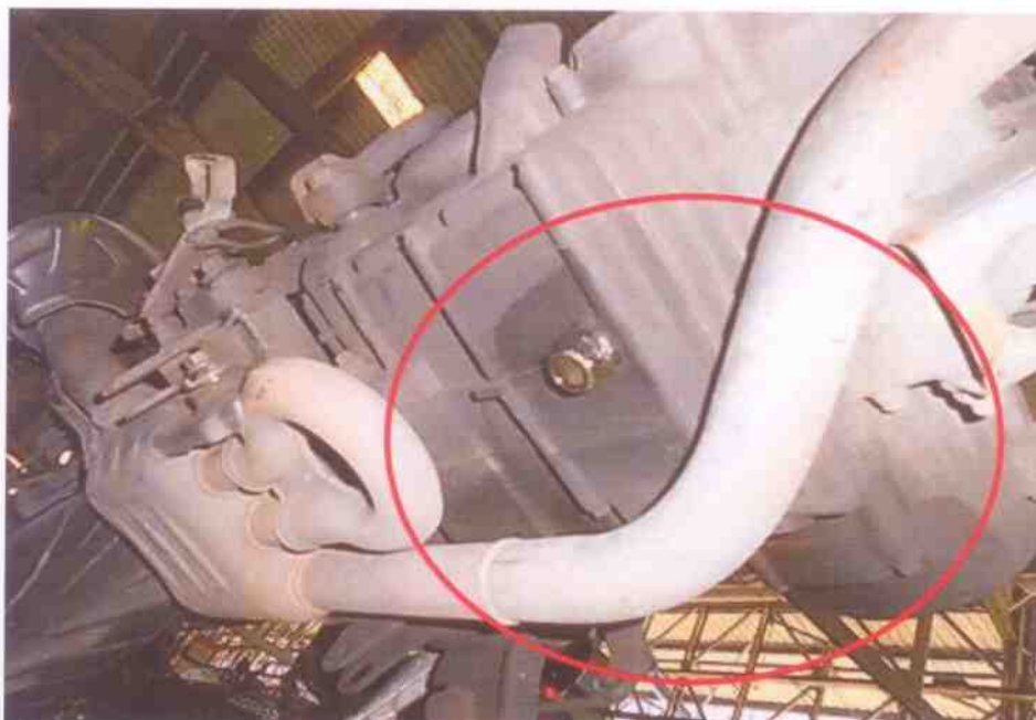
Photo 8 shows sign(s) or indication(s) of fluid leakage observed around the engine's underside area of the Motorcycle.
