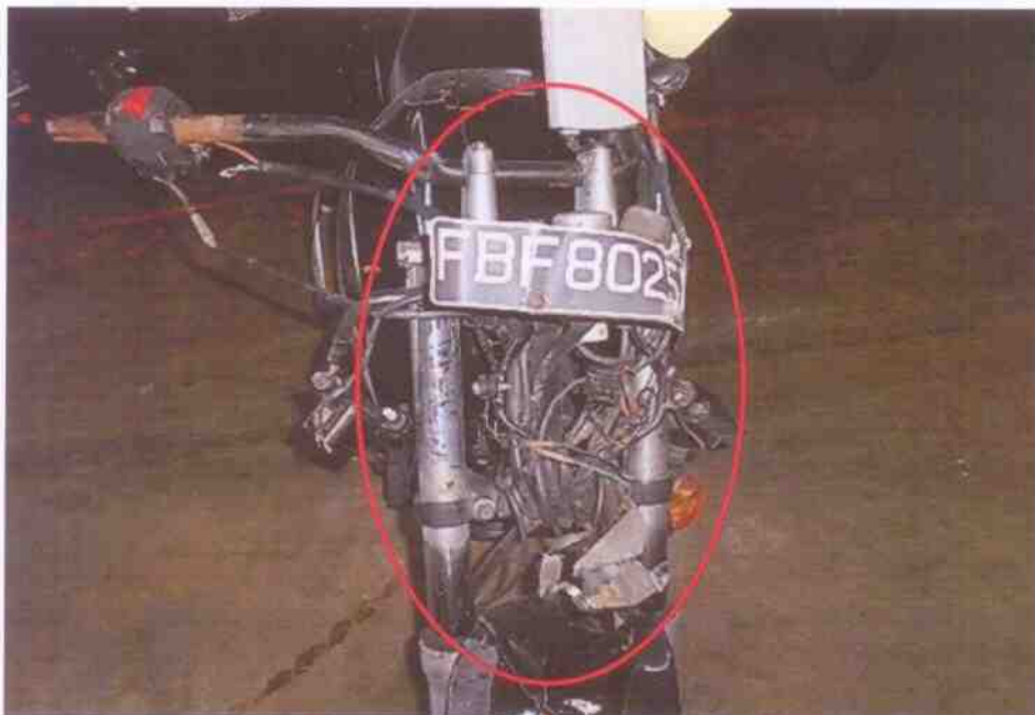
Photo 13 shows the front fork (circled) was observed to be misaligned as a result of the accident. Hence, we are unable to conduct any tests on the steering system of the Motorcycle.
