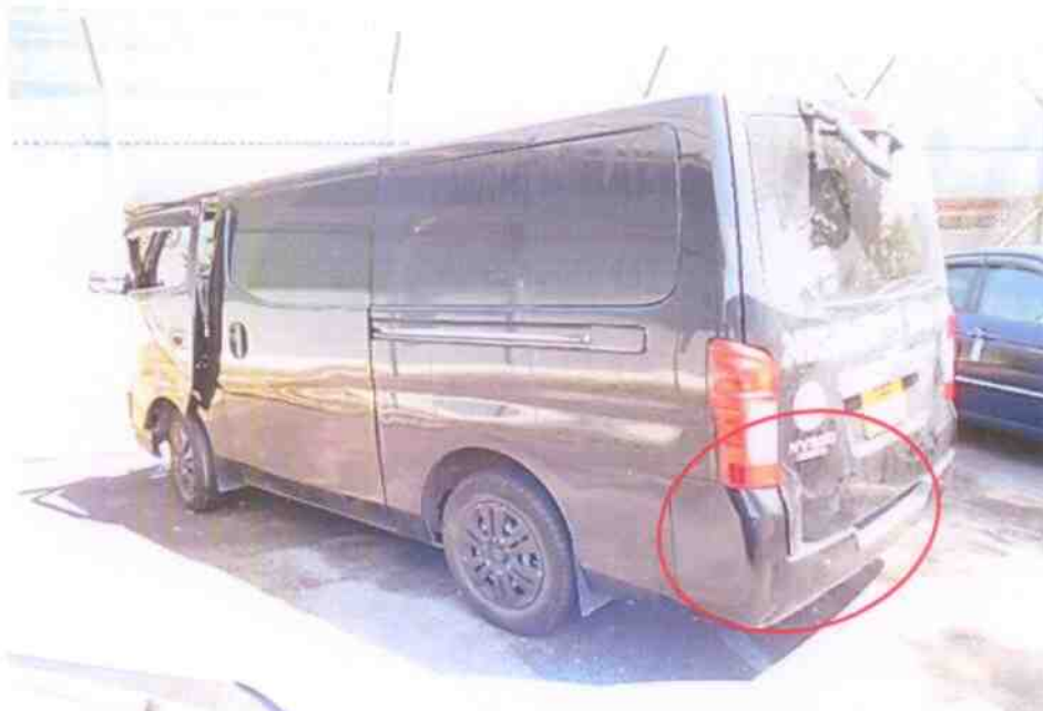
Photo 13 shows a general view of the rear left portion of the Motor Van at the time of our inspection. The rear portion was observed to have sustained with minor damages likely not related to the accident.
