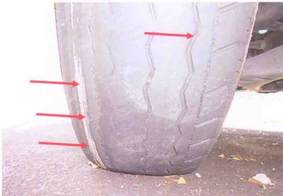
Photo 17 shows the condition of the front left tyre of the Motor Van, which was observed not to be in serviceable condition. Although the tread pattern was still visible, the inner cores of the tyre were found to be exposed at the outer side of the tyres.
