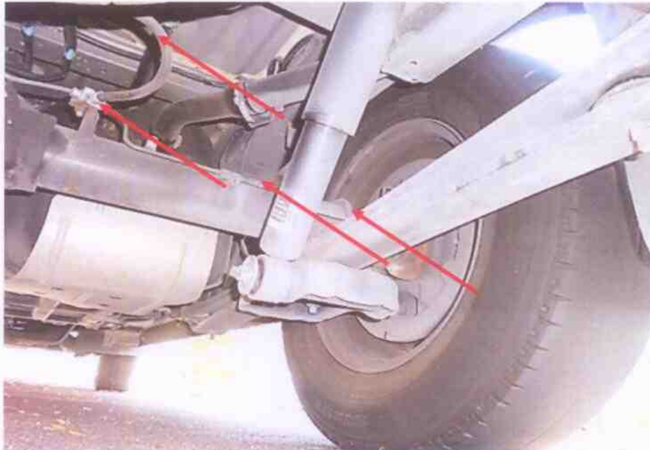
Photo 32 shows the braking components at the rear right wheel of the Motor Van. We did not observe any leakage of brake fluid at the time of our inspection of the Motor Van.
