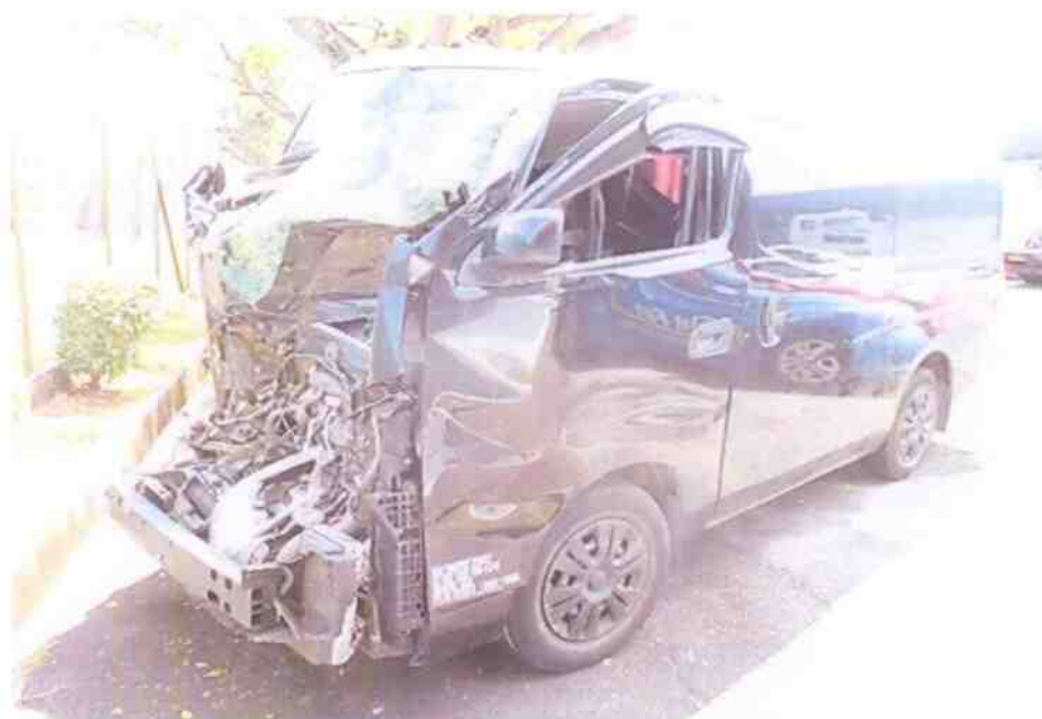
Photo 3 shows a general view of the front left portion of the Motor Van at the time of our inspection. The Motor Van was observed to have sustained with extensive impact damage at its frontal portion.
