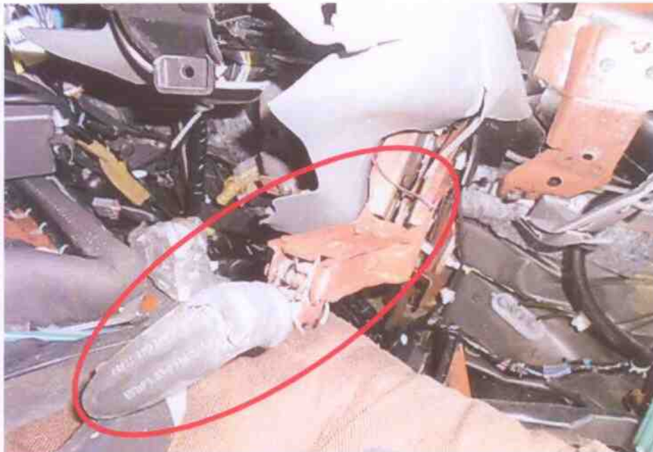
Photo 26 shows the close up view of the hand brake that was observed to be damaged likely due to the accident impact
