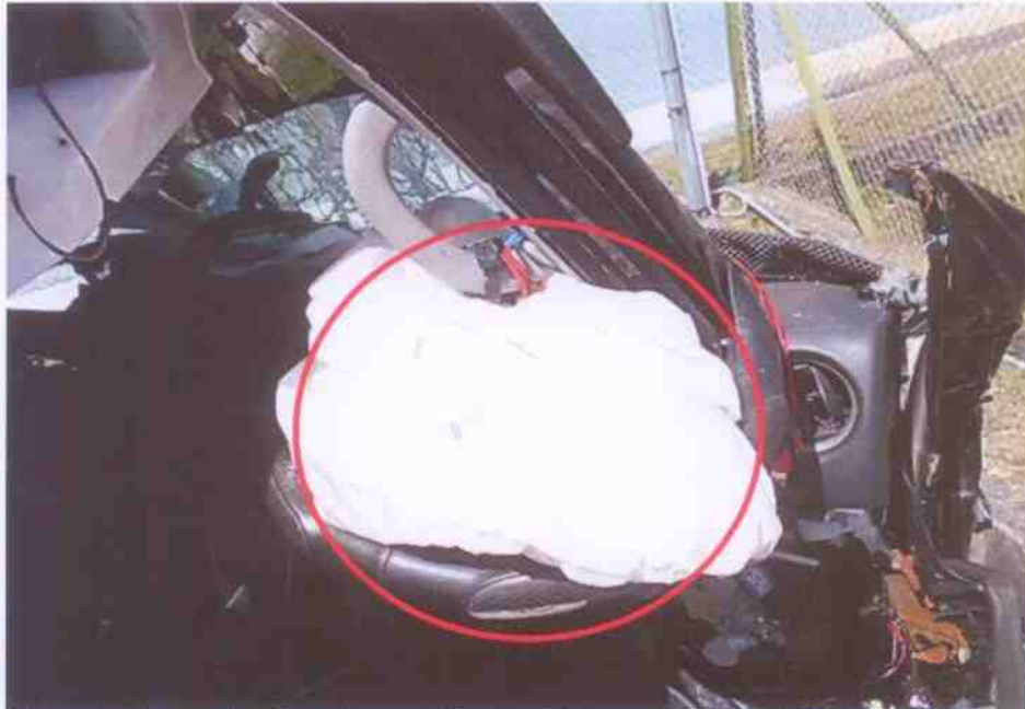
Photo 35 shows the Supplemental Restraint System (SRS) of the Motor Van was however likely to be in normal operating condition at the material time of the accident. The evidence of the deployed front passenger's airbag indicates that the impact sensors and control module of the Motor Van's SRS were all in serviceable condition at the material time of accident.
