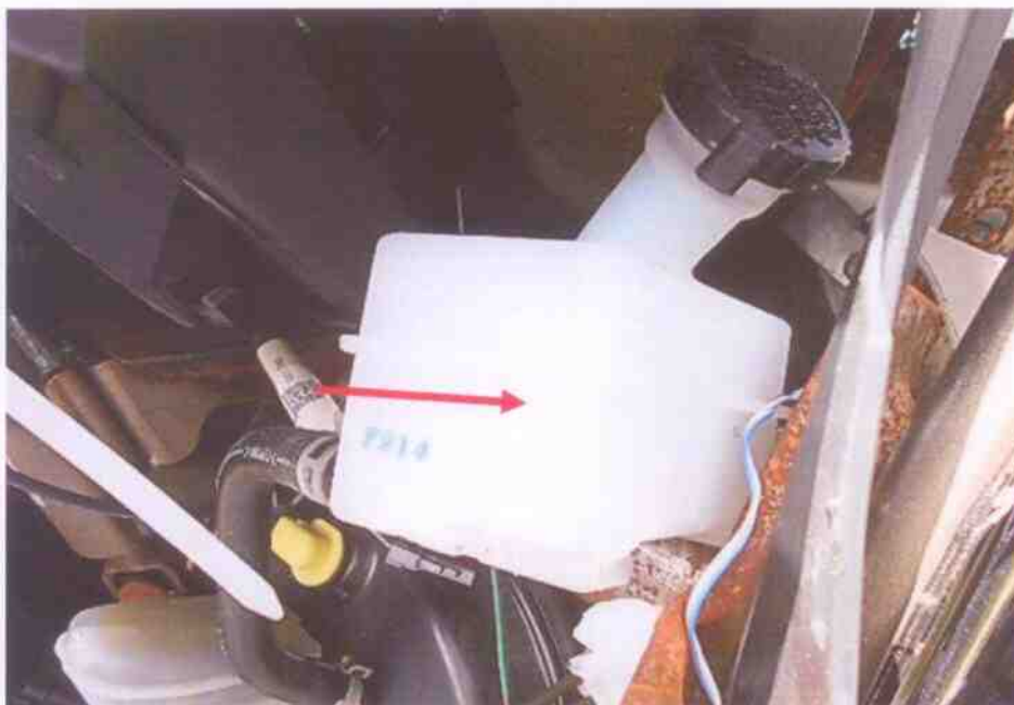
Photo 23 shows the close up view of the brake fluid reservoir that indicates empty likely due to the accident impact.
