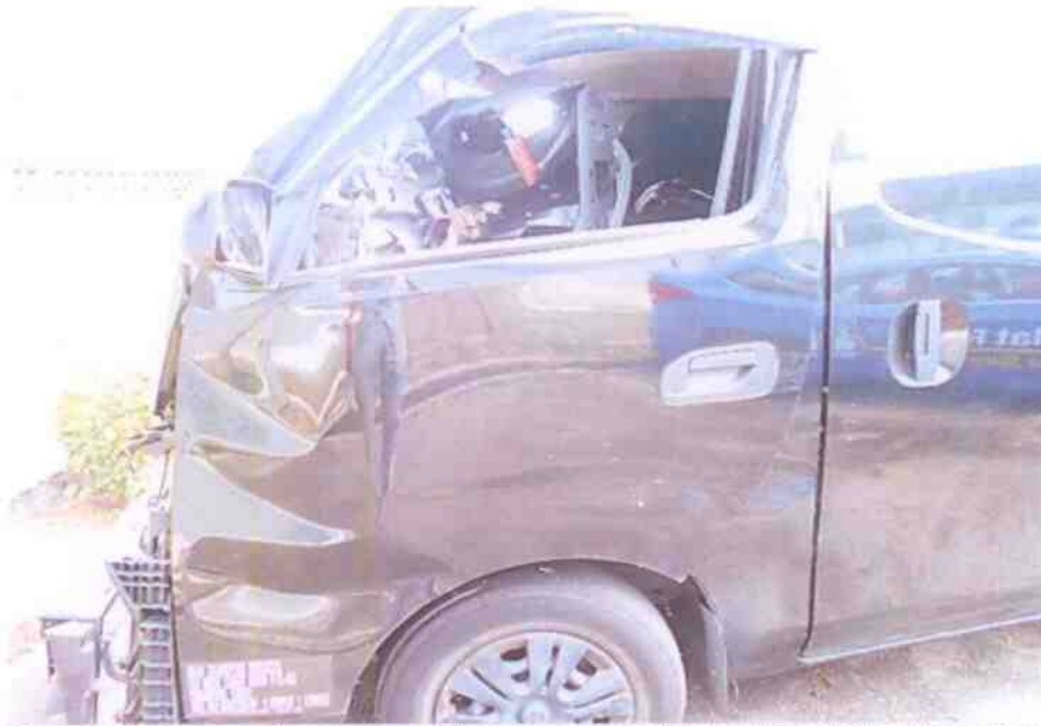
Photo 12 shows a closer view of the damaged left front door of the Motor Van. The impact force was significant, causing the various parts and components inside the engine compartment to be pushed inwards, towards the rear of the Motor Van.
