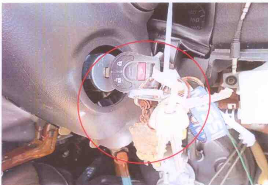
Photo 9 shows a closer view of the damage at the ignition section of the Motor Van. The impact force was significant, causing the various parts and components inside the interior compartment to be pushed inwards, including its ignition system.
