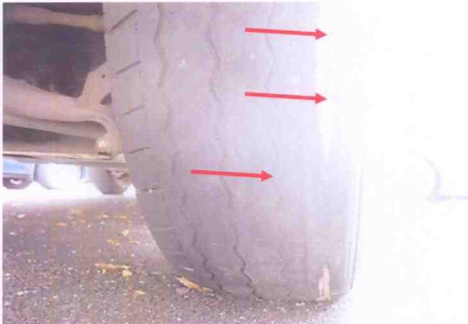
Photo 19 shows the condition of the front left tyre of the Motor Van, which was observed not to be in serviceable condition. Although the tread pattern was still visible, the inner core of the tyre was found to be exposed at the outer side of the tyres.
