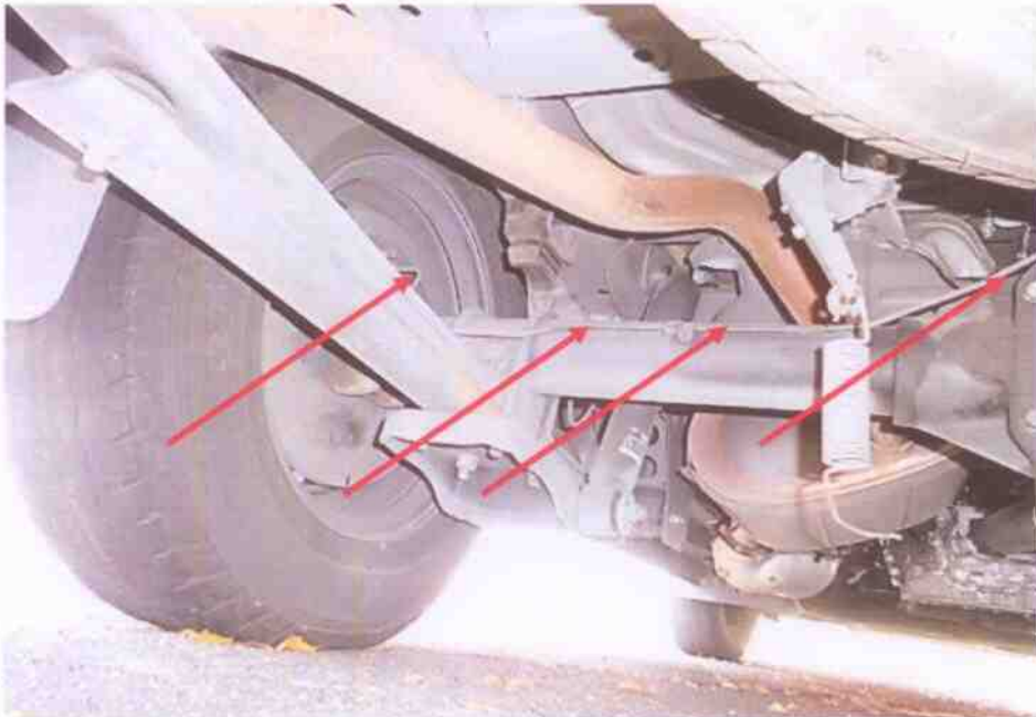
Photo 33 shows the braking component at the left right wheel of the Motor Van. We did not observe any leakage of brake fluid at the time of our inspection of the Motor Van.
