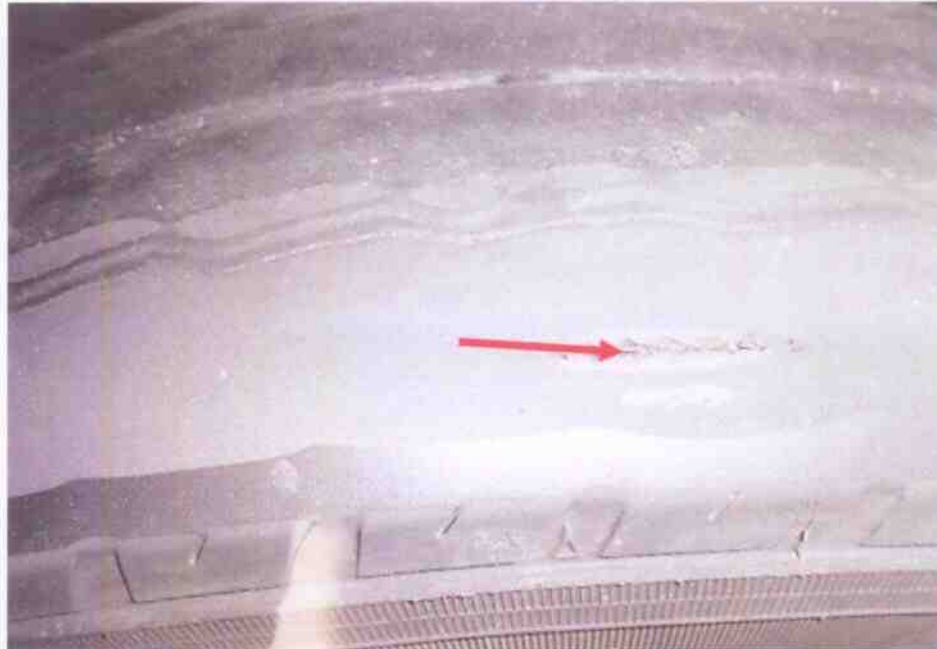
Photo 16 shows the condition of the front right tyre of the Motor Van. Although the tread pattern was still visible, the inner core of the tyre was found to be exposed at the outer side of the tyres.
