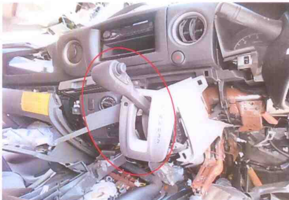
Photo 8 shows a closer view of the damage gear knob at the interior portion of the Motor Van. The impact force was significant, causing the various parts and components inside the engine compartment to be pushed inwards, towards the rear of the Motor Van including its transmission system.
