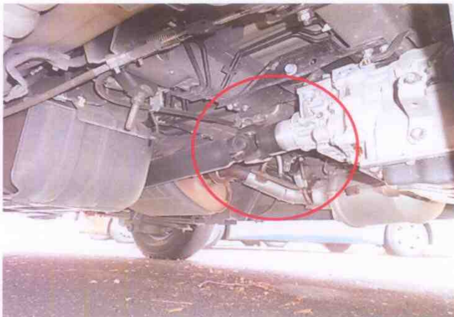
Photo 34 shows the engine transmission of the Motor Van. It was observed to be in good condition at the time of our inspection of the Motor Van.
