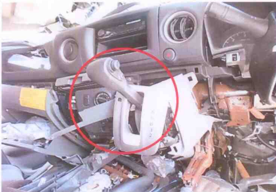
Photo 27 shows the close up view of the gear knob for transmission control that was observed to be damaged likely due to the accident impact
