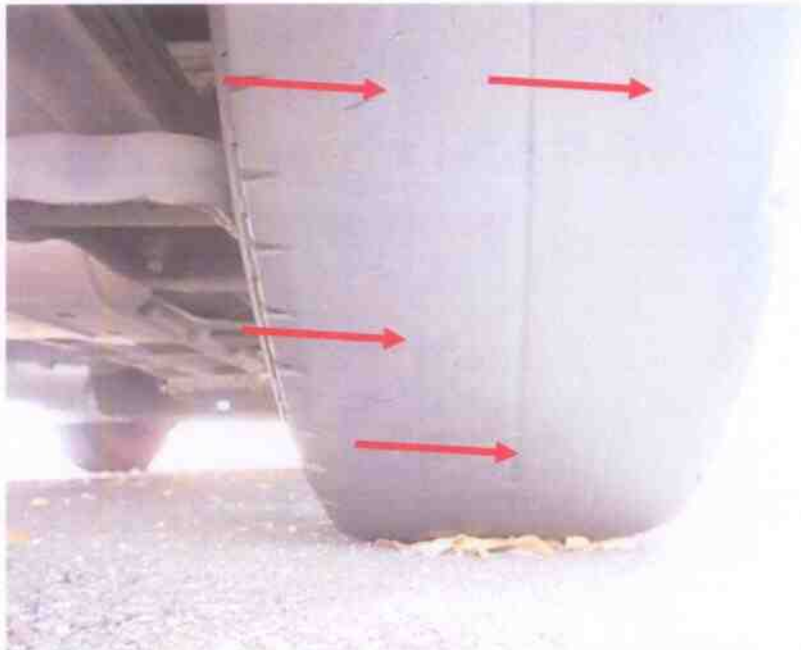
Photo 22 shows the condition of the rear right tyre of the Motor Van, which was observed not to be in serviceable condition. Although the tread pattern was still visible, its tread depth was found to be (0.2mm) below the minimum range of (1mm).
