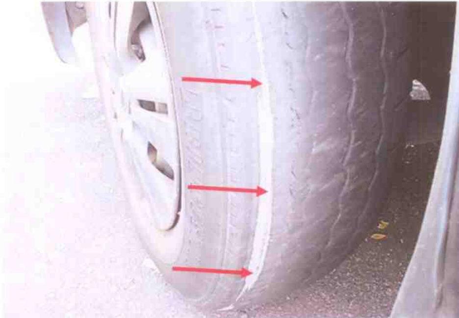
Photo 18 shows the condition of the front left tyre of the Motor Van, which was observed not to be in serviceable condition. Although the tread pattern was still visible, the inner core of the tyre was found to be exposed at the outer side of the tyres.
