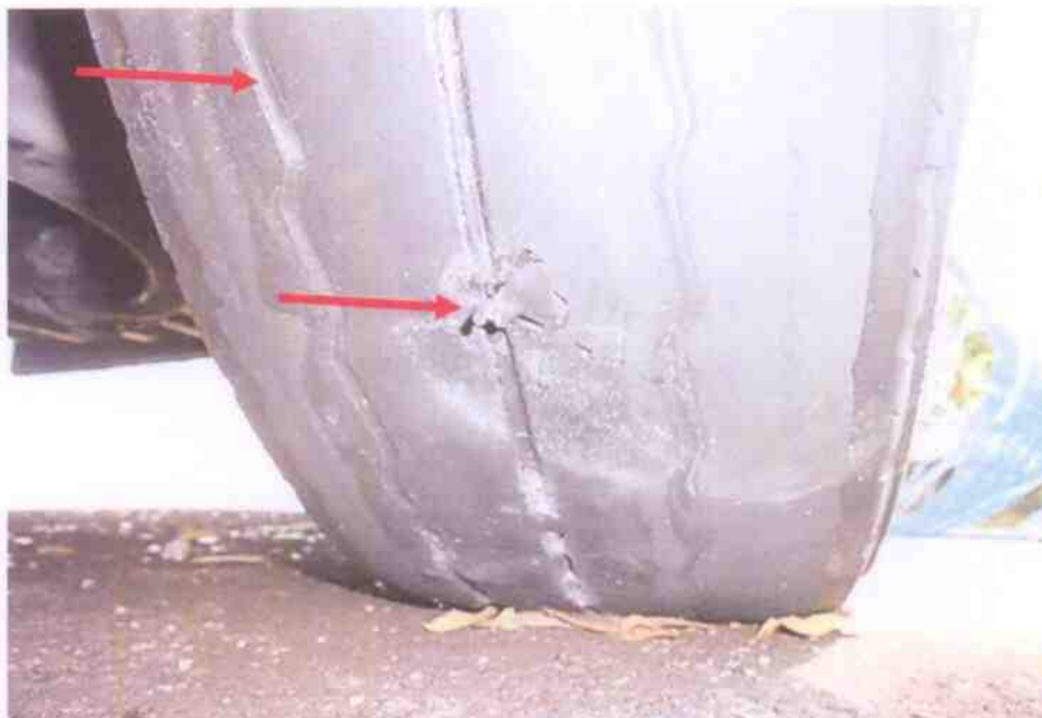
Photo 15 shows the condition of the front right tyre of the Motor Van, which was found to be cut at across the tread pattern of the tyres. However, the tread pattern was still visible (1.6mm) & observed to be inflated for operational purposes.
