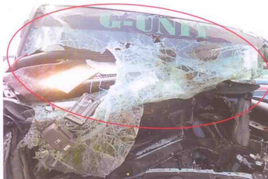
Photo 11 shows a closer view of the damage at the windscreen area of the Motor Van. The impact force was significant, causing the windscreen to sustain a shattering cracked.
