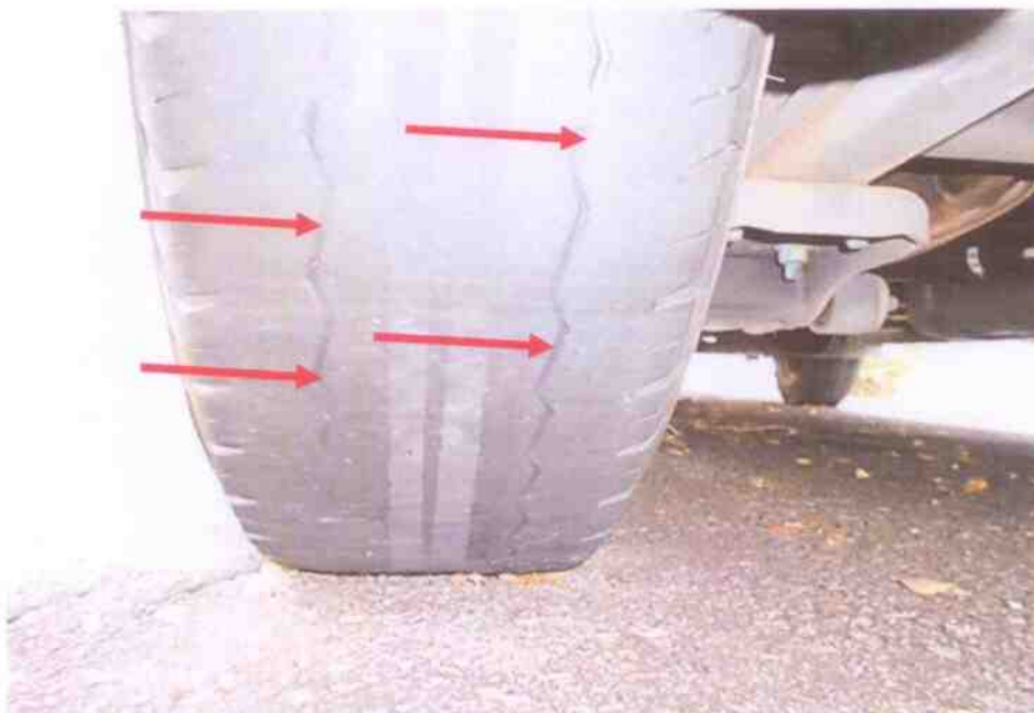
Photo 21 shows the condition of the rear left tyre of the Motor Van, which was observed not to be in serviceable condition. Although the tread pattern was still visible, its tread depth was found to be (0.5mm) below the minimum range of 1mm.
