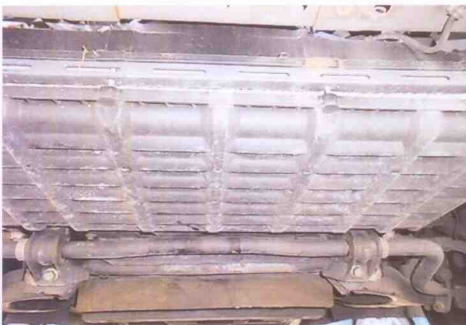
Photo 24 shows the close up view of the radiator undercarriage was observed to be unaffected by the accident.
