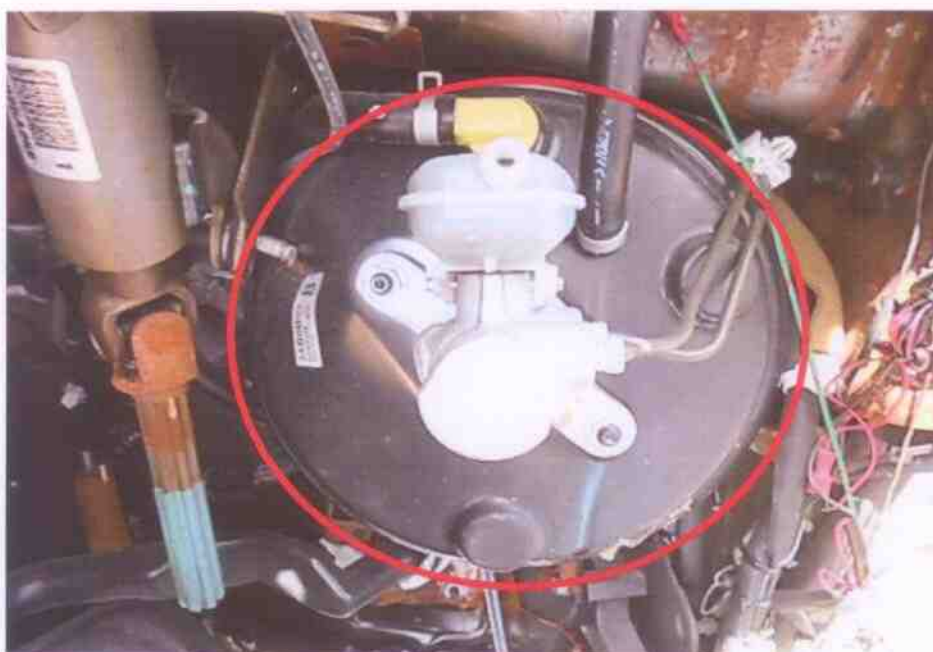
Photo 25 shows the close up view of the brake booster that was observed to be damaged likely due to the accident impact.
