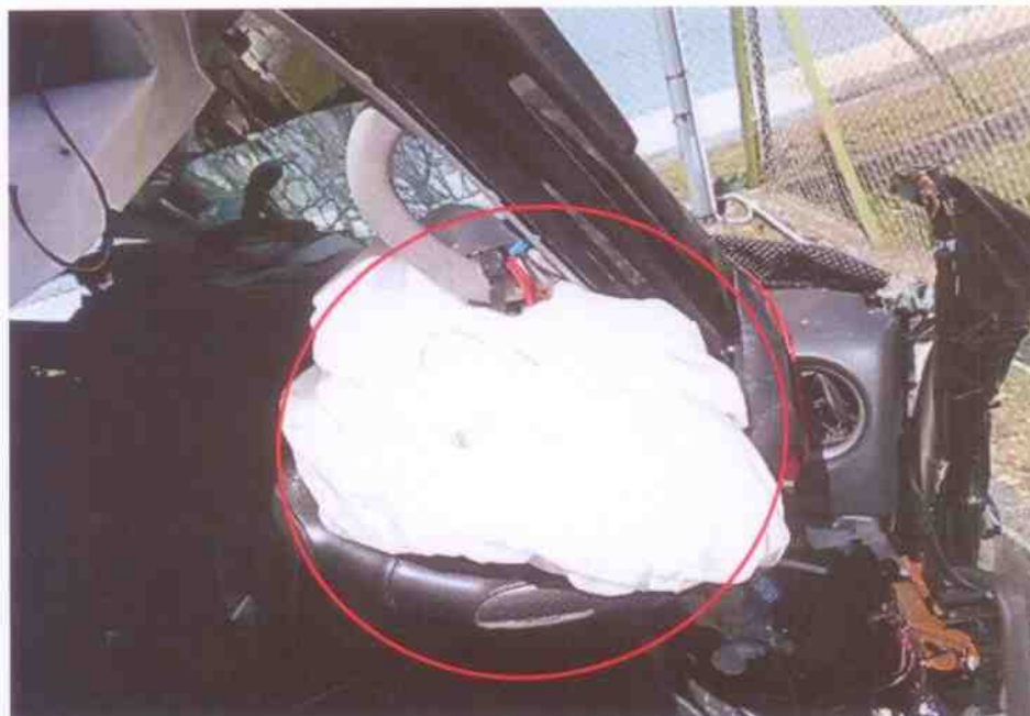
Photo 10 shows a closer view of the detached right front door of the Motor Van. The impact force was significant, causing the various parts and components inside the engine compartment to be pushed inwards, towards the rear of the Motor Van. That includes the driver's airbag activation.
