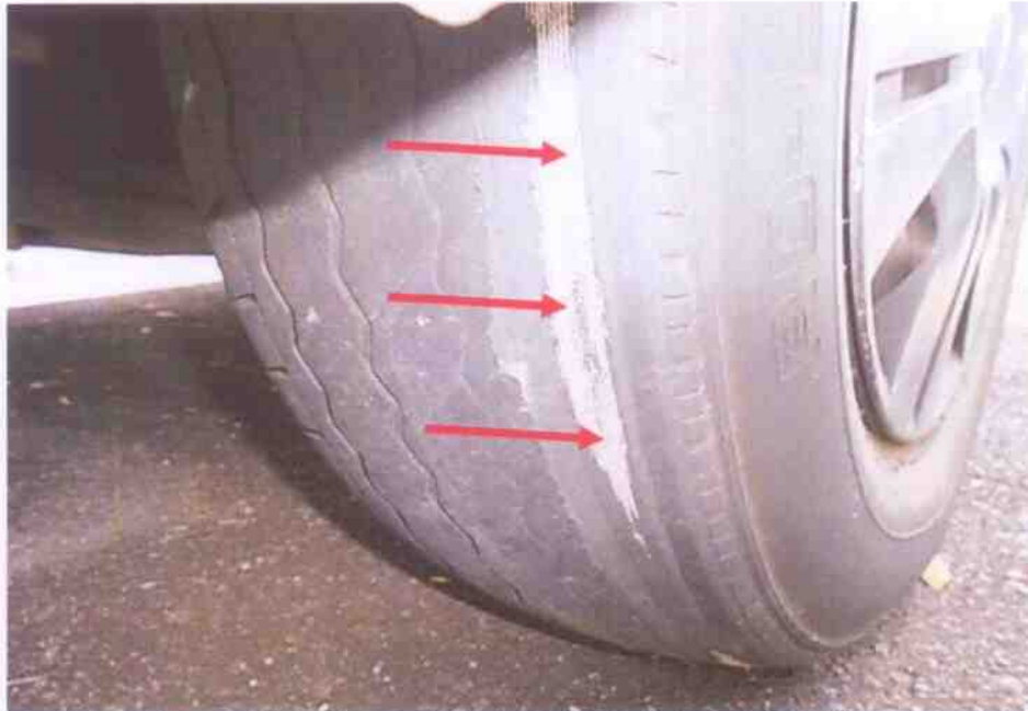
Photo 20 shows the condition of the front left tyre of the Motor Van, which was observed not to be in serviceable condition. Although the tread pattern was still visible, the inner core of the tyre was found to be exposed at the outer side of the tyres.
