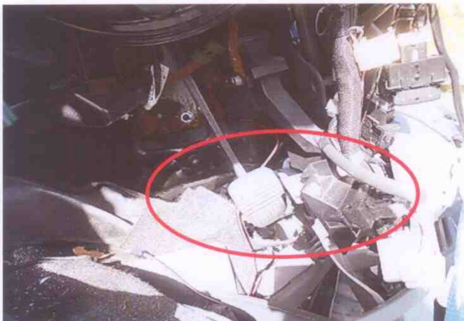
Photo 29 shows the close up view of the brake pedal & acceleration pedal that was observed to be damaged likely due to the accident impact
