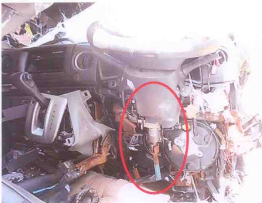
Photo 28 shows the close up view of the steering wheel rod that was observed to be damaged likely due to the accident impact
