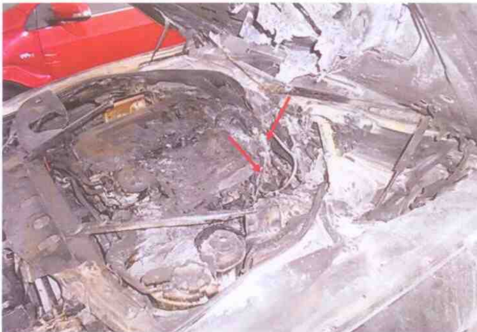
Photo 10 shows the wirings around the rear left side of the engine compartment which is near to the vicinity where the fire to the Insured Vehicle had likely started.
