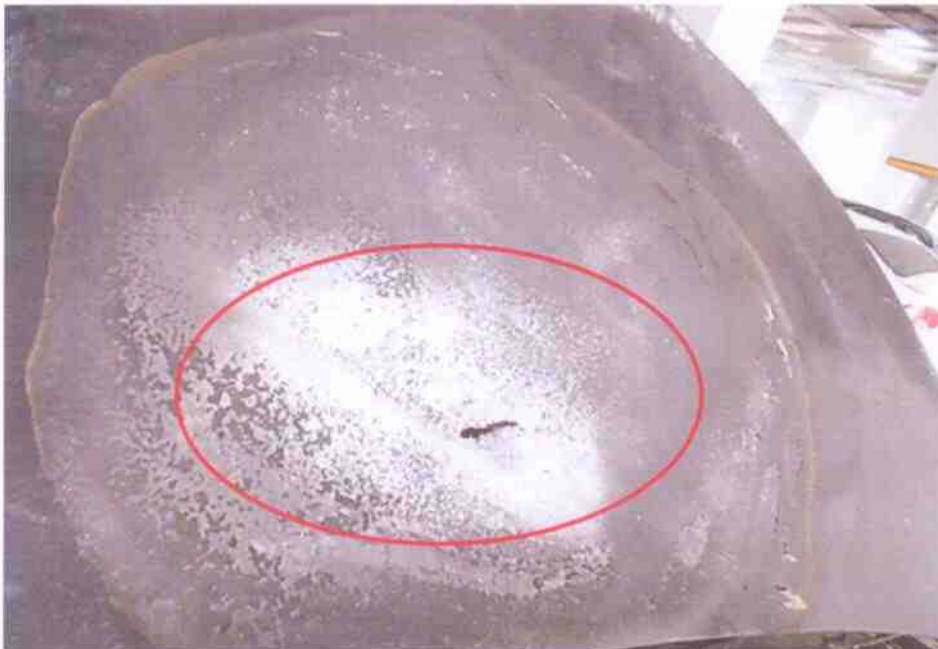
Photo 6 shows a close-up view of the burn pattern and whitish burn marks (circled) that were found on the rear left side of the front bonnet of the Insured Vehicle. Such whitish burn marks are a result of exposure to prolonged heat intensity, which may indicate where the fire had started. Rust would also begin to develop on these areas soon after the fire.
