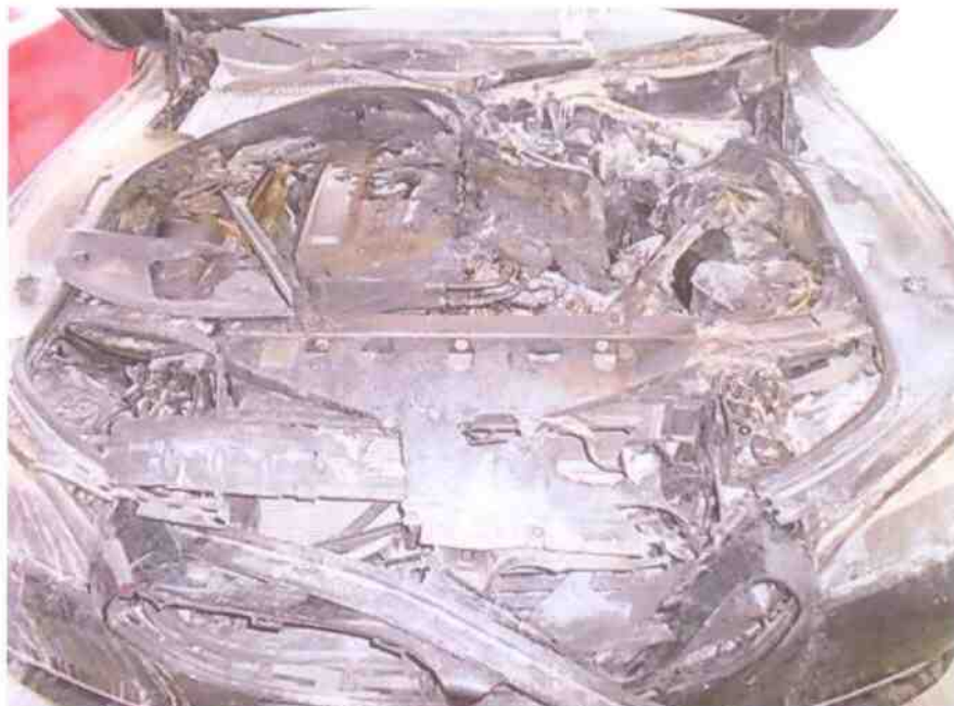
Photo 3 shows the engine compartment of the Insured Vehicle at the time of our inspection. The rear left side of the entire engine compartment of the Insured Vehicle was observed to be partially burnt. The parts around the rear left side of the engine compartment were found to be burnt and/or melted as a result of the fire.
