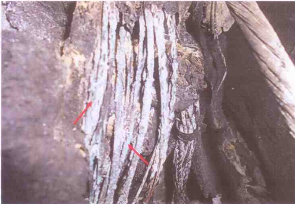
Photo 12 shows a closer view of the burnt wirings (red arrows) at the rear left side of the engine compartment. Such condition normally indicates internal heating of copper wires which is a sign of an electrical short circuit occurring.
