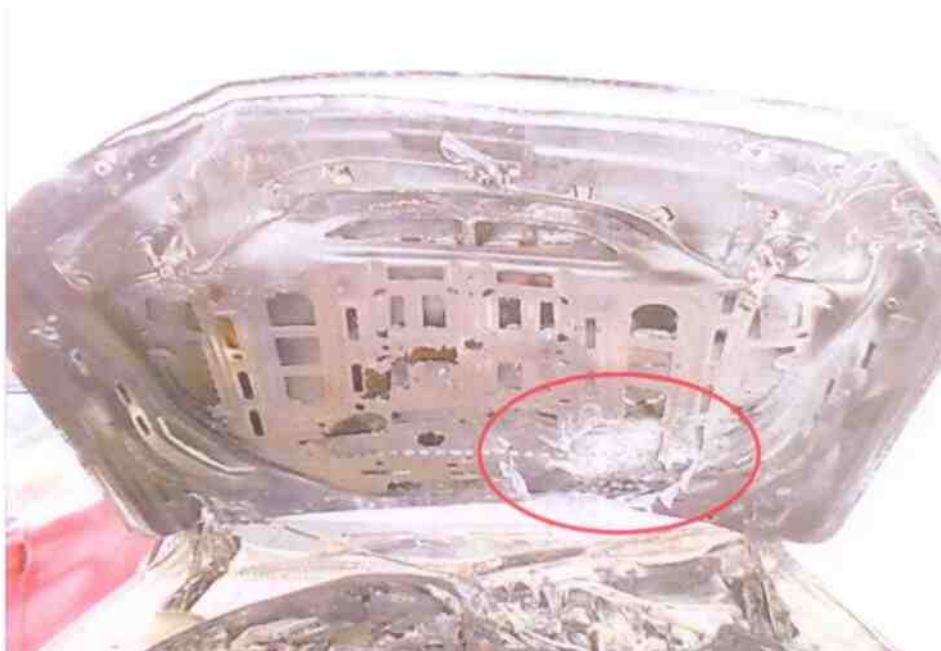
Photo 7 shows the discolouration of the insulating material on the underside of the front bonnet, around the rear left side area (circled). The discolouration of the insulating material is an indication that the rear left side area of the engine compartment had sustained exposure to prolonged high heat intensity. Hence the fire to the Insured Vehicle can be determined to have originated towards the rear left side of the engine compartment.
