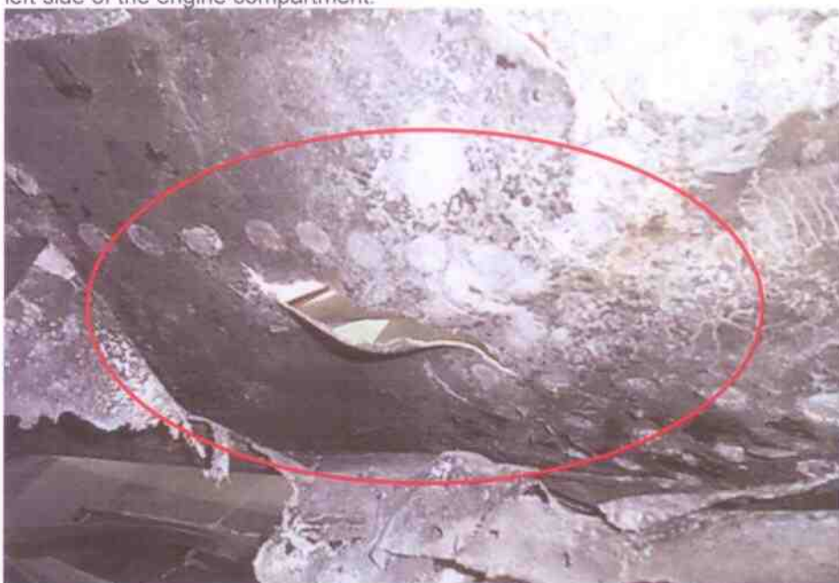
Photo 8 shows a close-up view of the discolouration of the insulating material on the underside of the front bonnet, around the rear left side area (circled). The discolouration of the insulating material is an indication that the rear left side area of the engine compartment had sustained exposure to prolonged high heat intensity. Hence the fire to the Insured Vehicle can be determined to have originated towards the rear left side of the engine compartment.
