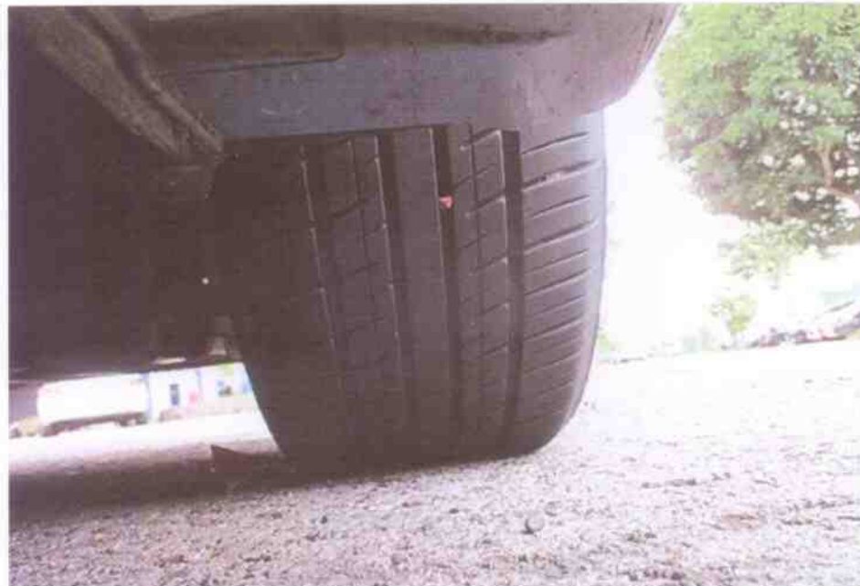
Photo 7 shows the condition of the front right tyre of the Motor Taxi, which was observed to be in serviceable condition with remaining tread depth of approximately 6mm. The tyre, which was wrapped around standard wheel rim, was also observed to be sufficiently inflated for vehicular operation.
