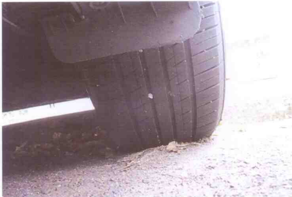
Photo 8 shows the condition of the rear left tyre of the Motor Taxi, which was observed to be in serviceable condition with remaining tread depth of approximately 6mm. The tyre, which was wrapped around standard wheel rim, was also observed to be sufficiently inflated for vehicular operation. There was no significant damage observed on the 4 wheel rims of the Motor Taxi apart for some relatively minor kerb grazing type of damage found on all the 4 wheel rims.
