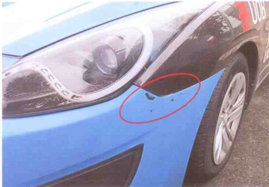
Photo 4 shows a closer view of the damage marks of grazing nature observed at the left corner of the front bumper of the Motor Taxi at the time of our inspection (circled).
