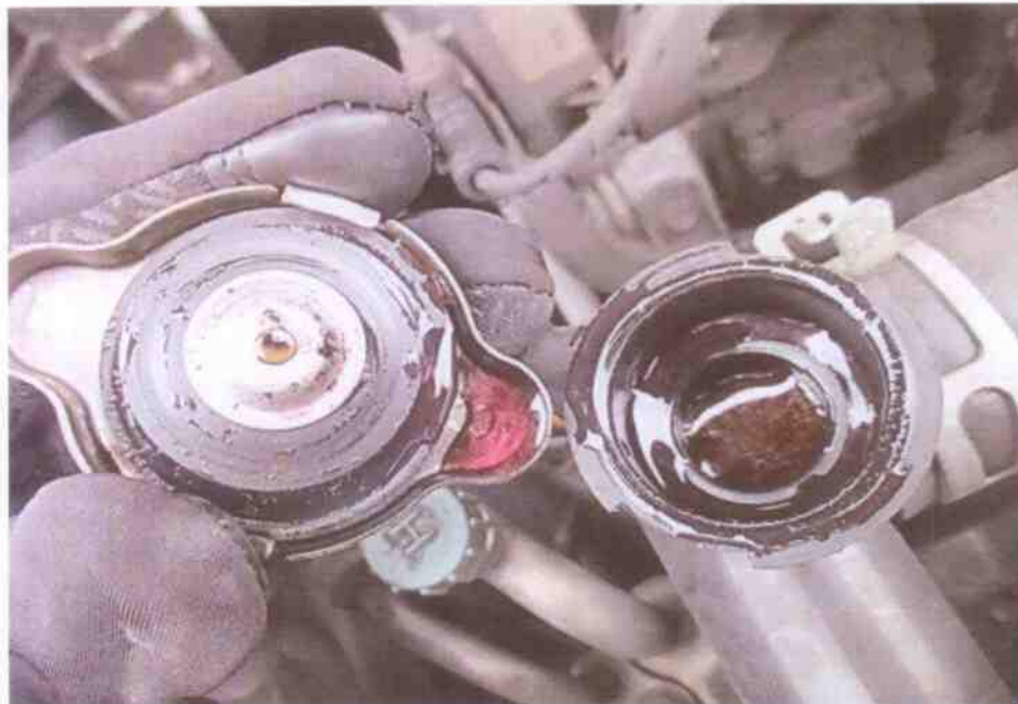
Photo 12 shows checks being carried out to the engine coolant of the Motor Taxi at the time of our inspection. The engine coolant was observed to be of sufficient level and without any visible contamination.
