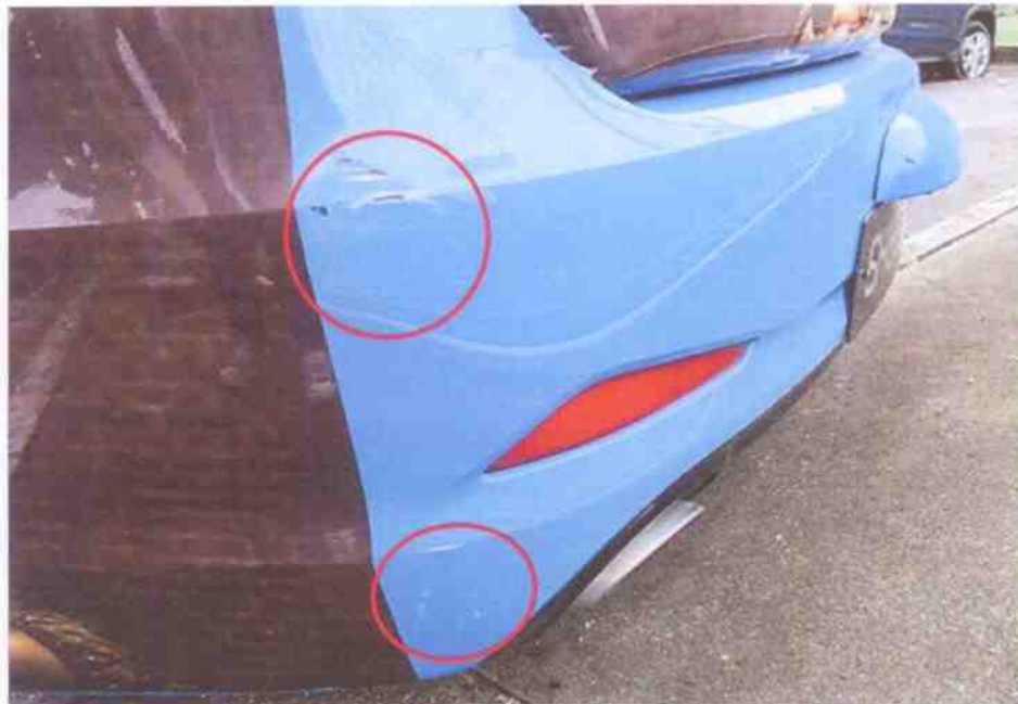
Photo 5 shows a closer view of the damage marks of grazing nature observed at the left side of the rear bumper of the Motor Taxi at the time of our inspection (circled).
