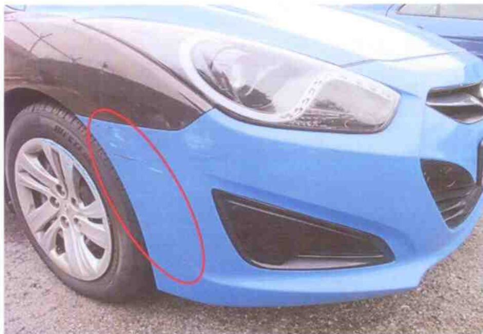
Photo 3 shows a closer view of the damage marks of grazing nature observed at the right corner of the front bumper of the Motor Taxi at the time of our inspection (circled).
