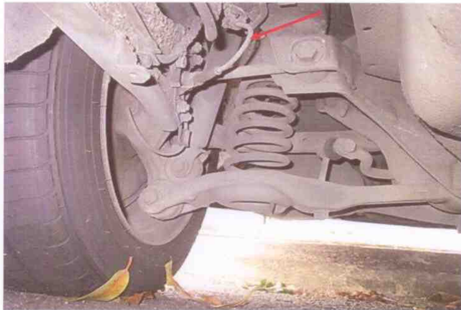
Photo 14 shows the brake hose (arrowed) at the rear left wheel of the Motor Taxi. We did not observe any leakage of brake fluid at the time of our inspection of the Motor Taxi. Our visual inspection of the various mechanical components of the Motor Taxi's braking system revealed all to be intact and without visible damage, indicating that the braking system was likely to be in serviceable condition at the material time of accident.
