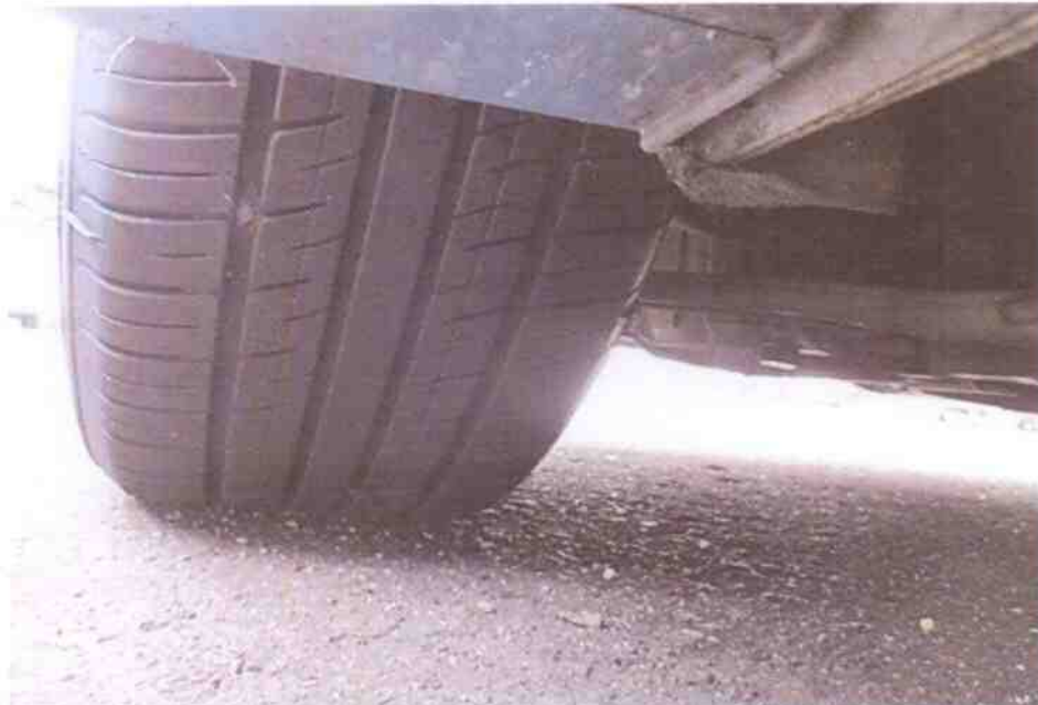
Photo 6 shows the condition of the front left tyre of the Motor Taxi, which was observed to be in serviceable condition with remaining tread depth of approximately 5mm. The tyre, which was wrapped around standard wheel rim, was also observed to be sufficiently inflated for vehicular operation. There was no tear, cut or burst mark(s) on the outer and the inner sidewalls as well as across the tread of the Motor Taxi's 4 tyres.
