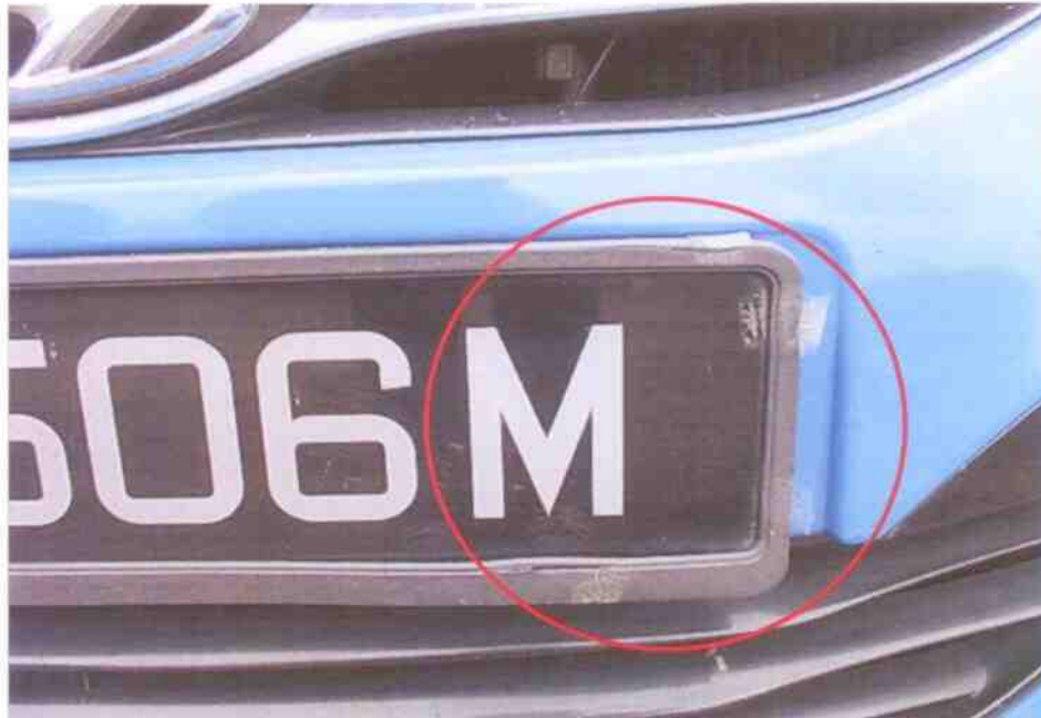
Photo 2 shows a closer view of the damaged front number plate holder of the Motor Taxi at the time of our inspection (circled).
