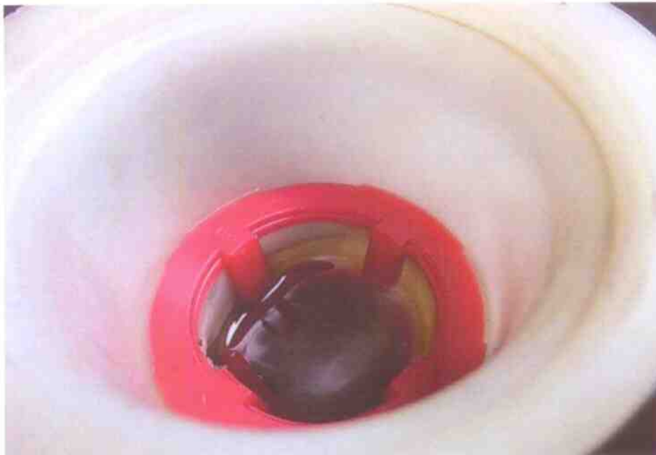
Photo 11 shows the brake fluid reservoir of the Motor Taxi at the time of our inspection. The brake fluid was observed to be of sufficient level and without any visible contamination.
