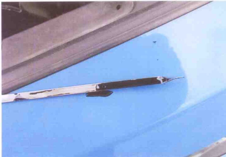
Photo 13 shows the engine oil dipstick of the Motor Taxi at the time of our inspection. The engine oil was observed to be of sufficient level and without any visible contamination.
