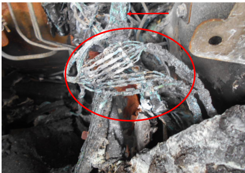
Photo 10 shows another stretch of wirings with greenish residue (arrowed and circled) at the rear left area of the Insured Vehicle's engine compartment. The presence of such greenish residue suggests occurrence of an electrical short circuit.
