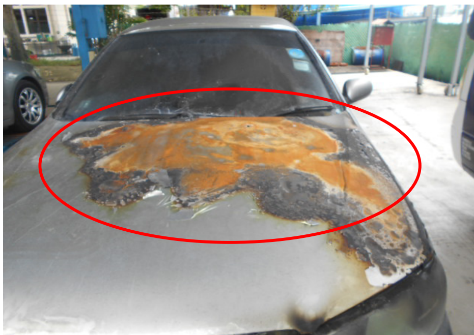
Photo 5 shows the rust (circled) that was found on the top side of the front bonnet of the Insured Vehicle. The presence of rust on a steel/metal material body panel of a vehicle that was involved in a fire incident is a consequence of that body panel being exposed to natural environmental condition after the layers of paint and its related compounds were melted due to prolong exposure of high heat intensity to that body panel. Such physical evidence can normally indicate where the fire of a vehicle had originated.
