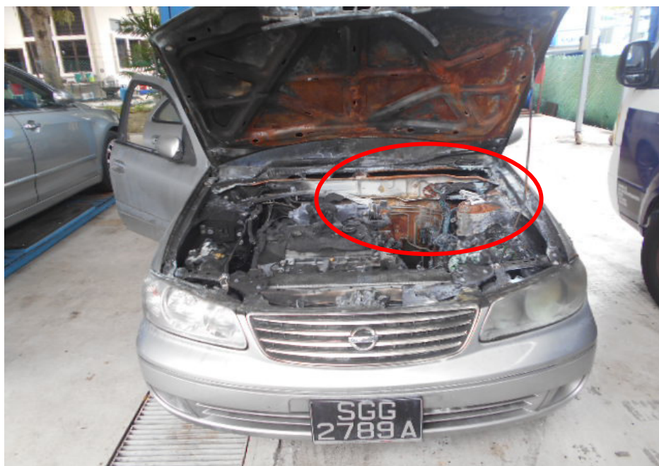
Photo 7 shows a general view of where the fire to the Insured Vehicle had originated, which was somewhere around the left and towards the rear of the engine compartment (circled). This was established given the localized area on the Insured Vehicle where rust had developed.
