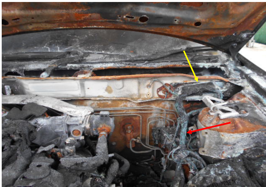
Photo 8 shows the wirings around the left rear of the engine compartment, which is in the immediate vicinity where the fire to the Insured Vehicle had likely started. Greenish residue was found on the wirings (red arrow) leading to the Engine Control Module (ECM) (yellow arrow). The presence of such greenish residue suggests occurrence of an electrical short circuit.
