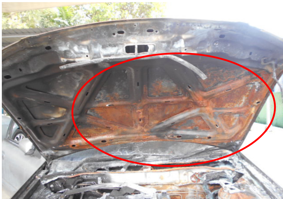
Photo 6 shows the rust (circled) that was found on the underside of the front bonnet of the Insured Vehicle, directly under the area of the top side of the front bonnet, where rust had also developed.
