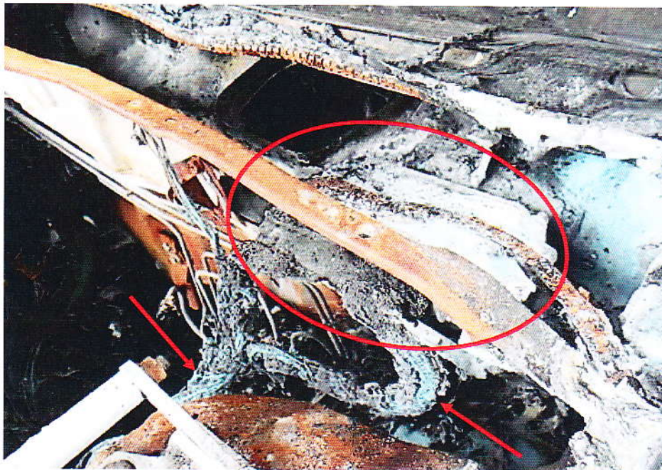
Photo 11 shows a closer view of the Engine Control Module (ECM) (circled). The wirings leading to this Engine Control Module (ECM) was found with greenish residue (arrowed) suggesting occurrence of an electrical short circuit.
