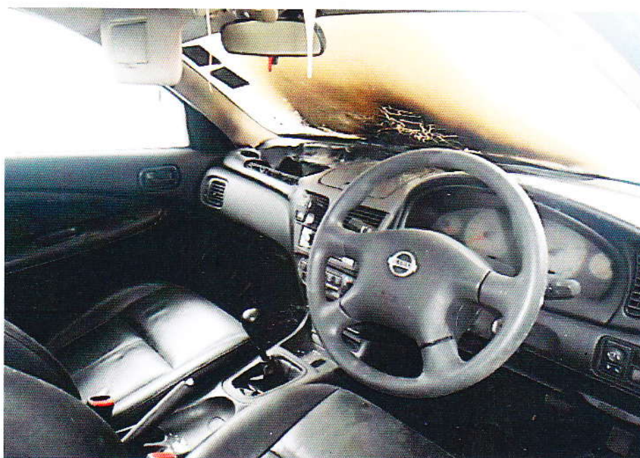
Photo 4 shows the interior compartment of the Insured Vehicle, which was observed to be partially burnt and/or melted. The front dashboard and roof upholstery were amongst the parts that were found to have been burnt and/or melted as a result of the fire.
