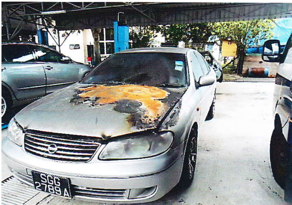
Photo 2 shows a general view of the front left portion of the Insured Vehicle at the time of my inspection. The fire damage to the Insured Vehicle was confined to its front portion. Its front bumper, front bonnet, front left headlamp and front left fender were amongst the body parts that were found to have been affected as a result of the fire.
