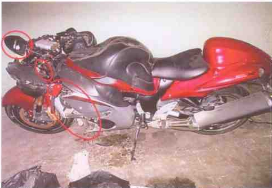
Photo 2 shows a general view of the left body of the Motorcycle at the time of our inspection. Body parts that were found to have been damaged include its left side mirror, clutch lever and left side cover.
