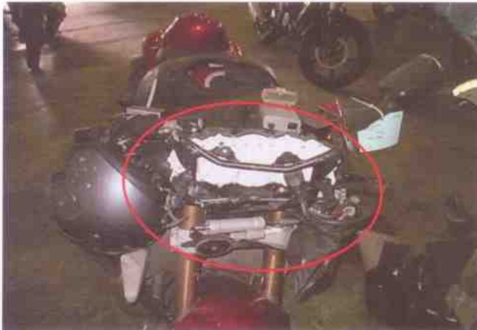
Photo 5 shows a closer view of the headlamp assembly and speedometer (circled) which were amongst the body parts at the front body of the Motorcycle that had sustained damage as a result of the accident.
