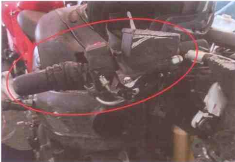
Photo 7 shows a close up view of the front brake lever, front brake reservoir, right handlebar grip and right handlebar end (circled) of the Motorcycle. These parts were amongst the body parts of the Motorcycle which were damaged as a result of the accident.
