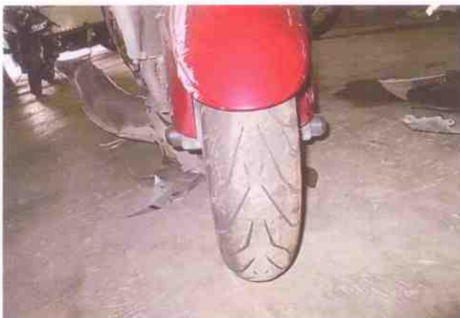
Photo 12 shows the condition of the Motorcycle's front tyre. The front tyre was observed to be in serviceable condition with remaining tread depth of approximately 2mm. The tyre was also observed to be sufficiently inflated for vehicular operation. We did not observe any tear, burst mark(s) and/or punctured hole(s) on the sidewalls as well as across the tread of the front tyre.
