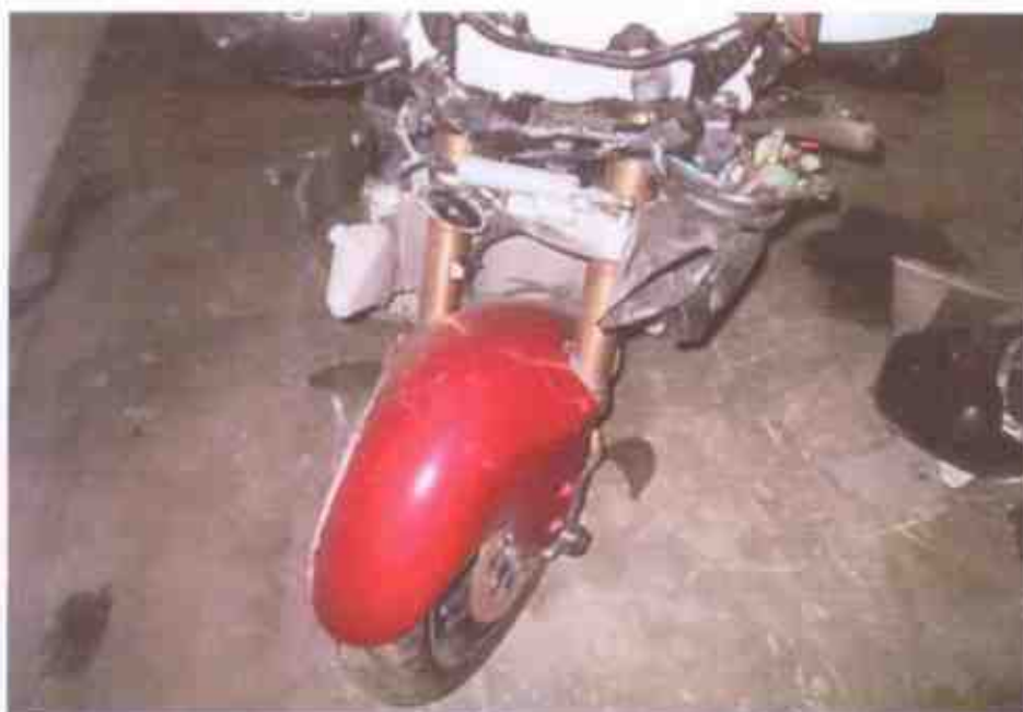
Photo 20 shows the front wheel of the Motorcycle turned towards its full right. Turning the Motorcycle's handlebars towards the left and right did not produce any abnormal free play and/or resistance. This would indicate that the steering system of the Motorcycle was in serviceable condition at the time of our inspection.
