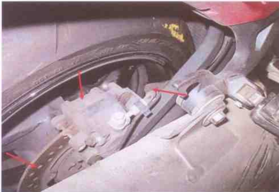
Photo 24 shows a close up view of the rear brake caliper, rear brake disc and rear brake hose (arrowed) of the Motorcycle, which are all part of the components in the hydraulic rear brake system of the Motorcycle. Our visual checks of these various components revealed all to be intact with no visible damage. No leakage of brake fluid was also observed.
