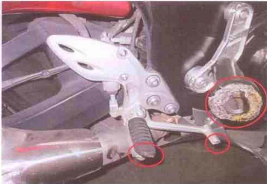
Photo 13 shows the damaged right frame slider, rear brake pedal and right side rider footrest (circled) of the Motorcycle. The damages sustained to these parts were mainly of grazing nature.
