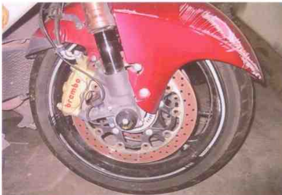
Photo 11 shows the front wheel rim and tyre of the Motorcycle at the time of our inspection. The front tyre was observed to be in serviceable condition and sufficiently inflated for vehicular operation. There was no visible damage observed on the front wheel rim.
