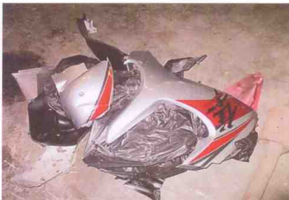
Photo 4 shows a closer view of the damaged headlamp assembly, left side cover and right side cover of the Motorcycle at the time of our inspection.
