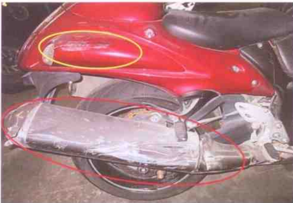
Photo 14 shows the damaged rear right side cover and right exhaust muffler (circled) of the Motorcycle as a result of the accident.
