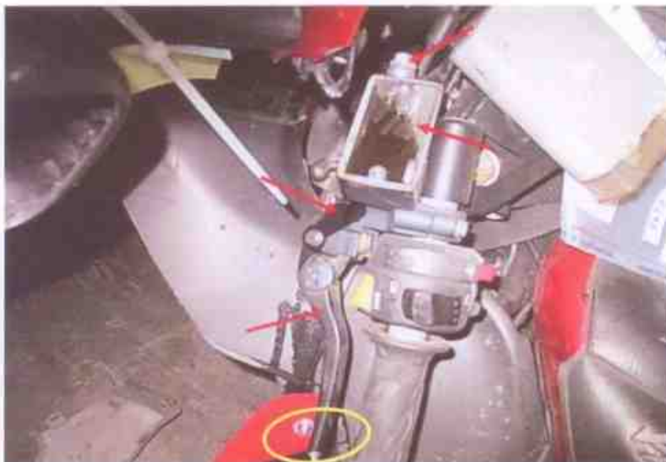
Photo 21 shows a close up view of the clutch pump, clutch lever, clutch fluid reservoir and clutch hose (arrowed) of the Motorcycle, which are all part of the components in the hydraulic clutch system of the Motorcycle. Our visual checks of these various components revealed all to be intact with no visible damage except for the clutch lever. The hydraulic clutch fluid was observed to be of sufficient level and without contamination for operational purposes. No leakage of clutch fluid was also observed. We were unable to carry out an operational test of the Motorcycle's hydraulic clutch system due to the damage sustained to the clutch lever (circled).
