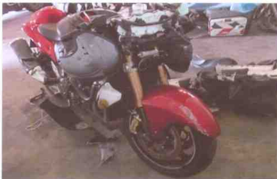
Photo 3 shows a general view of the right body of the Motorcycle at the time of our inspection. Body parts that were found to have been damaged include its headlamp assembly, speedometer, front mudguard, right side mirror, front brake lever, front brake reservoir, right front fork slider, petrol tank, right side cover, right frame slider, rear brake pedal, right exhaust muffler, rear right side cover and right rear axle slider amongst others.
