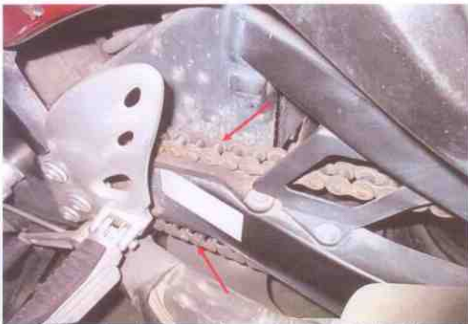
Photo 19 shows the closer view of the gear chain (arrowed) of the Motorcycle, which was observed to be intact with no misalignment. It was also adequately lubricated for operating purposes.
