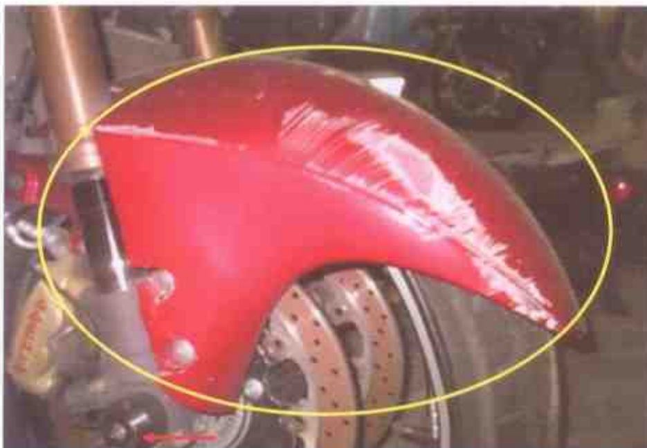
Photo 6 shows a closer view of the front mudguard (circled) and right front fork slider (arrowed), which were amongst the body parts at the front body of the Motorcycle that had sustained damage as a result of the accident.
