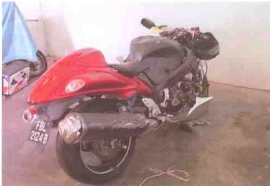
Photo 1 shows a general view of the rear right body of the Motorcycle at the time of our inspection. The Motorcycle had sustained damages all around, significantly at its front portion and right body. The mileage of the Motorcycle was not recorded at the time of our inspection due to the damage sustained to the odometer display screen as a result of the accident.
