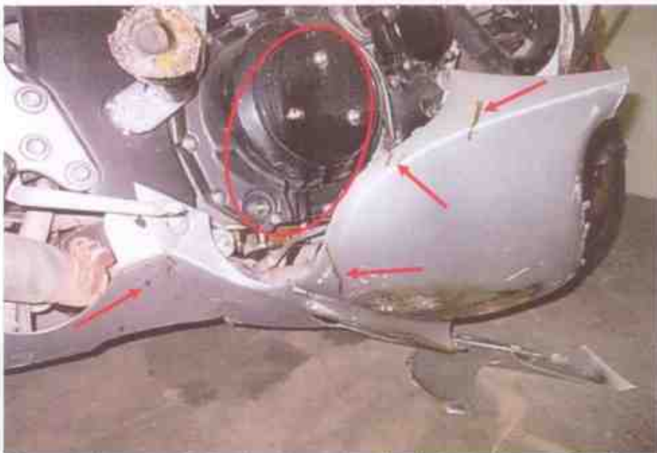
Photo 17 shows wet fluid stains observed on the clutch plate cover (circled) and damaged right side cover (arrowed) of the Motorcycle, indicating that the fluid leak had occurred as a result of the accident.
