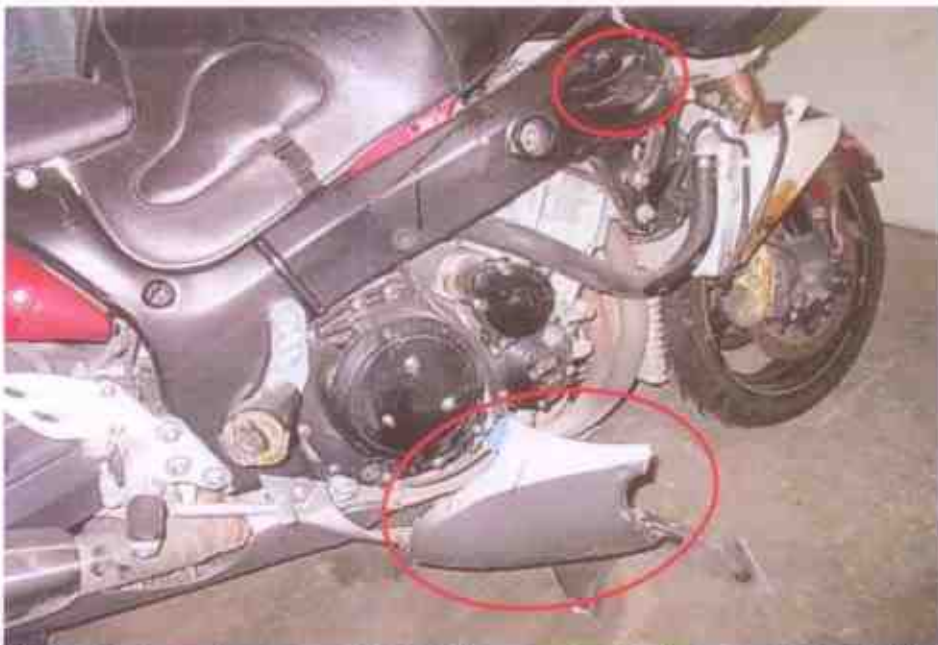
Photo 10 shows the damaged right side cover and right frame (circled) of the Motorcycle. The damage sustained at the right frame of the Motorcycle was mainly of grazing nature.
