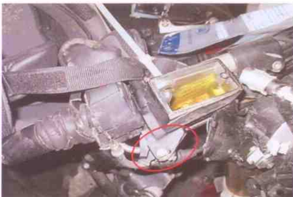
Photo 23 shows the brake fluid reservoir for the front brake of the Motorcycle. The brake fluid was observed to be of sufficient level and without contamination for operational purposes. We were unable to carry out an operational test of the Motorcycle's front braking system due to the damage sustained to the front brake lever (circled).
