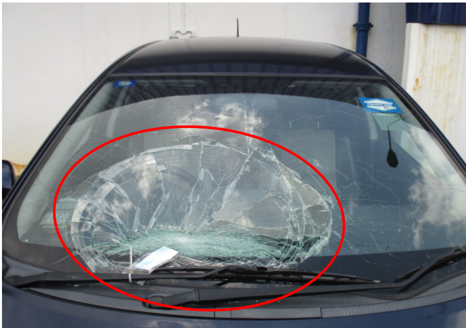
Photo 3 shows a general view of the Motor Car's front windscreen at the time of our inspection. The right side of the front windscreen of the Motor Car was observed to be cracked (circled).
