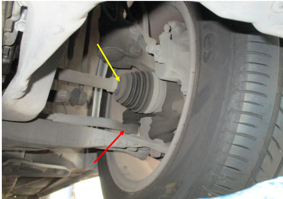
Photo 18 shows the various undercarriage components at the front left wheel of the Motor Car, which had included the steering tie rod (red arrow) and left drive shaft (yellow arrow). The various undercarriage components of the Motor Car were all found to be intact without any visible damage. There was also no sign of fluid stain observed on the various undercarriage components.
