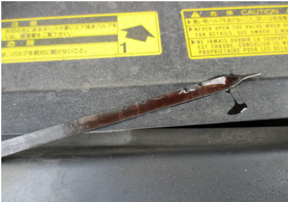
Photo 14 shows the ATF dipstick of the Motor Car at the time of our inspection. The ATF was observed to be of sufficient level and without any visible contamination.
