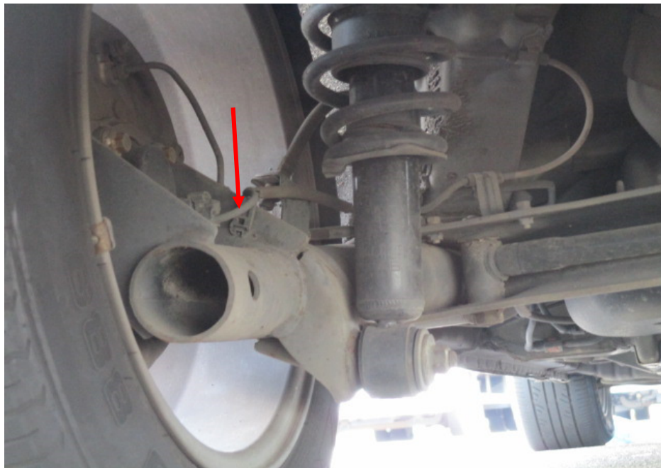
Photo 15 shows the brake hose (arrowed) at the rear left wheel of the Motor Car. We did not observe any leakage of brake fluid at the time of our inspection of the Motor Car. Our visual inspection of the various mechanical components of the Motor Car's braking system revealed all to be intact and without visible damage, indicating that the braking system was likely to be in serviceable condition at the material time of accident.
