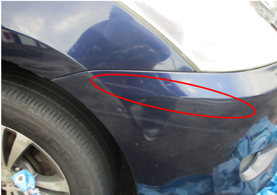
Photo 4 shows a general view of the Motor Car's right front body at the time of our inspection. The Motor Car was observed to be in good general condition. Its front bumper was however observed to be scratched at the right side (circled).
