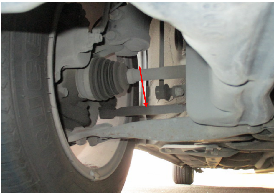
Photo 17 shows the various undercarriage components at the front right wheel of the Motor Car, in particular the steering tie rod (arrowed). The various steering components were all found to be intact, suggesting that the steering system of the Motor Car was likely to be in serviceable condition.
