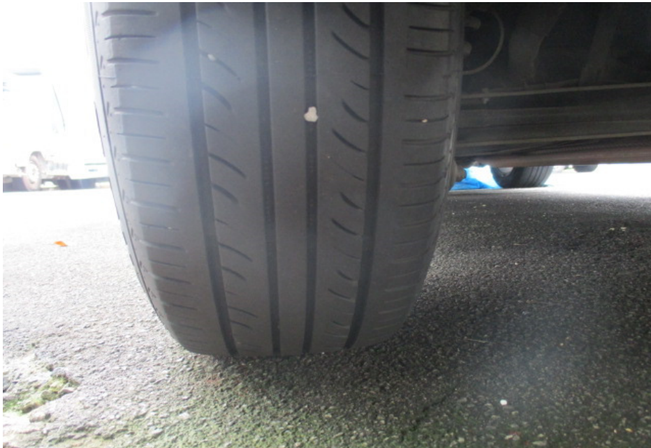
Photo 8 shows the condition of the rear left tyre of the Motor Car, which was observed to be in serviceable condition with remaining tread depth of approximately 4mm. The tyre, which was wrapped around alloy wheel rim, was also observed to be sufficiently inflated for vehicular operation. There was also no significant damage found on the 4 wheel rims of the Motor Car except for some marks of grazing nature on the outer spokes of all the wheel rims.
