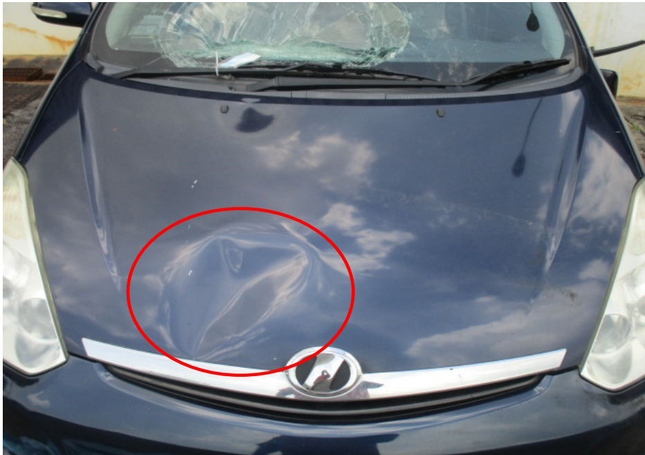
Photo 2 shows a general view of the front bonnet of the Motor Car at the time of our inspection. The Motor Car was observed to be in good general condition. Its front bonnet was however observed to be dented at the right side (circled).
