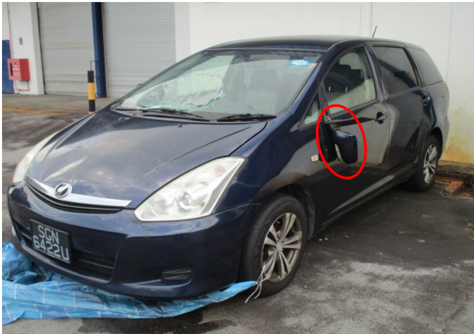
Photo 5 shows a general view of the Motor Car's left front body at the time of our inspection. The Motor Car was observed to be in good general condition. Its left side mirror was however observed to be dislodged (circled).
