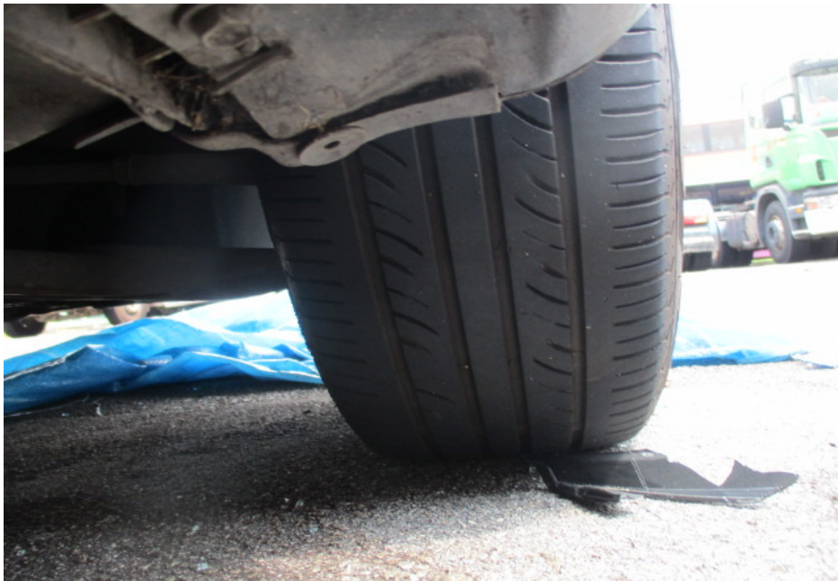
Photo 7 shows the condition of the front right tyre of the Motor Car, which was observed to be in serviceable condition with remaining tread depth of approximately 4mm. The tyre, which was wrapped around alloy wheel rim, was also observed to be sufficiently inflated for vehicular operation.
