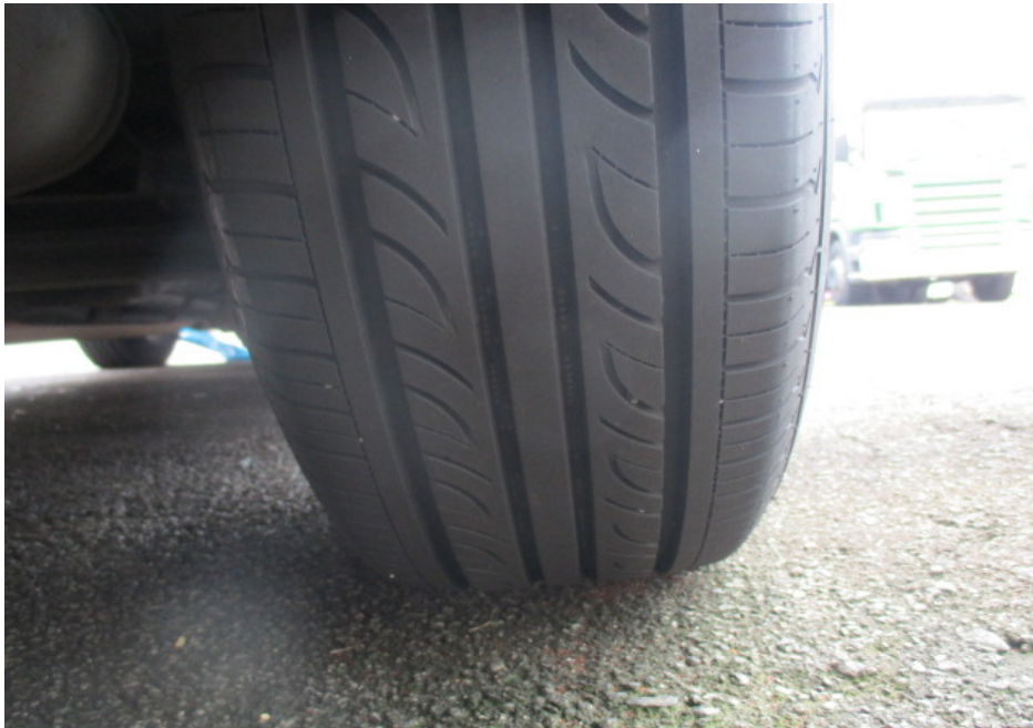
Photo 9 shows the condition of the rear right tyre of the Motor Car, which was observed to be in serviceable condition with remaining tread depth of approximately 7mm. There was also no tear, cut or burst mark(s) on the outer and the inner sidewalls as well as across the tread of the 4 tyres.
