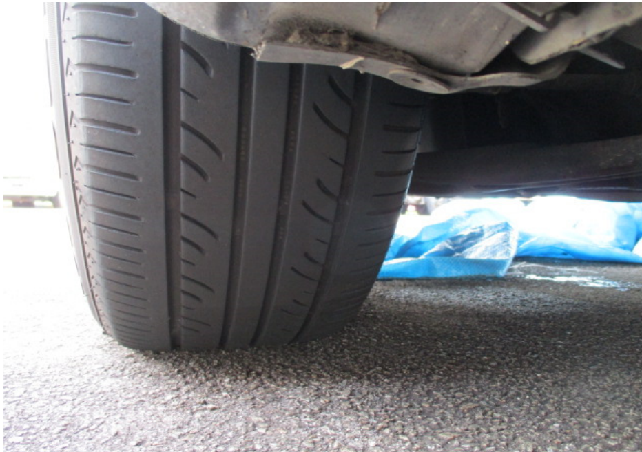
Photo 6 shows the condition of the front left tyre of the Motor Car, which was observed to be in serviceable condition with remaining tread depth of approximately 4mm. The tyre, which was wrapped around alloy wheel rim, was also observed to be sufficiently inflated for vehicular operation. There was no tear, cut or burst mark(s) on the outer and the inner sidewalls as well as across the tread of the 4 tyres.
