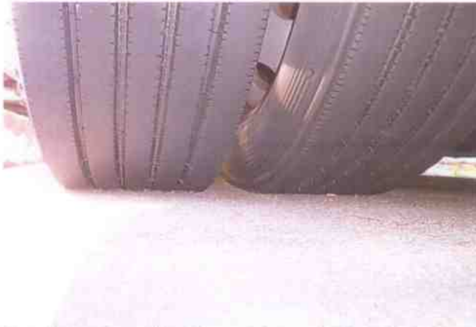
Photo 14 shows the condition of the rear right tyres of the Motor Bus, which were observed to be in serviceable condition with remaining tread depth of approximately 11mm. The tyres, which were wrapped around standard alloy wheels rims, were also observed to be sufficiently inflated for vehicular operation.
