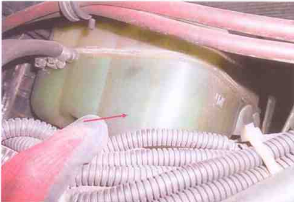
Photo 19 shows the engine coolant of the Motor Bus. It was observed to be of sufficient level without any contamination at time of our inspection.
