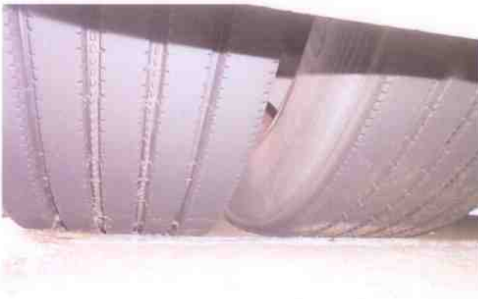
Photo 14 shows the condition of the rear right tyres of the Motor Bus, which were observed to be in serviceable condition with remaining tread depth of approximately 11mm. The tyres, which were wrapped around standard alloy wheels rims, were also observed to be sufficiently inflated for vehicular operation.
