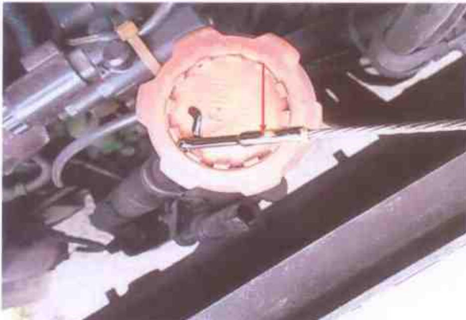
Photo 18 shows the engine fluid of the Motor Bus. It was observed to be of sufficient level without any contamination at time of our inspection.
