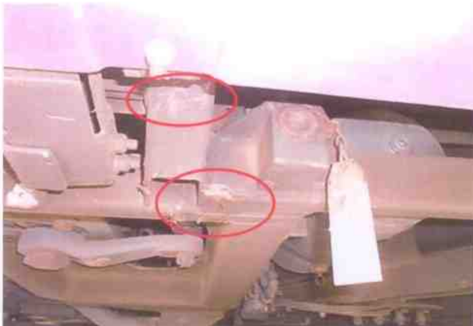
Photo 8 shows a close-up view of the Motor Bus's front undercarriage area. It was observed to have sustained with minor scratches likely due to the accident's impact.
