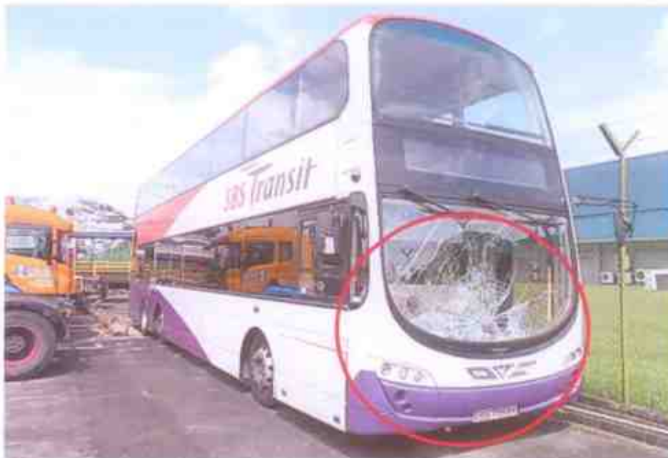
Photo 2 shows a general view of the front right body of the Motor Bus at the time of our inspection. The Motor Bus was observed to have sustained relatively minor damage at its front body. Its windshield was observed to be cracked.
