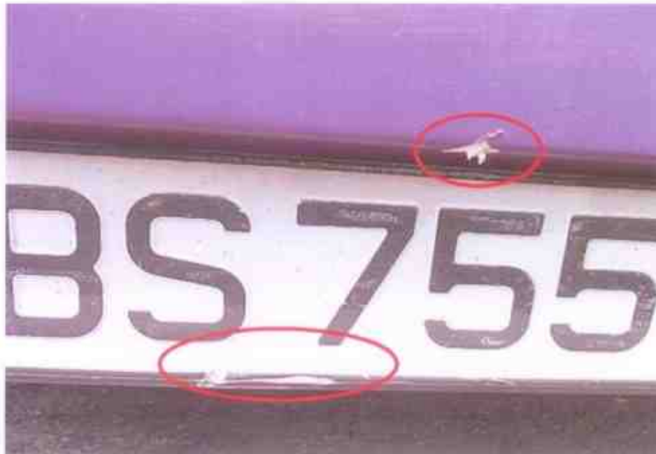
Photo 7 shows a close-up view of the Motor Bus's number plate area. It was observed to have sustained with minor scratches likely due to the accident's impact.
