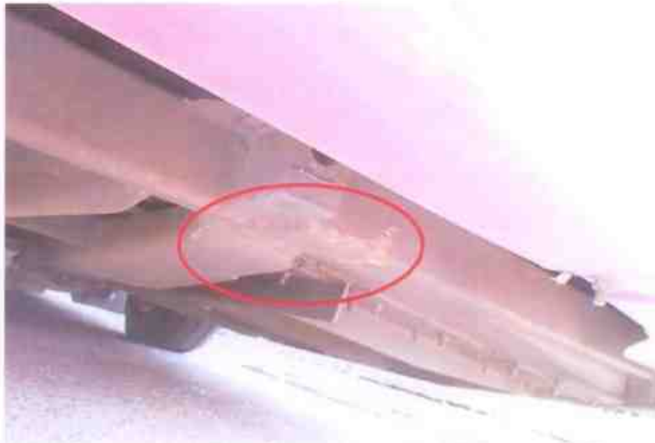
Photo 9 shows a close-up view of the Motor Bus's front undercarriage area. It was observed to have sustained with minor scratches likely due to the accident's impact
