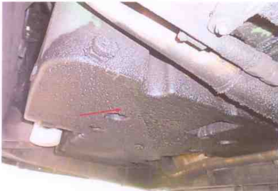
Photo 20 shows the engine underside of the Motor Bus. It was observed to be sighted with fluid leakage. However it was noted to be a pre-existed fluid leakage due to the dust stain that associated with it.
