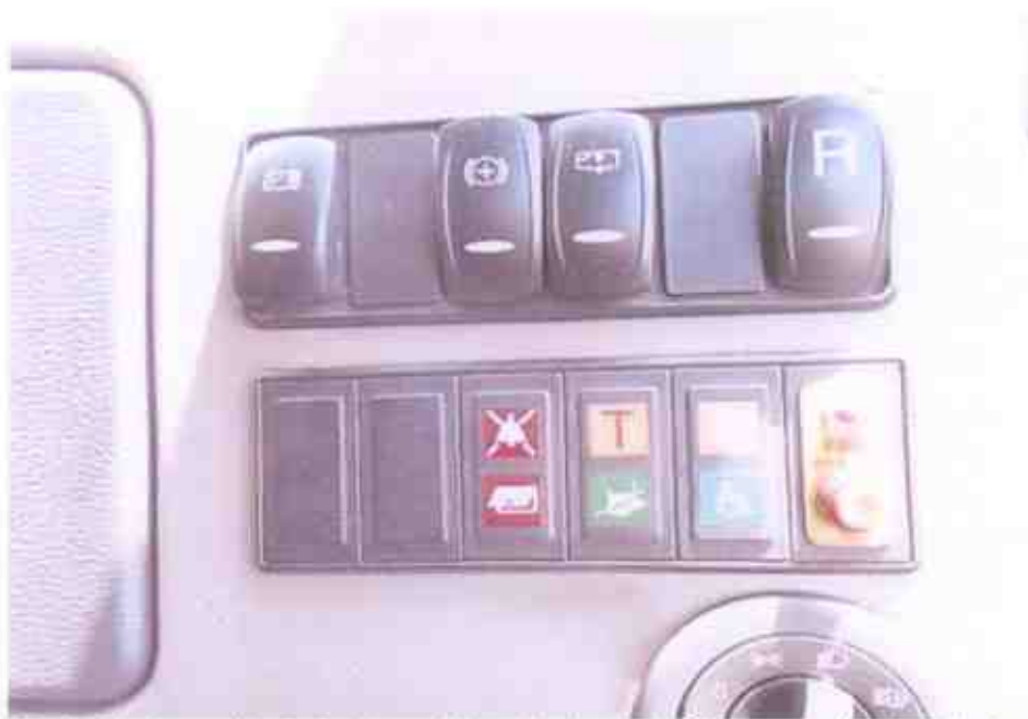
Photo 25 shows the indicators at the driver's seat. Other operational indicators were unable to be initialized due to the flat battery. Hence, no test was carried out to the Motor Bus additional devices.
