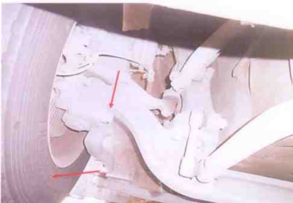
Photo 23 shows the undercarriage components at the front left wheel of the Motor Bus. The various undercarriage components of the Motor Bus were all observed to be intact and without any visible damage. This had included the steering rack and steering ball joints (arrowed) of the Motor Bus, which were observed to be securely attached to the front left wheel and front right wheel.
