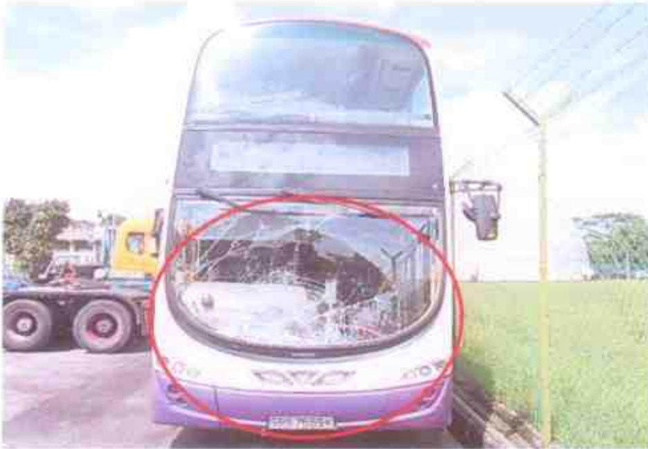
Photo 1 shows a general view of the front body of the Motor Bus at the time of our inspection. The Motor Bus was observed to have sustained relatively minor damage at its front body. Its windshield was observed to be cracked.
