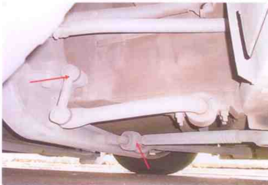
Photo 21 shows some of the mechanical components (arrowed) of the Motor Bus's steering system. Our visual checks on the various mechanical components of the steering system revealed all to be intact and in good condition. The steering system of the Motor Bus is hence likely to be in serviceable condition at the time of accident.
