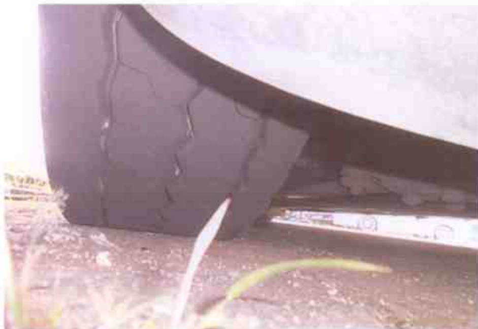
Photo 13 shows the condition of the rear left tyres (centre axle) of the Motor Bus, which were observed to be in serviceable condition with remaining tread depth of approximately 10mm. The tyres, which were wrapped around standard alloy wheel rims, were also observed to be sufficiently inflated for vehicular operation.
