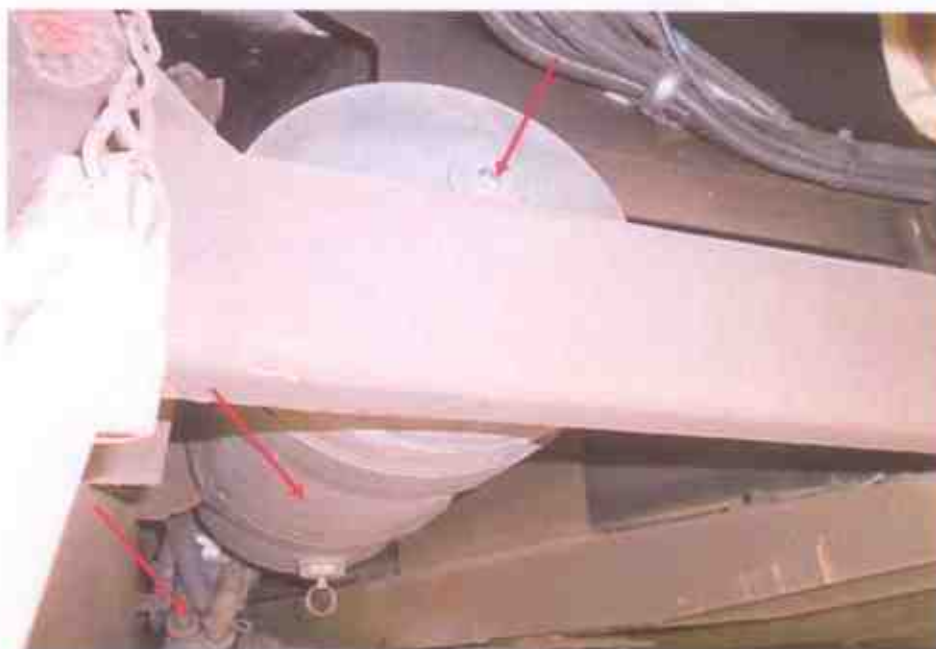
Photo 24 shows a general view of the air tank, valves, pipes and hoses, which are some of the components for the air-assisted braking system of the Motor Bus. This was at the underside of the Motor Bus's front right body. We were however not able to carry out any operational test(s) to the braking system of the Motor Bus as its engine was unable to be started.
