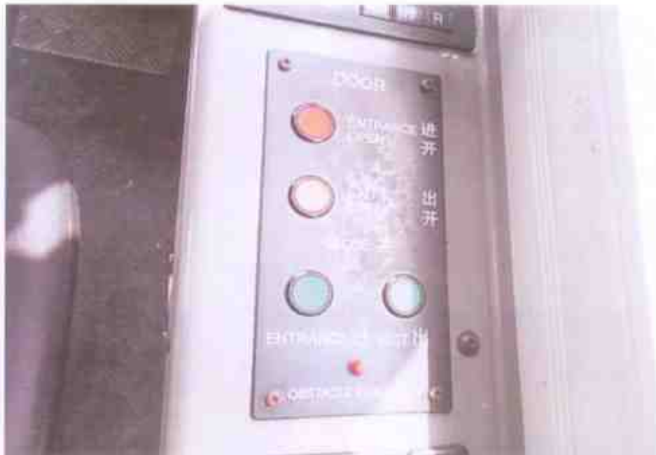
Photo 26 shows the indicators at the driver's seat. Other operational indicators were unable to be initialized due to the flat battery. Hence, no test was carried out to the Motor Bus additional devices.
