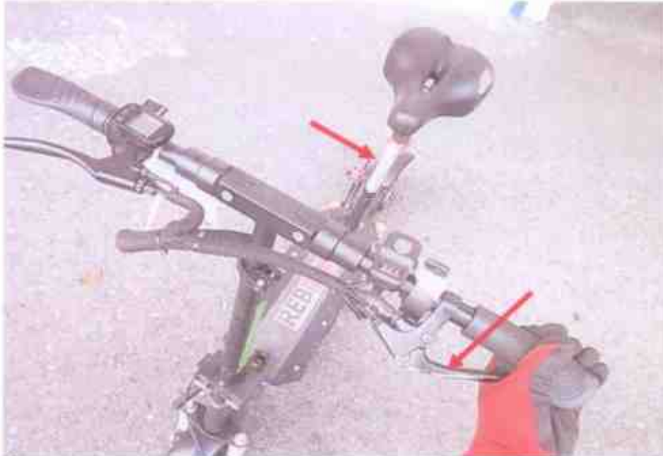
Photo 13 shows a static brake test was conducted only on the Bicycle's rear brake. The test was conducted by lifting the rear tyre above ground & applies a little spinning action to it. The hand brake lever was then gripped in order to stop the spinning front tyre. The result was unsatisfactory. It didn't stop after gripping the left hand brake to the fullest. It shows that the rear brake clamps was not responding to the gripping action. This had appeared to indicate that the rear brake was not in a serviceable condition.
