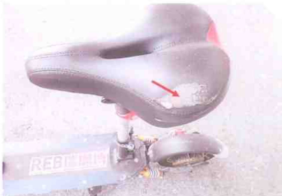
Photo 7 shows the seat of the Electric Scooter at time of inspection. Damage on the right portion of the seat was observed likely due to the accident.
