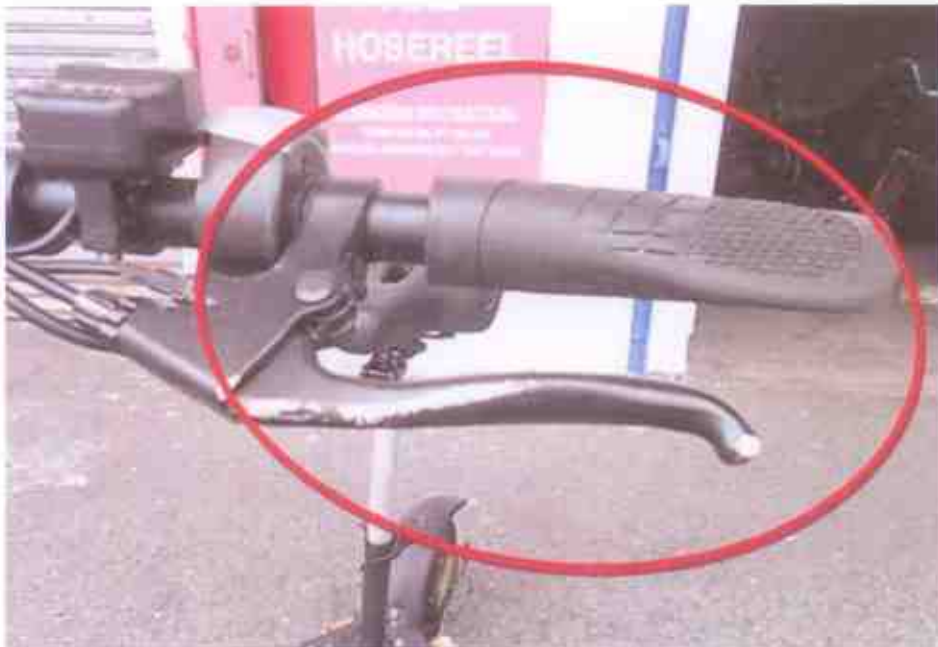
Photo 6 shows the left portion of the Electric Scooter at time of inspection. Damage on the left hand handle & brake lever was observed likely due to the accident.
