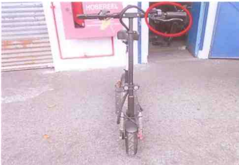
Photo 2 shows the frontal portion of the Electric Scooter at time of inspection. Damage on the left hand handle, left hand portion of the seat & right hand brake lever was observed likely due to the accident.
