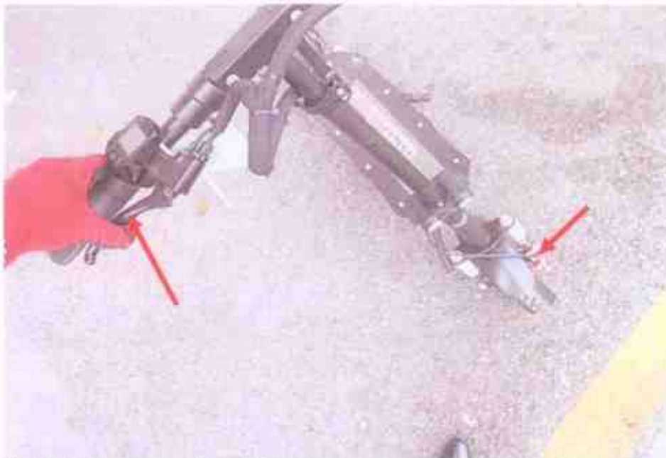
Photo 14 shows a static brake test was conducted only on the Bicycle's front brake. The test was conducted by lifting the front tyre in the air & applies a little spinning action to it. The hand brake lever was then gripped in order to stop the spinning front tyre. The result was satisfactory. It stops after gripping the hand brake to the fullest.
