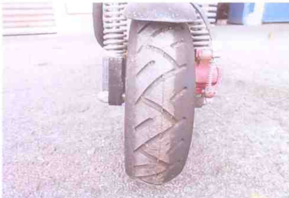
Photo 9 shows the front tyre of the Electric Scooter at the time of our inspection. The tread pattern of the 2 tyres was clearly visible. We did not observe any tear, burst mark(s) and/or punctured hole(s) on the sidewalls.
