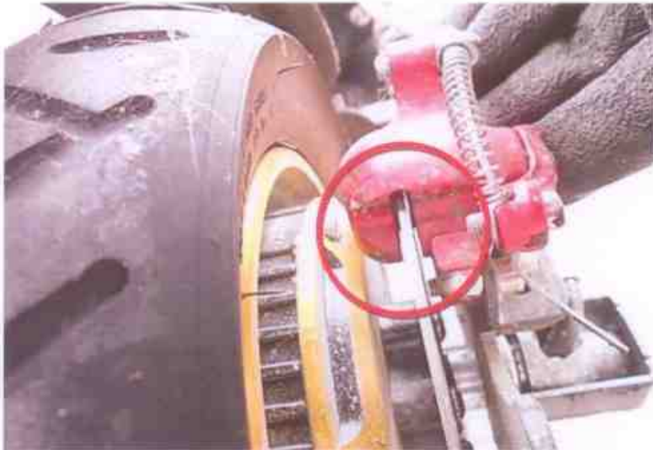
Photo 12 shows the close-up view of the rear brake calliper (circled) of the Electric Scooter, which was observed to be intact with no damages.
