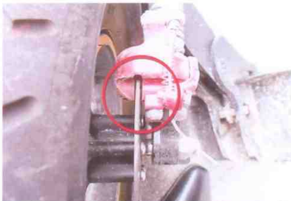
Photo 11 shows the close-up view of the front brake calliper (circled) of the Electric Scooter, which was observed to be intact with no damages.
