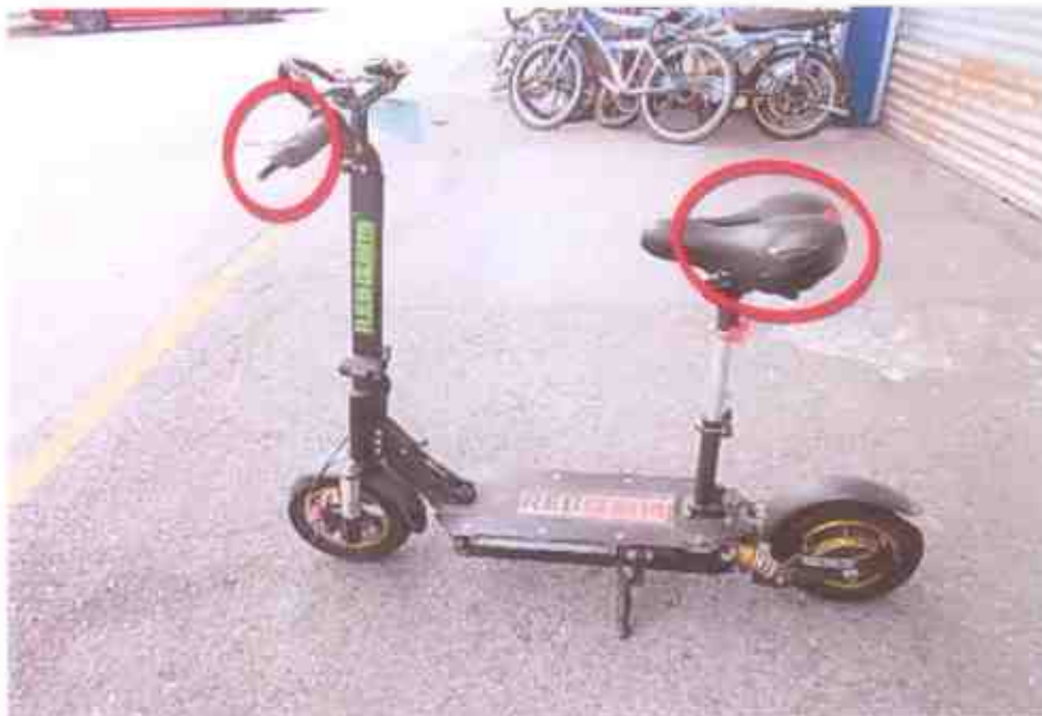
Photo 4 shows the left portion of the Electric Scooter at time of inspection. Damage on the left hand handle, left hand portion of the seat & right hand brake lever was observed likely due to the accident.
