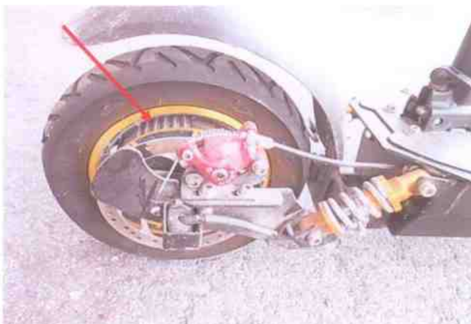
Photo 10 shows the general view of the drive motor (arrowed) of the Electric Scooter, which was observed to be intact with no misalignment.
